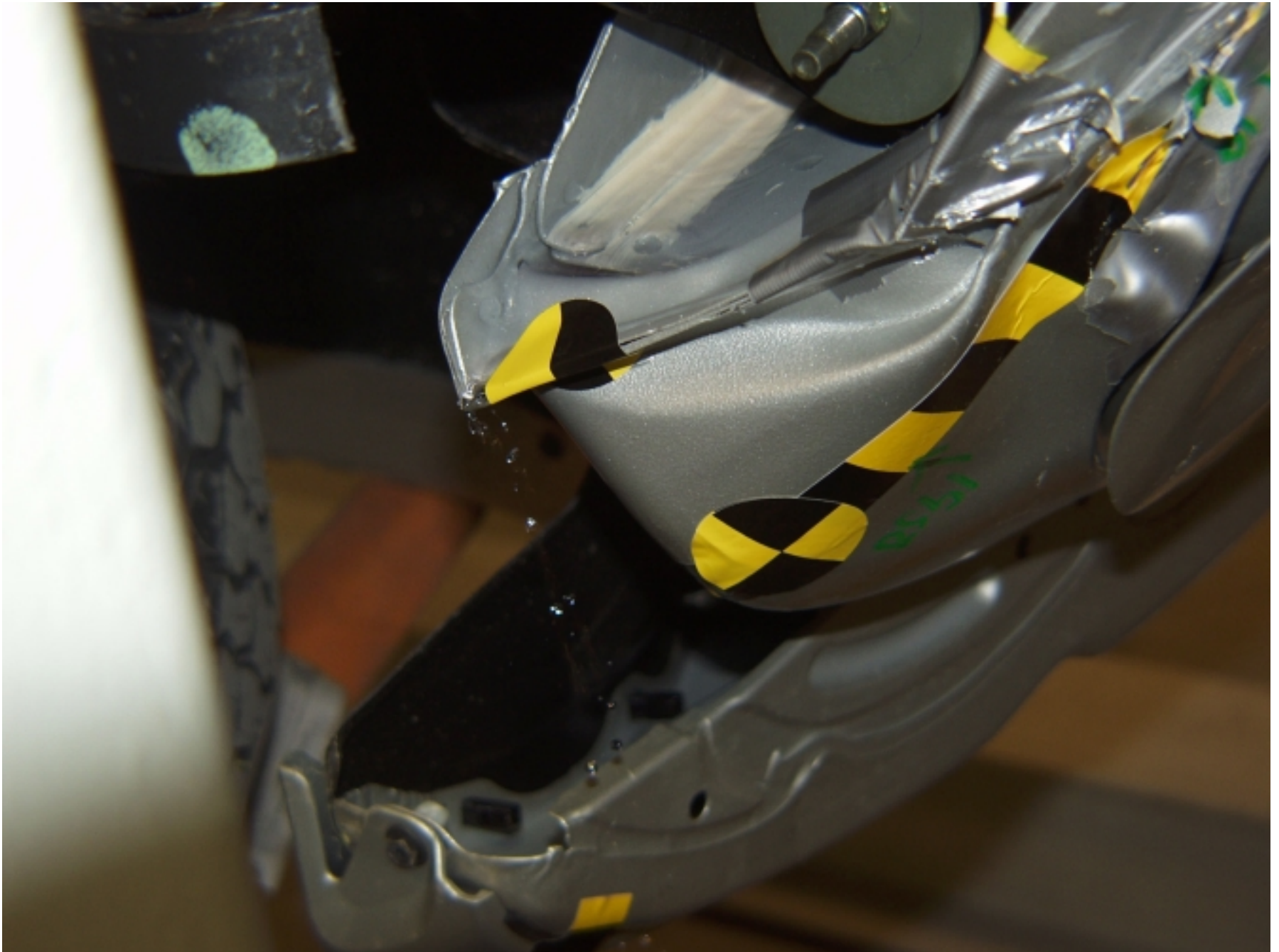
Figure A-45: STODDARD LEAK @ 90 DEGREES
