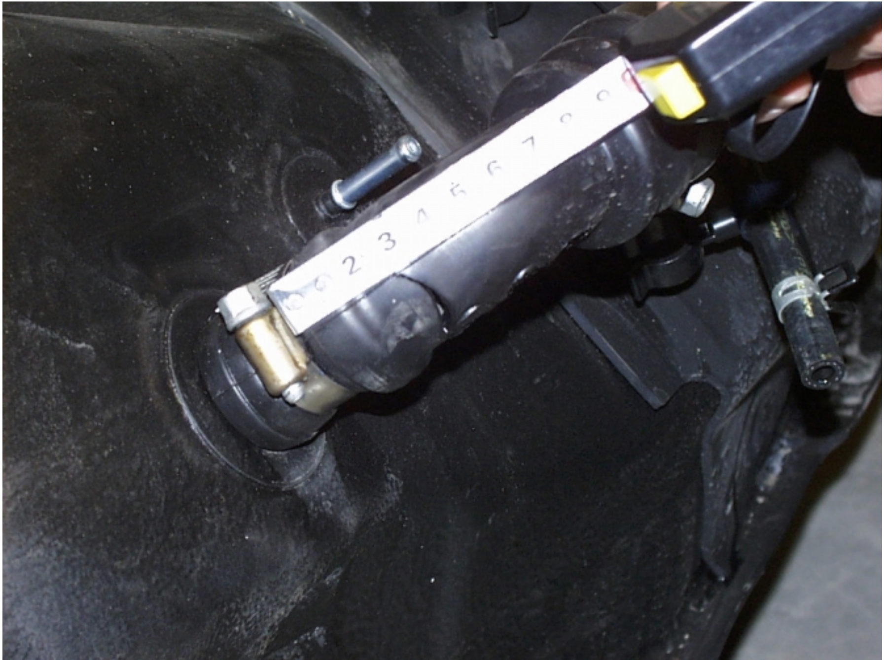
Figure A-47: HOLE IN FILLER NECK
