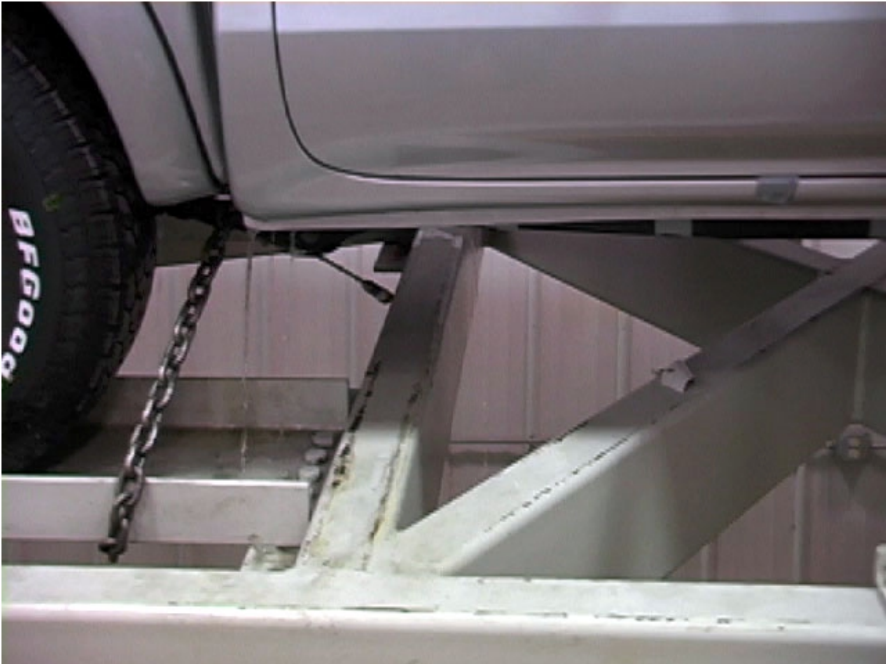
Figure A-46: STODDARD LEAK 270-360 DEGREE ROLL
