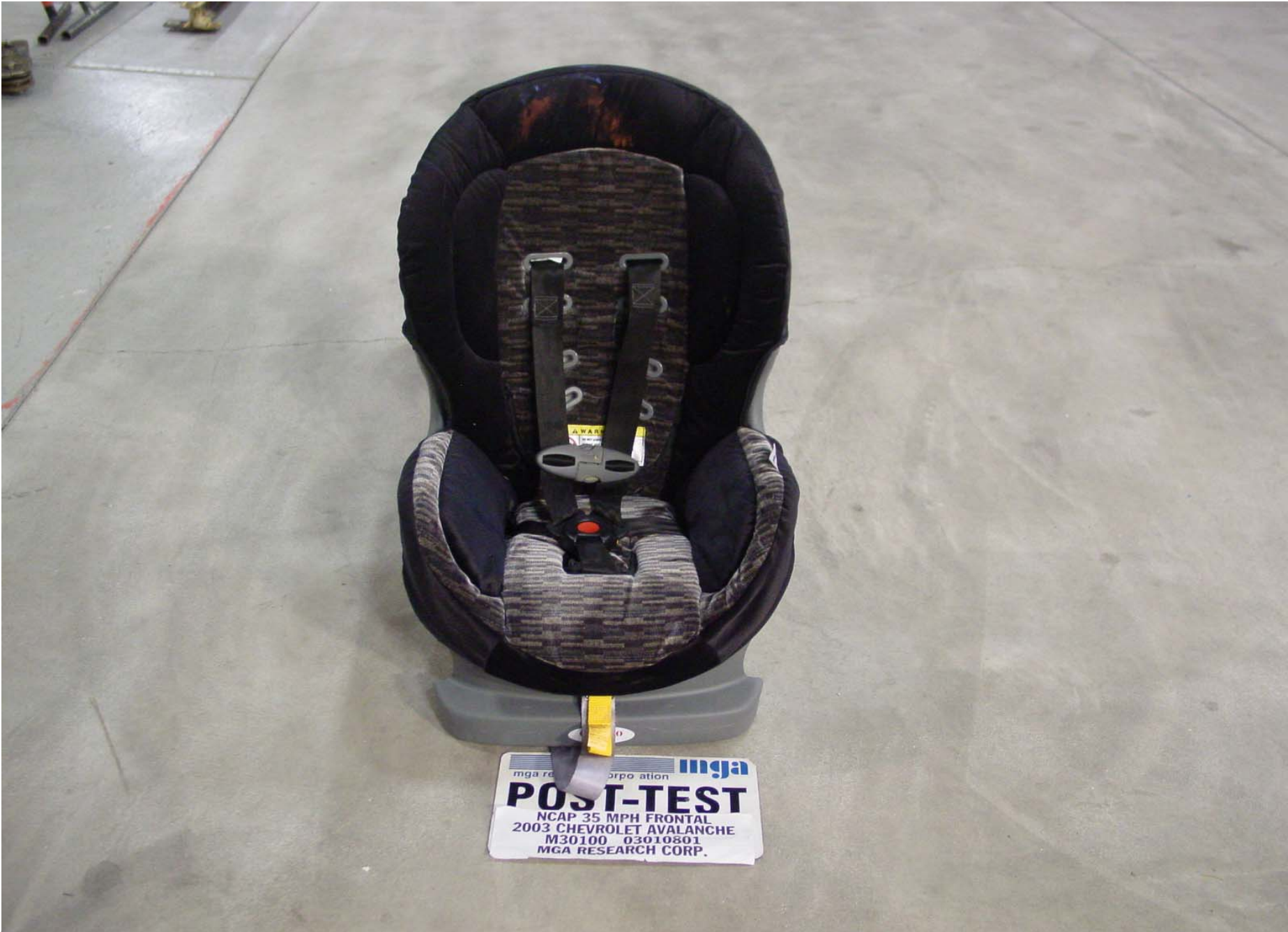
Post-Test Front View of Position 3 CRS
