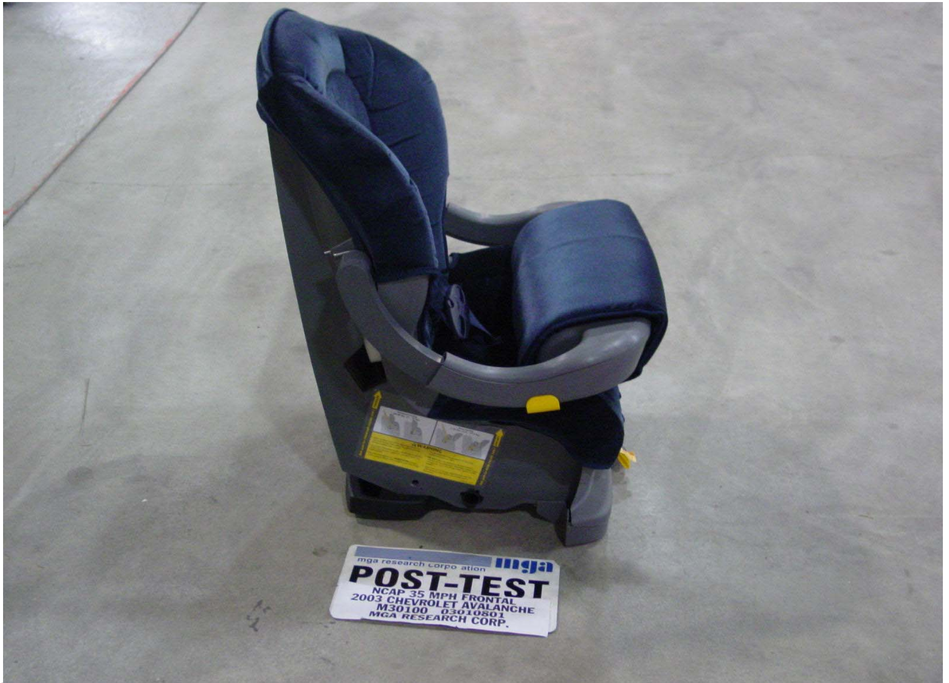
Post-Test Right Side View of Position 4 CRS
