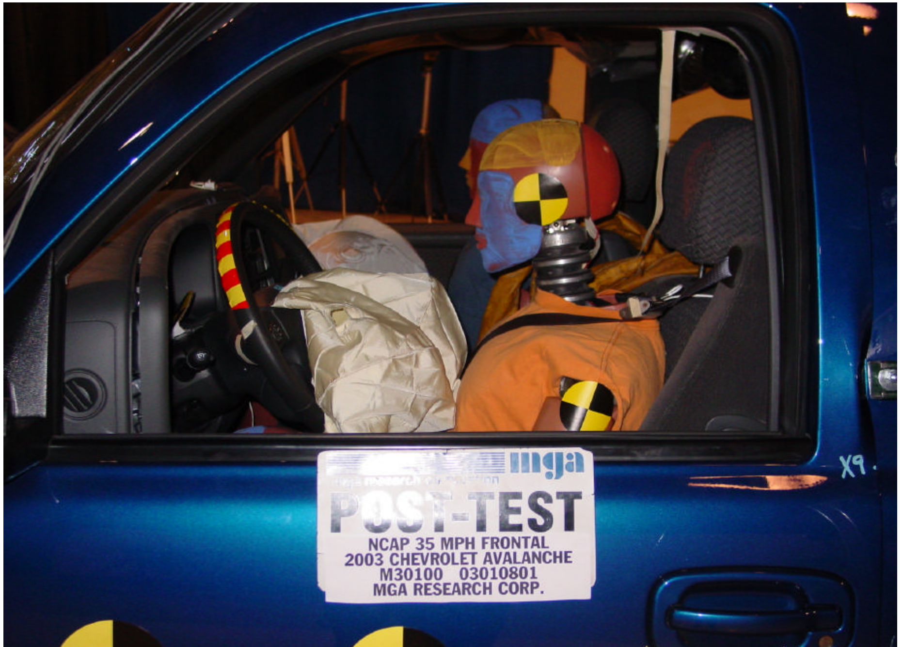
Post-Test Driver Dummy Position Left Side View
