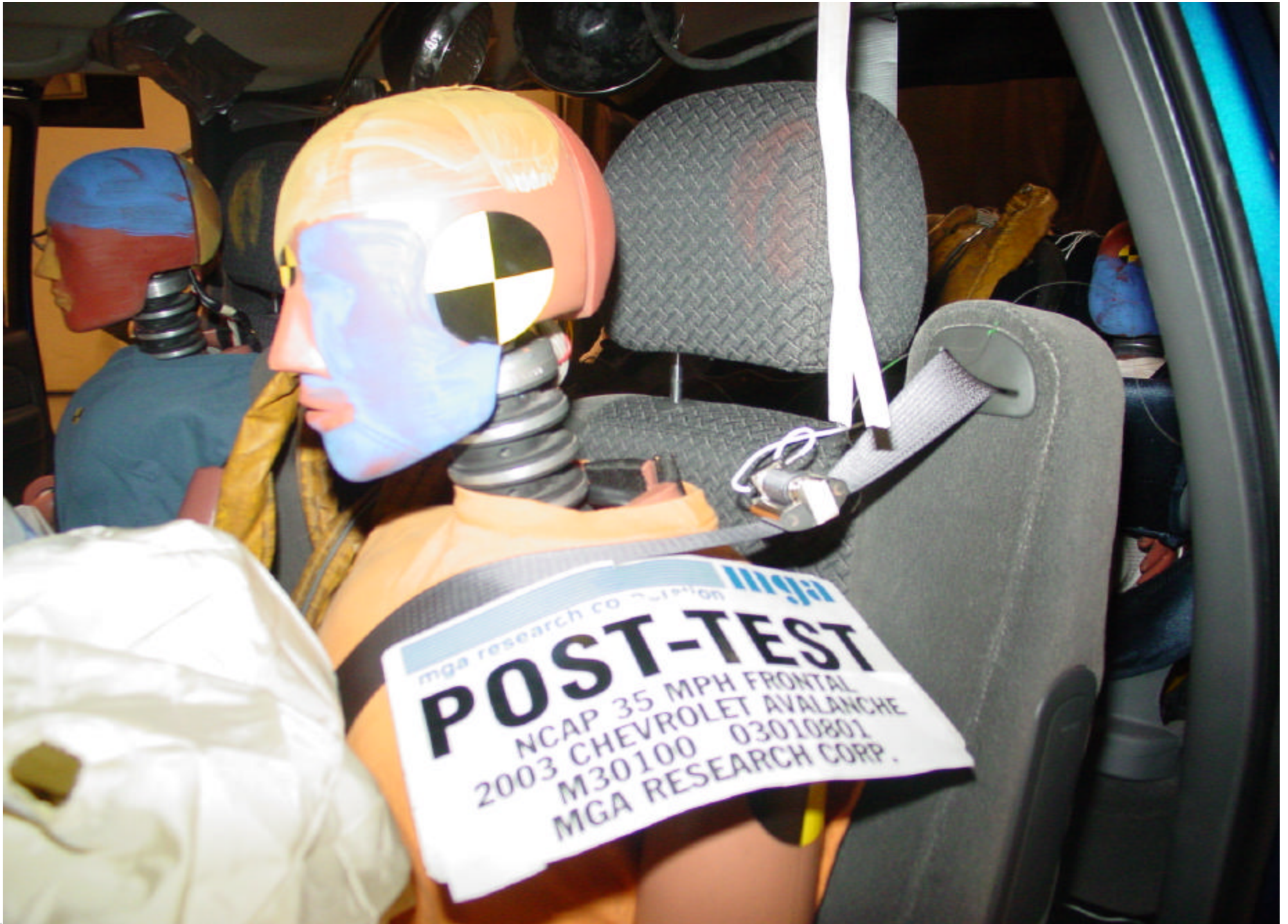
Post-Test Driver Dummy Head Contact
