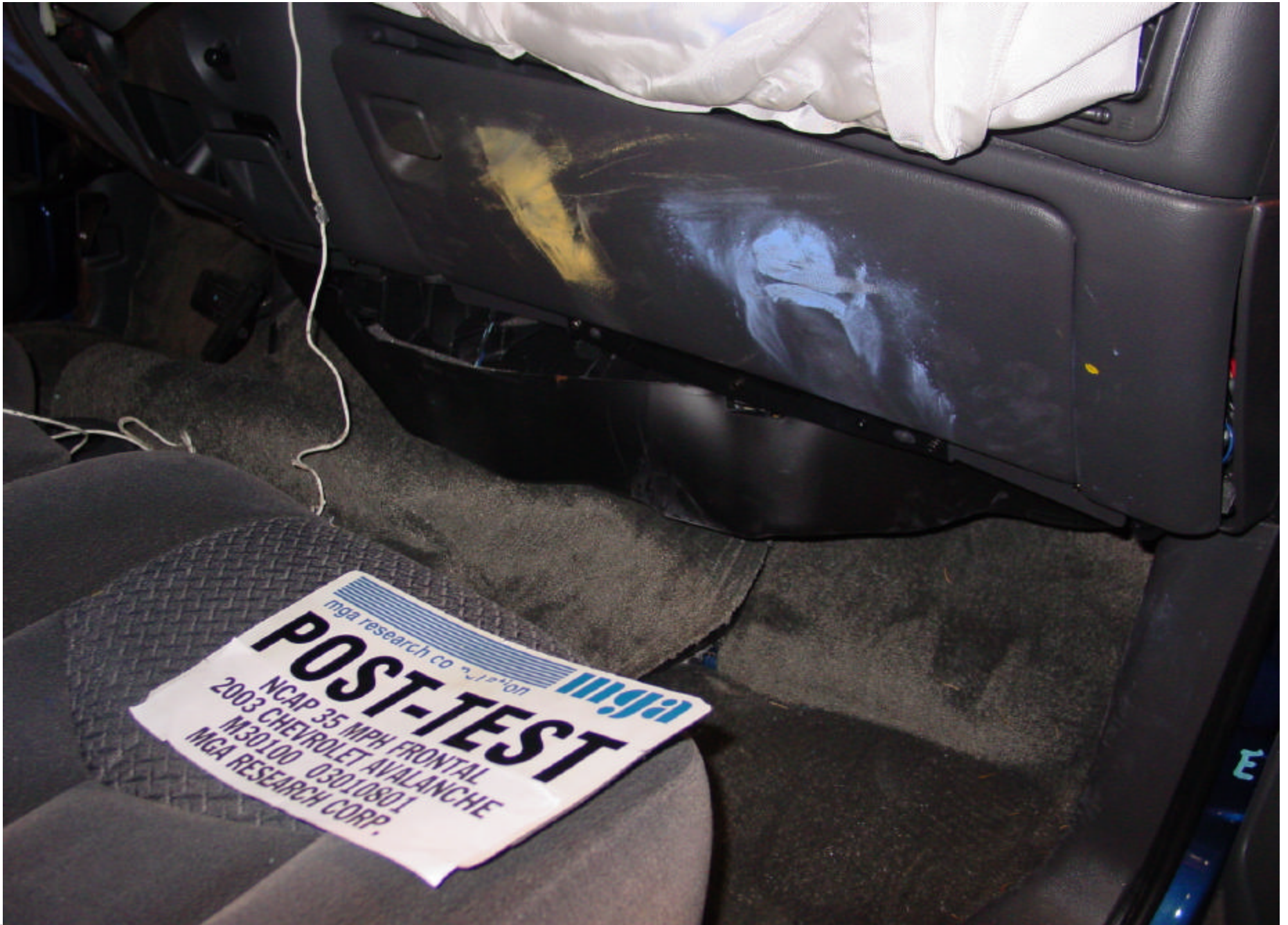
Post-Test Passenger Dummy Knee Contact
