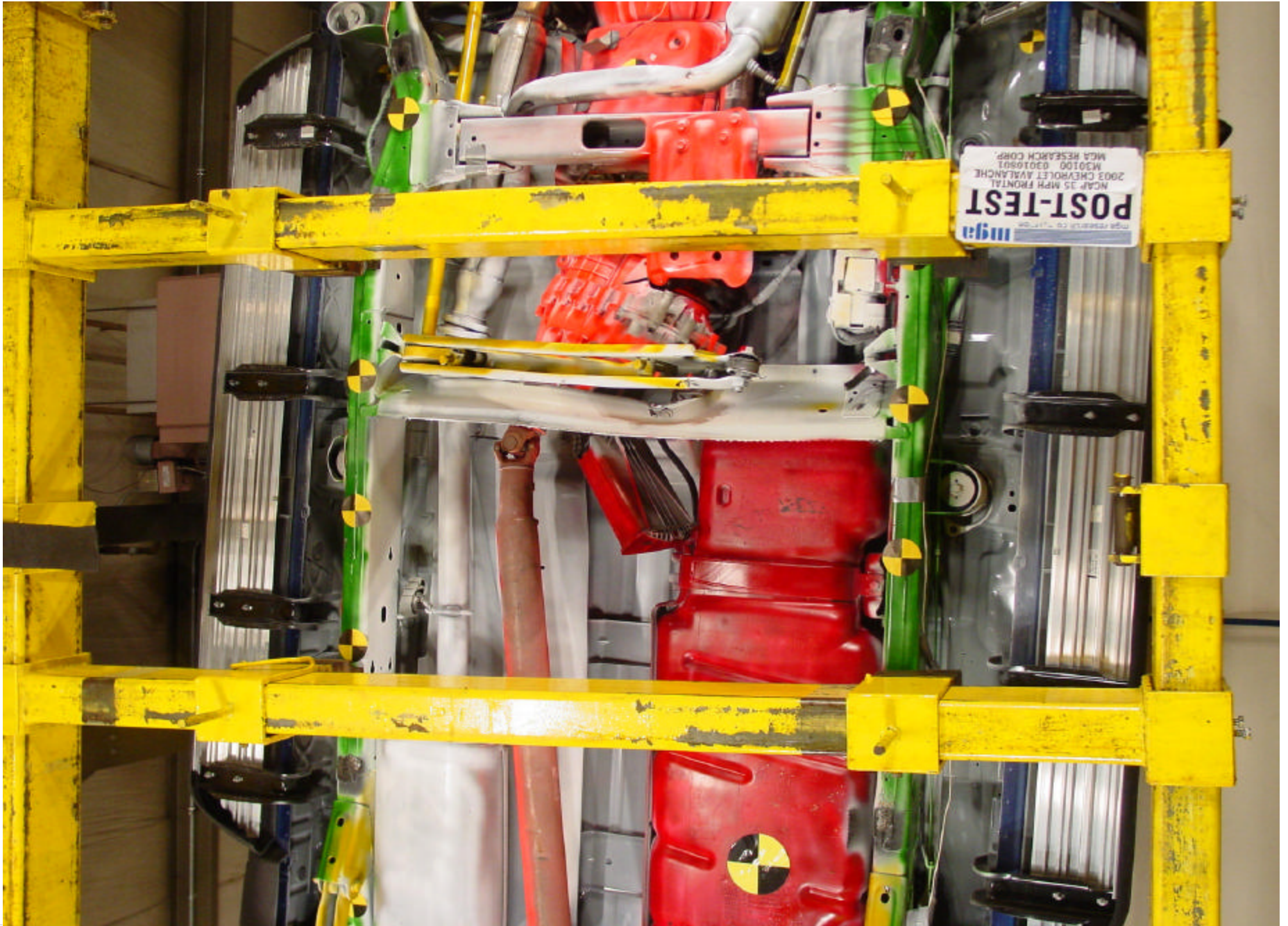
Post-Test Mid Underbody
