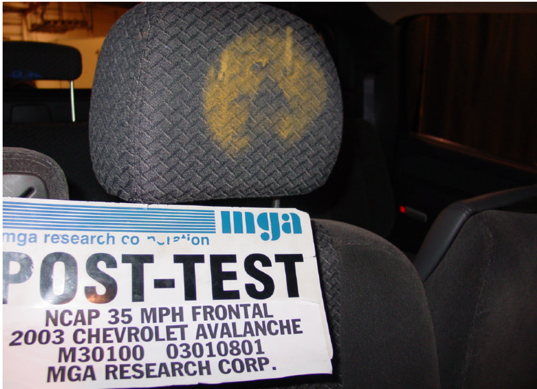
Post-Test Passenger Dummy Head Contact
