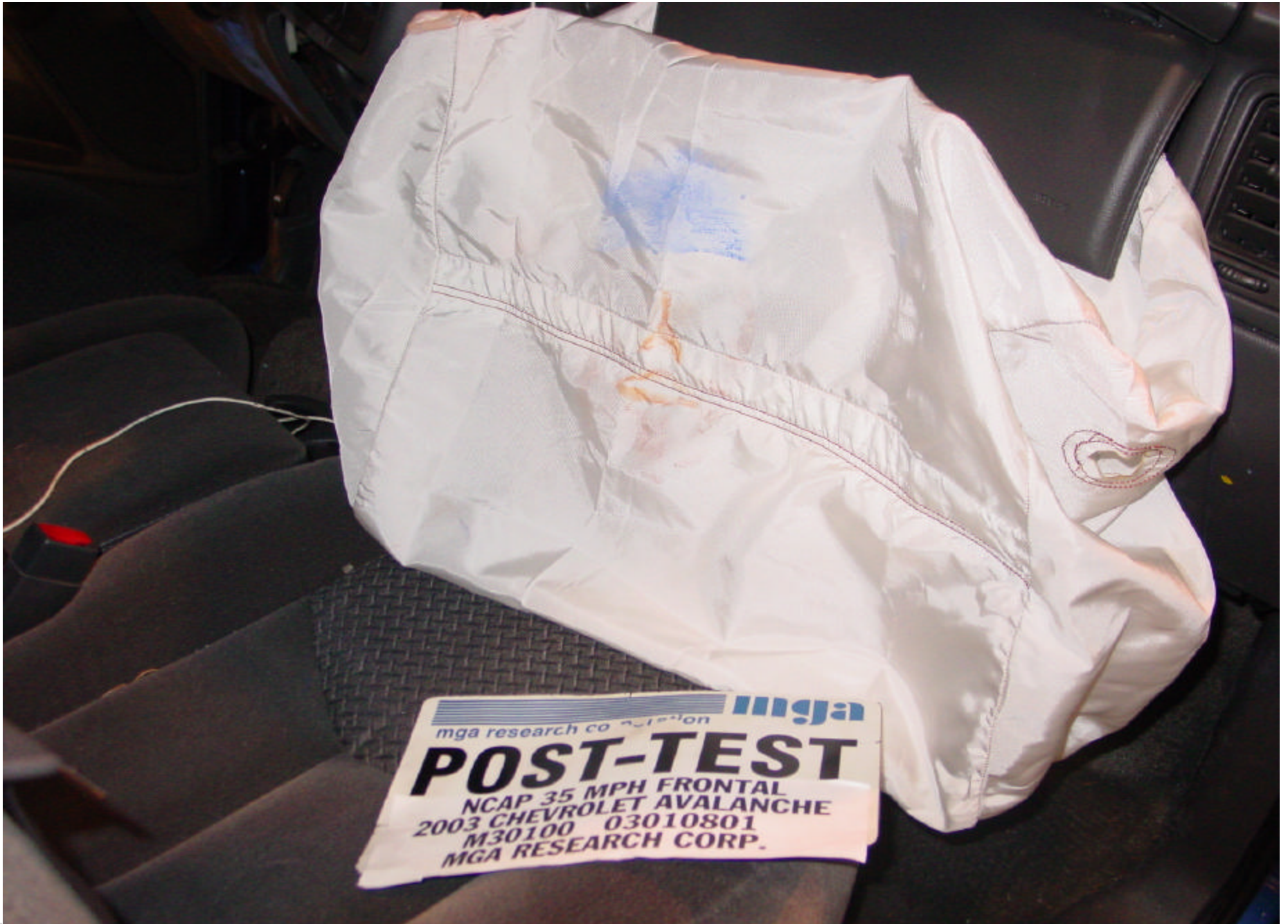
Post-Test Passenger Dummy Airbag Contact
