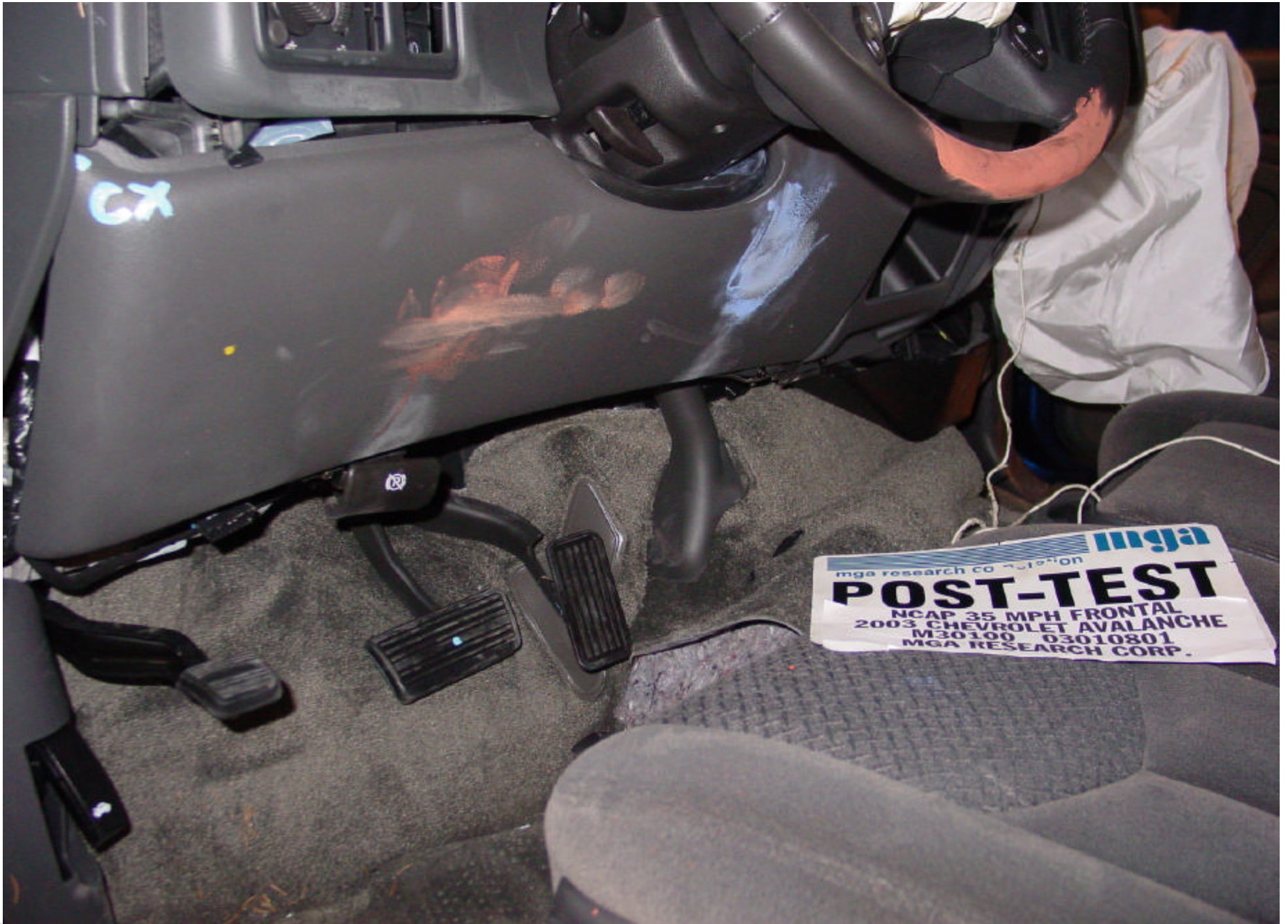
Post-Test Driver Dummy Knee Contact
