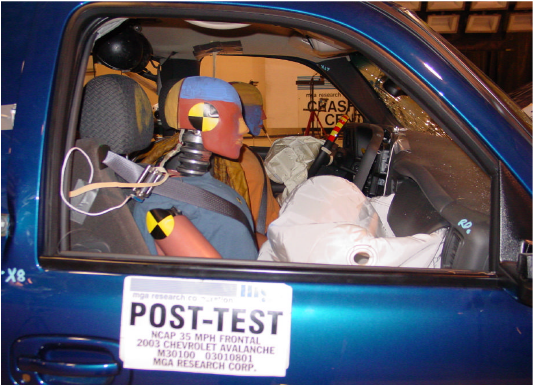
Post-Test Passenger Dummy Position Right Side View
