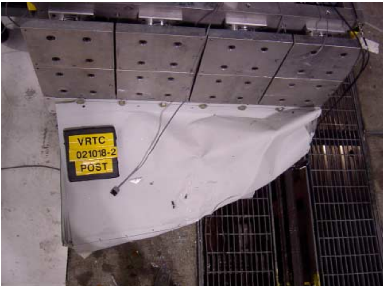
Figure A-46 Post-Test Overhead Barrier Face View
