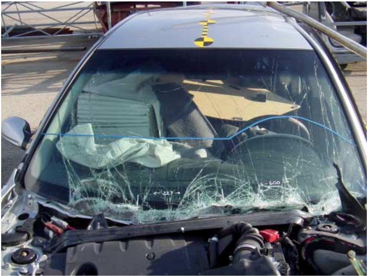
Figure A-36 Post-Test Windshield Loss of Retention - View 1
