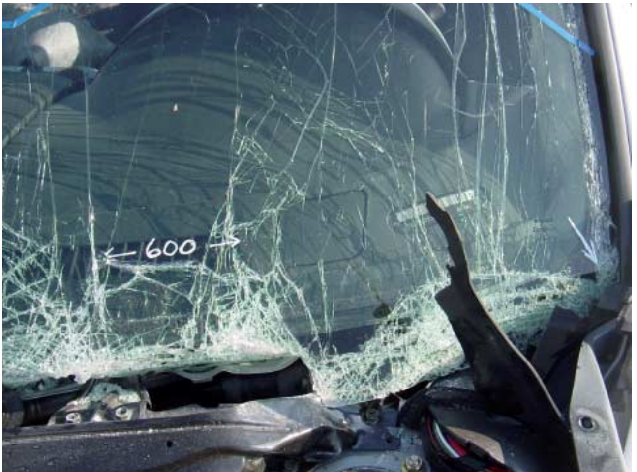
Figure A-37 Post-Test Windshield Loss of Retention - View 2
