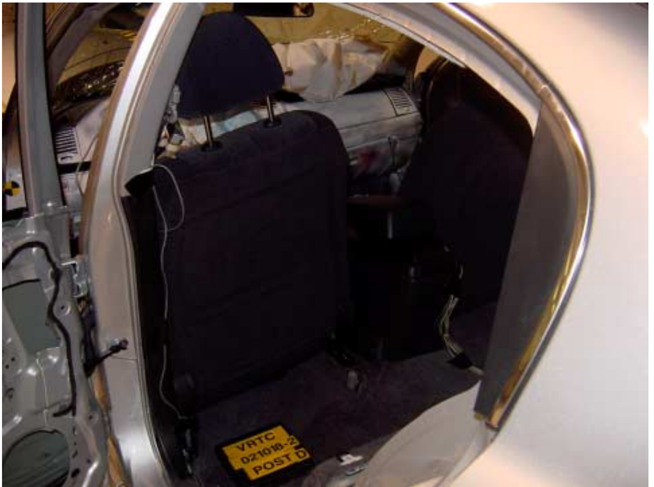
Figure A-81 Post-Test Driver Seat Damage - View 1
