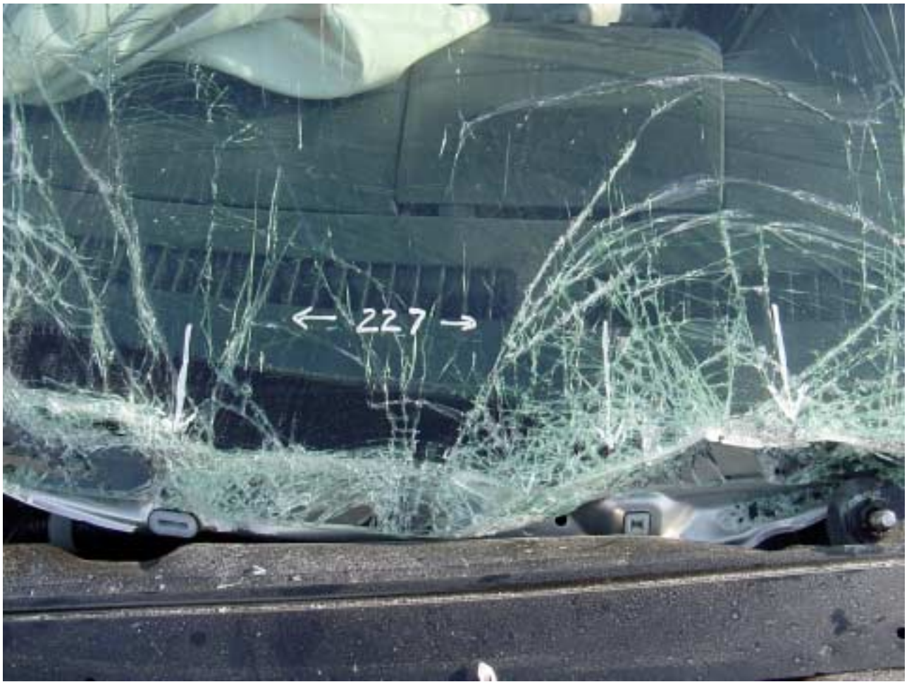
Figure A-38 Post-Test Windshield Loss of Retention - View 3
