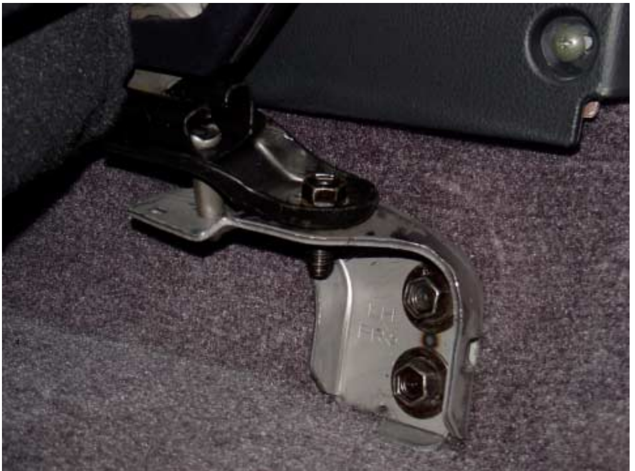
Figure A-82 Post-Test Driver Seat Damage - View 2
