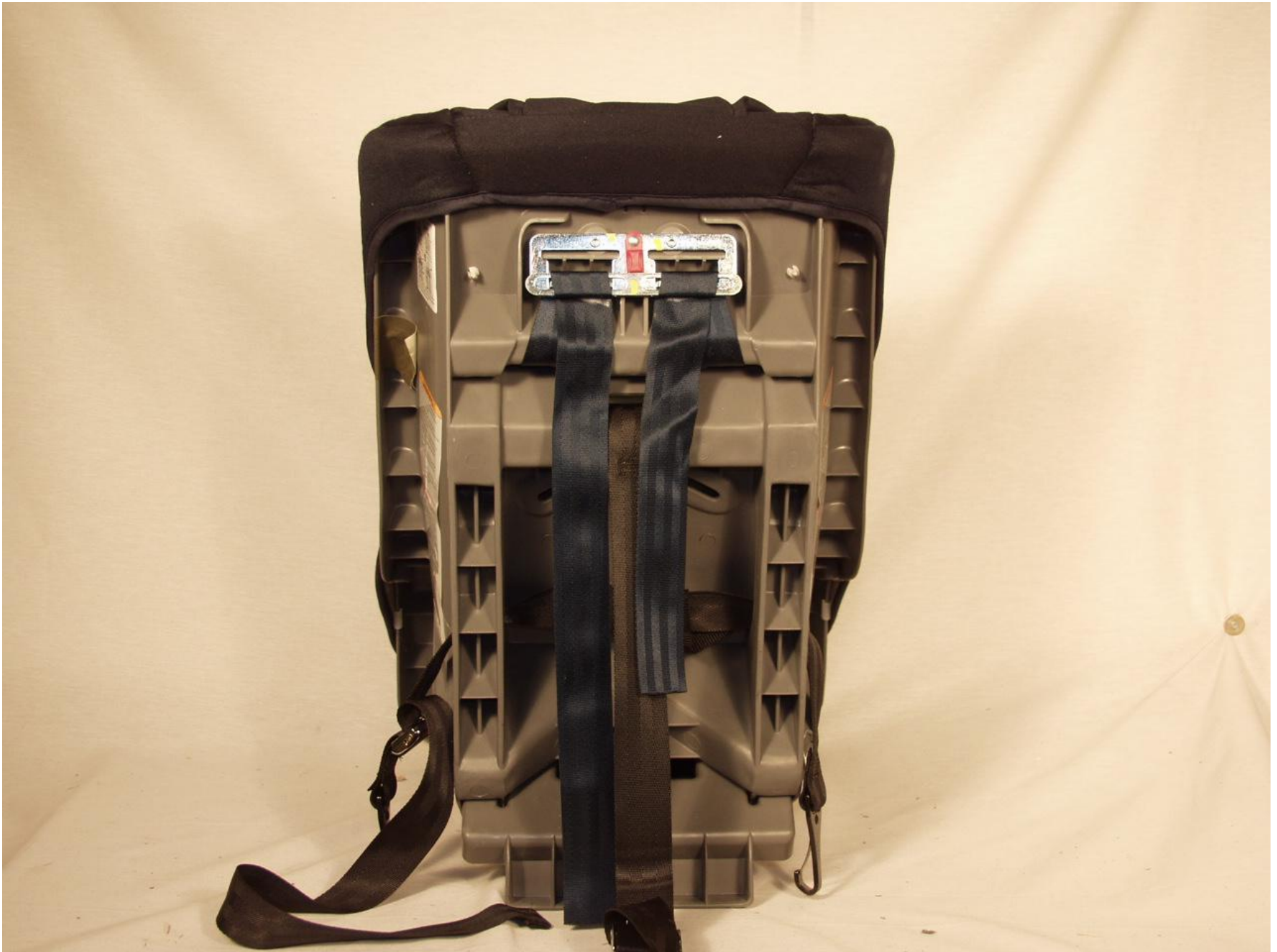
Figure 3-5: POST-TEST REAR VIEW OF POSITION 3 CRS
