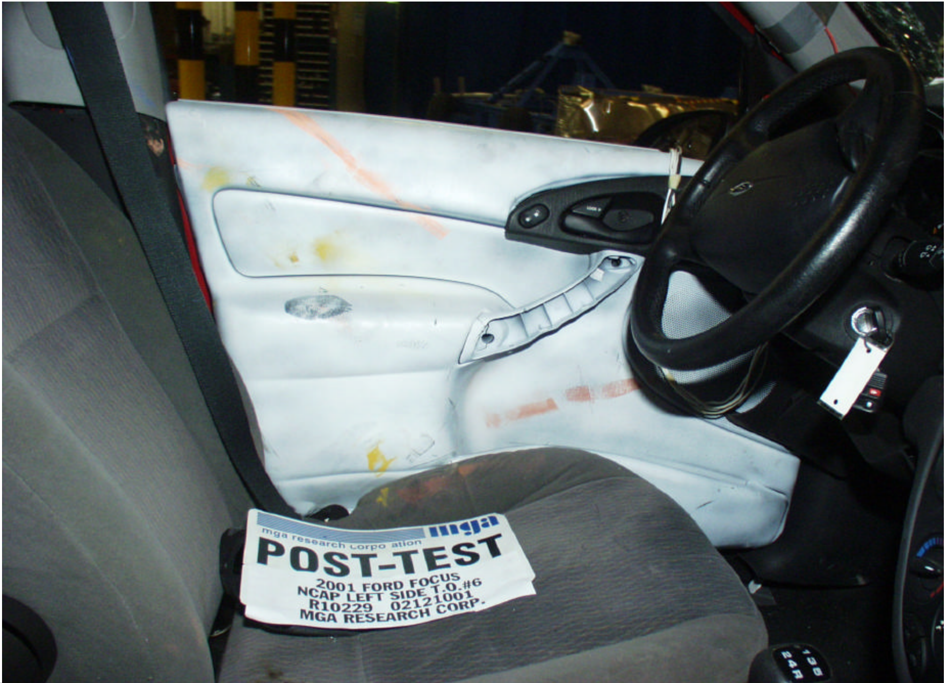
Post-Test Driver Dummy Lower Body Contact
