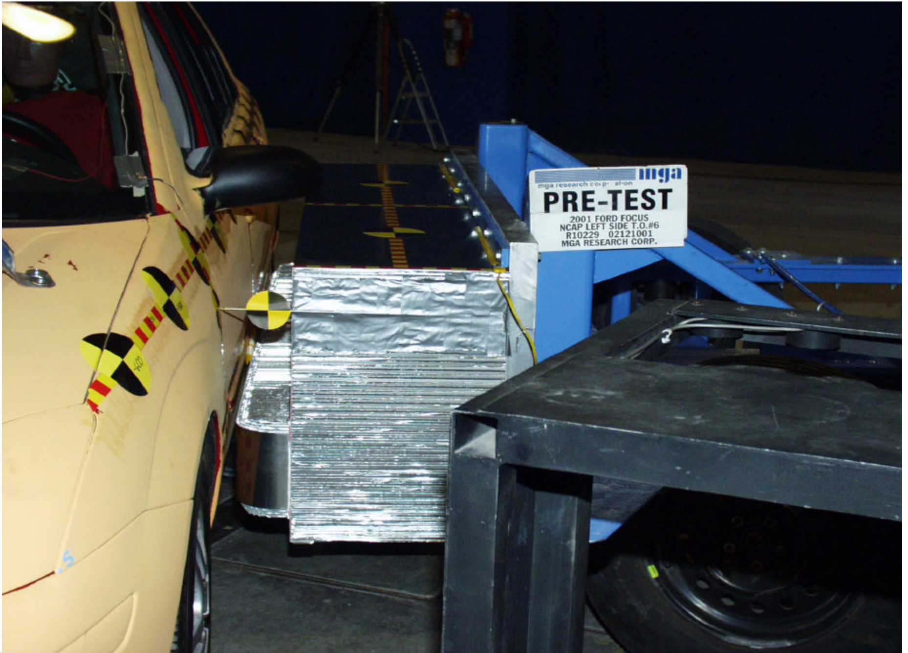
Pre-Test MDB Positioned Against Vehicle (left side)
