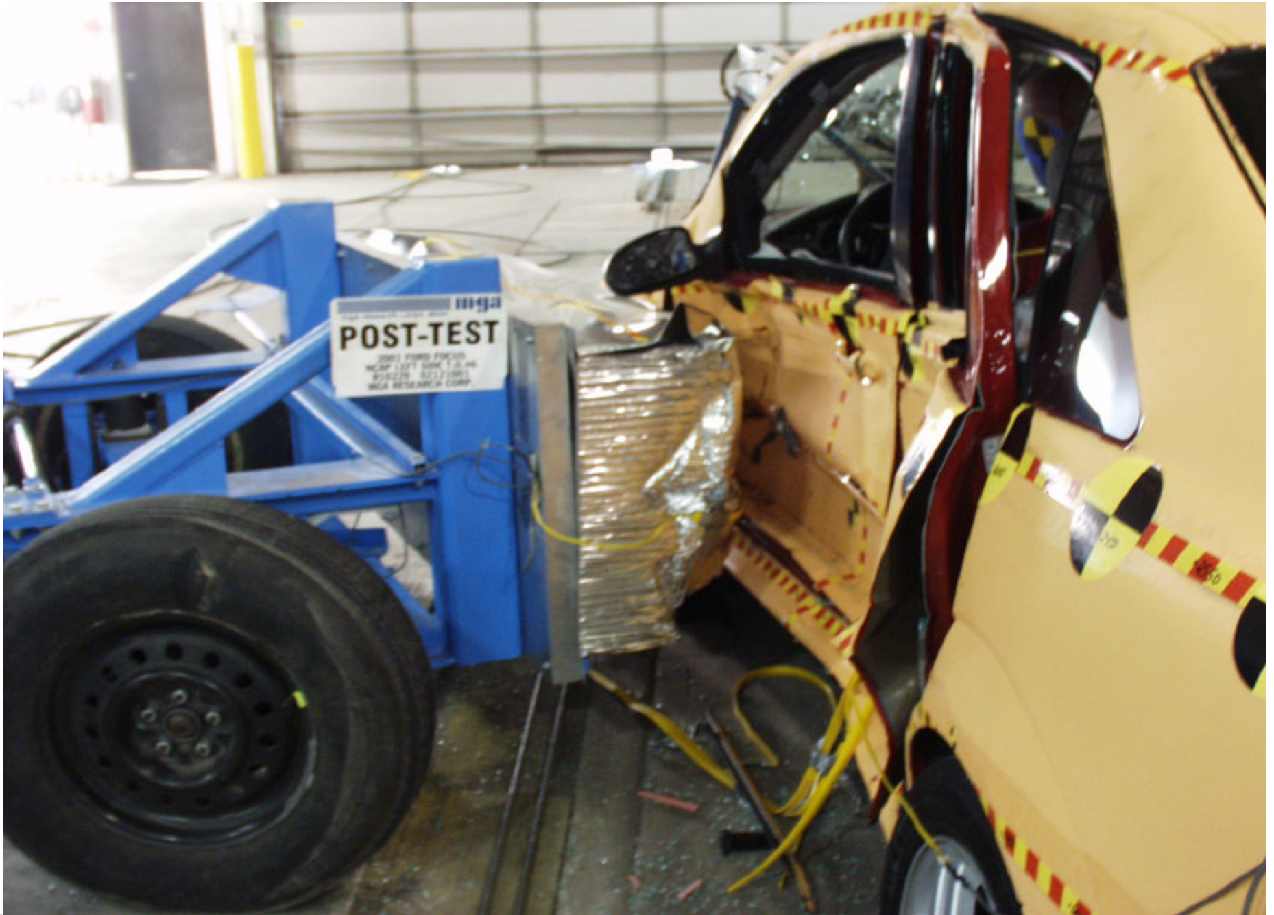
Post-Test MDB and Vehicle (right side)
