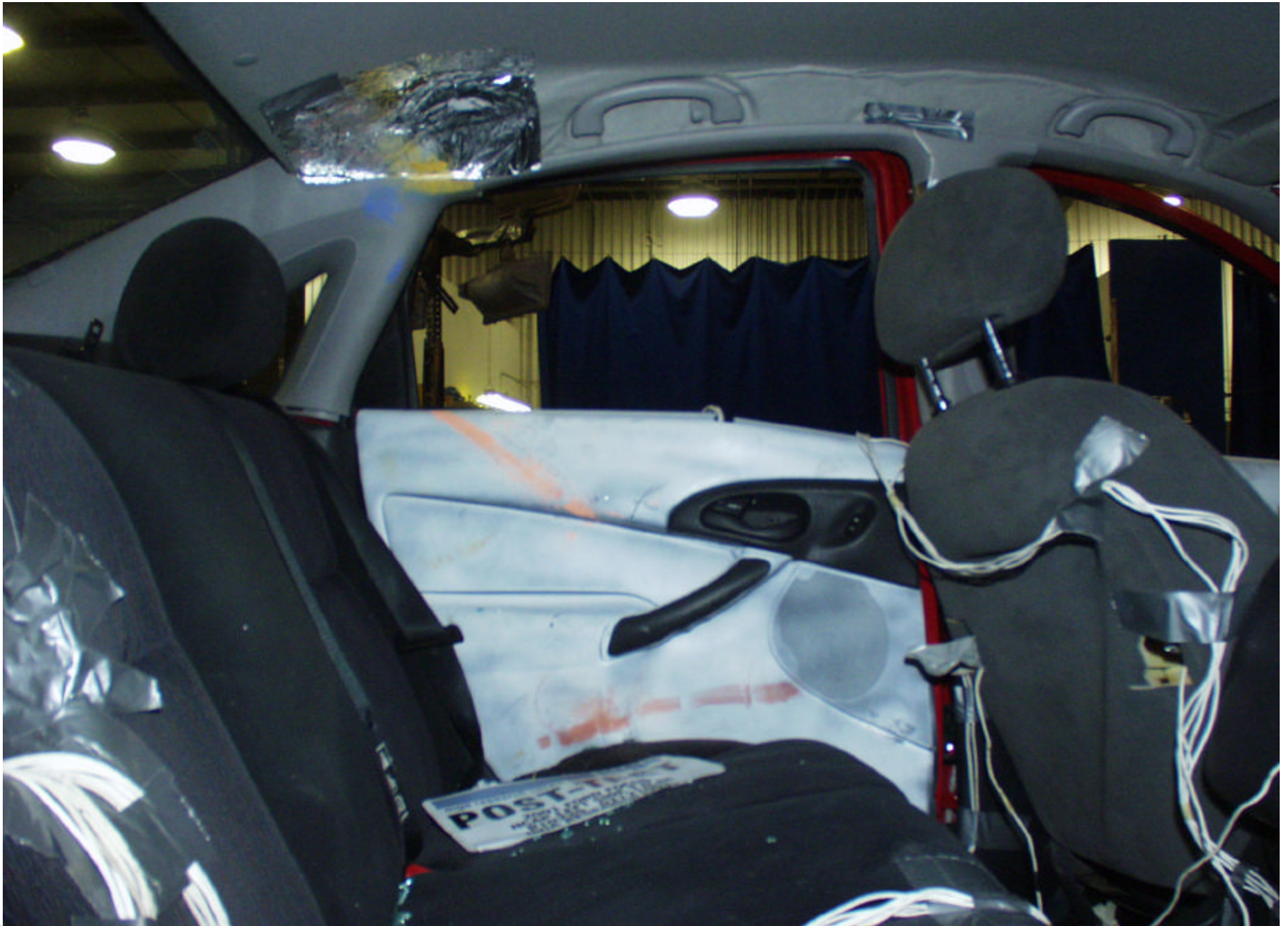
Post-Test Passenger Dummy Lower Body Contact
