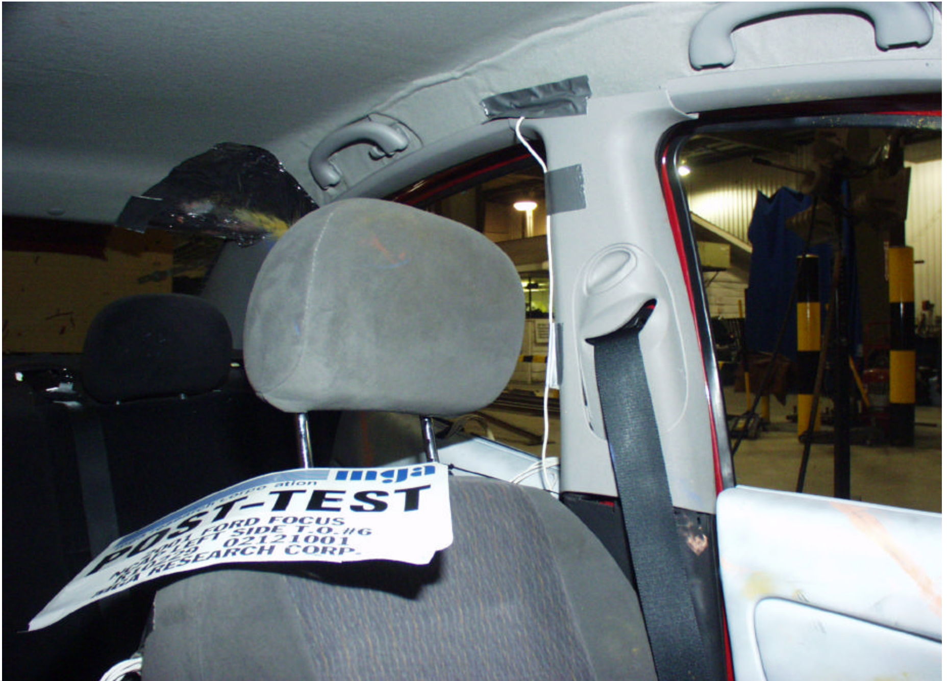
Post-Test Driver Dummy Head Contact
