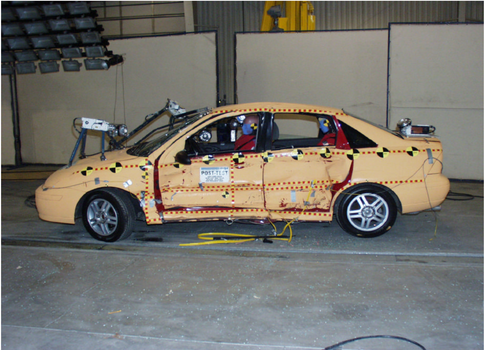
Post-Test Left Side View of Test Vehicle
