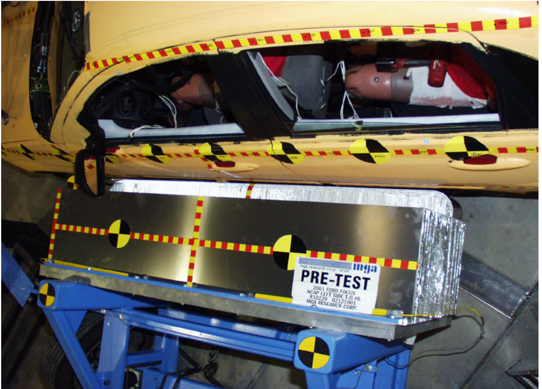
Pre-Test MDB Positioned Against Vehicle (overhead view)
