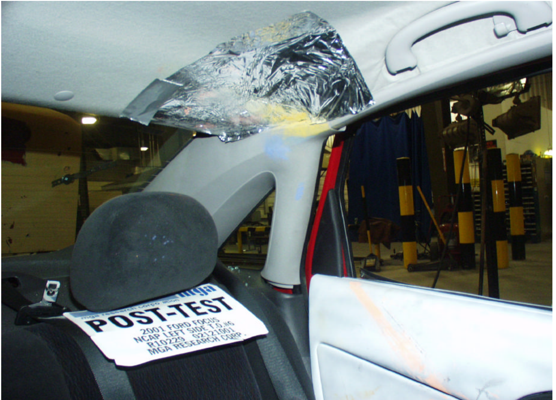
Post-Test Passenger Dummy Head Contact
