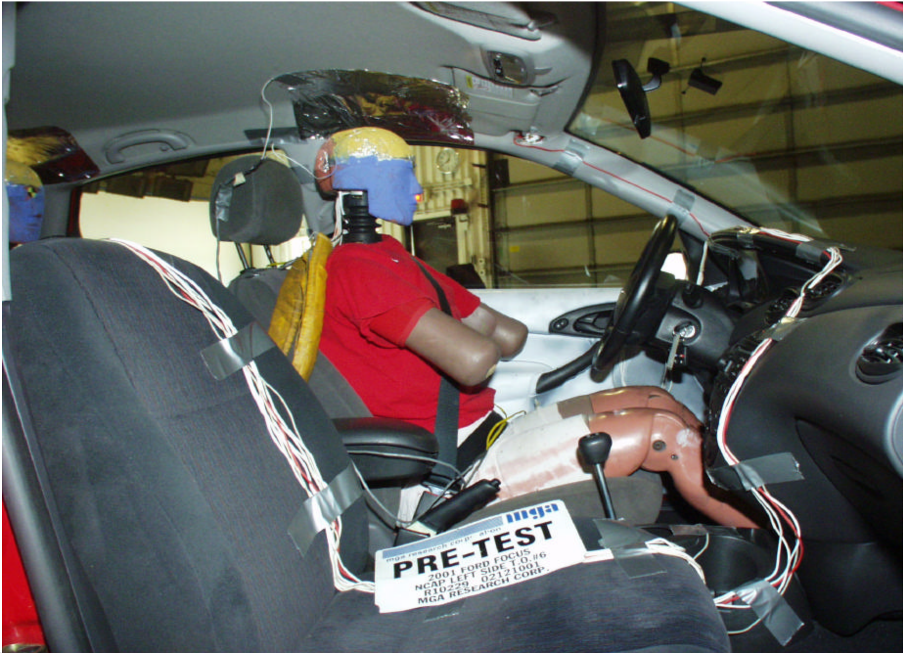
Pre-Test Driver Dummy Right Side View
