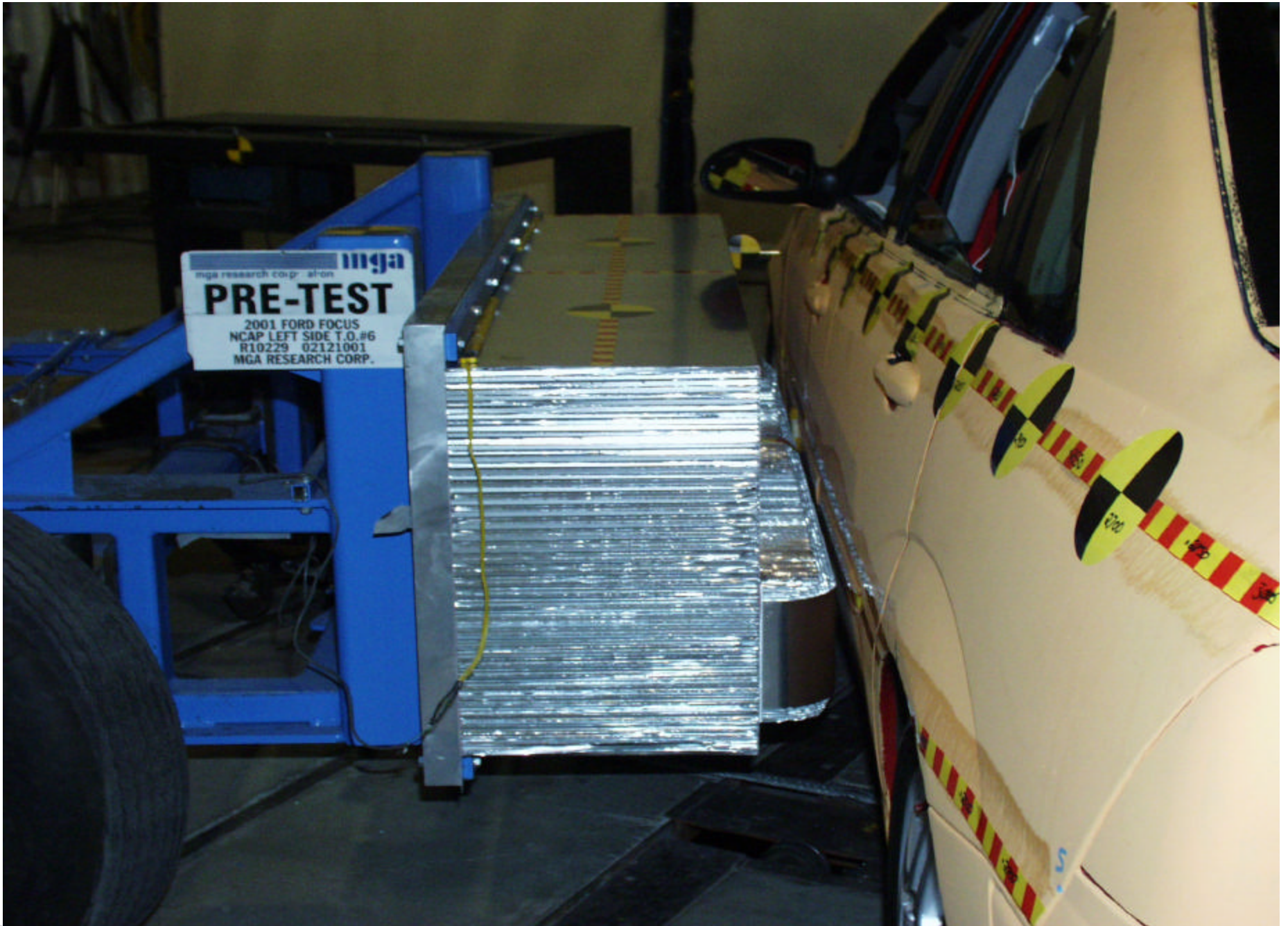
Pre-Test MDB Positioned Against Vehicle (right side)
