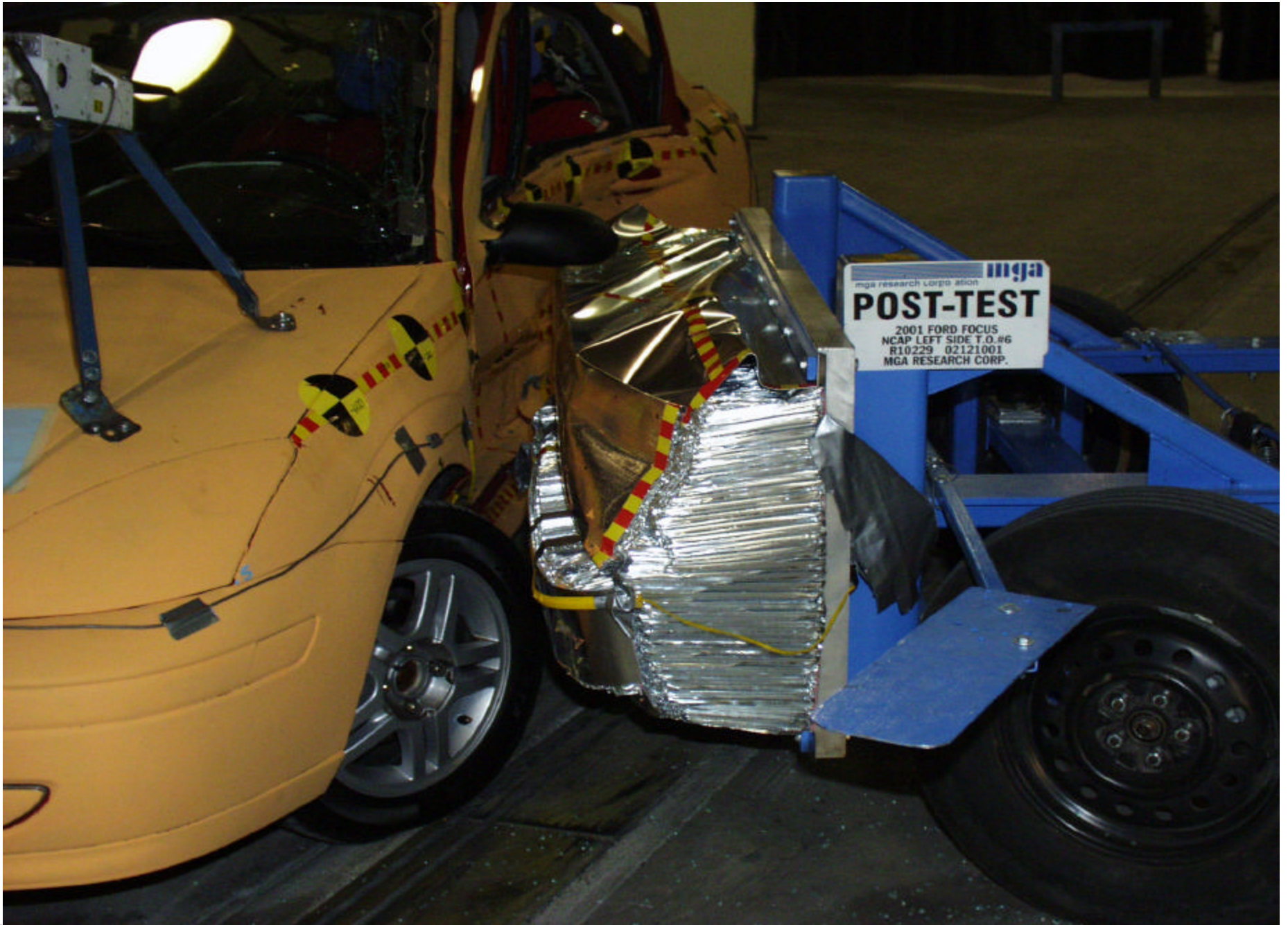
Post-Test MDB and Vehicle (left side)
