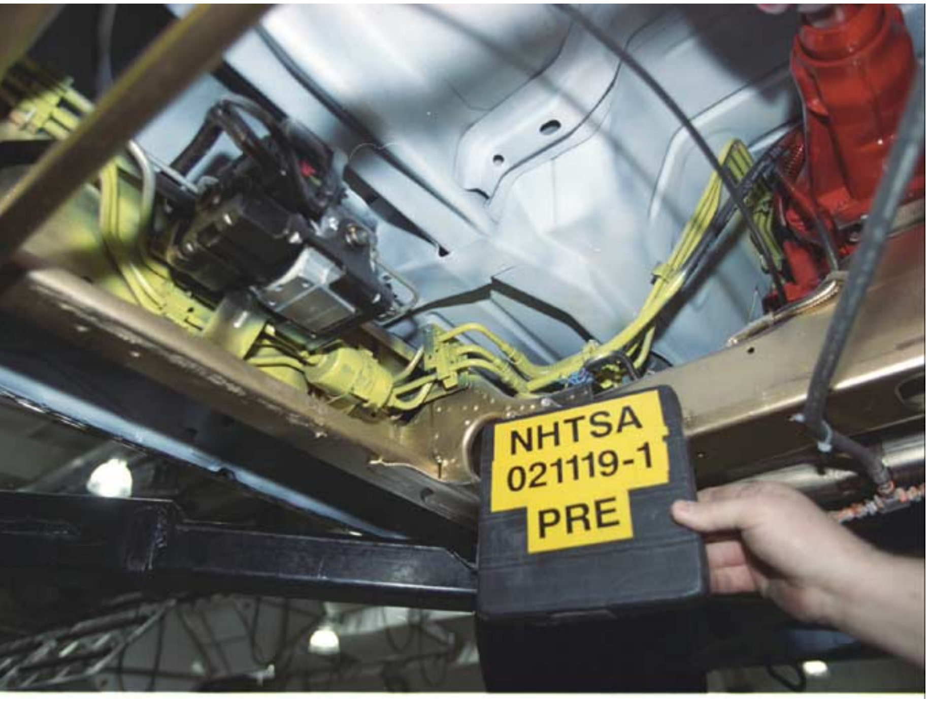
Image 29 Pre-Test Fuel Lines and Filter View
