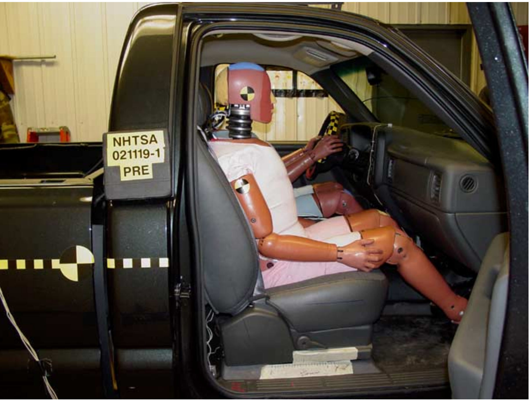
Image 43 Pre-Test Passenger Dummy Position View
