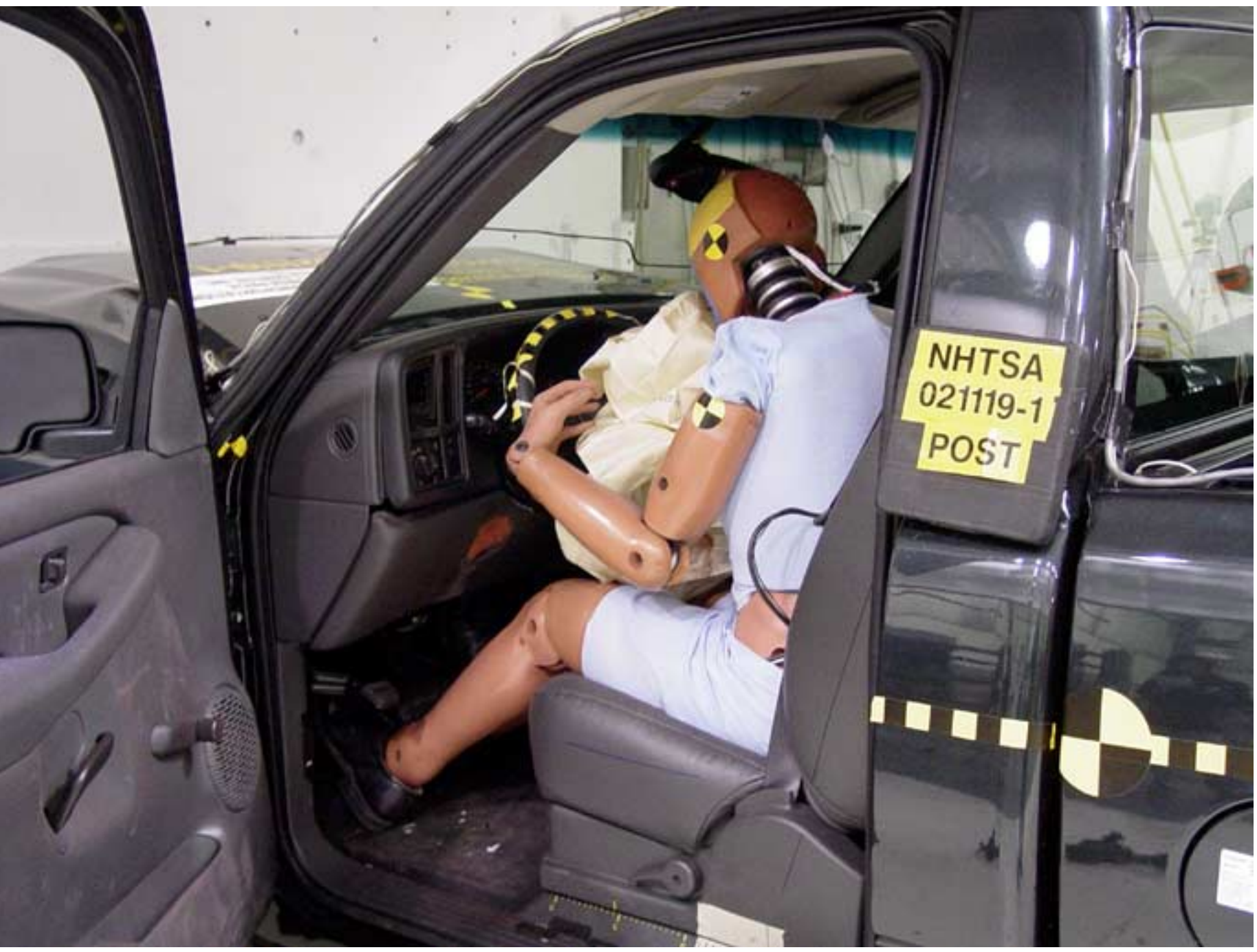
Image 40 Post-Test Driver Dummy & Vehicle Intrusion View
