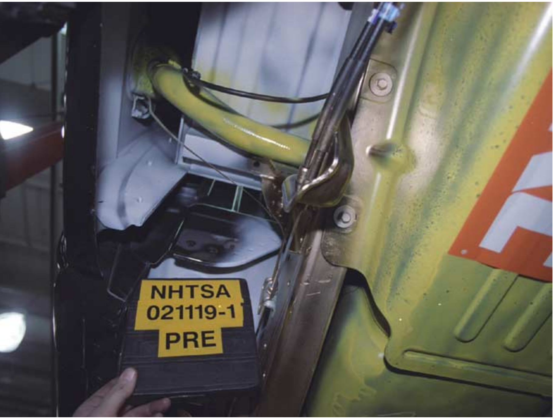
Image 31 Pre-Test Fuel Filler Neck View
