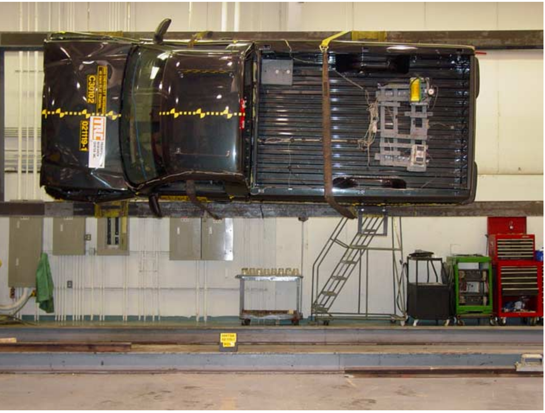
Image 59 Post-Test Vehicle on Static Rollover Device - 90° View
