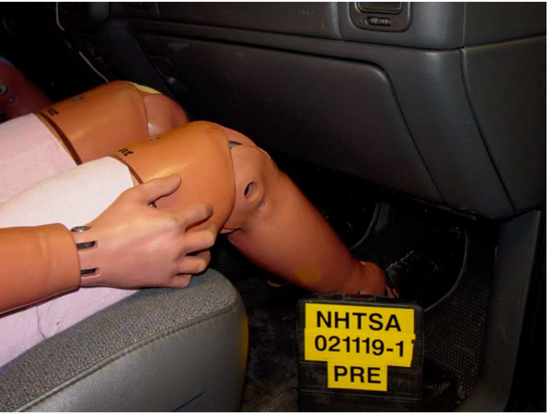
Image 56 Pre-Test Passenger Dummy Knee Bolster View
