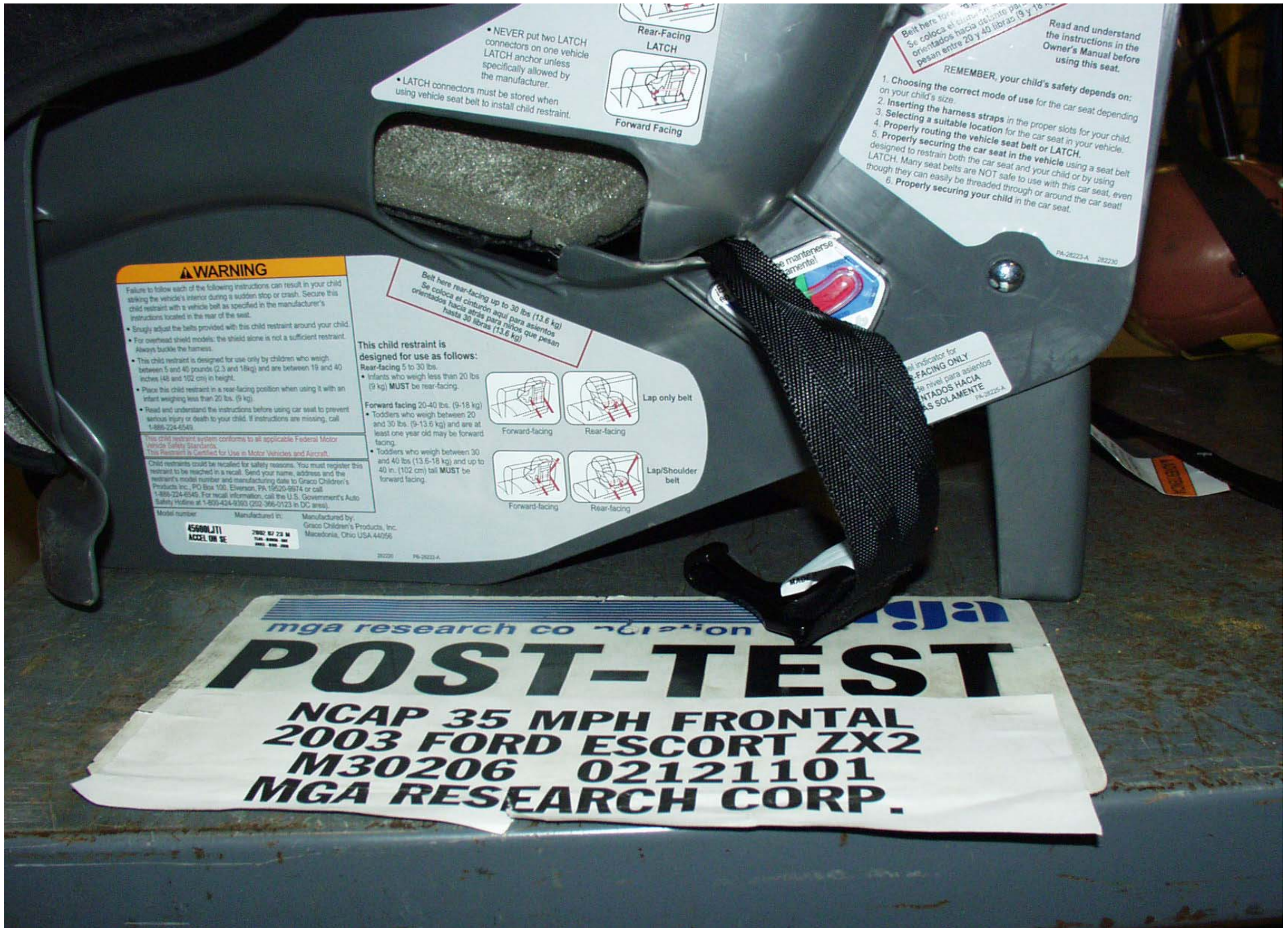
Post-Test Position 4 Left Lower Anchor Strap
