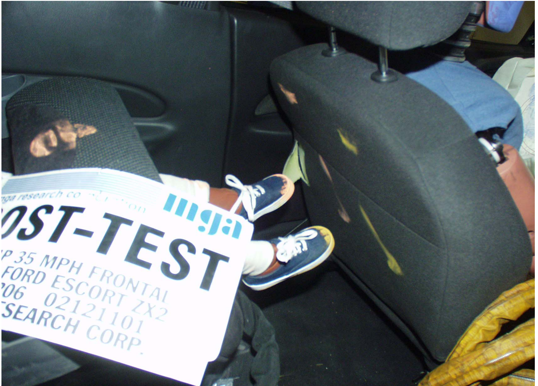
Post-Test Position 4 Head and Feet Contact
