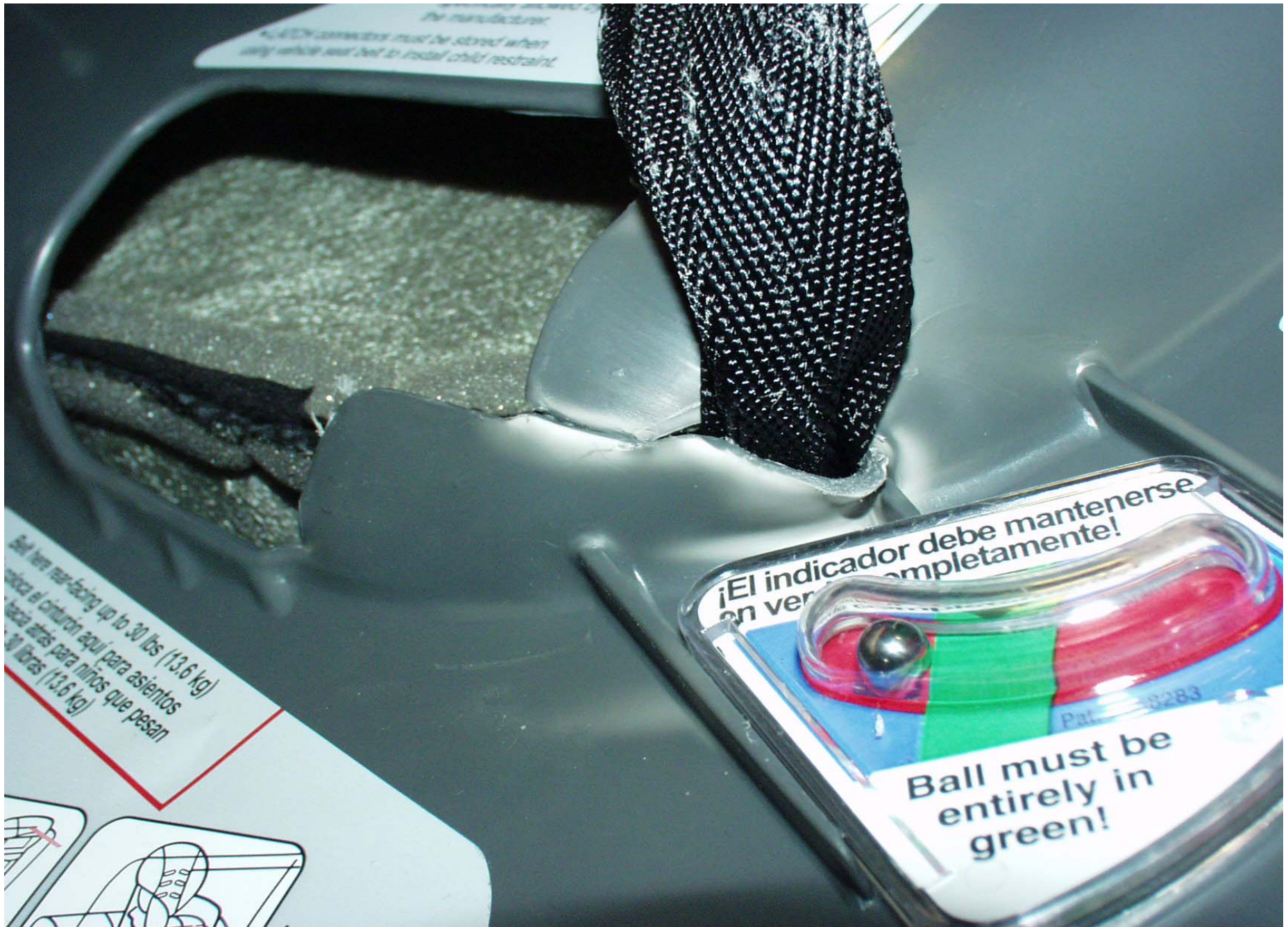
Post-Test Position 4 Left Lower Anchor Strap
