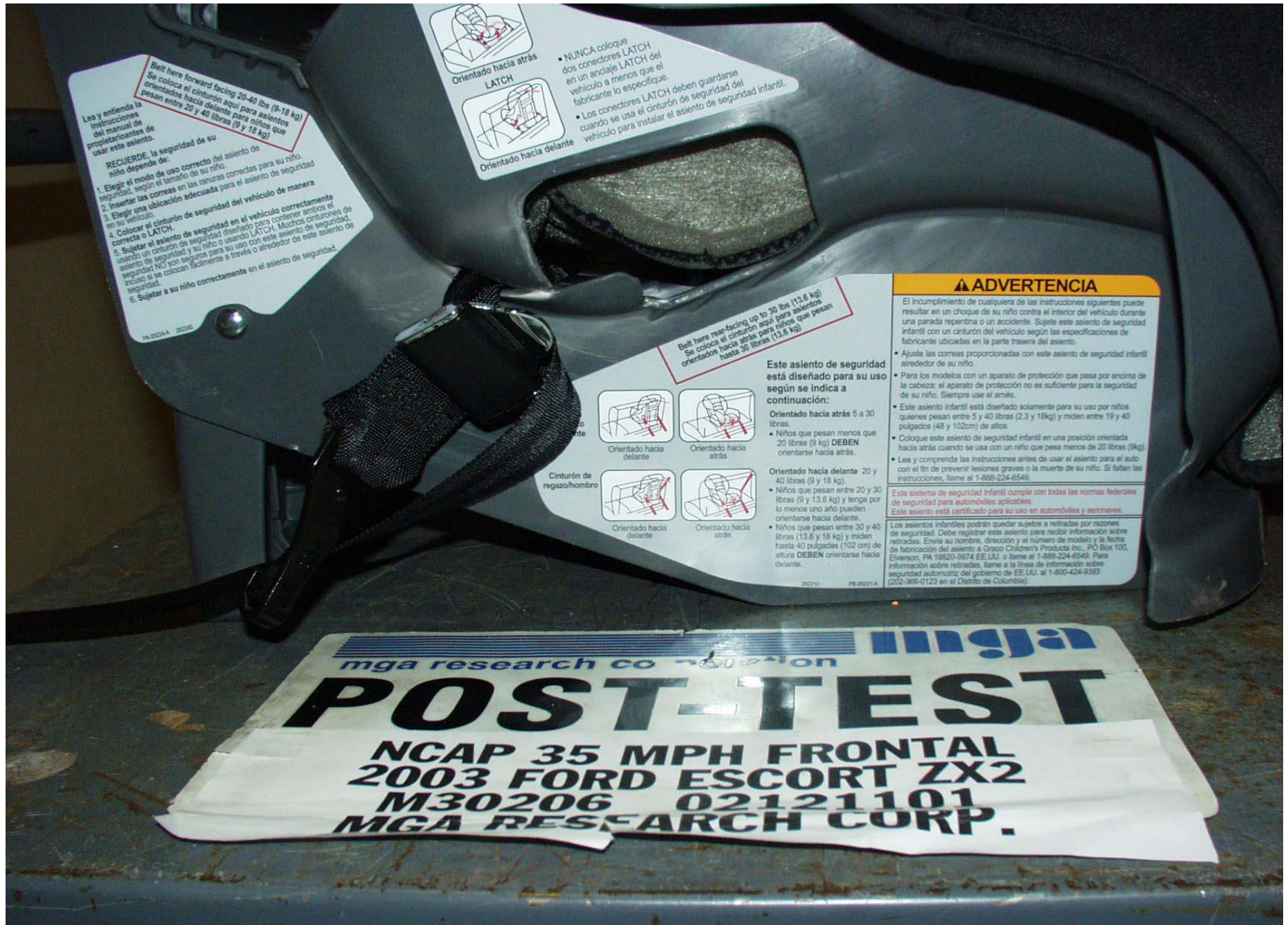
Post-Test Position 4 Right Lower Anchor Strap
