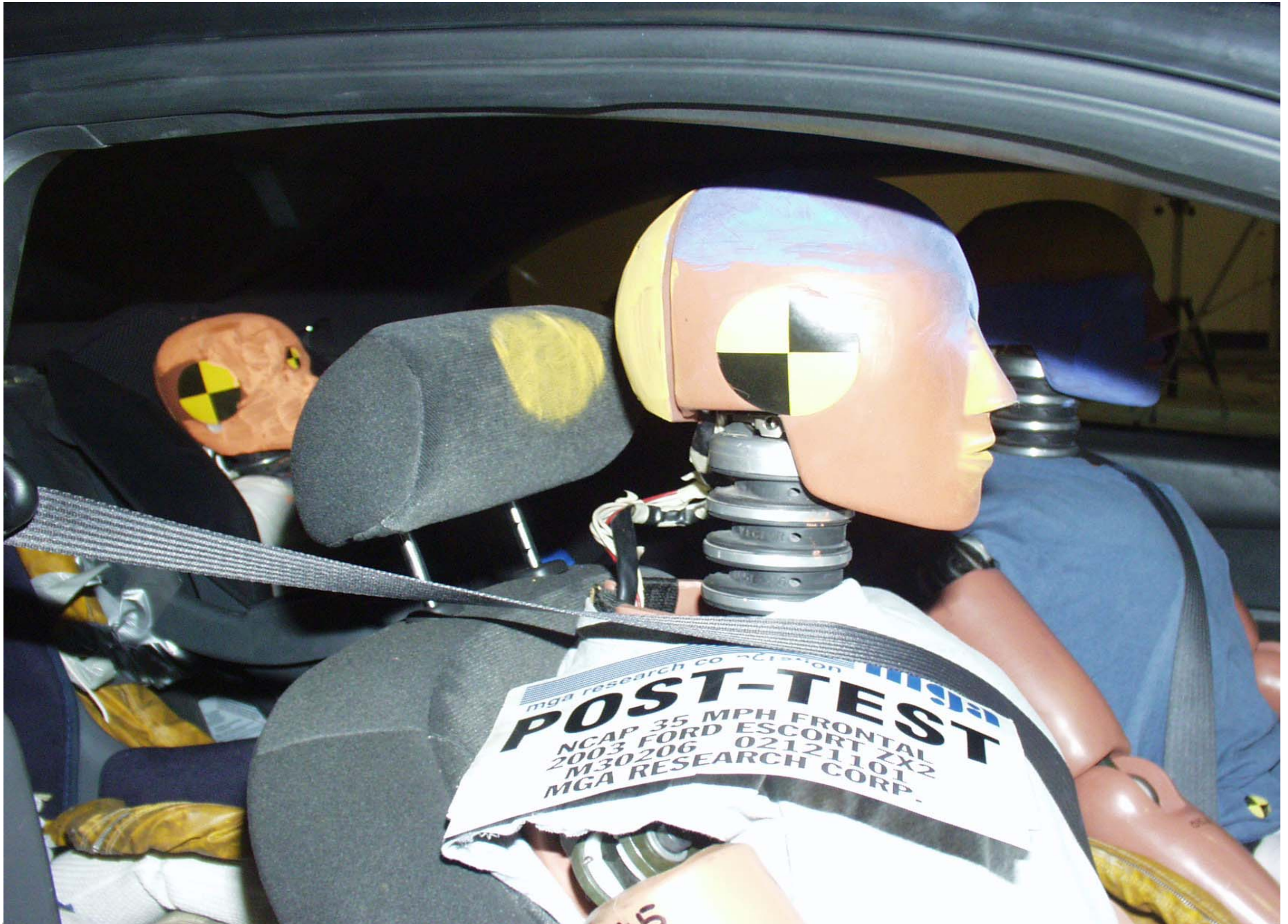
Post-Test Passenger Dummy Head Contact
