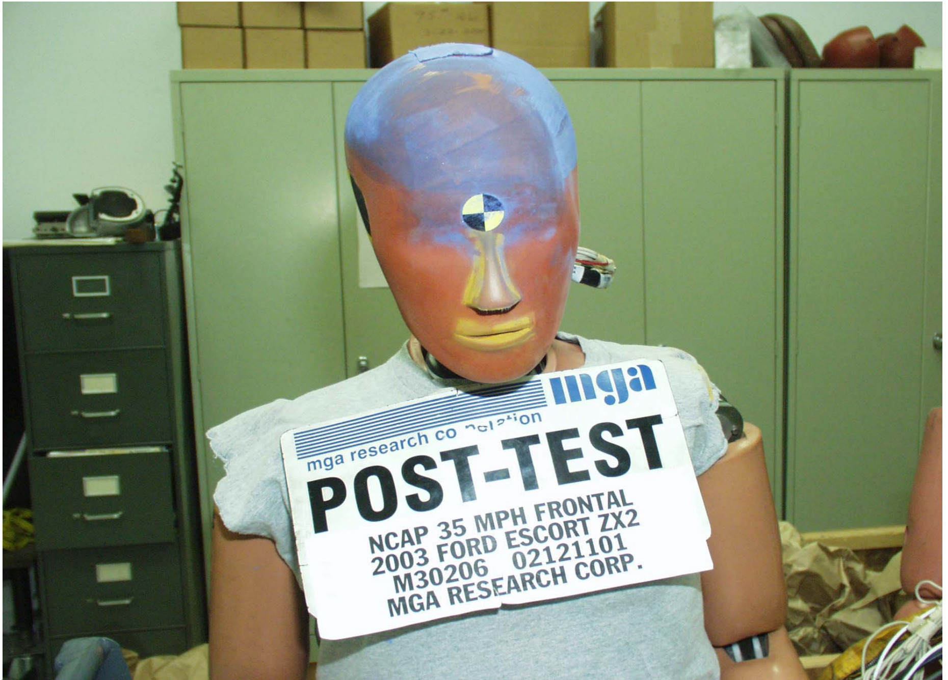
Post-Test Passenger Dummy Head
