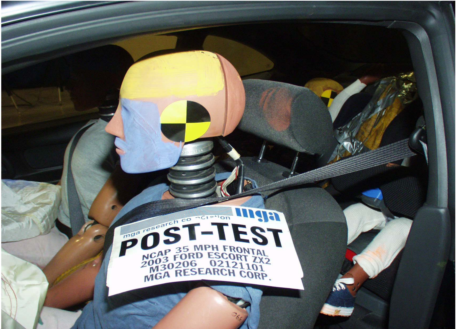
Post-Test Driver Dummy Head Contact
