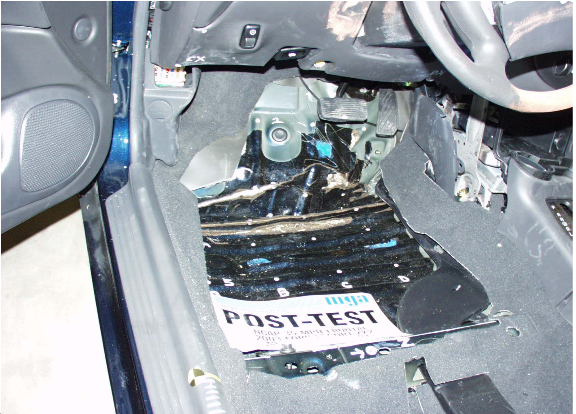
Post-Test Driver Side Floor Pan View
