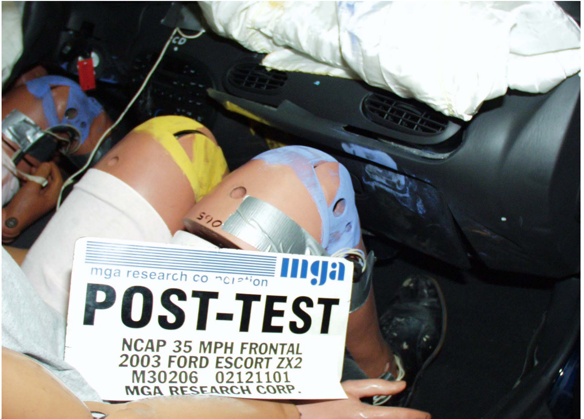
Post-Test Passenger Side Knee Bolster View
