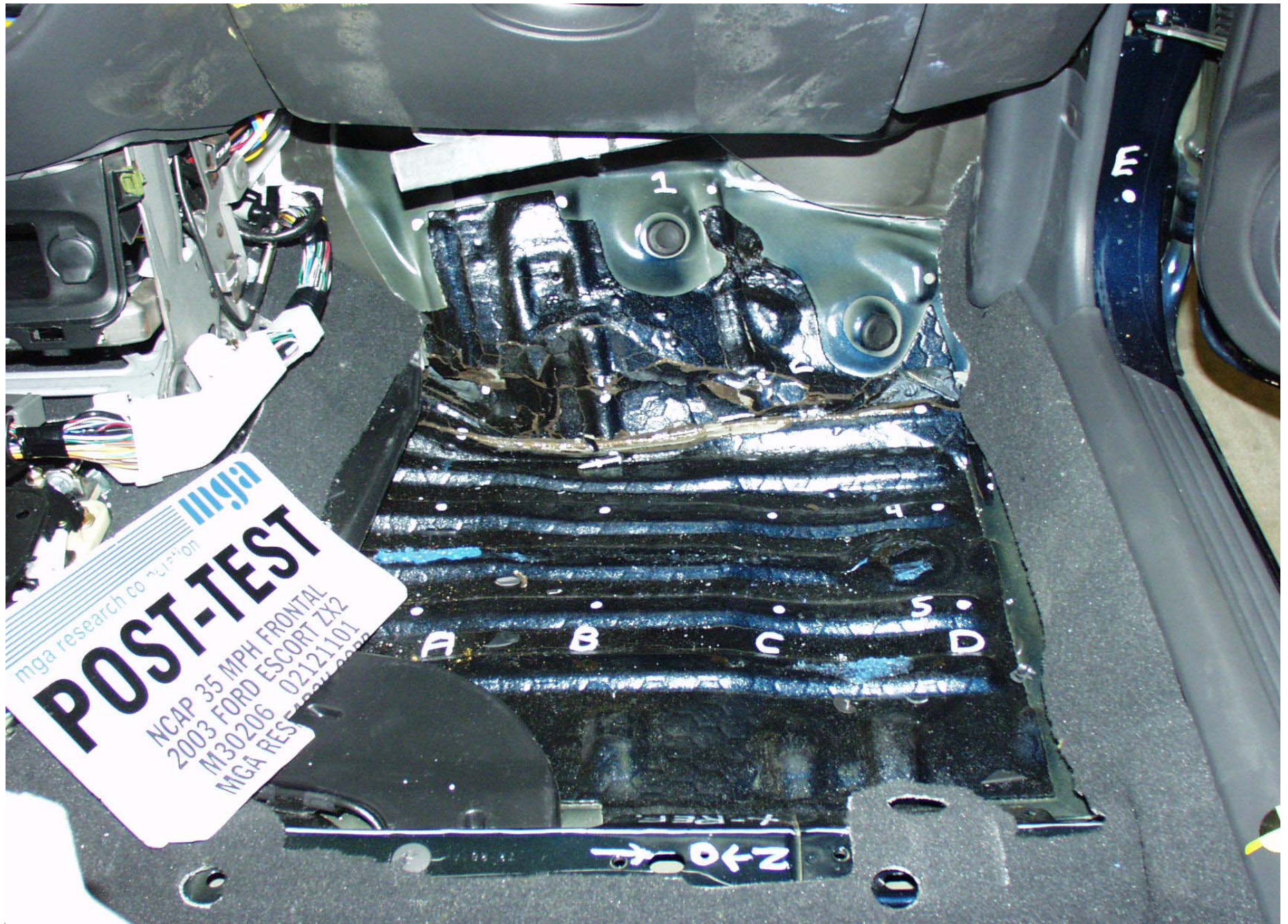
Post-Test Passenger Side Floor Pan View
