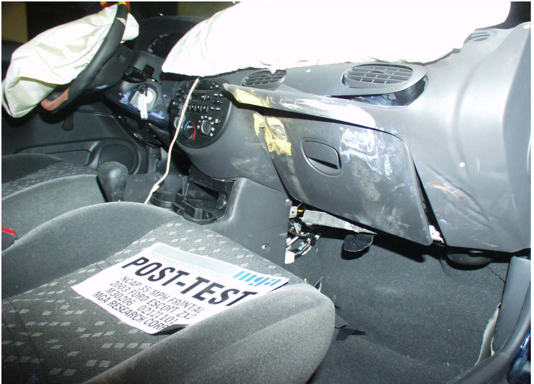
Post-Test Passenger Dummy Knee Contact
