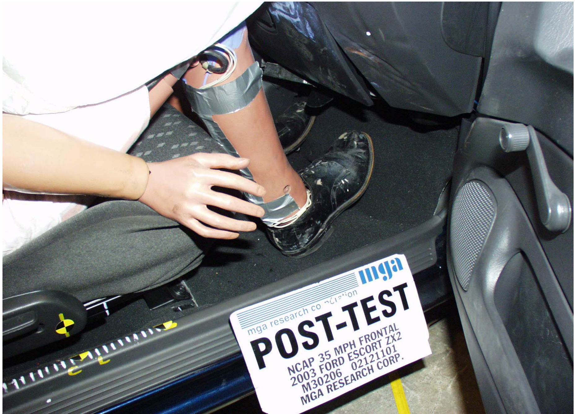
Post-Test Passenger Dummy Feet Position
