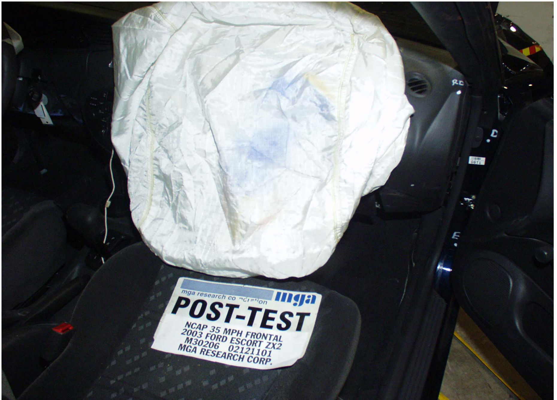
Post-Test Passenger Dummy Airbag Contact
