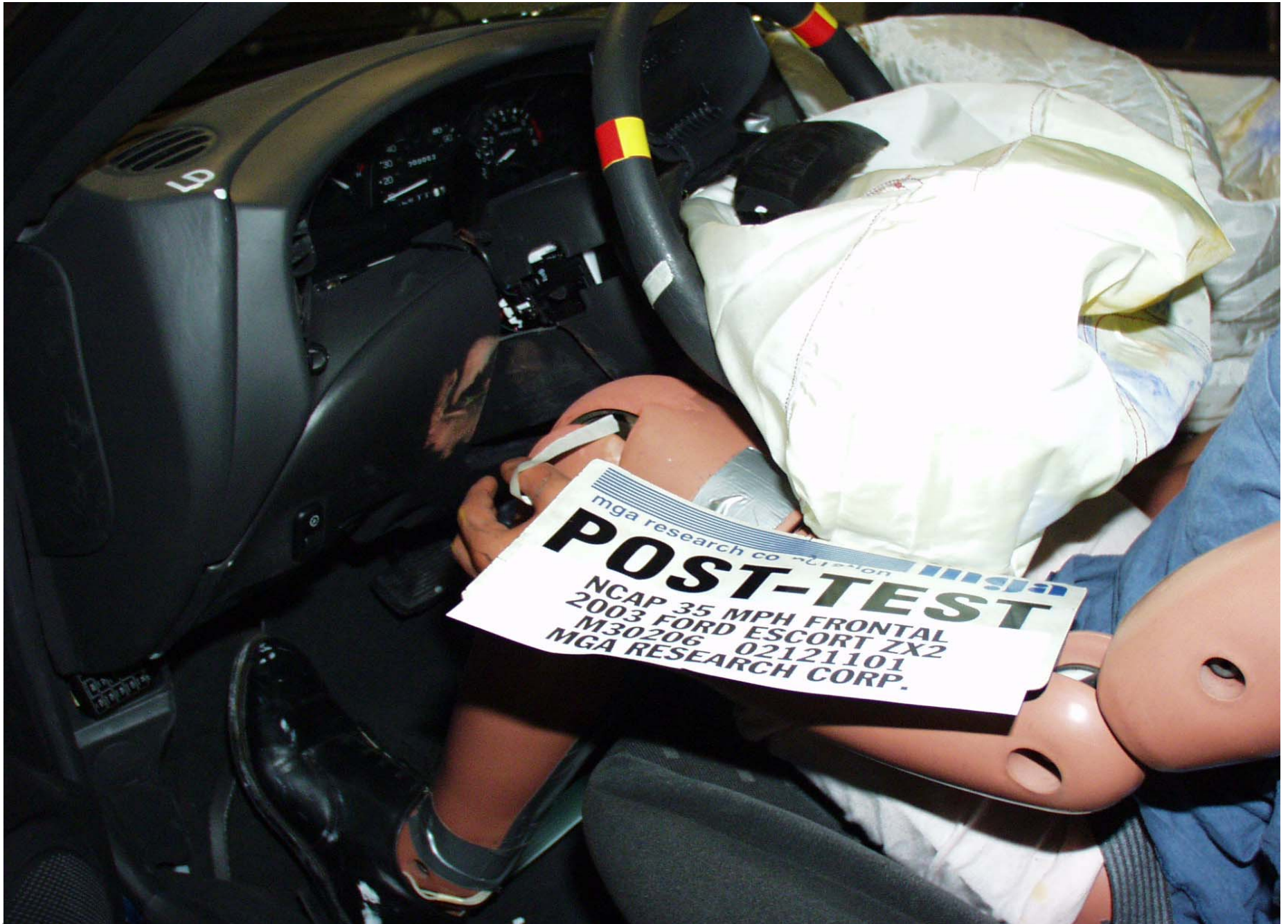
Post-Test Driver Side Knee Bolster View
