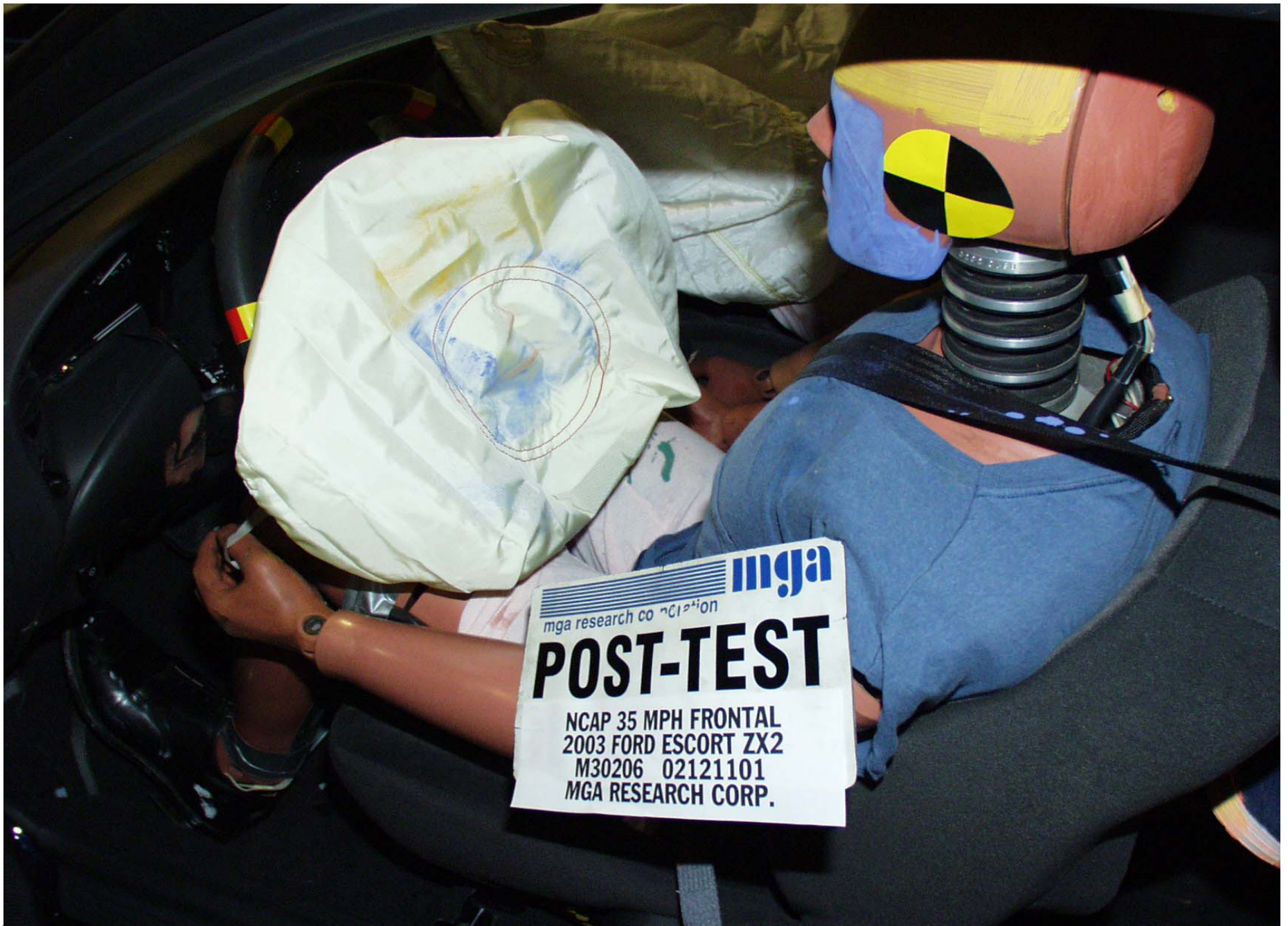
Post-Test Driver Dummy Airbag Contact
