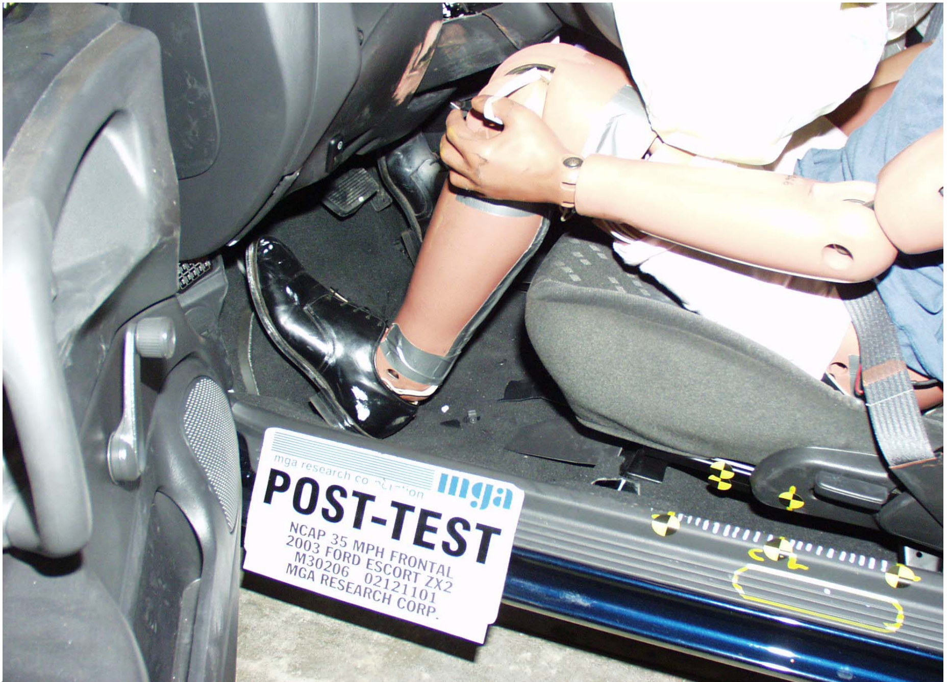
Post-Test Driver Dummy Feet Position
