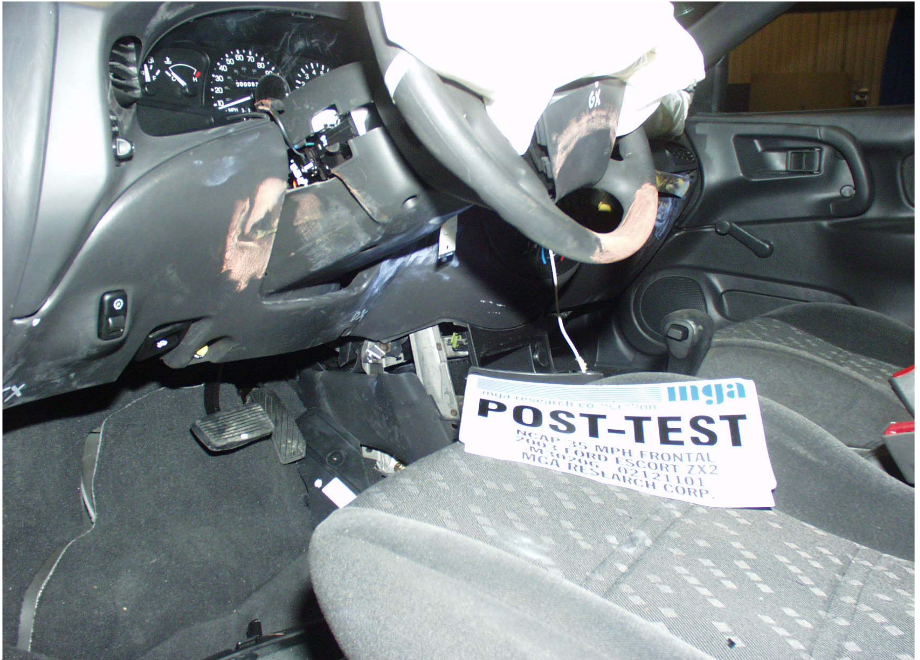
Post-Test Driver Dummy Knee Contact
