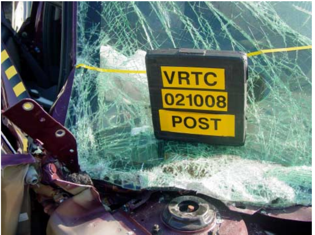
Figure A-80 Post-Test Windshield Retention Loss View
