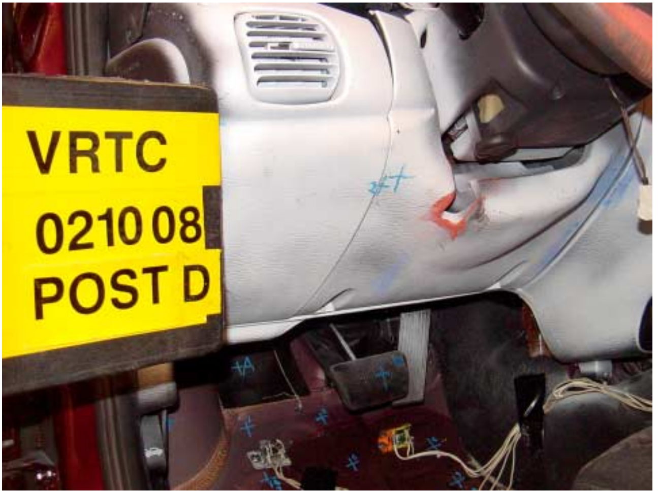
Figure A-66 Post-Test Driver Toeboard View
