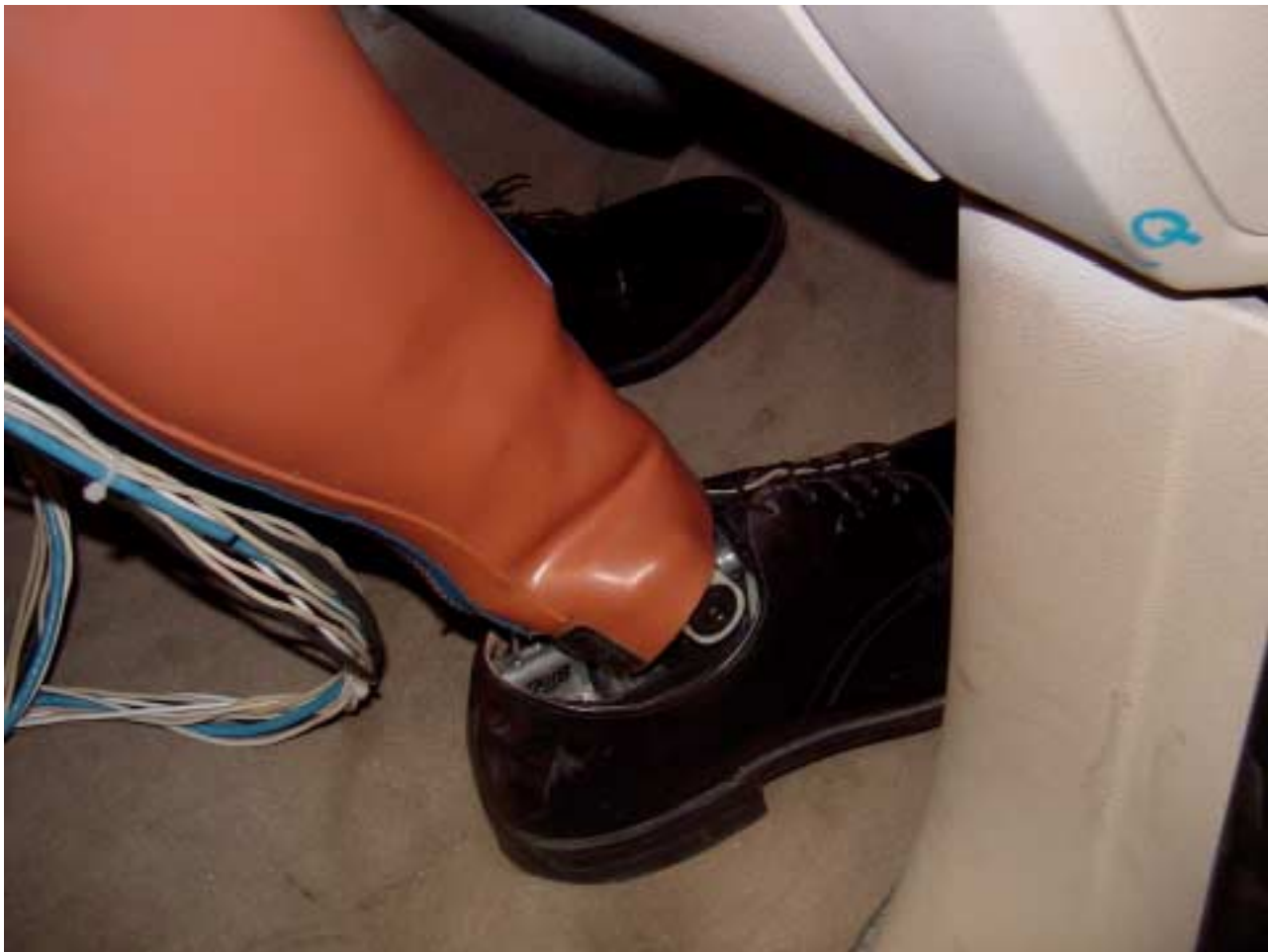
Figure A-72 Pre-Test Passenger Feet Position and Toeboard View
