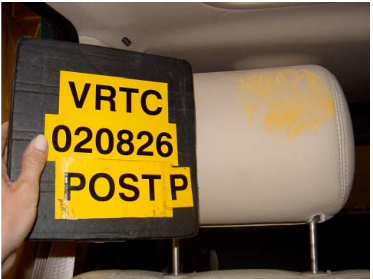
Figure A-69 Post-Test Passenger Dummy Head Contact - View 2
