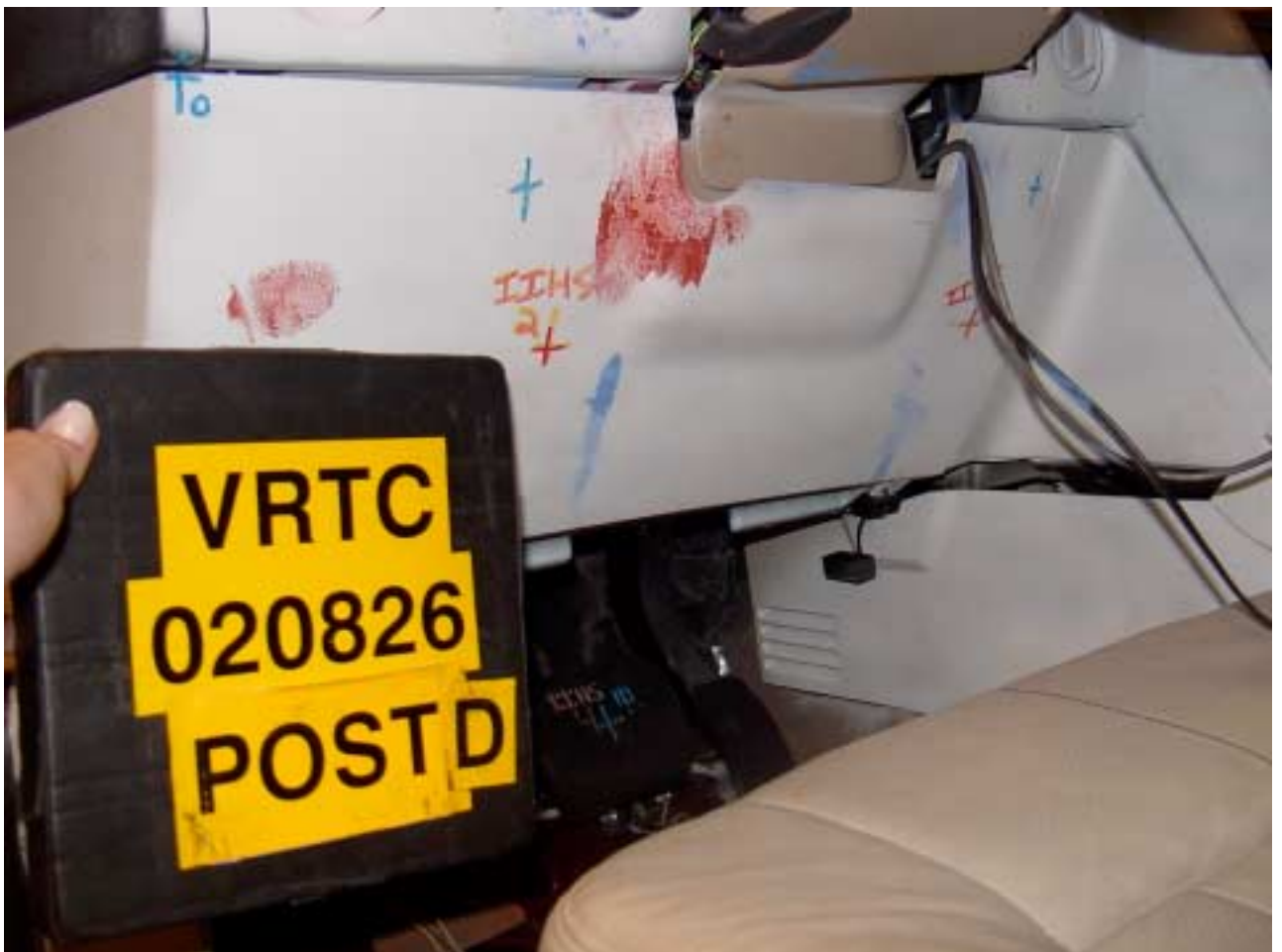
Figure A-64 Post-Test Driver Knee Contact - View 2
