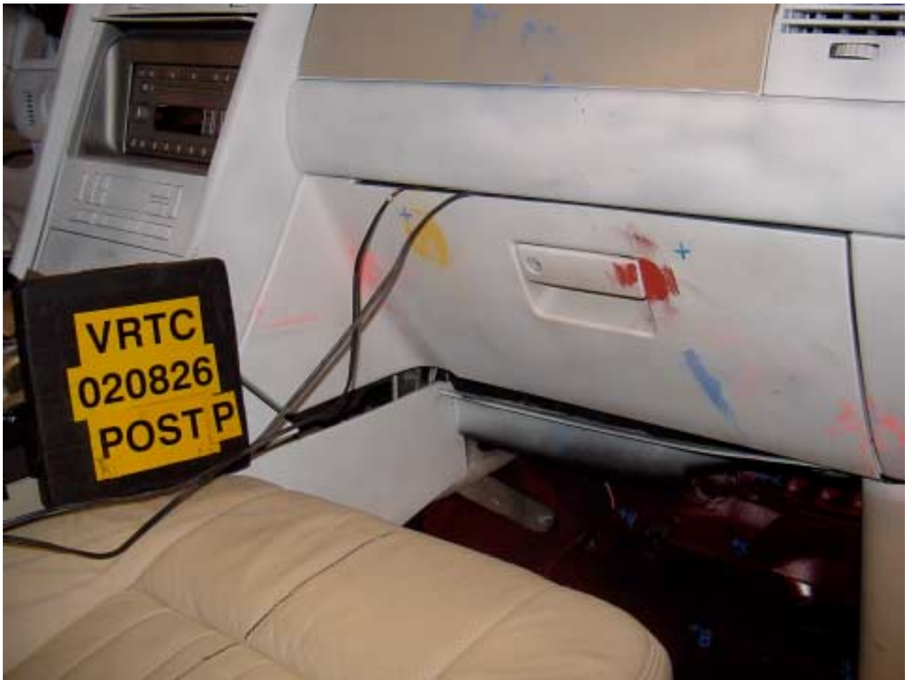
Figure A-71 Post-Test Passenger Dummy Knee Contact - View 2
