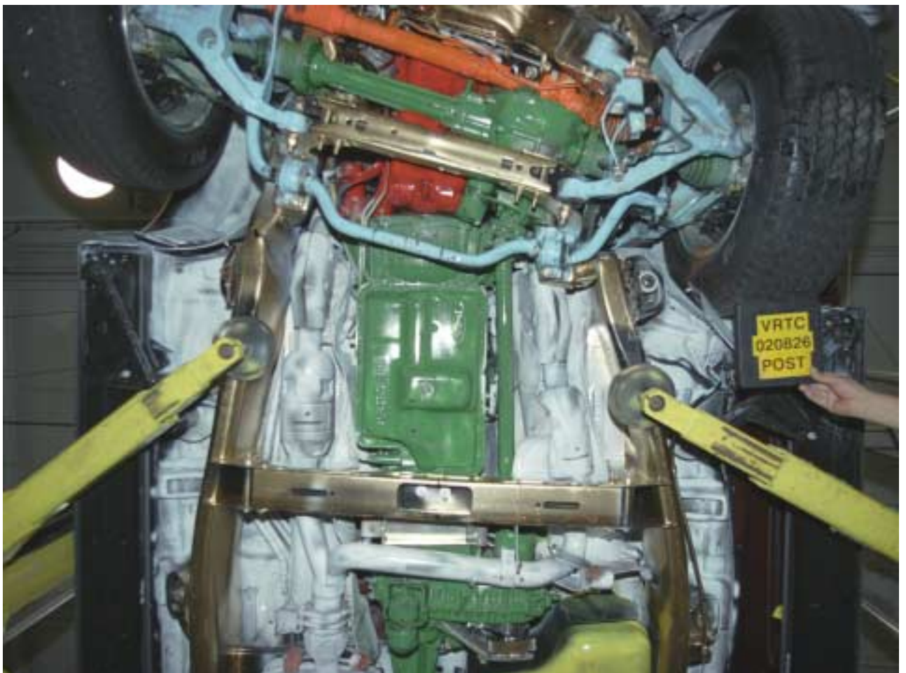
Figure A-22 Post-Test Front Mid Underbody View
