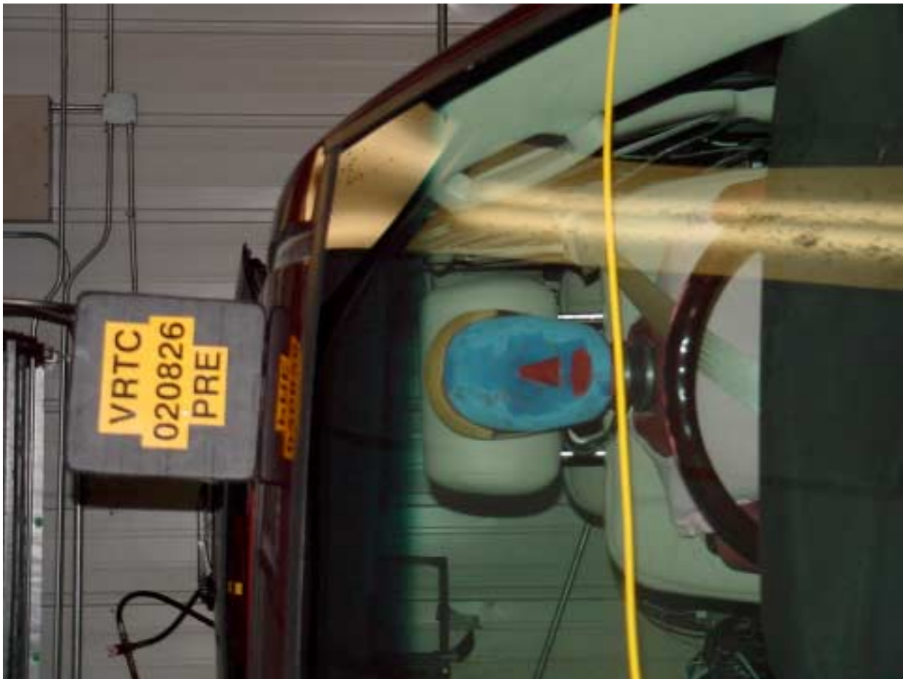
Figure A-45 Pre-Test Driver Dummy Position - View 1
