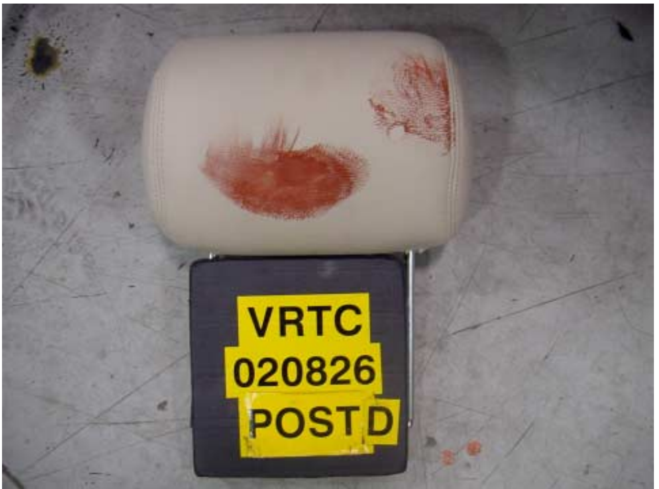
Figure A-62 Post-Test Driver Dummy Head Contact - View 3
