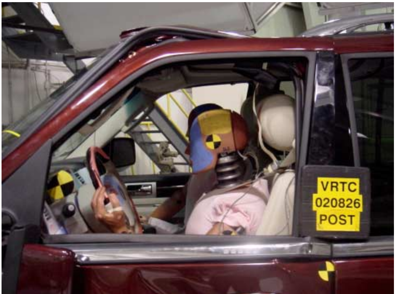
Figure A-48 Post-Test Driver Dummy Position - View 2
