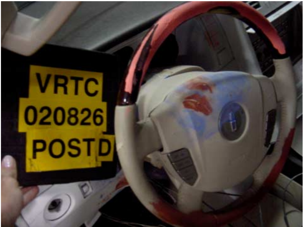
Figure A-61 Post-Test Driver Dummy Head Contact - View 2
