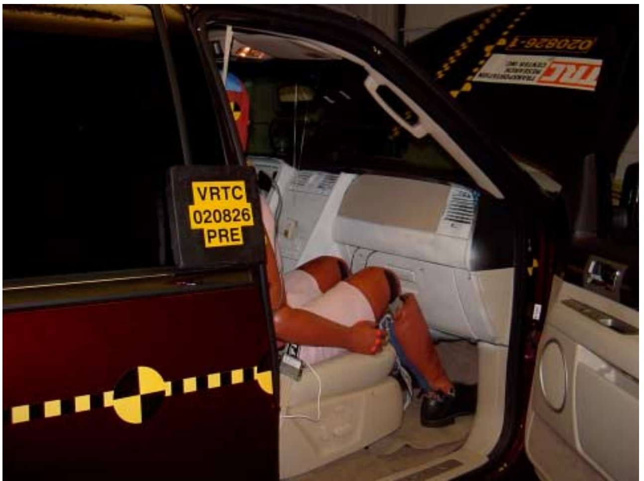
Figure A-57 Pre-Test Passenger Dummy & Vehicle Interior - View 2
