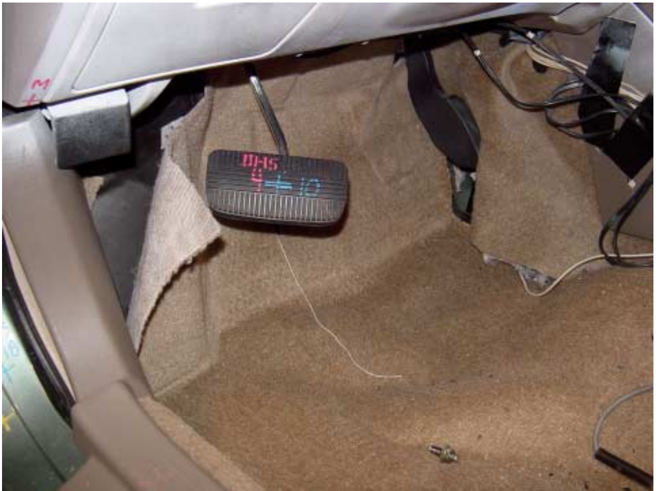
Figure A-72 Post-Test Driver Toeboard/Floorpan with Carpet Removed View
