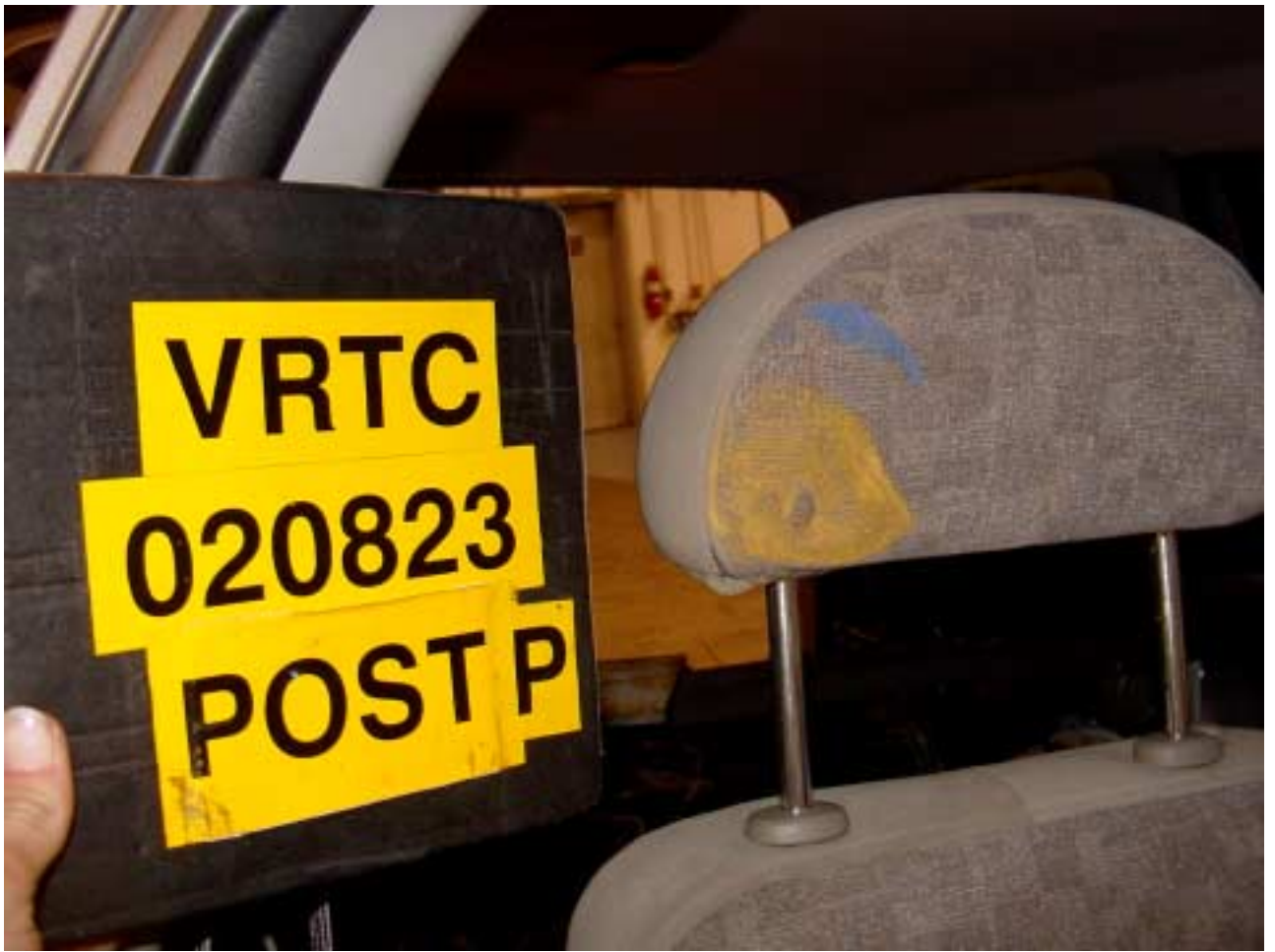
Figure A-75 Post-Test Passenger Dummy Head Contact - View 3
