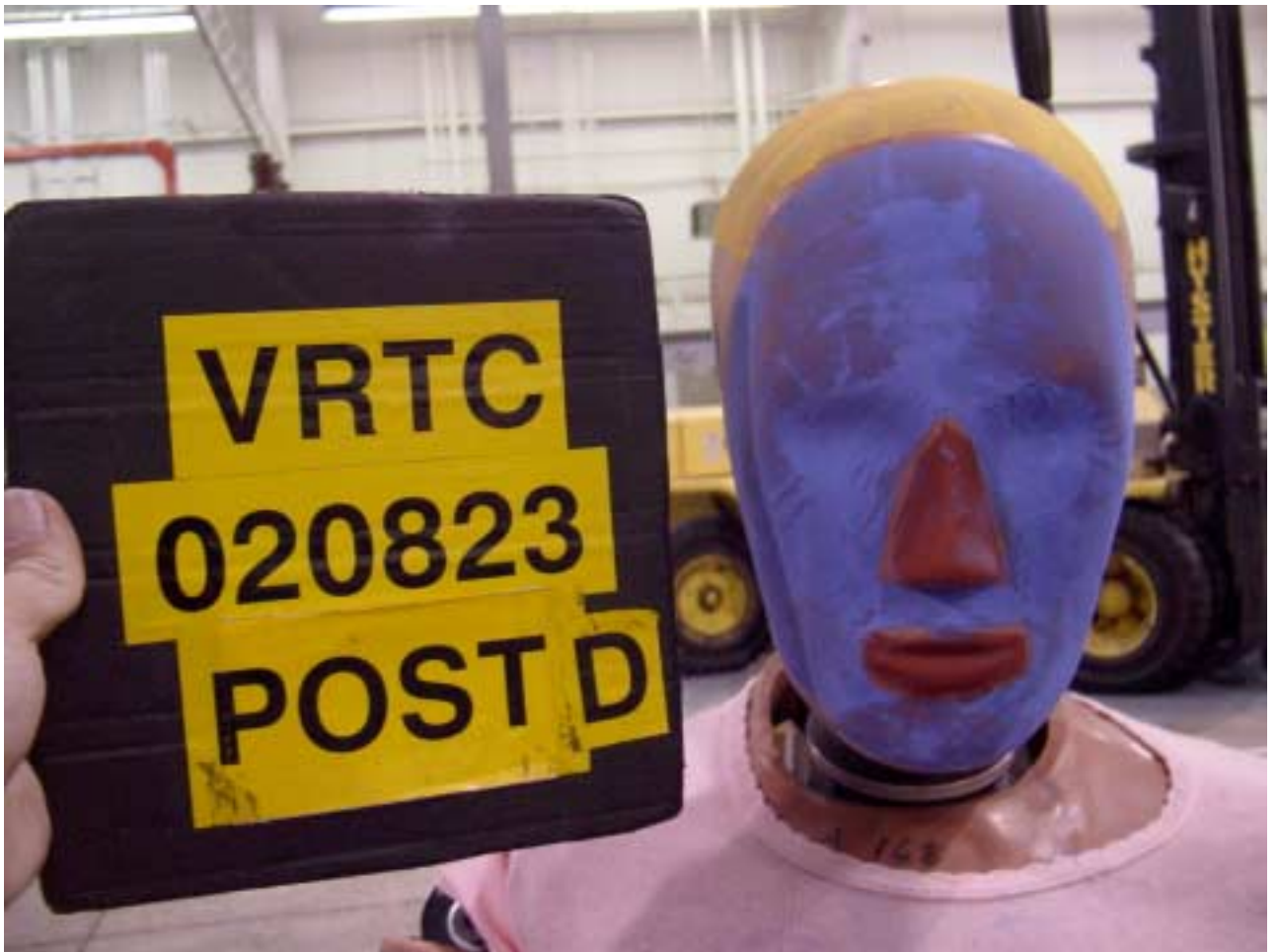
Figure A-63 Post-Test Driver Dummy Head Contact - View 1
