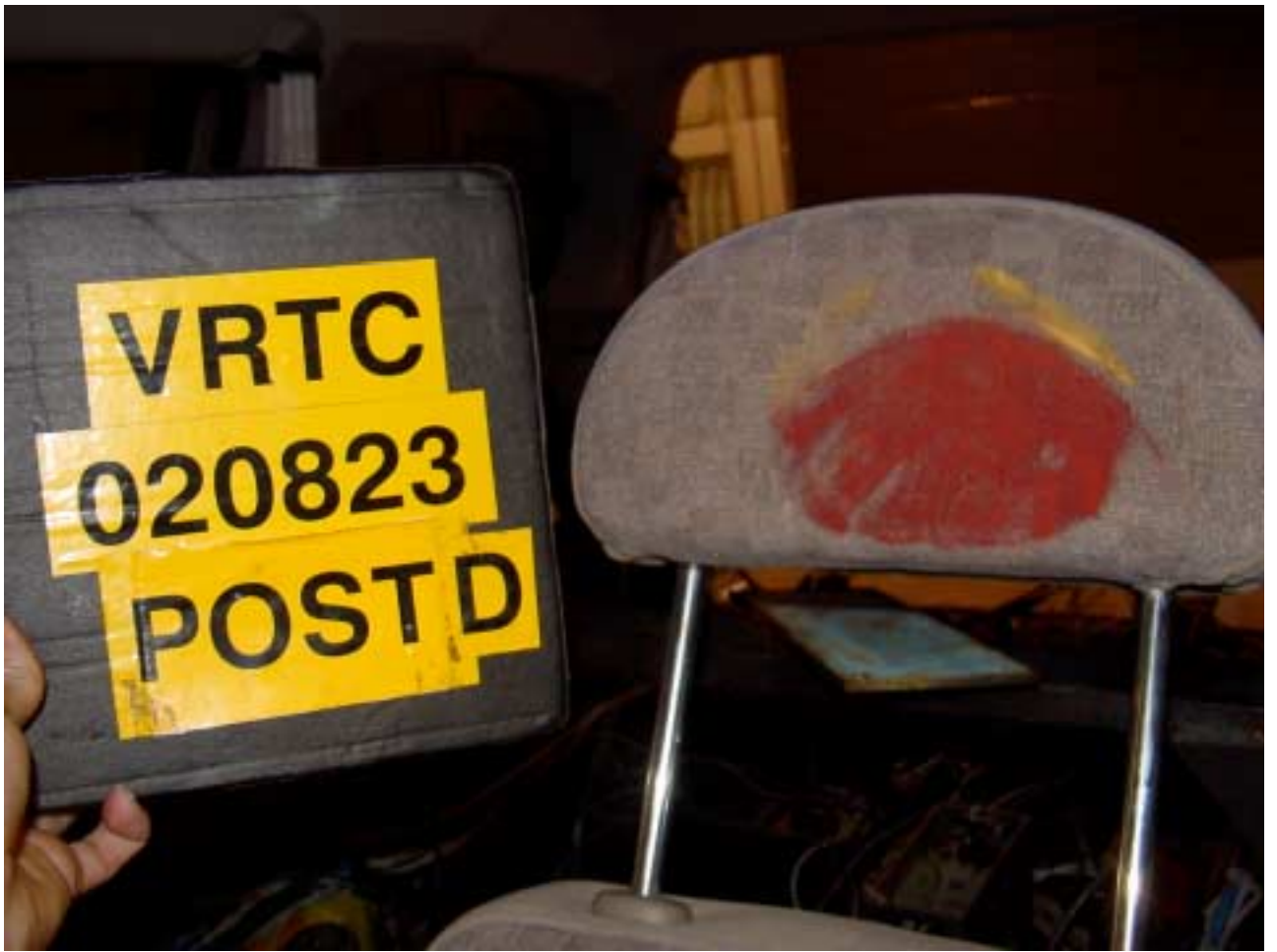
Figure A-65 Post-Test Driver Dummy Head Contact - View 3
