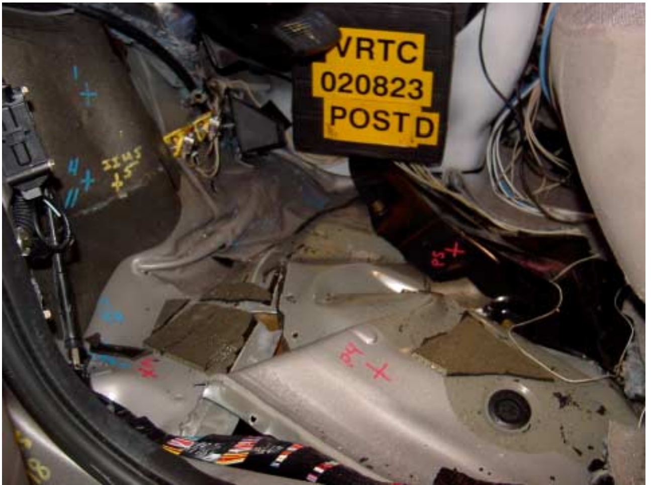
Figure A-70 Post-Test Driver Toeboard/Floorpan with Carpet Removed – View 1
