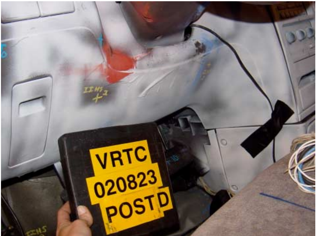
Figure A-67 Post-Test Driver Dummy Knee Contact - View 2
