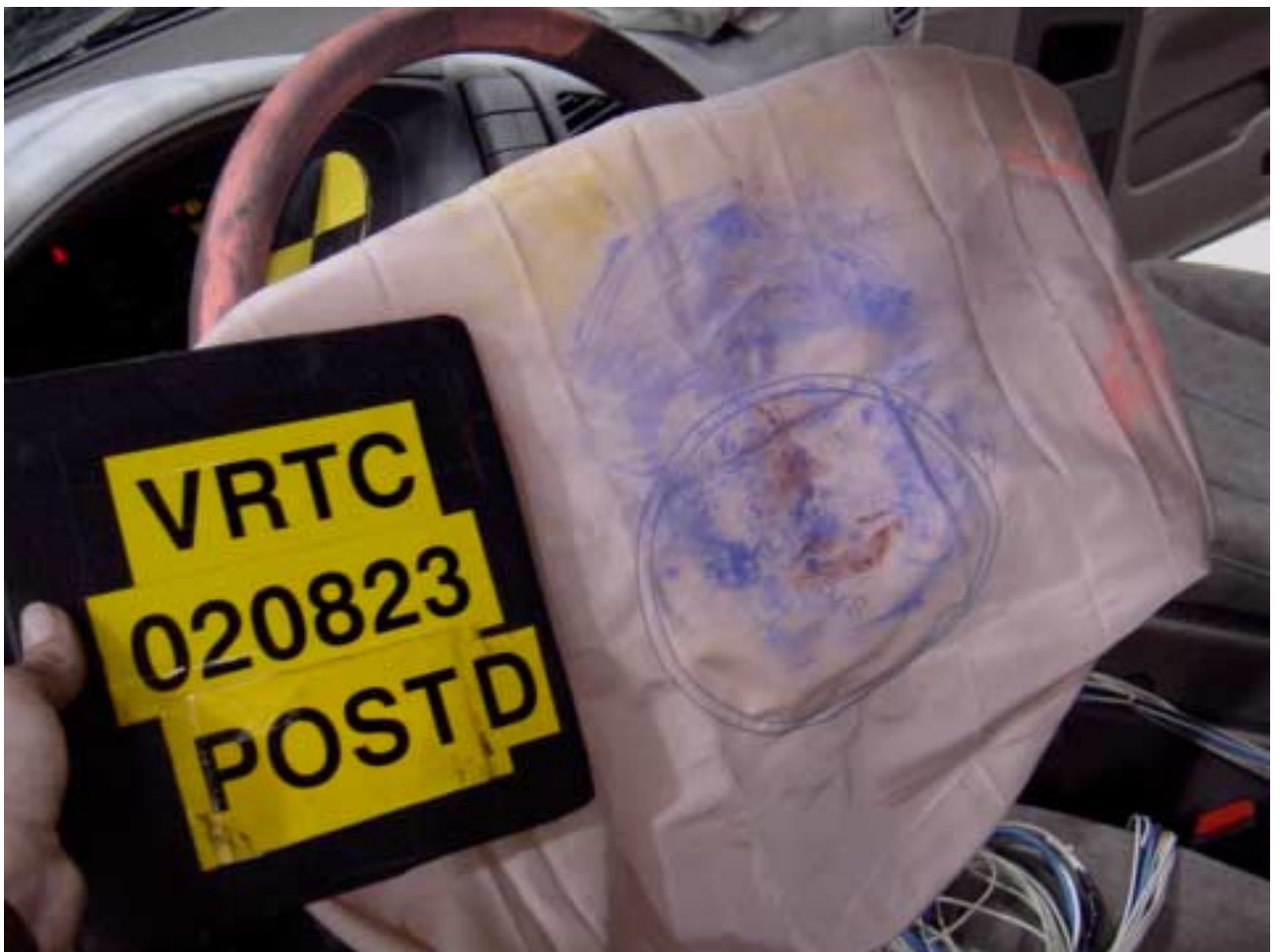
Figure A-64 Post-Test Driver Dummy Head Contact - View 2
