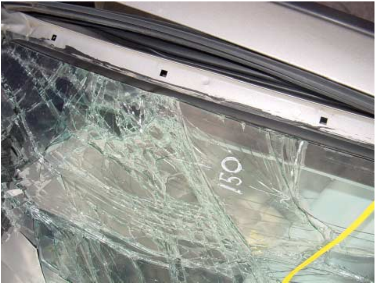
Figure A-33. Post-Test Left Side Windshield Closeup View
