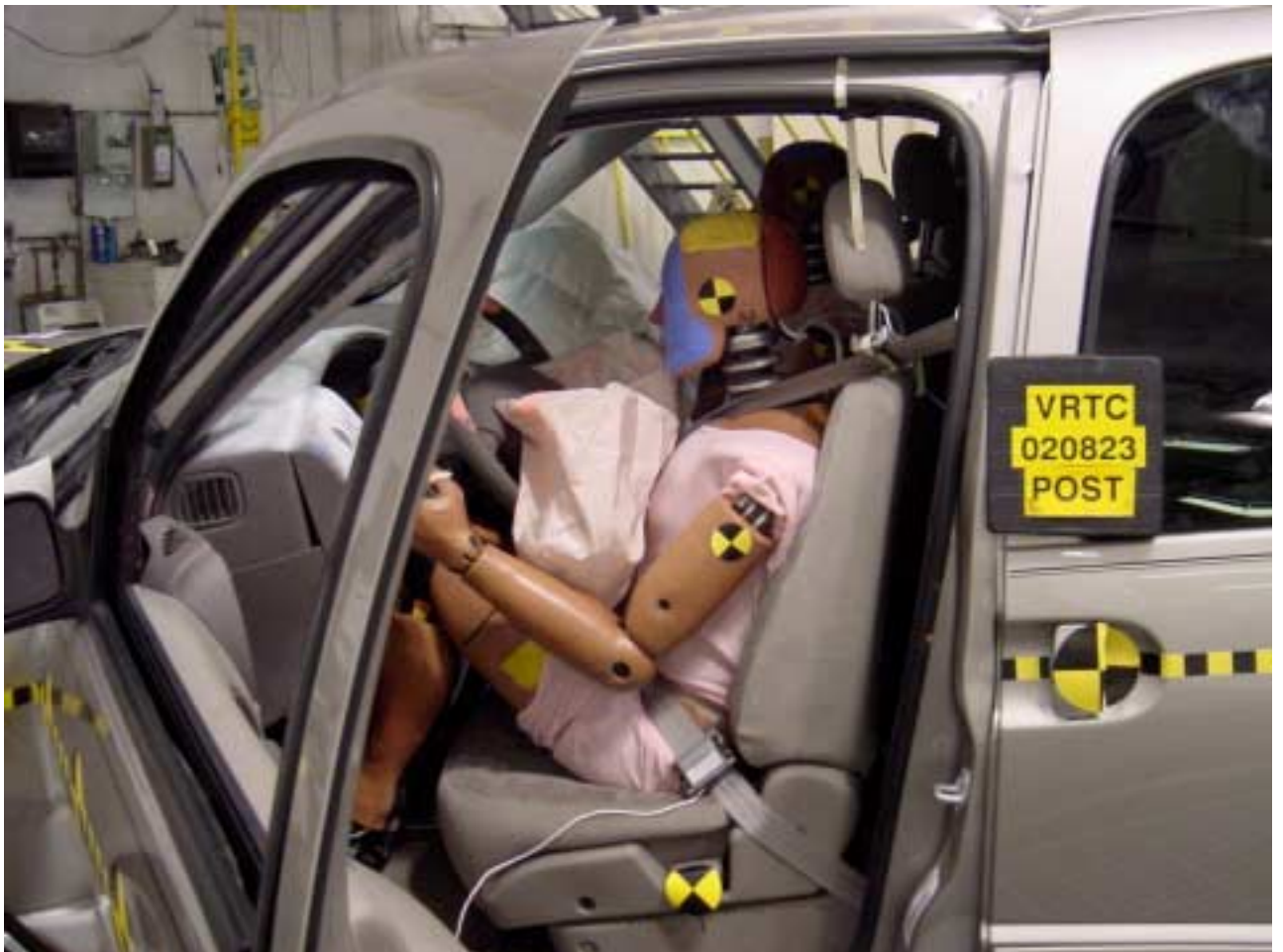
Figure A-51 Post-Test Driver Dummy & Vehicle Interior - View 1
