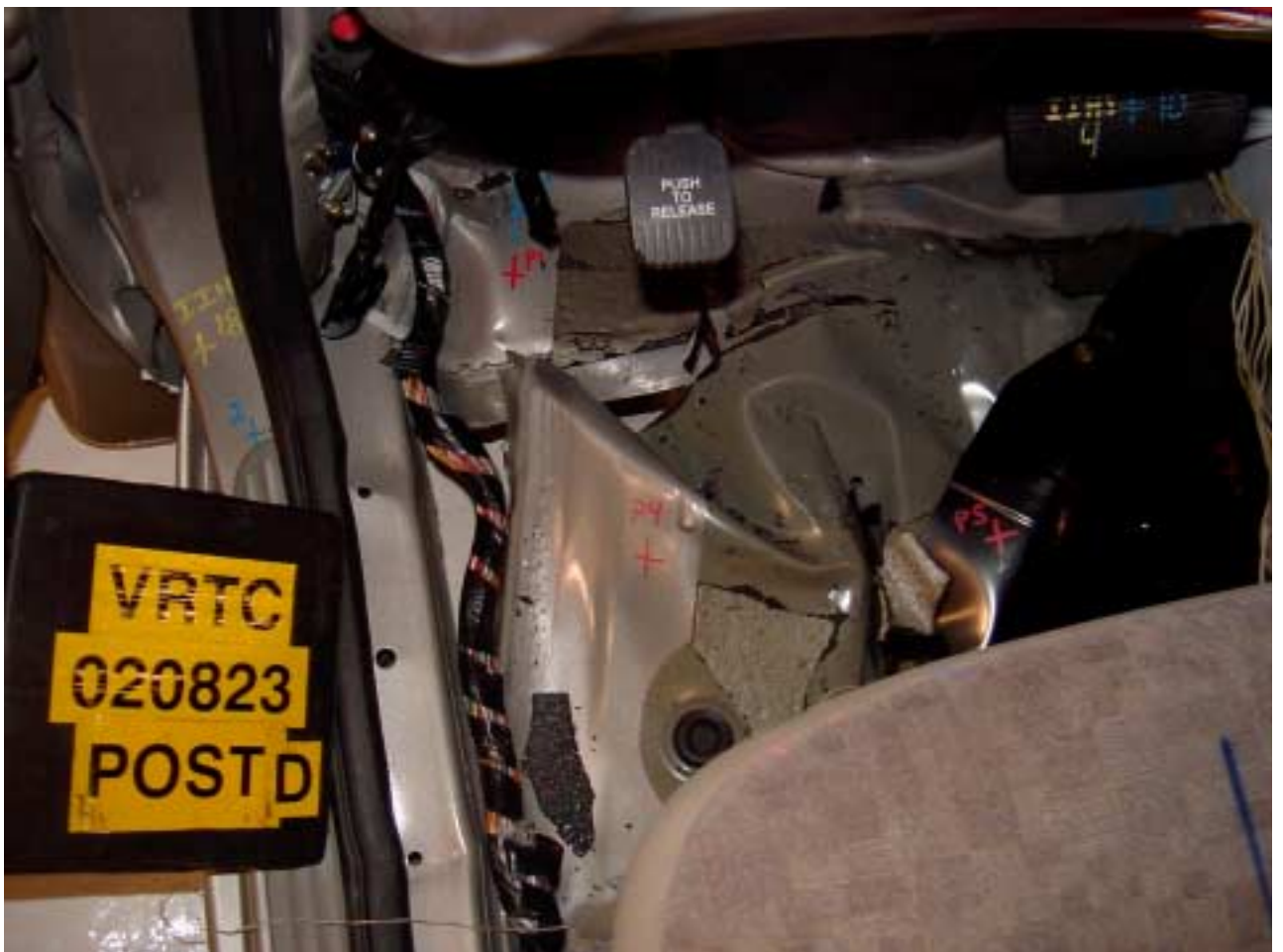
Figure A-71 Post-Test Driver Toeboard/Floorpan with Carpet Removed – View 2
