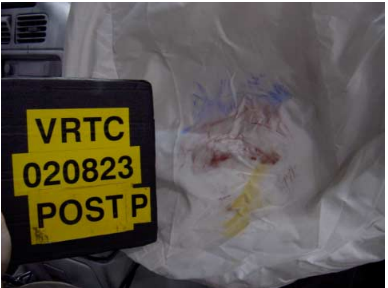
Figure A-74 Post-Test Passenger Dummy Head Contact - View 2
