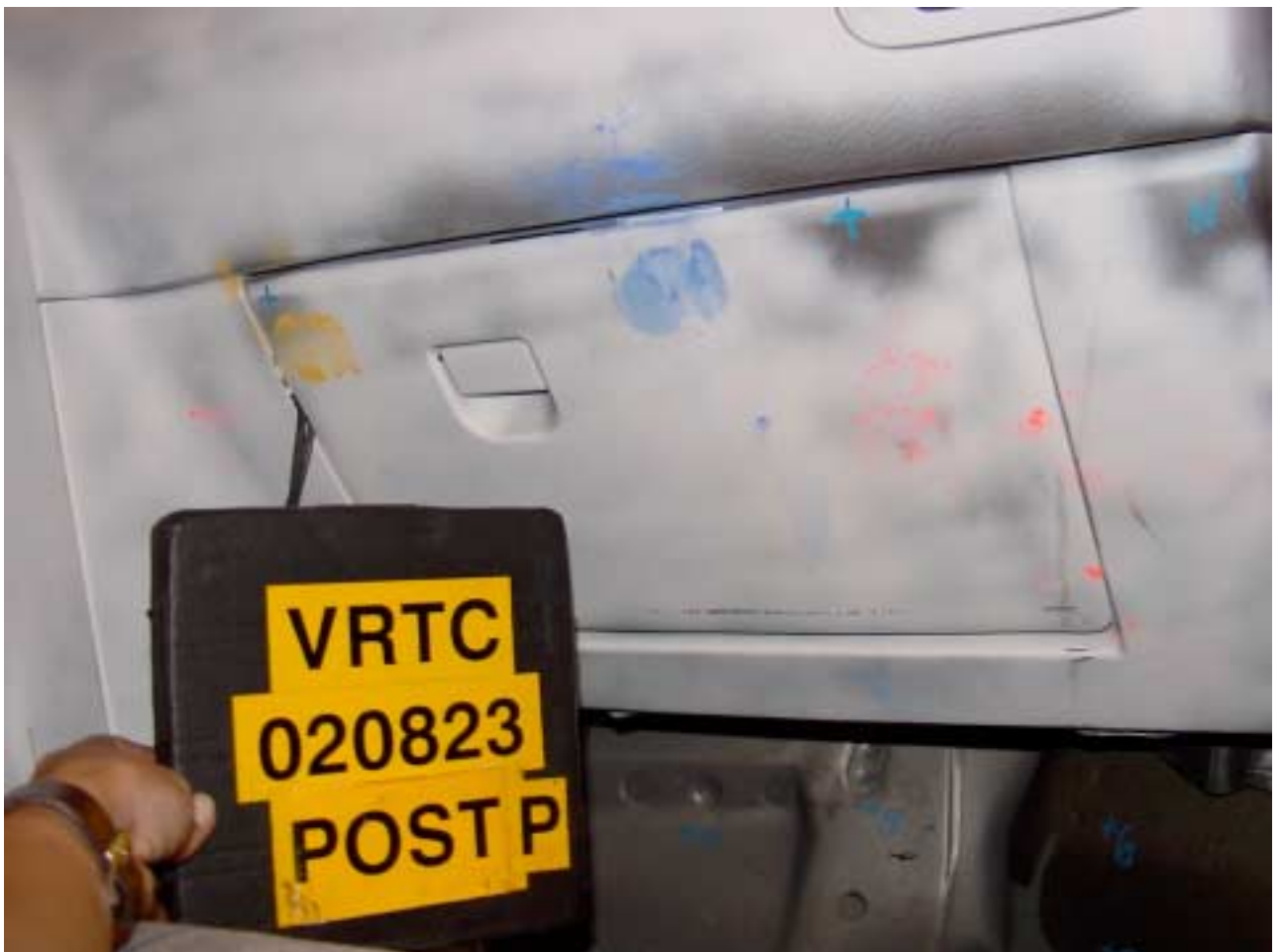
Figure A-77 Post-Test Passenger Dummy Knee Contact - View 2
