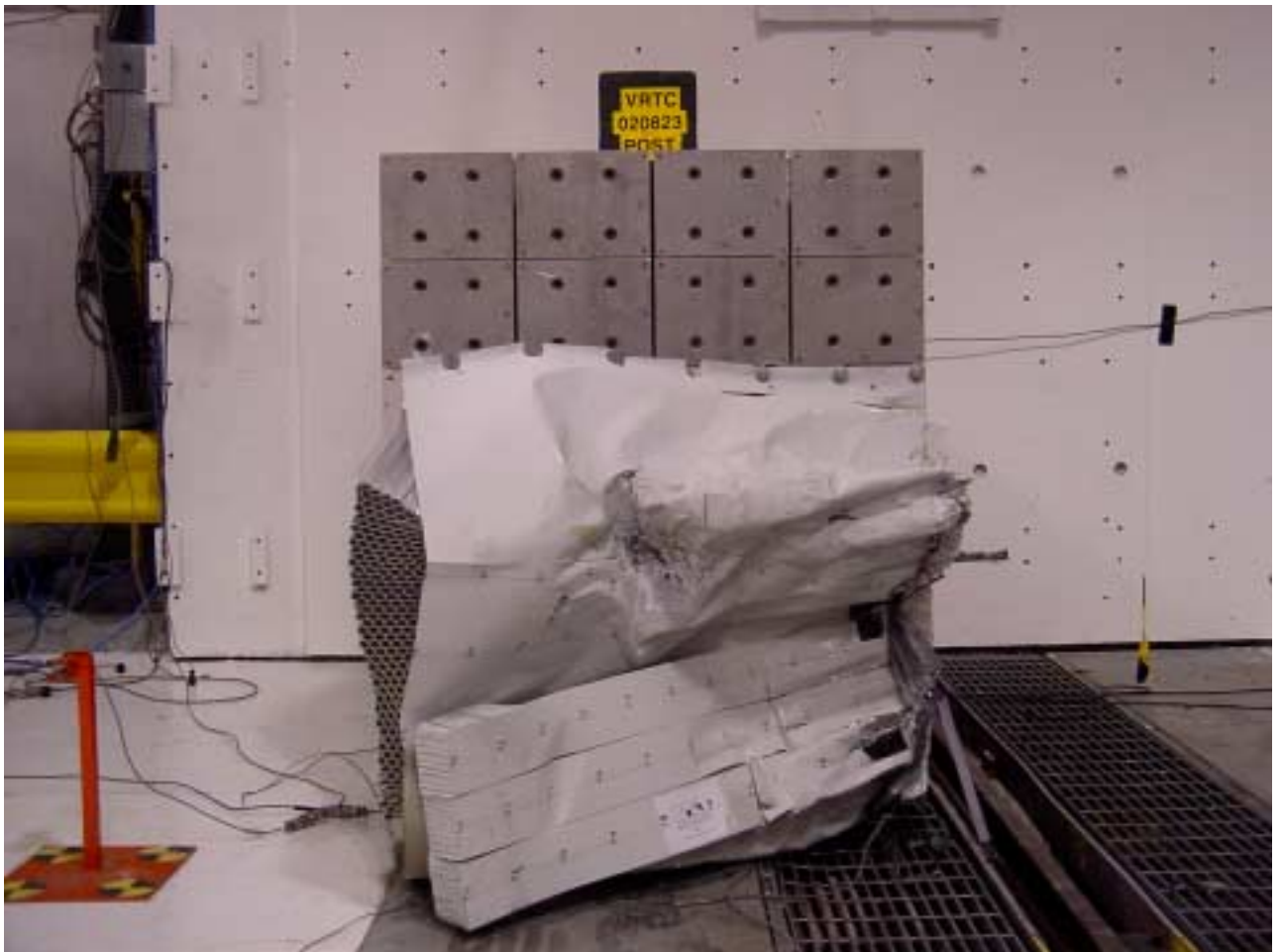
Figure A-37 Post-Test Front Barrier Face View
