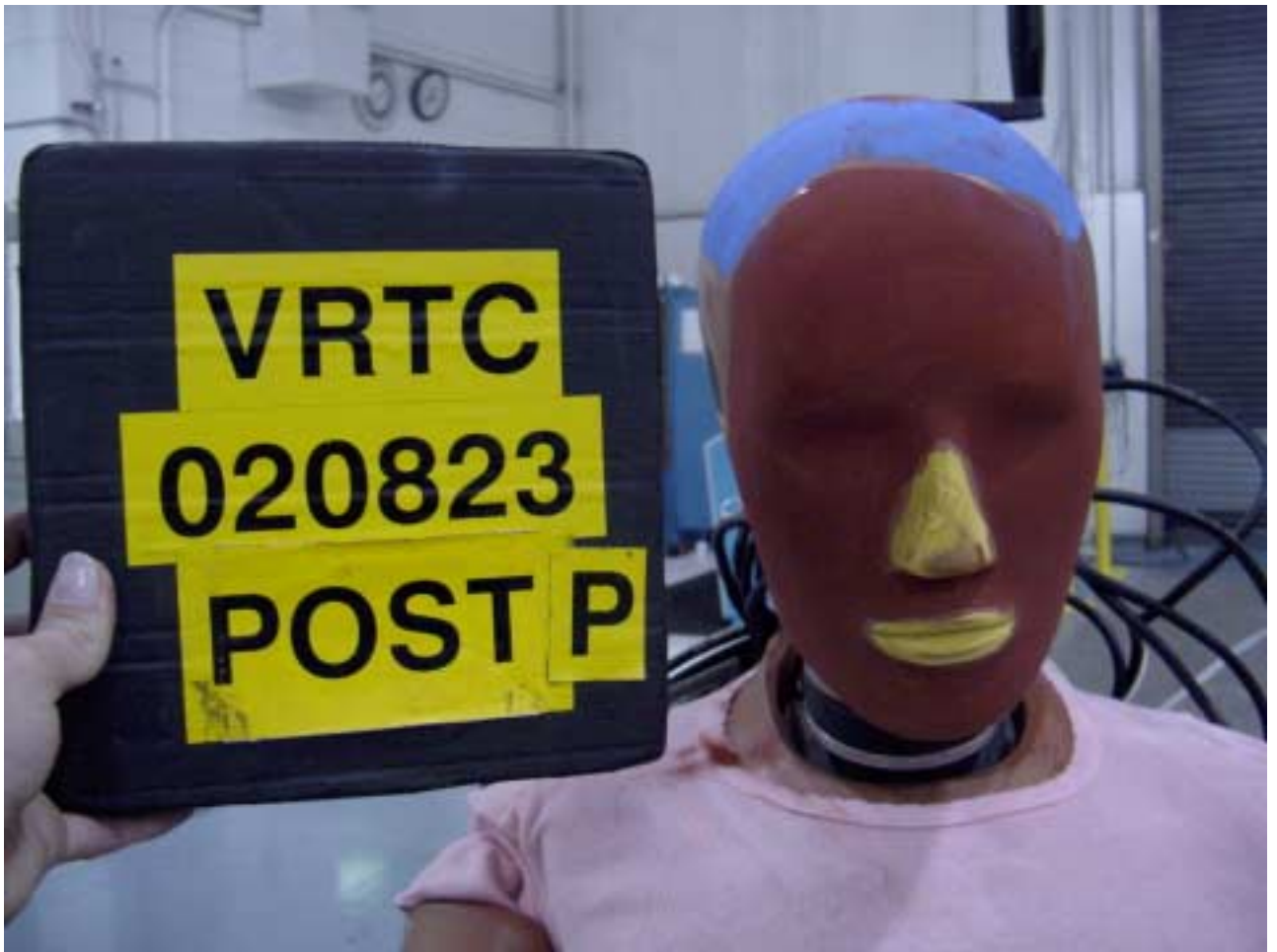
Figure A-73 Post-Test Passenger Dummy Head Contact - View 1
