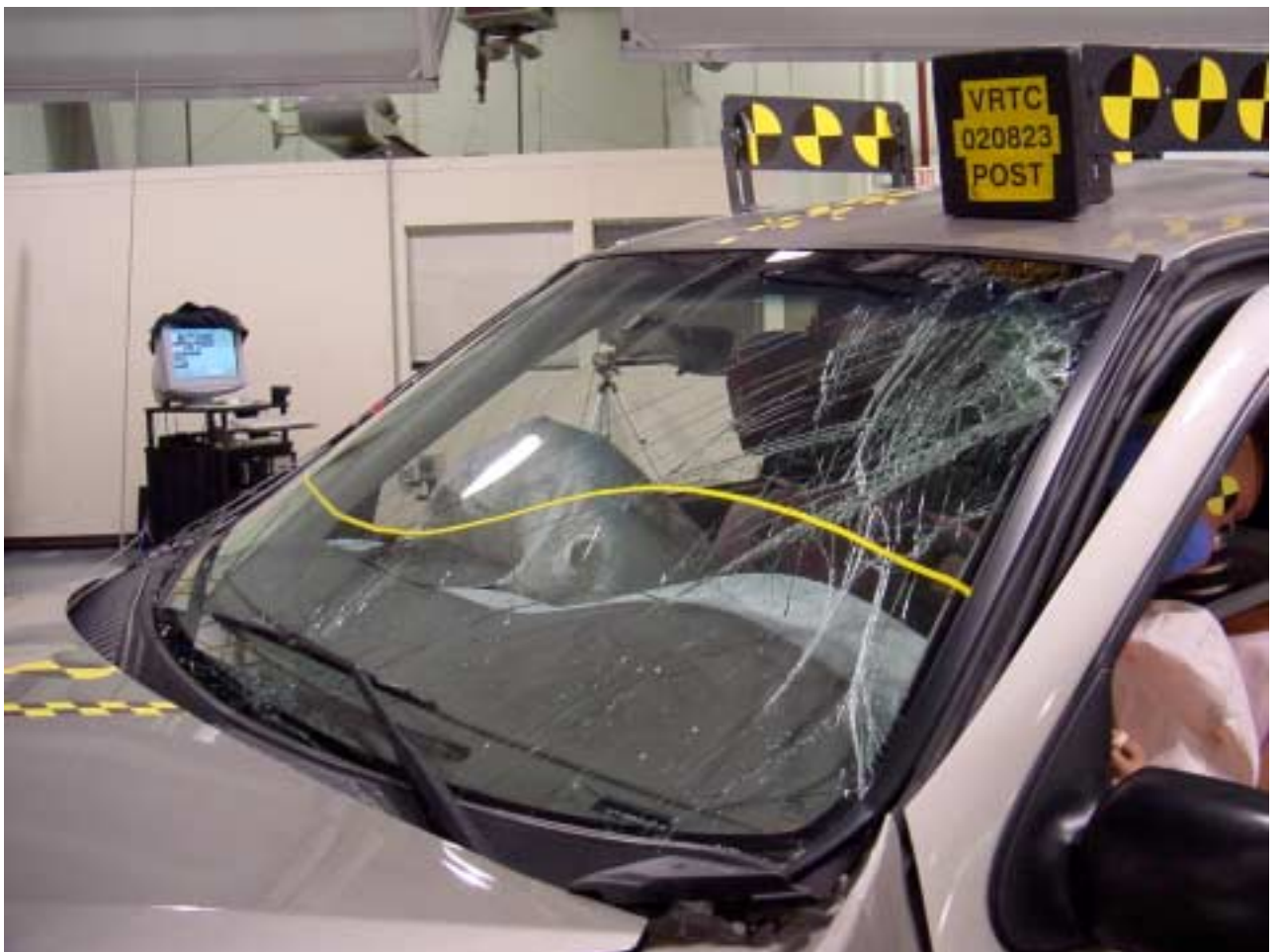
Figure A-32 Post-Test Left Side Angled Windshield View
