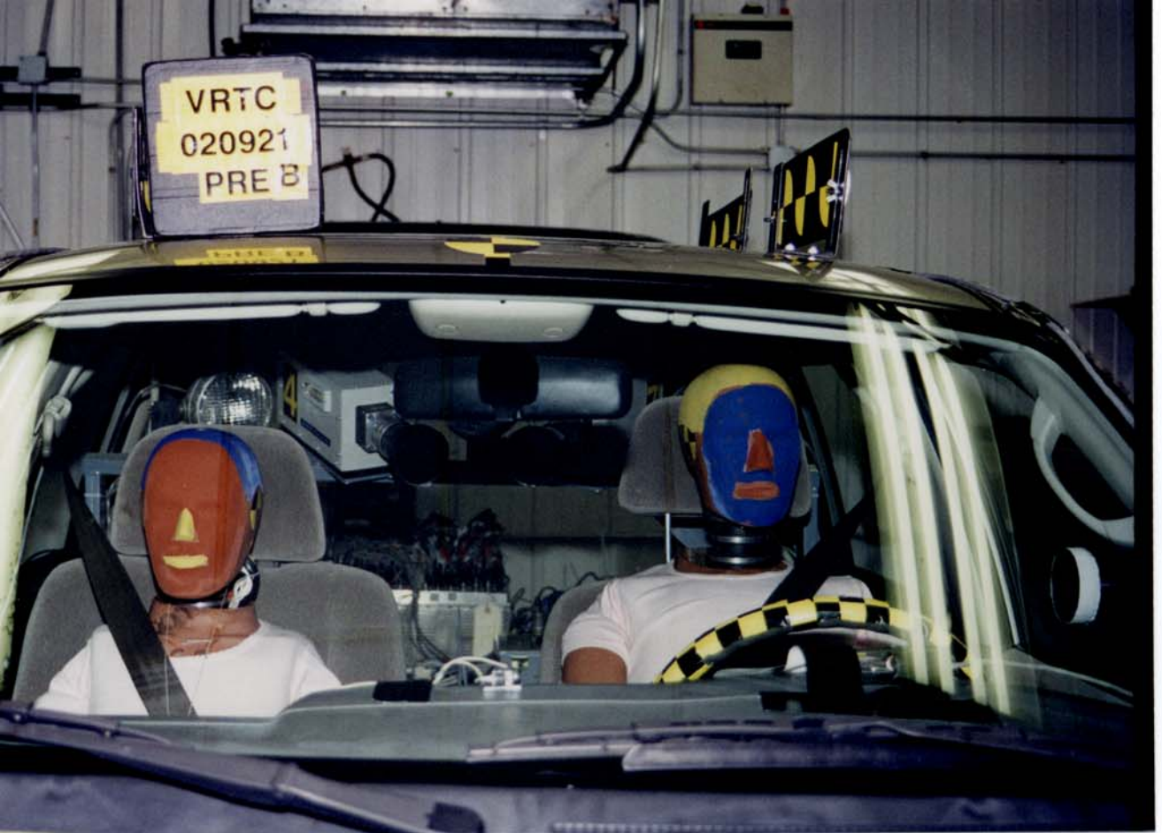
Figure A-64 Pre-Test Bullet Vehicle Driver and Passenger Dummies through Windshield View
