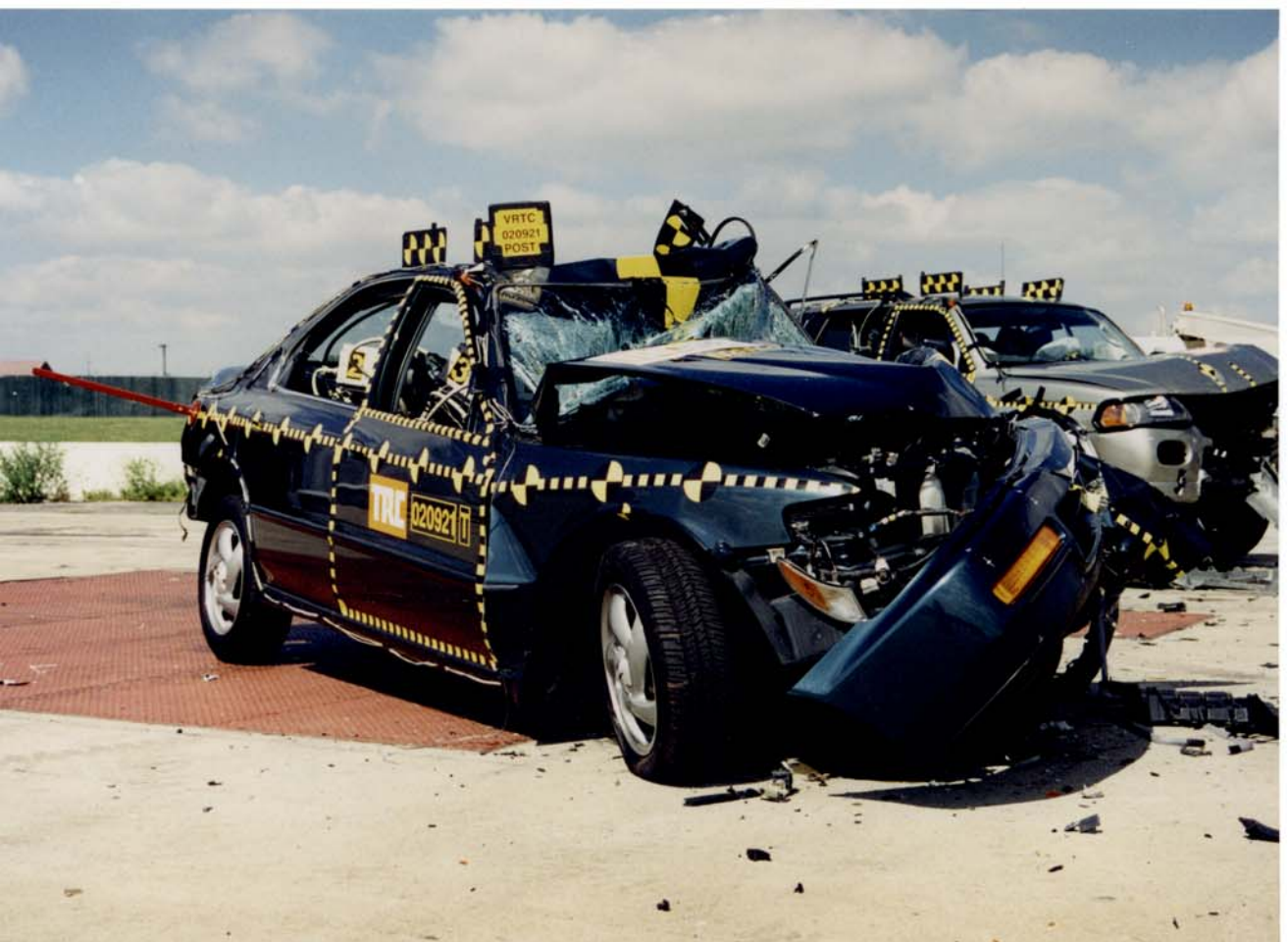
Figure A-18 Post-Test Target Vehicle Right Front View
