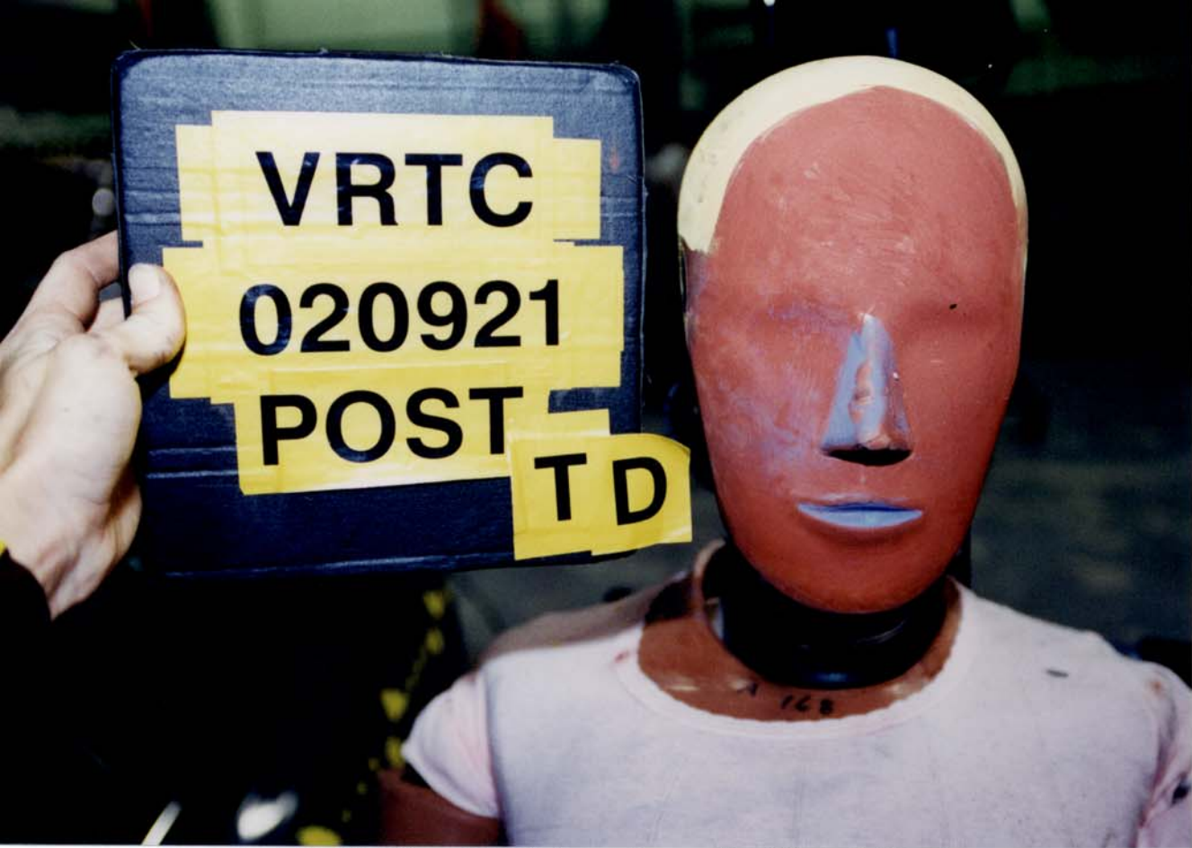
Figure A-83 Post-Test Target Vehicle Driver Dummy Head Contact - View 1
