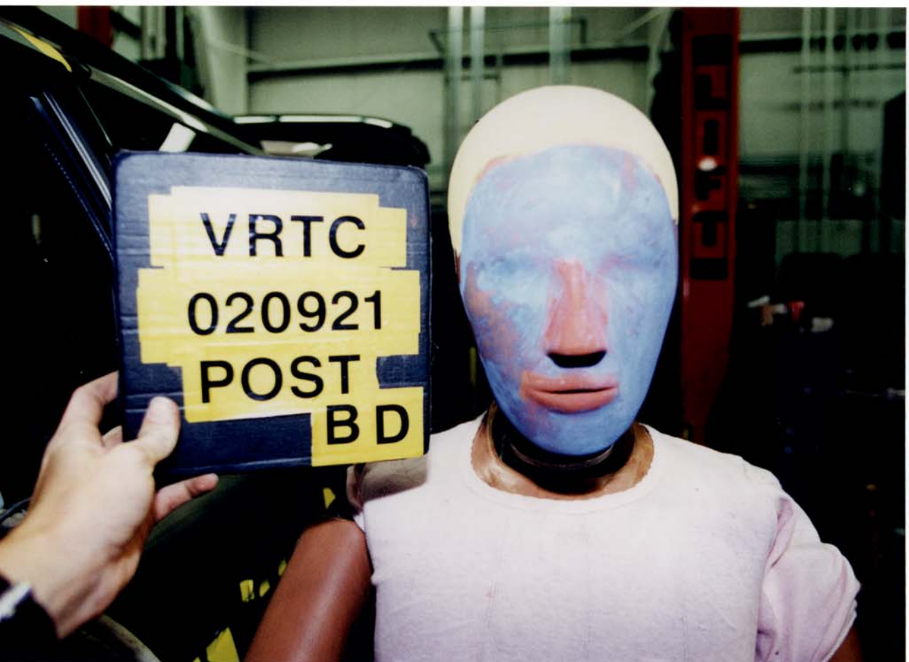
Figure A-94 Post-Test Bullet Vehicle Driver Dummy Head Contact - View 1
