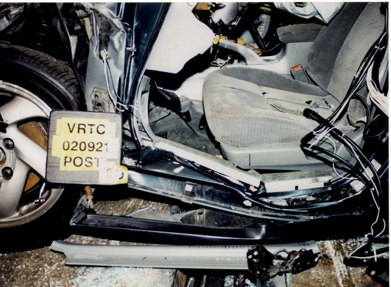
Figure A-92 Post-Test Target Vehicle Deformation - View 2
