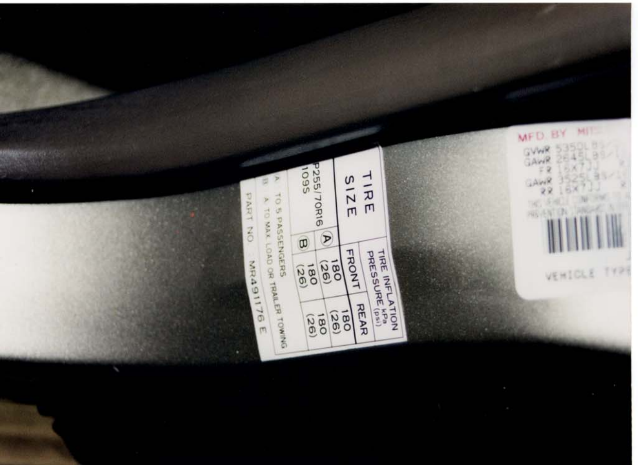
Figure A-110 Bullet Vehicle Tire Load Label View
