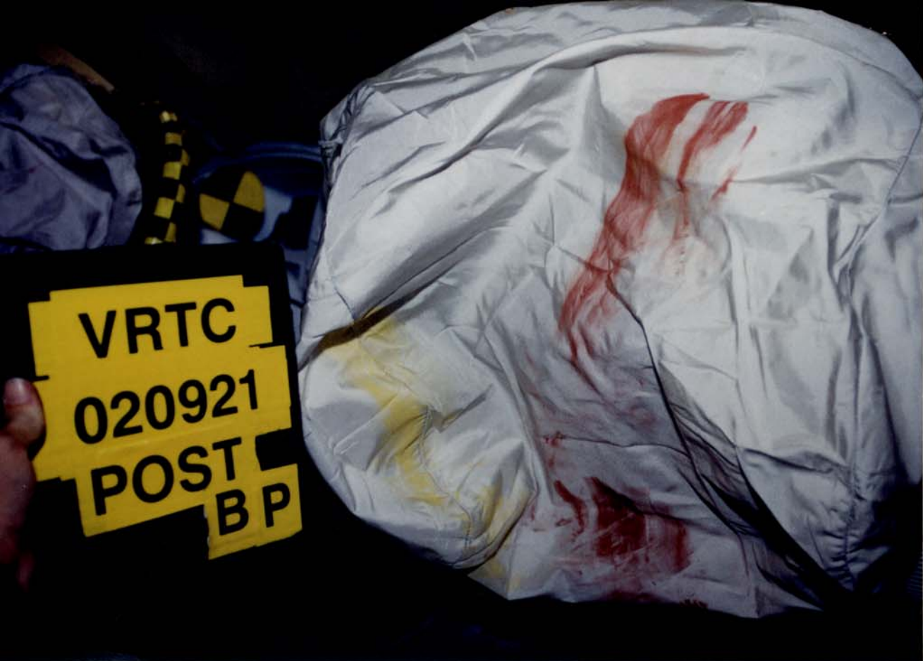
Figure A-103 Post-Test Bullet Vehicle Passenger Dummy Head Contact - View 3
