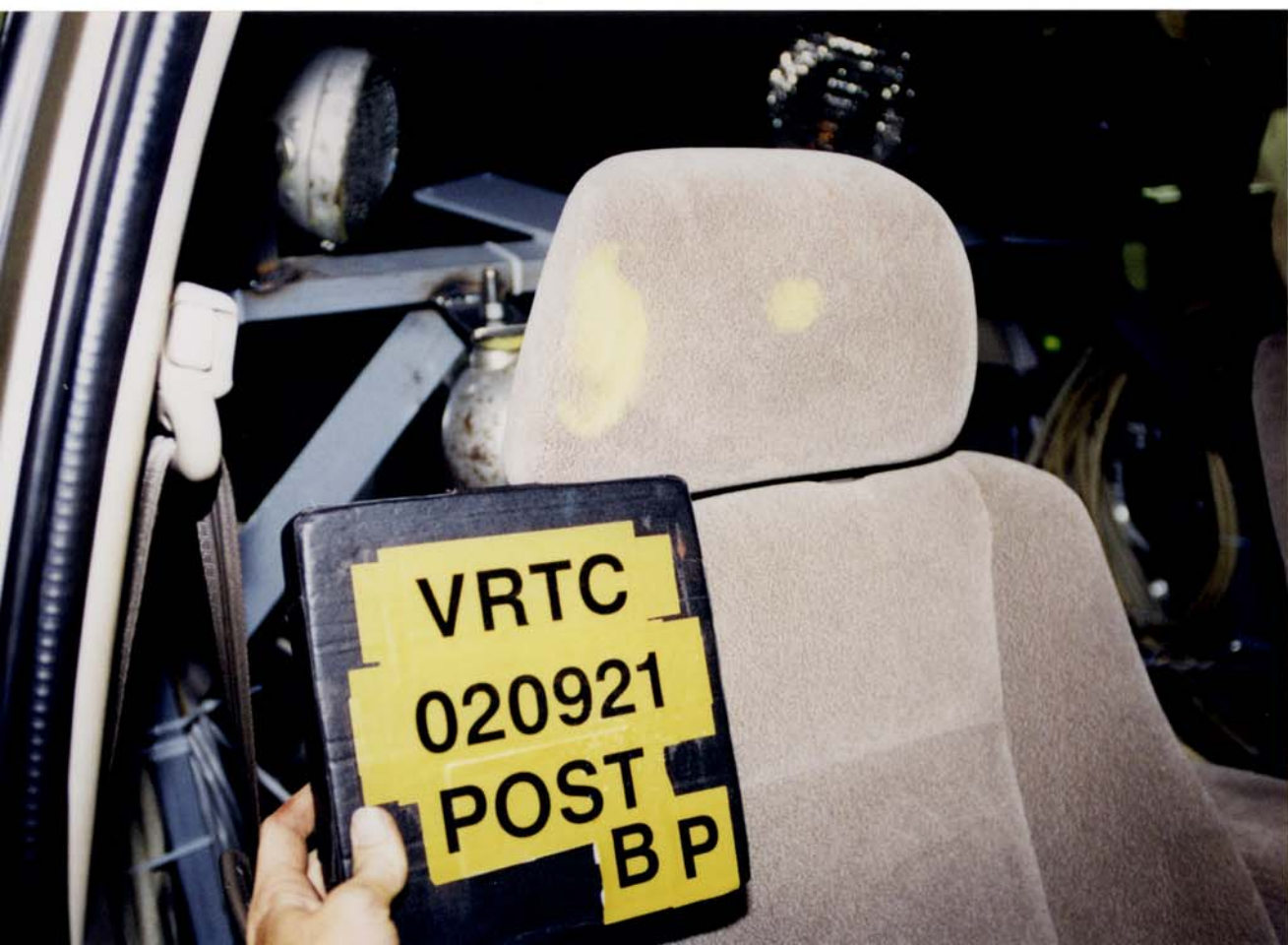
Figure A-104 Post-Test Bullet Vehicle Passenger Dummy Head Contact - View 4
