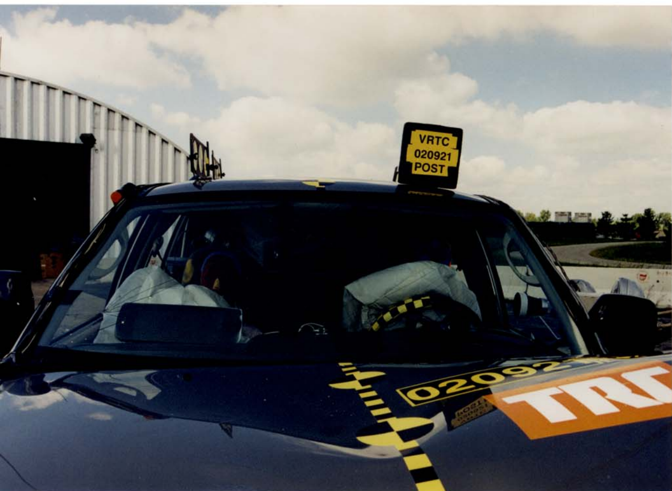
Figure A-44 Post-Test Windshield View
