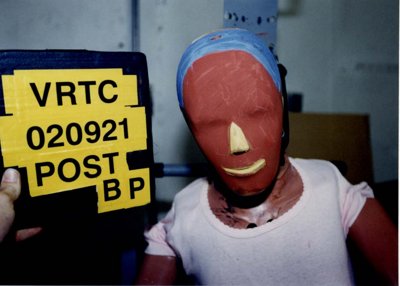
Figure A-101 Post-Test Bullet Vehicle Passenger Dummy Head Contact - View 1
