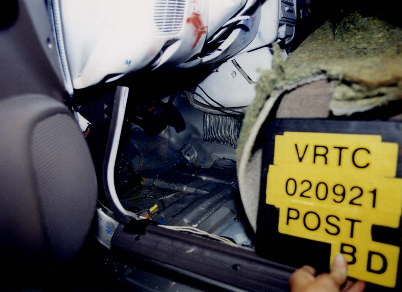
Figure A-99 Post-Test Bullet Vehicle Driver Floorpan Deformation View
