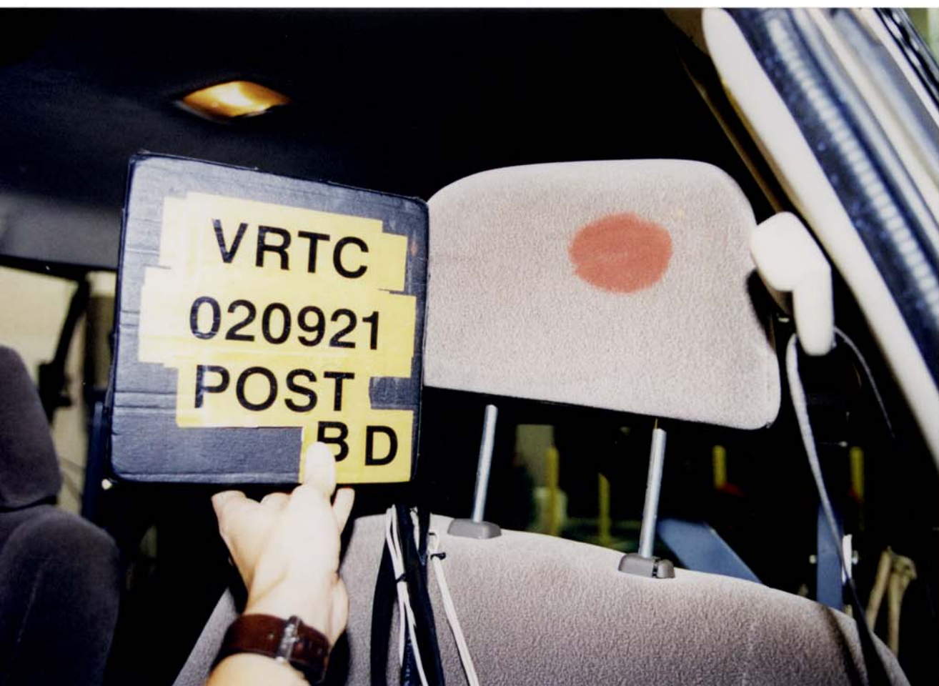
Figure A-96 Post-Test Bullet Vehicle Driver Dummy Head Contact - View 3
