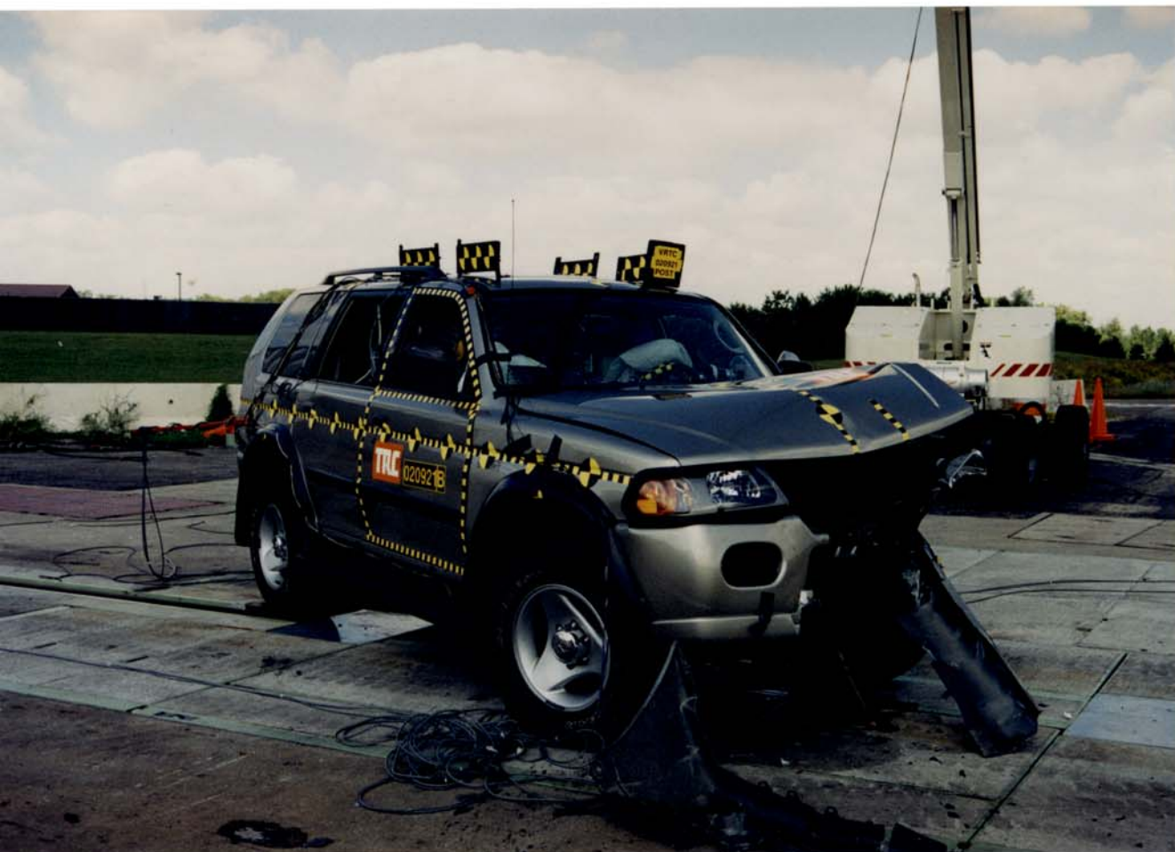
Figure A-42 Post-Test Bullet Vehicle Right Front View
