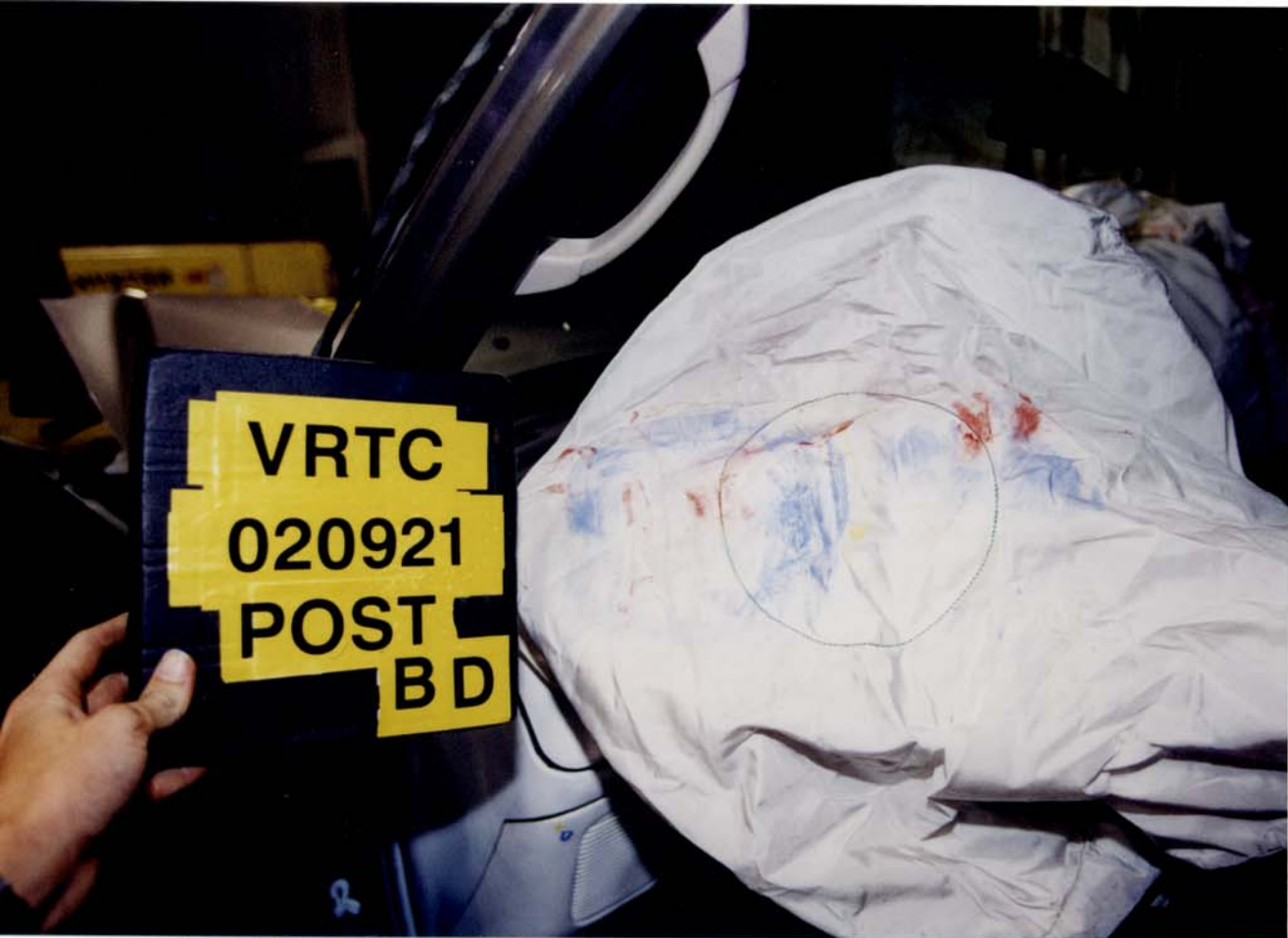
Figure A-95 Post-Test Bullet Vehicle Driver Dummy Head Contact - View 2
