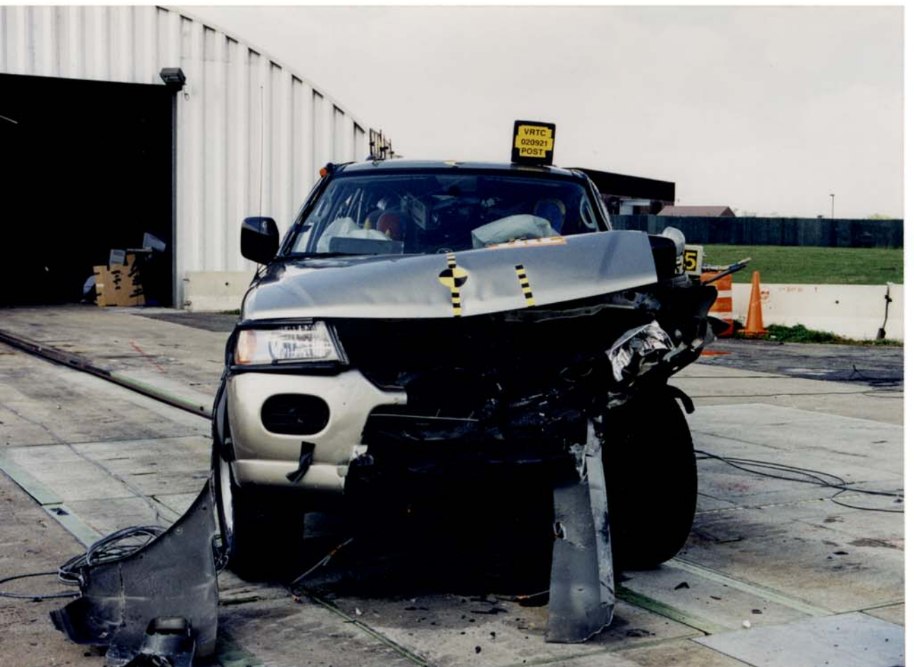
Figure A-28 Post-Test Bullet Vehicle Front View
