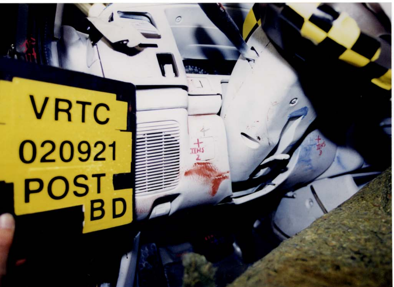
Figure A-98 Post-Test Bullet Vehicle Driver Dummy Knee Contact - View 2
