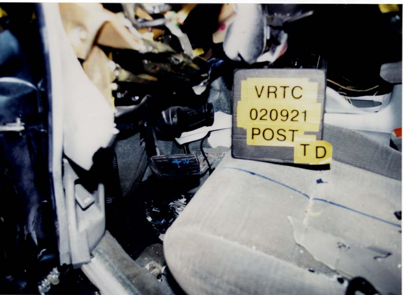
Figure A-90 Post-Test Target Vehicle Driver Floorpan Deformation
