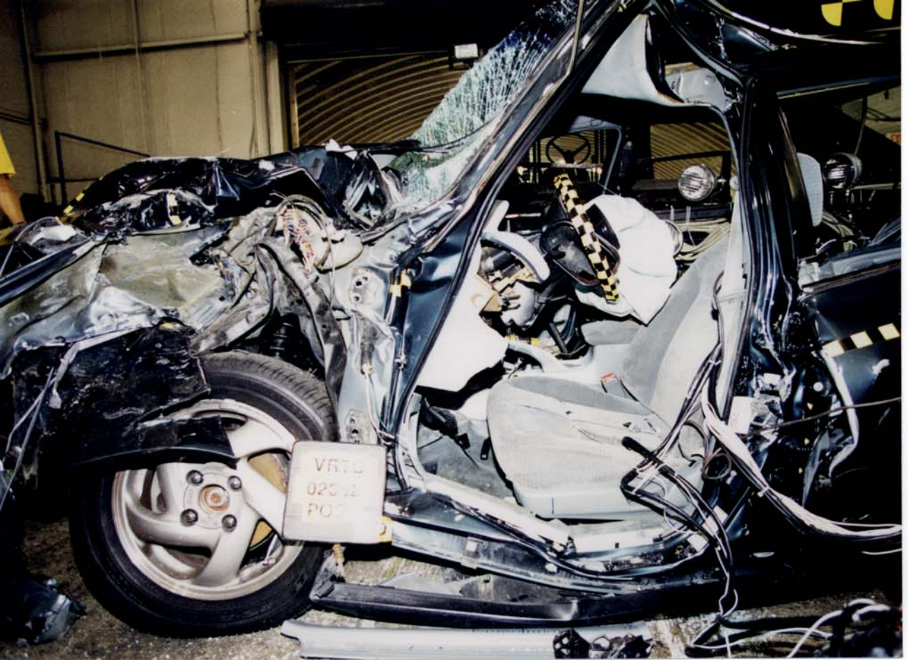
Figure A-91 Post-Test Target Vehicle Deformation - View 1
