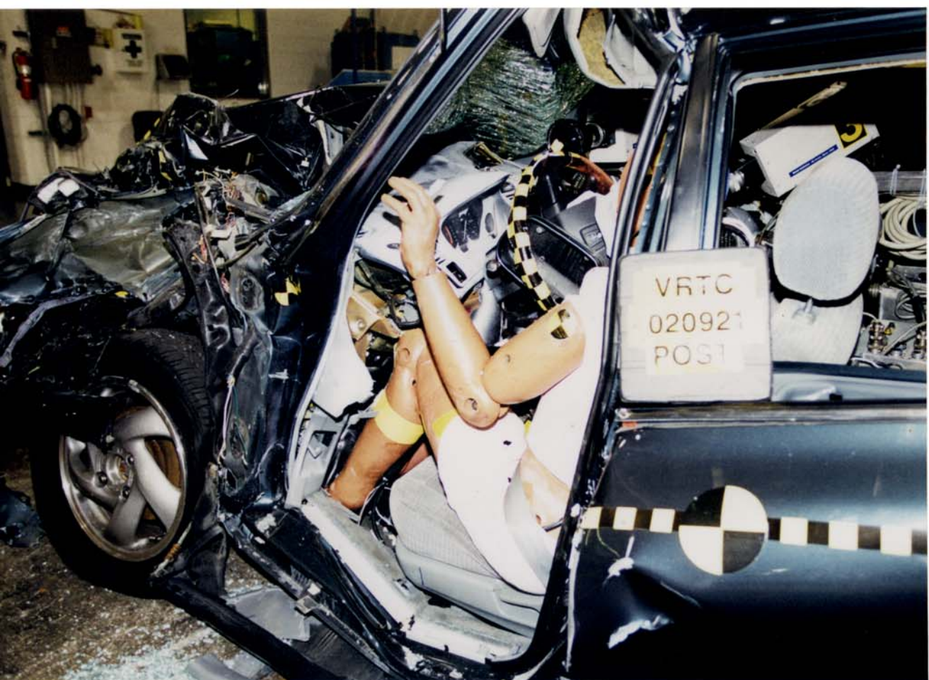
Figure A-63 Post-Test Target Vehicle Driver Dummy - View 4
