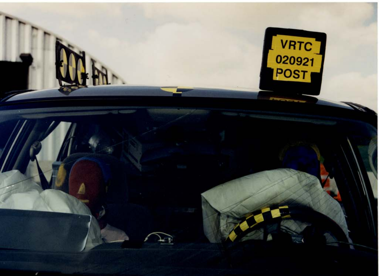
Figure A-65 Post-Test Bullet Vehicle Driver and Passenger Dummies through Windshield View
