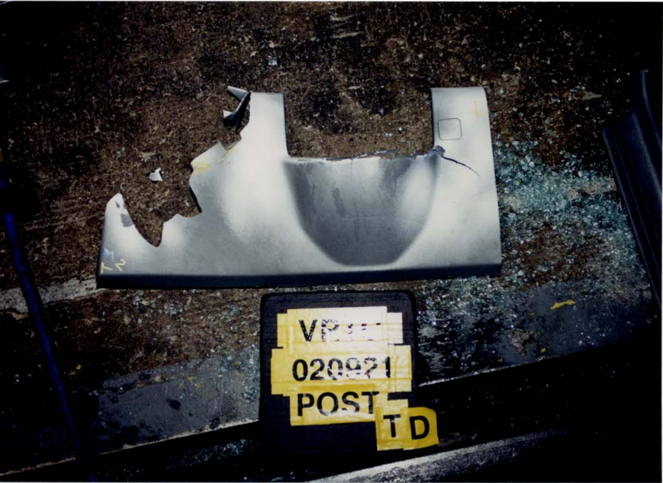
Figure A-89 Post-Test Target Vehicle Driver Dummy Knee Contact - View 3
