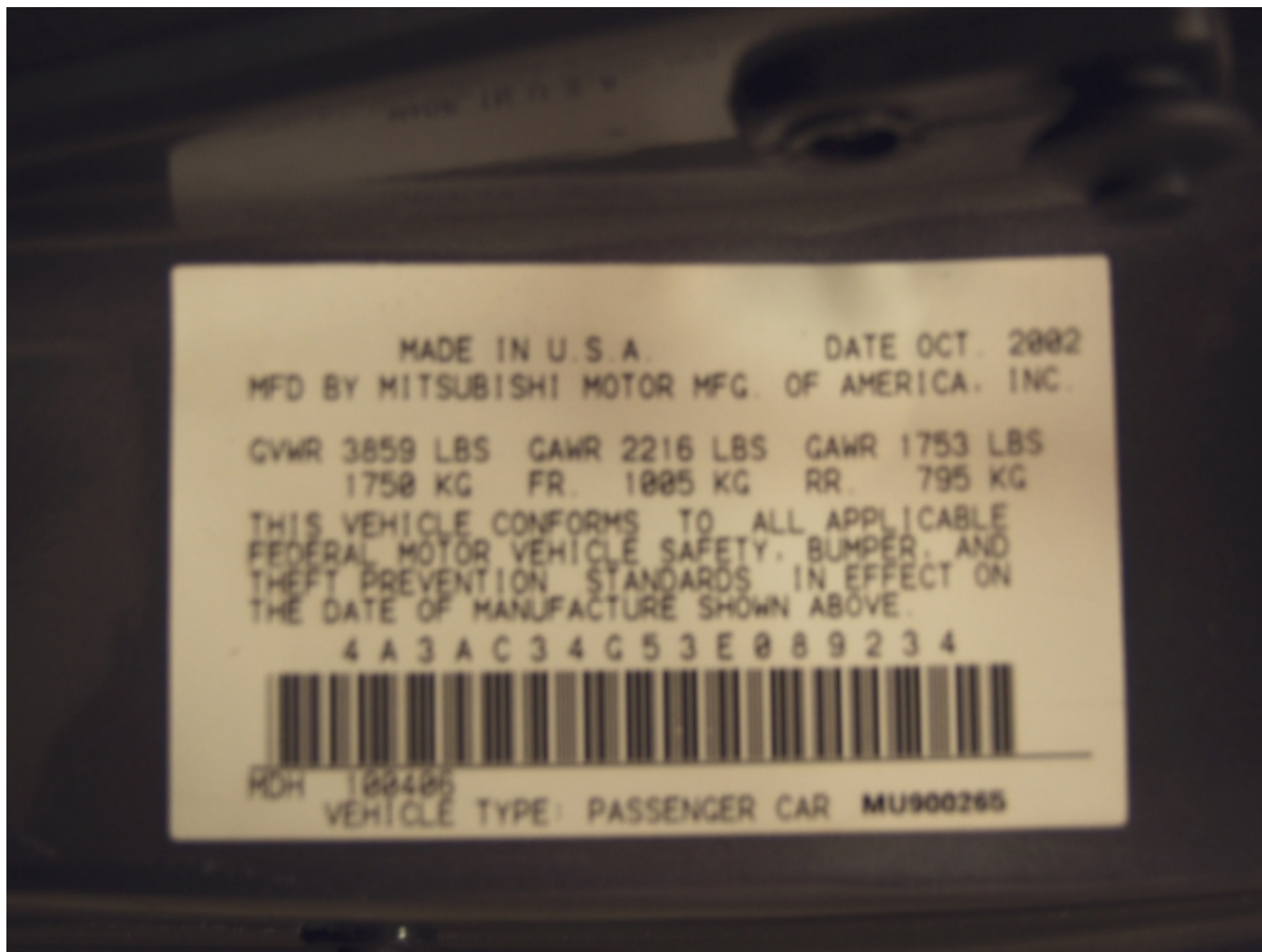
Figure A-31: CLOSE-UP OF VEHICLE'S CERTIFICATION LABELS
