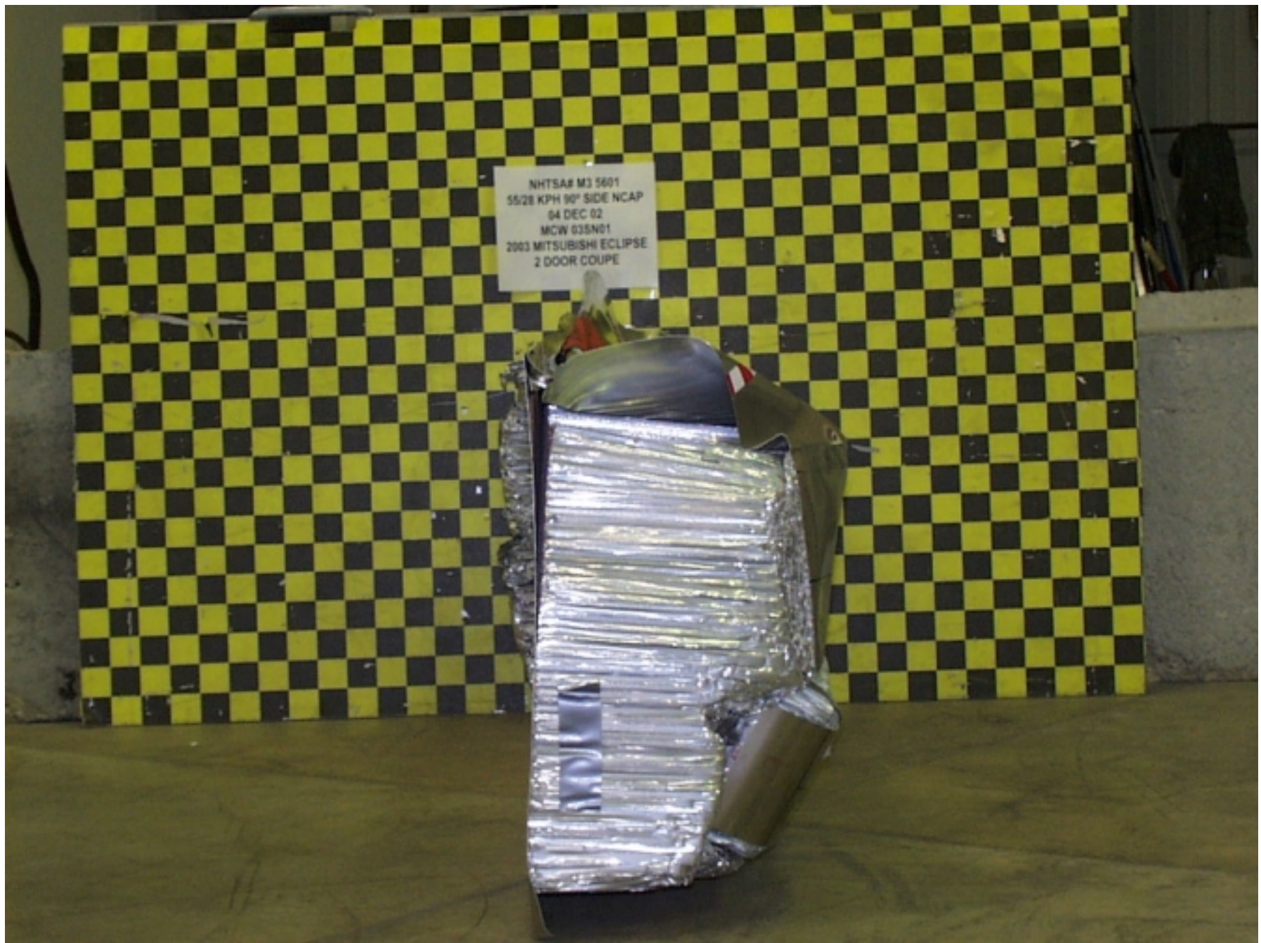
Figure A-44: POST-TEST ALUMINUM BARRIER RIGHT SIDE
