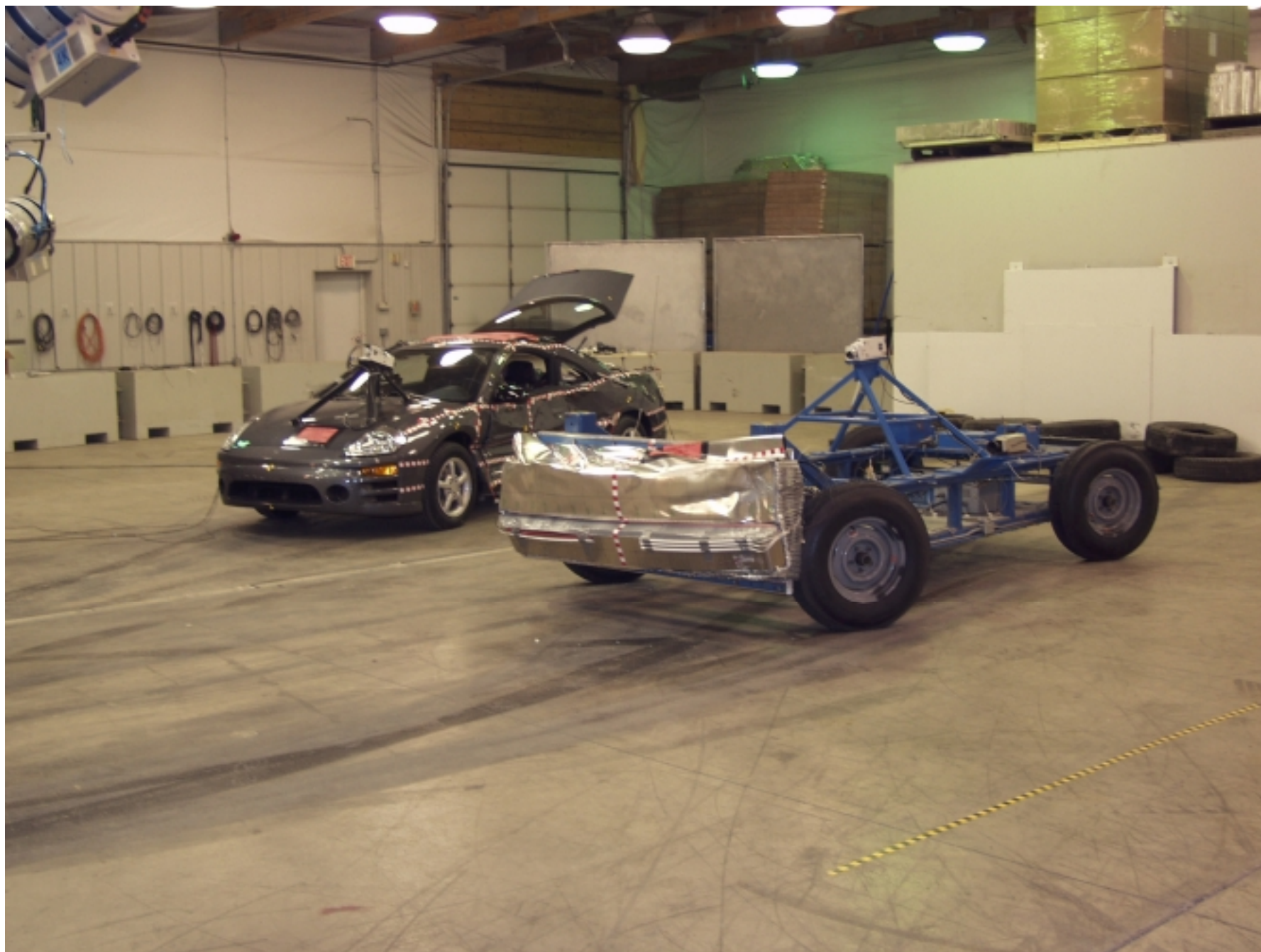
Figure A-24: POST-TEST LEFT SIDE VIEW OF MDB
