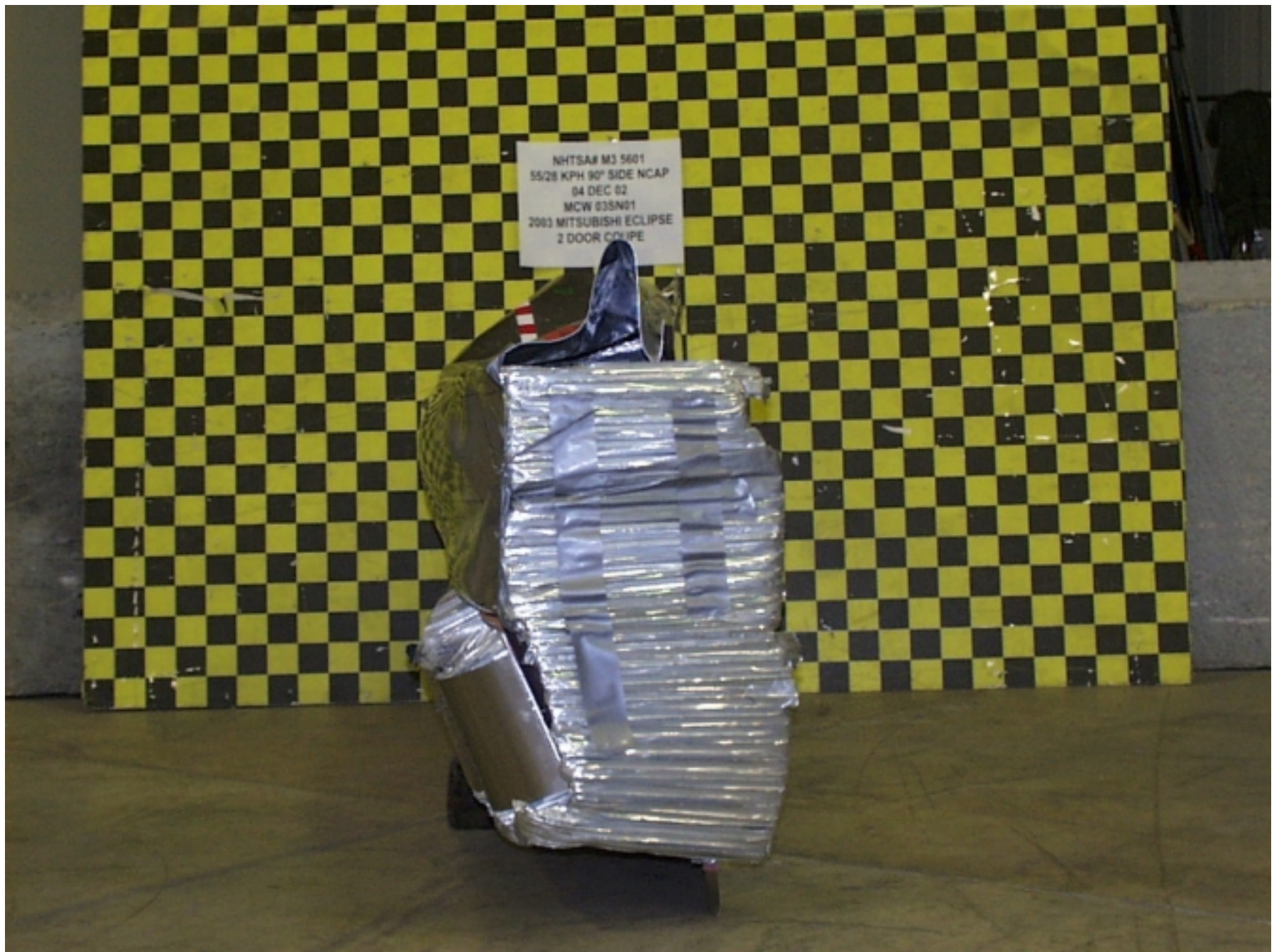
Figure A-42: POST-TEST ALUMINUM BARRIER LEFT SIDE
