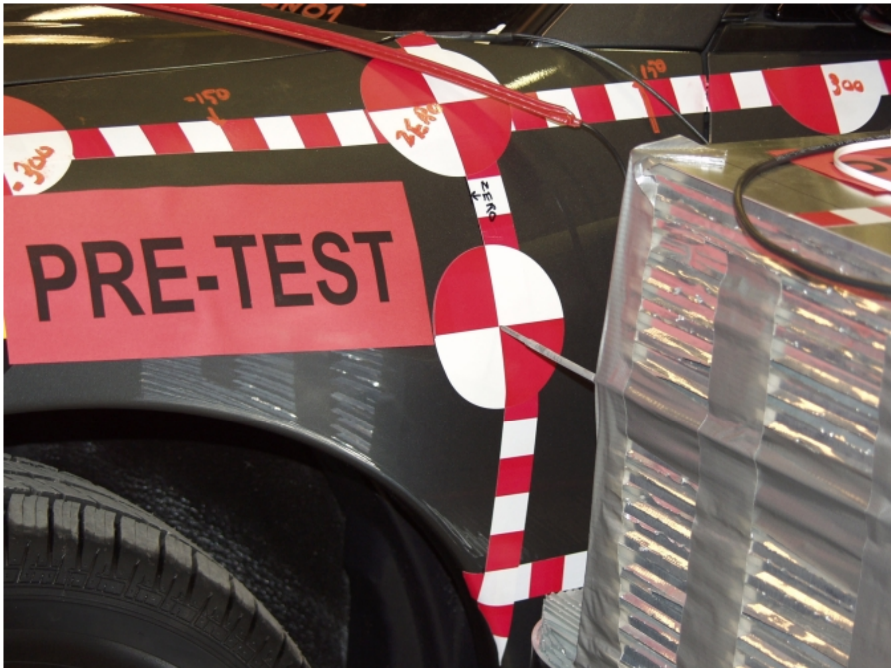
Figure A-29: PRE-TEST CLOSE-UP OF IMPACT POINT TARGET SHOWING WELDING ROD
