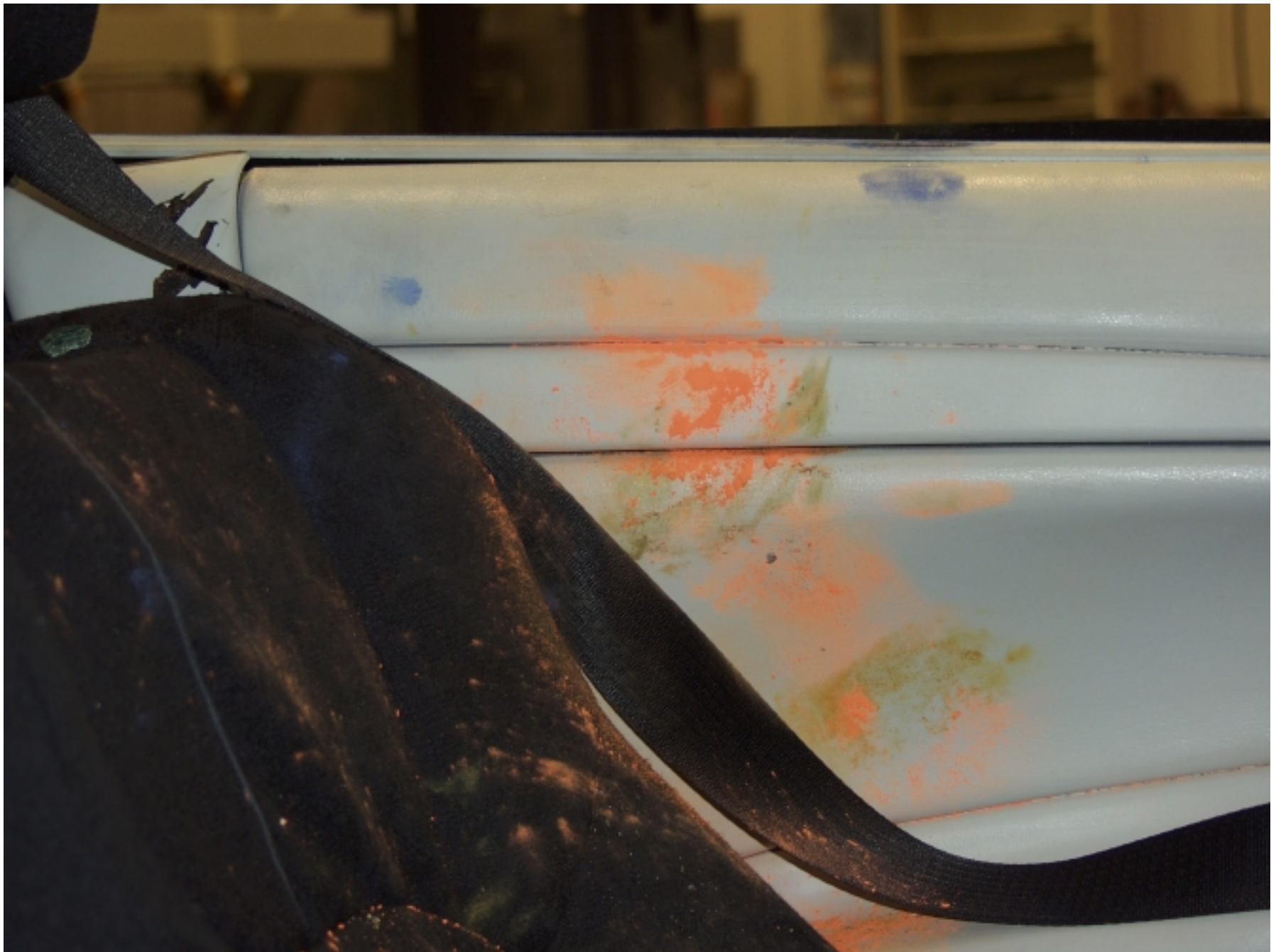
Figure A-22: POST-TEST INTERIOR OF FRONT DOOR SHOWING SID IMPACT LOCATIONS
