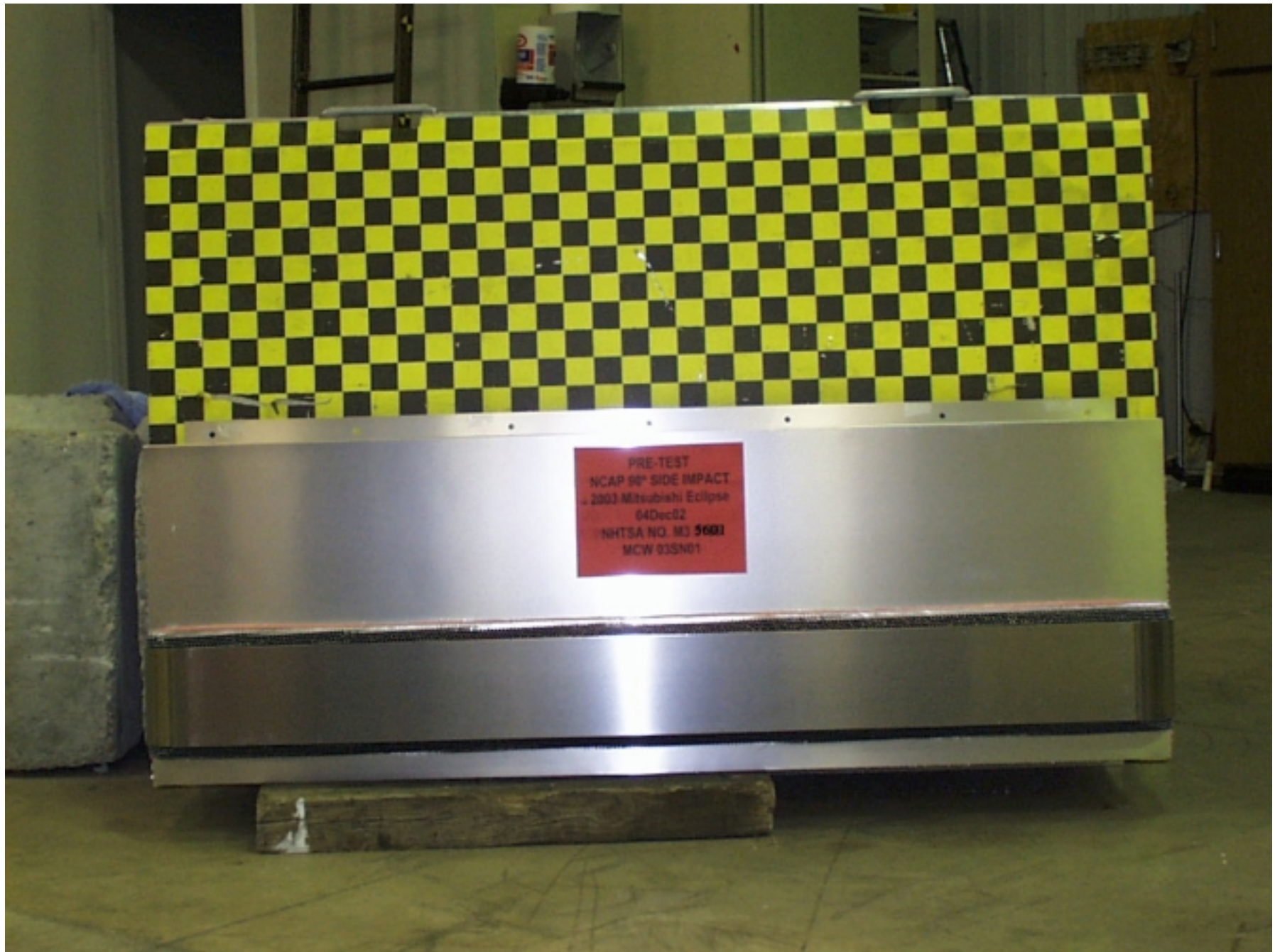
Figure A-39: PRE-TEST ALUMINUM BARRIER FRONT
