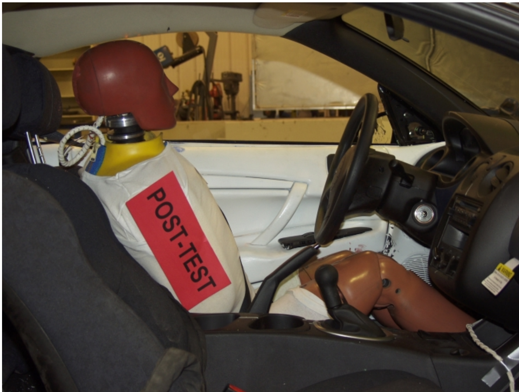
Figure A-18: POST-TEST RIGHT OCCUPANT COMPARTMENT VIEW OF FRONT SID (MDB MOVED)
