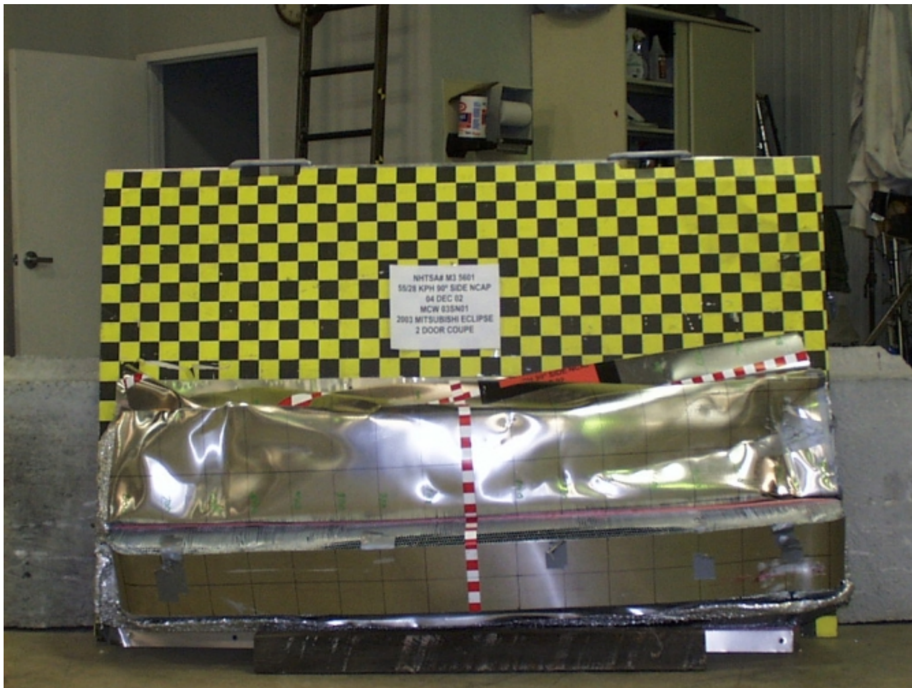
Figure A-40: POST-TEST ALUMINUM BARRIER FRONT
