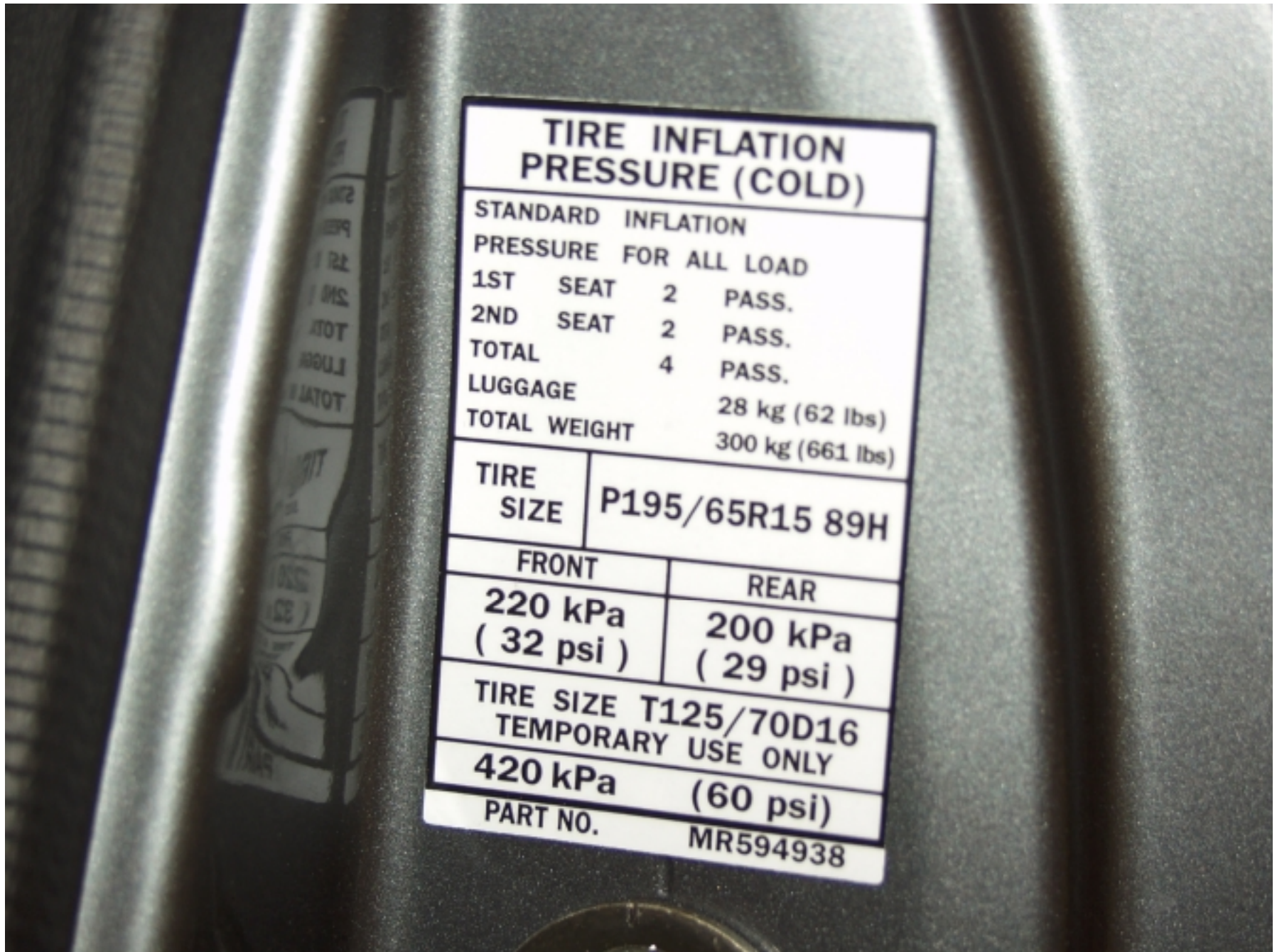
Figure A-32: CLOSE-UP OF VEHICLE'S TIRE PLACARD LABELS
