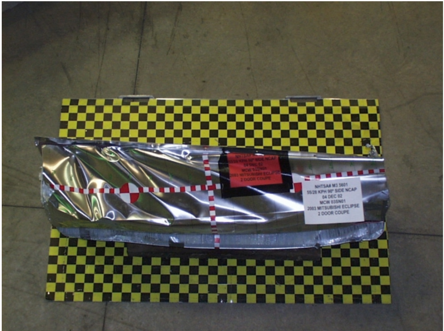
Figure A-46: POST-TEST ALUMINUM BARRIER OVERHEAD
