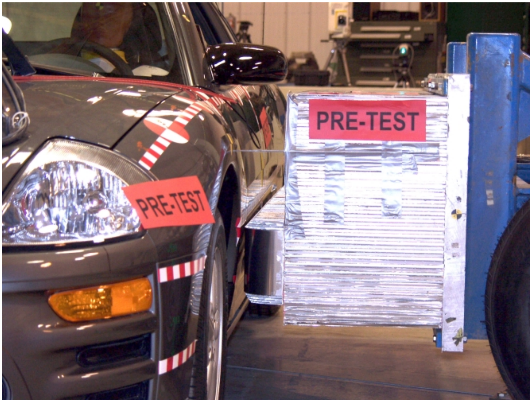
Figure A-23: PRE-TEST LEFT SIDE VIEW OF MDB IN IMPACT POSITION
