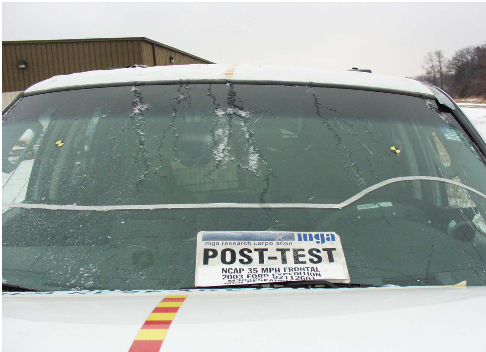
Post-Test Windshield View
