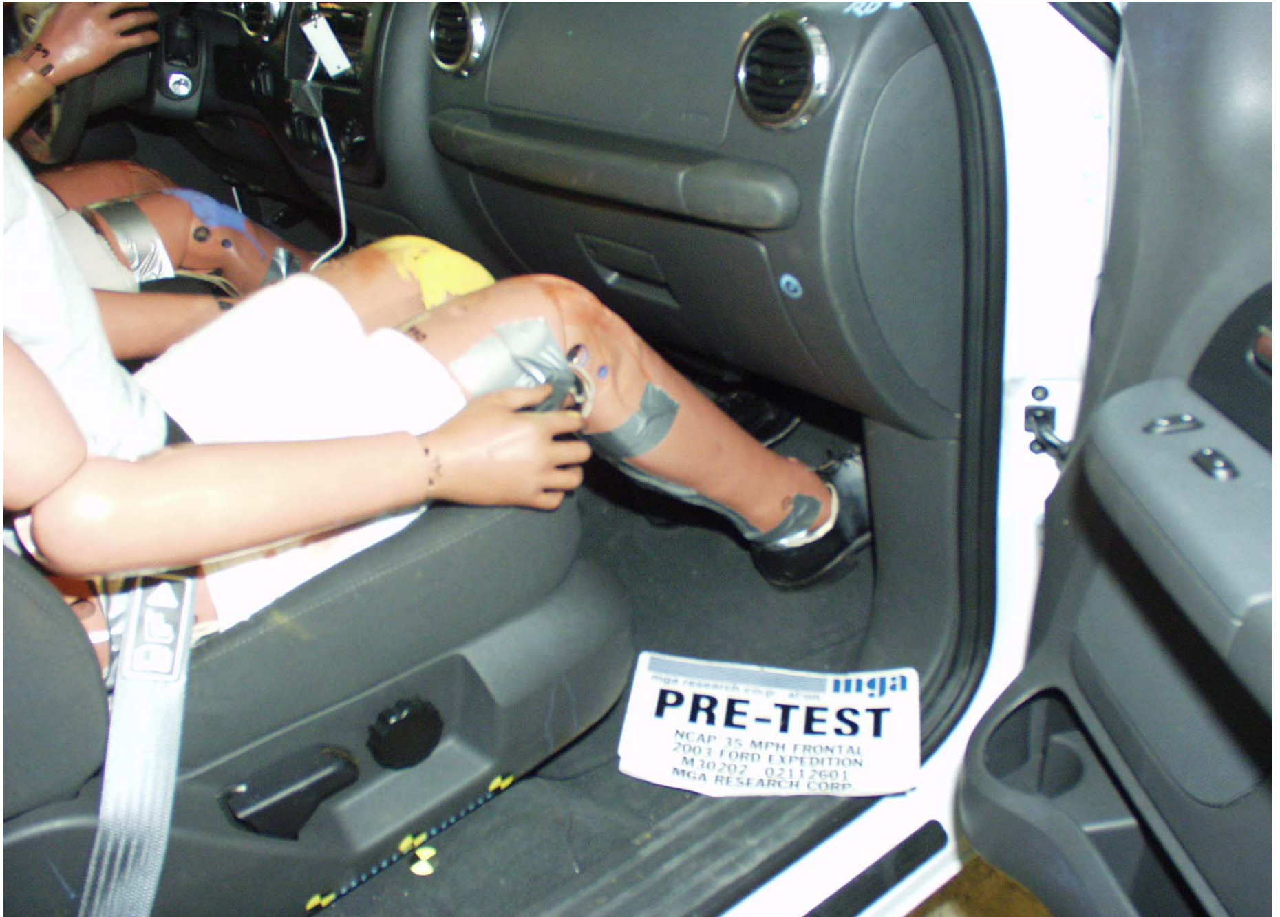
Pre-Test Passenger Side Knee Bolster View
