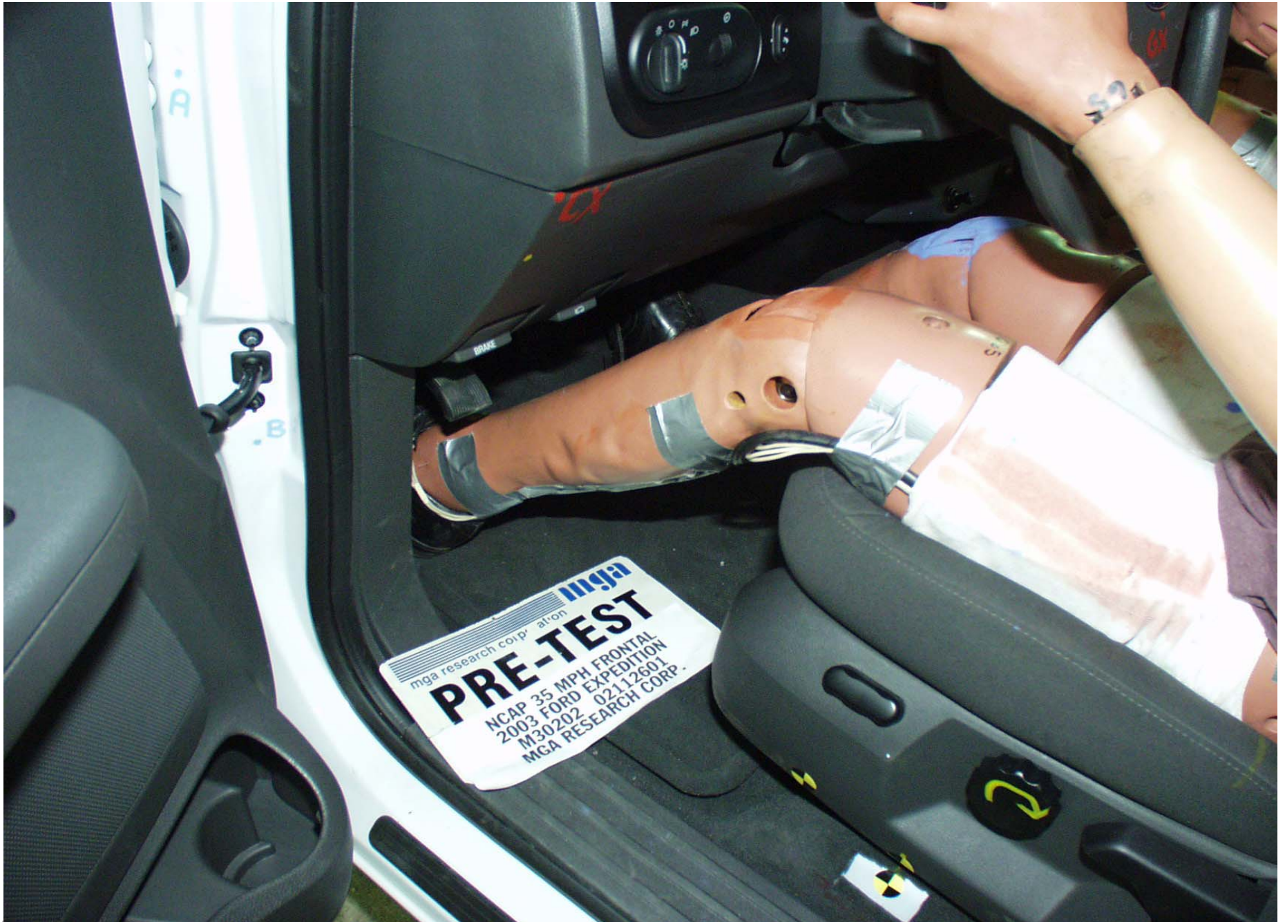
Pre-Test Driver Side Knee Bolster View
