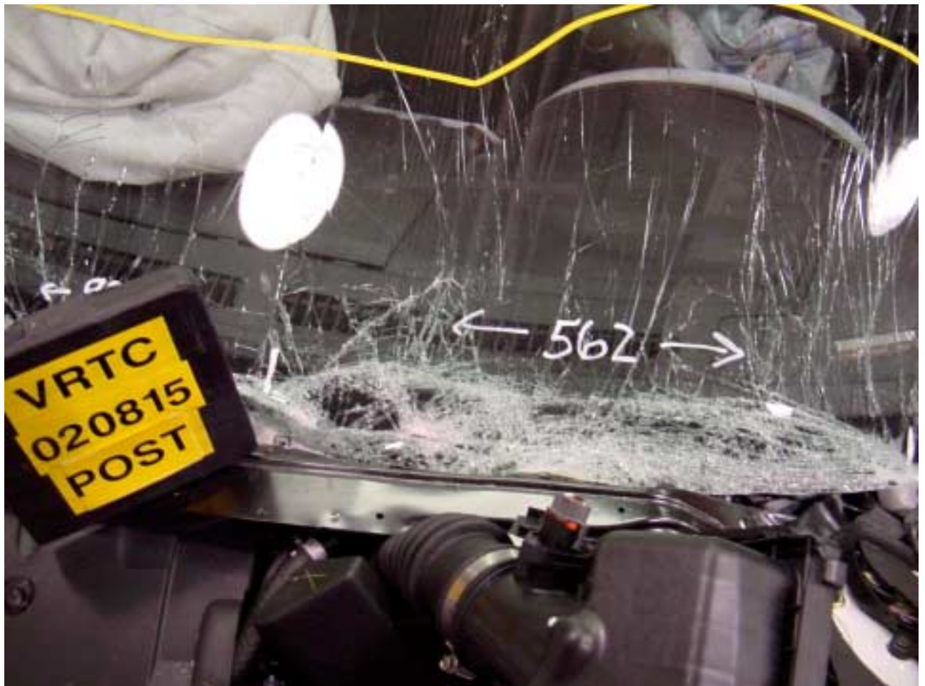
Figure A-36 Post-Test Windshield Close-up - View 2
