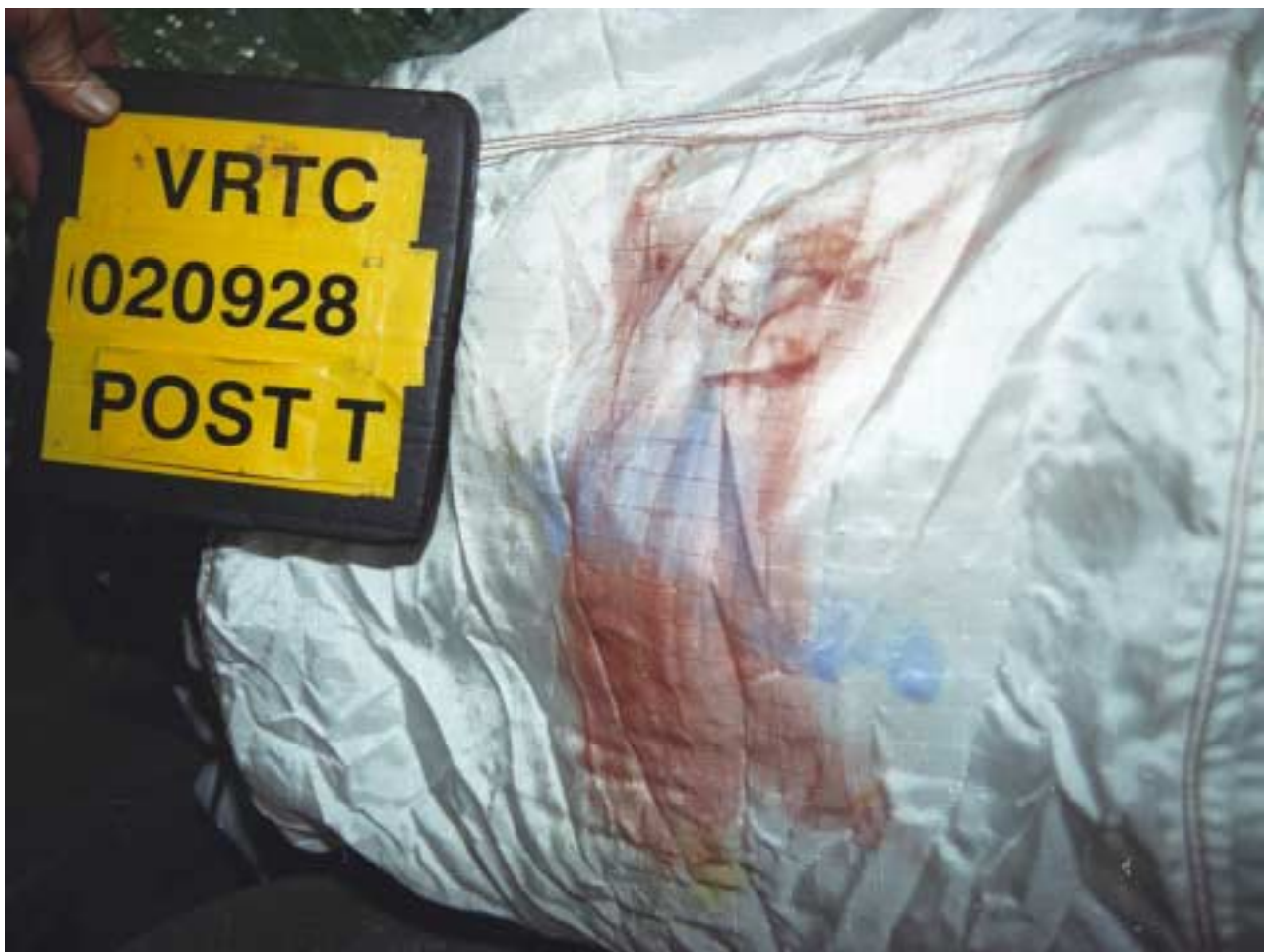
Figure A-108 Post-Test Target Vehicle Passenger Dummy Head Contact - View 2
