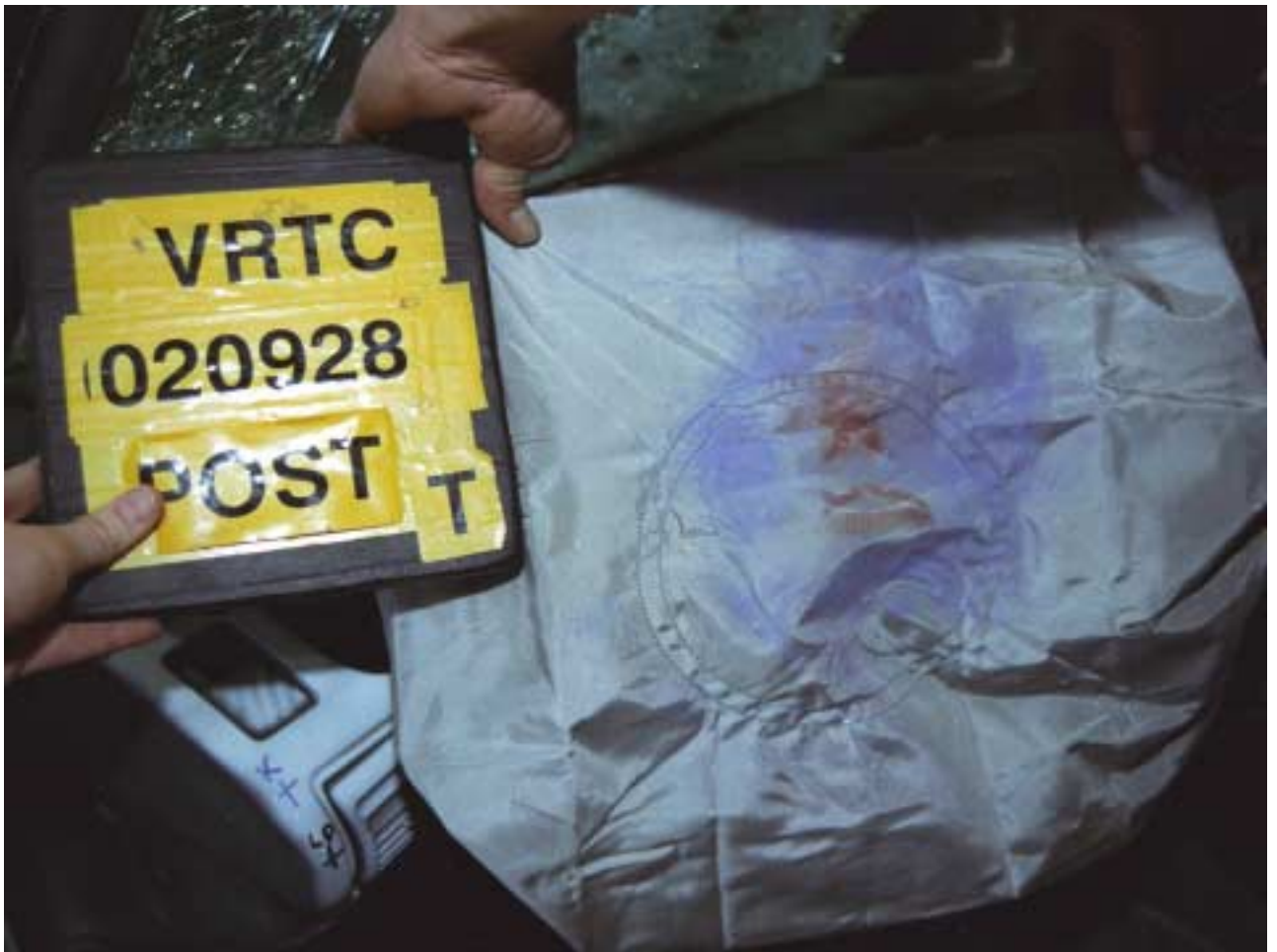
Figure A-100 Post-Test Target Vehicle Driver Dummy Head Contact - View 2
