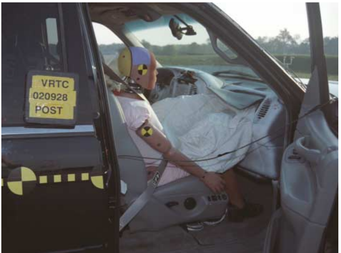
Figure A-95 Post-Test Bullet Vehicle Passenger Dummy - View 3
