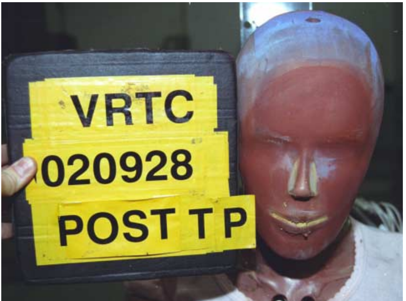
Figure A-107 Post-Test Target Vehicle Passenger Dummy Head Contact - View 1
