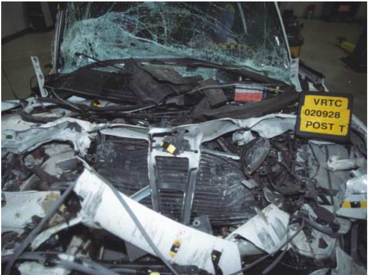
Figure A-31 Post-Test Target Vehicle Engine Compartment View
