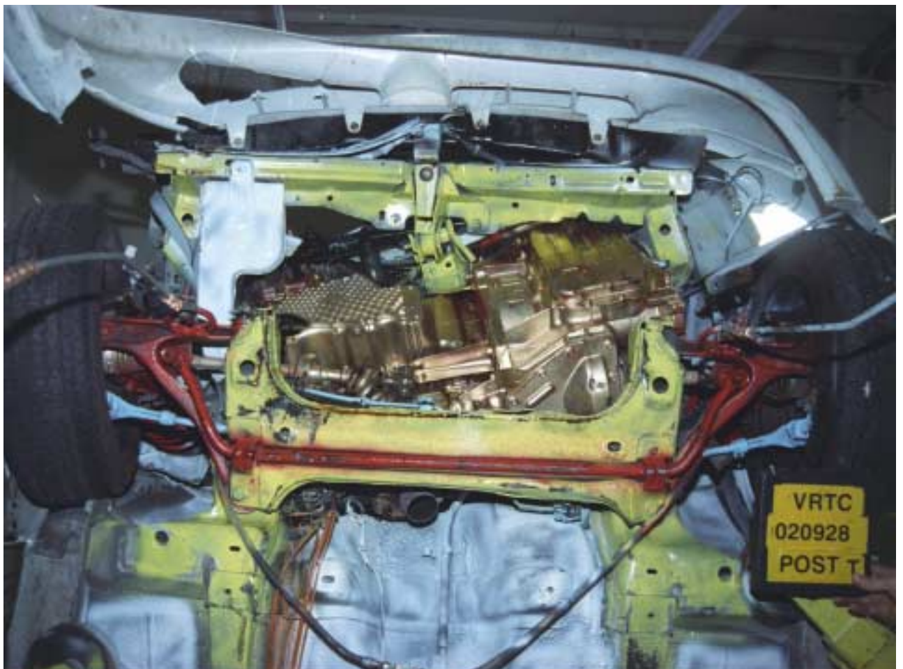
Figure A-33 Post-Test Target Vehicle Front Underbody View
