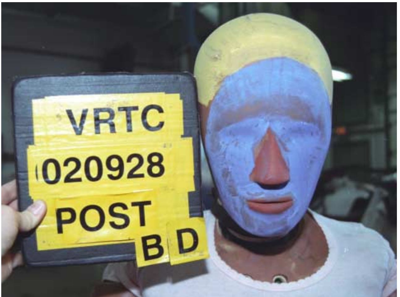
Figure A-113 Post-Test Bullet Vehicle Driver Dummy Head Contact - View 1
