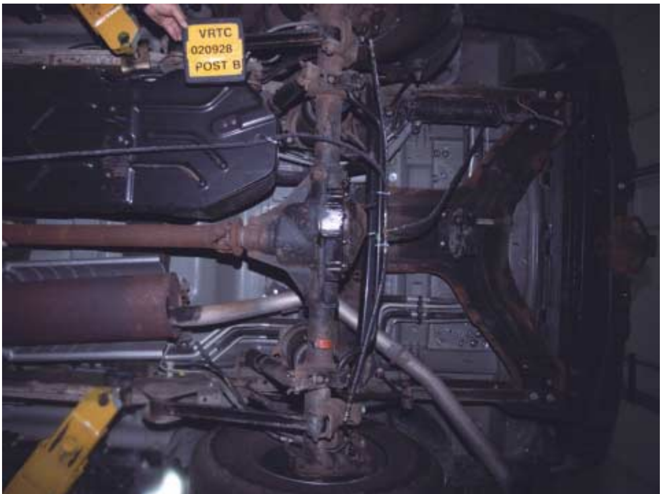
Figure A-64 Post-Test Bullet Vehicle Rear Underbody View
