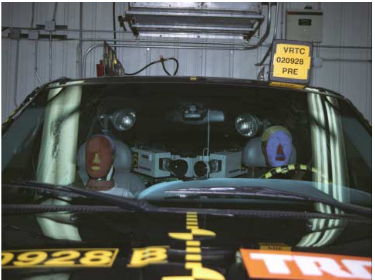
Figure A-80 Pre-Test Bullet Vehicle Driver and Passenger Dummies through Windshield View
