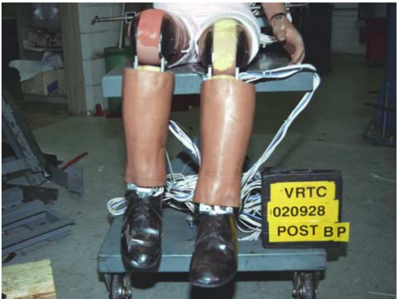
Figure A-124 Post-Test Bullet Vehicle Passenger Dummy Knee Contact - View 1
