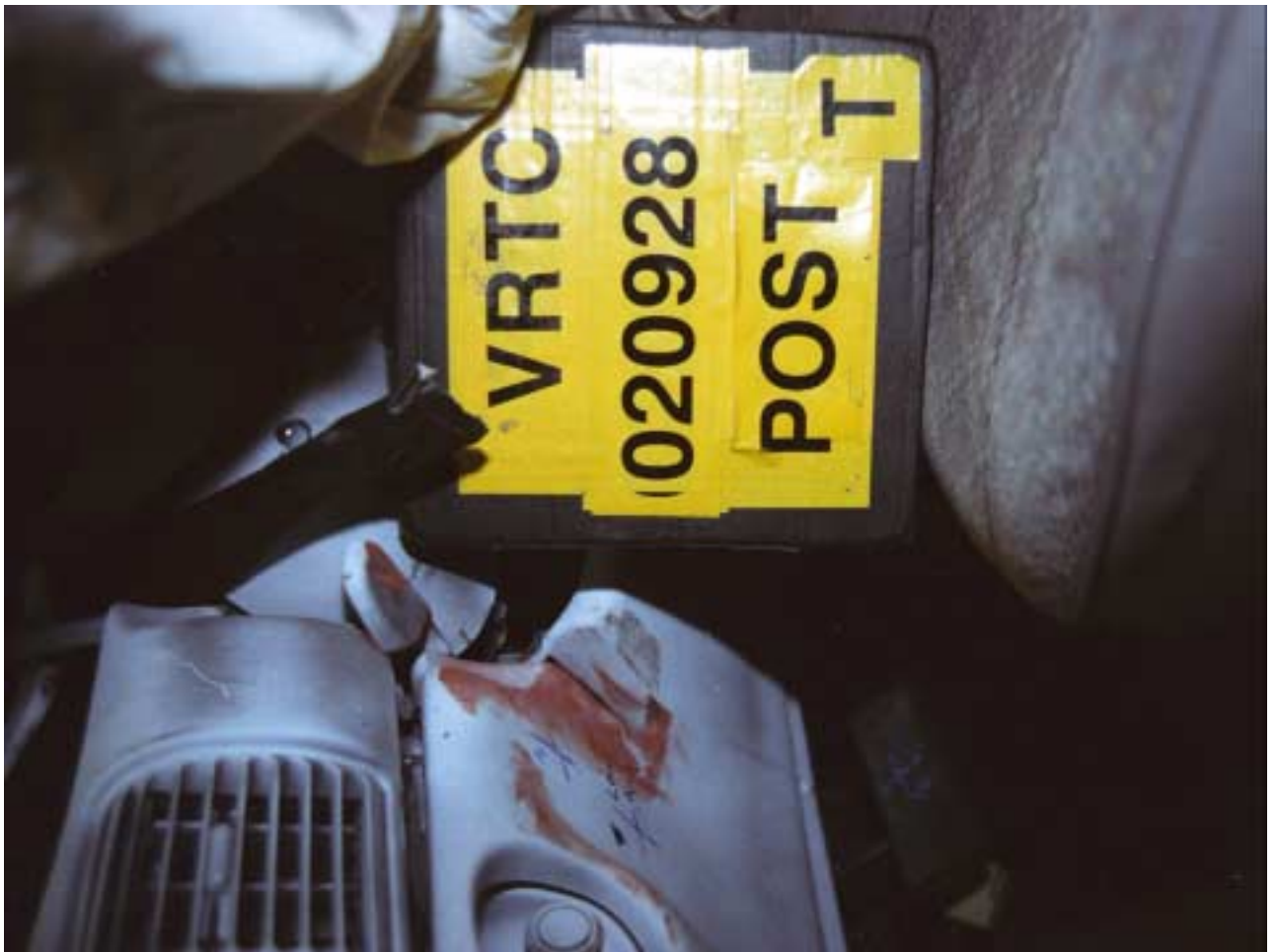
Figure A-104 Post-Test Target Vehicle Driver Dummy Knee Contact - View 2
