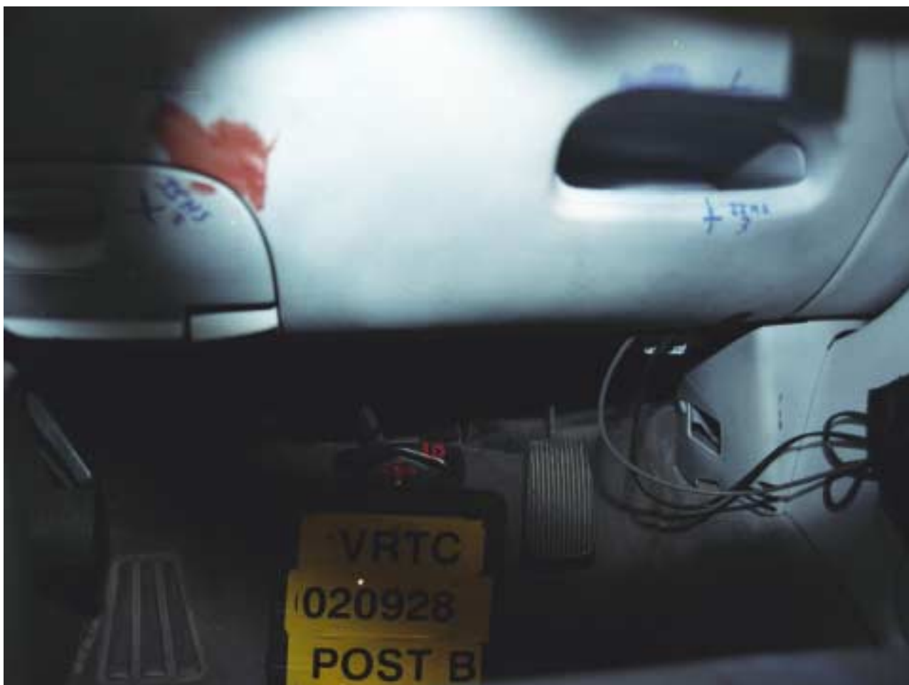
Figure A-117 Post-Test Bullet Vehicle Driver Dummy Knee Contact - View 2
