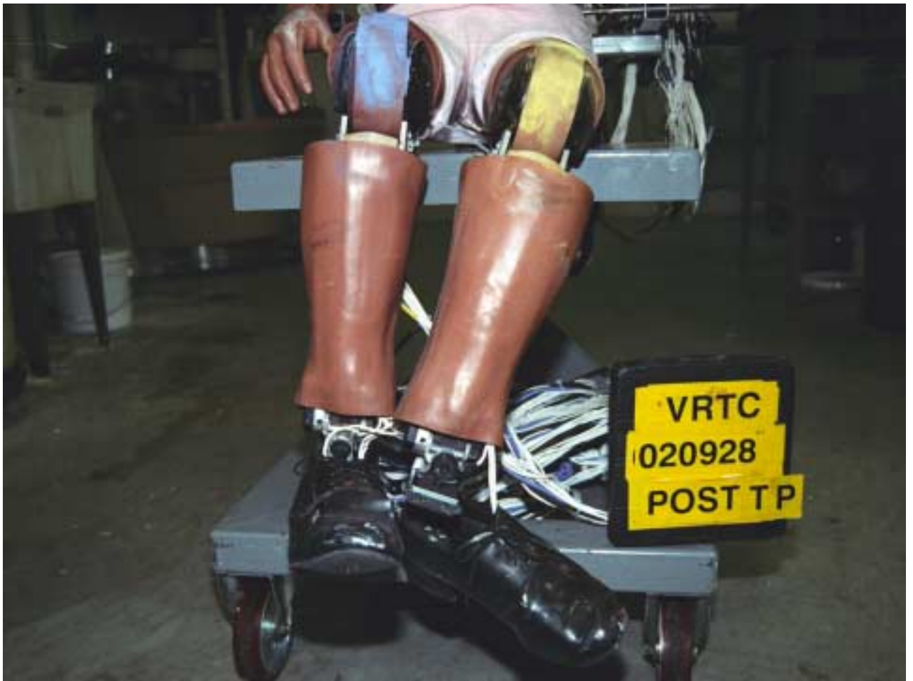
Figure A-110 Post-Test Target Vehicle Passenger Dummy Knee Contact - View 1
