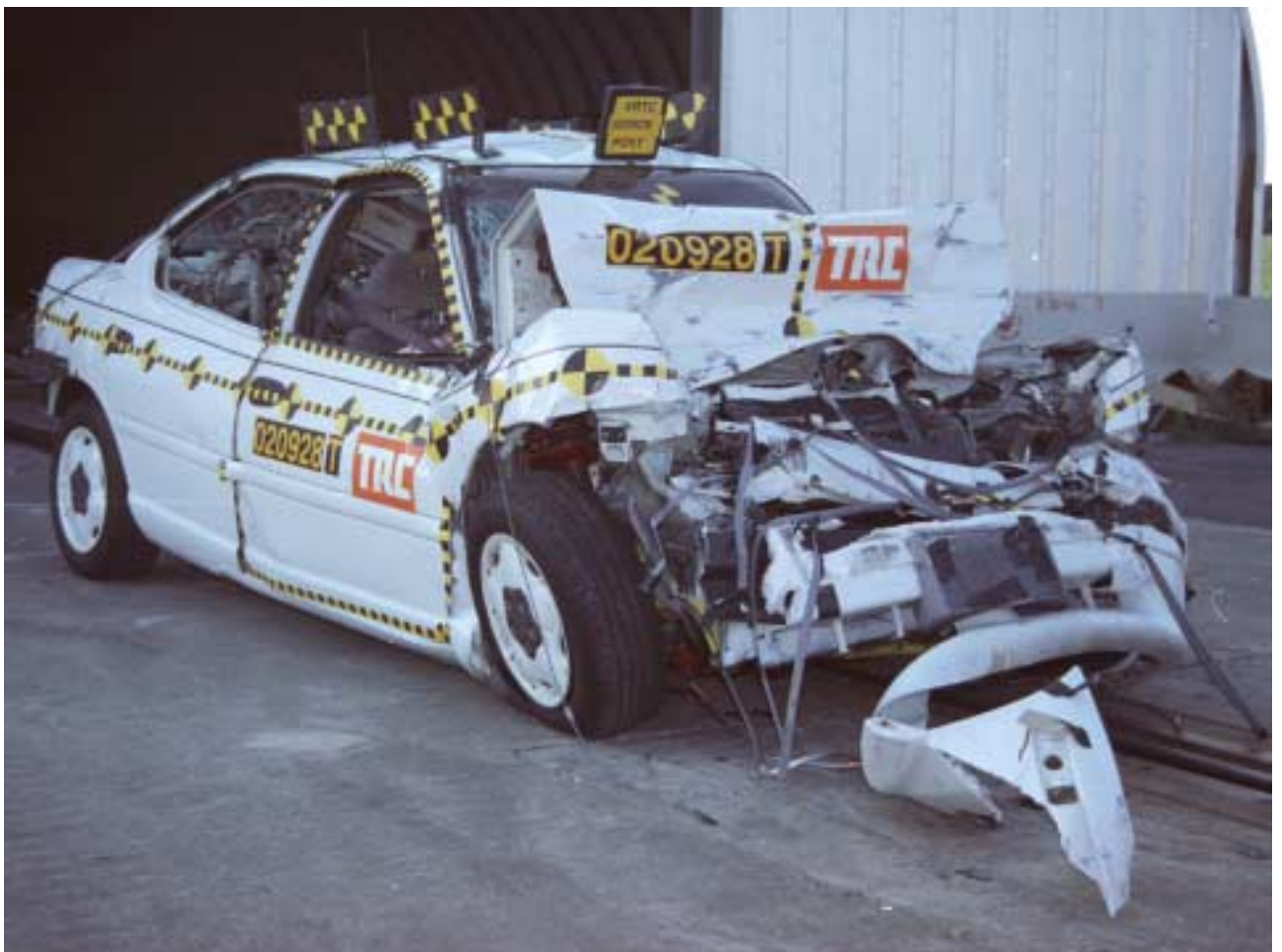
Figure A-29 Post-Test Target Vehicle Right Front View
