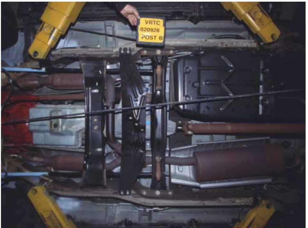
Figure A-62 Post-Test Bullet Vehicle Mid Underbody View
