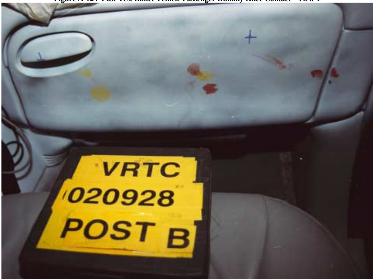
Figure A-125 Post-Test Bullet Vehicle Passenger Dummy Knee Contact - View 2
