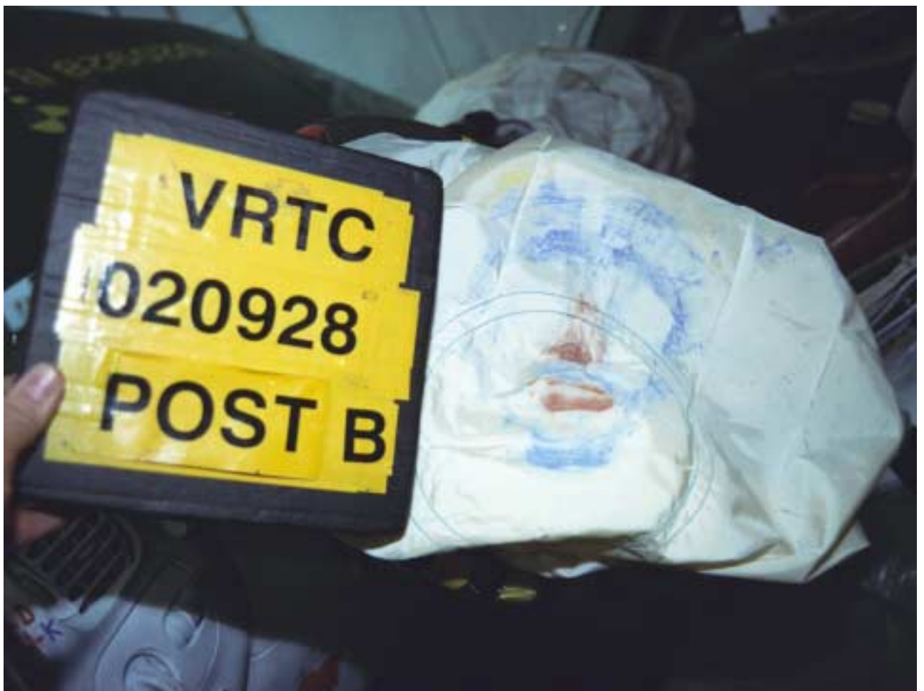
Figure A-114 Post-Test Bullet Vehicle Driver Dummy Head Contact - View 2
