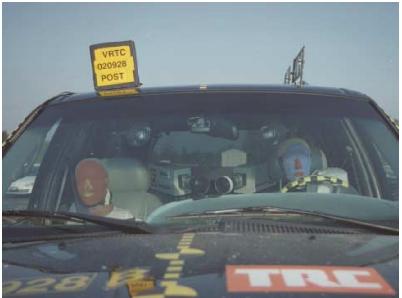
Figure A-81 Post-Test Bullet Vehicle Driver and Passenger Dummies through Windshield View
