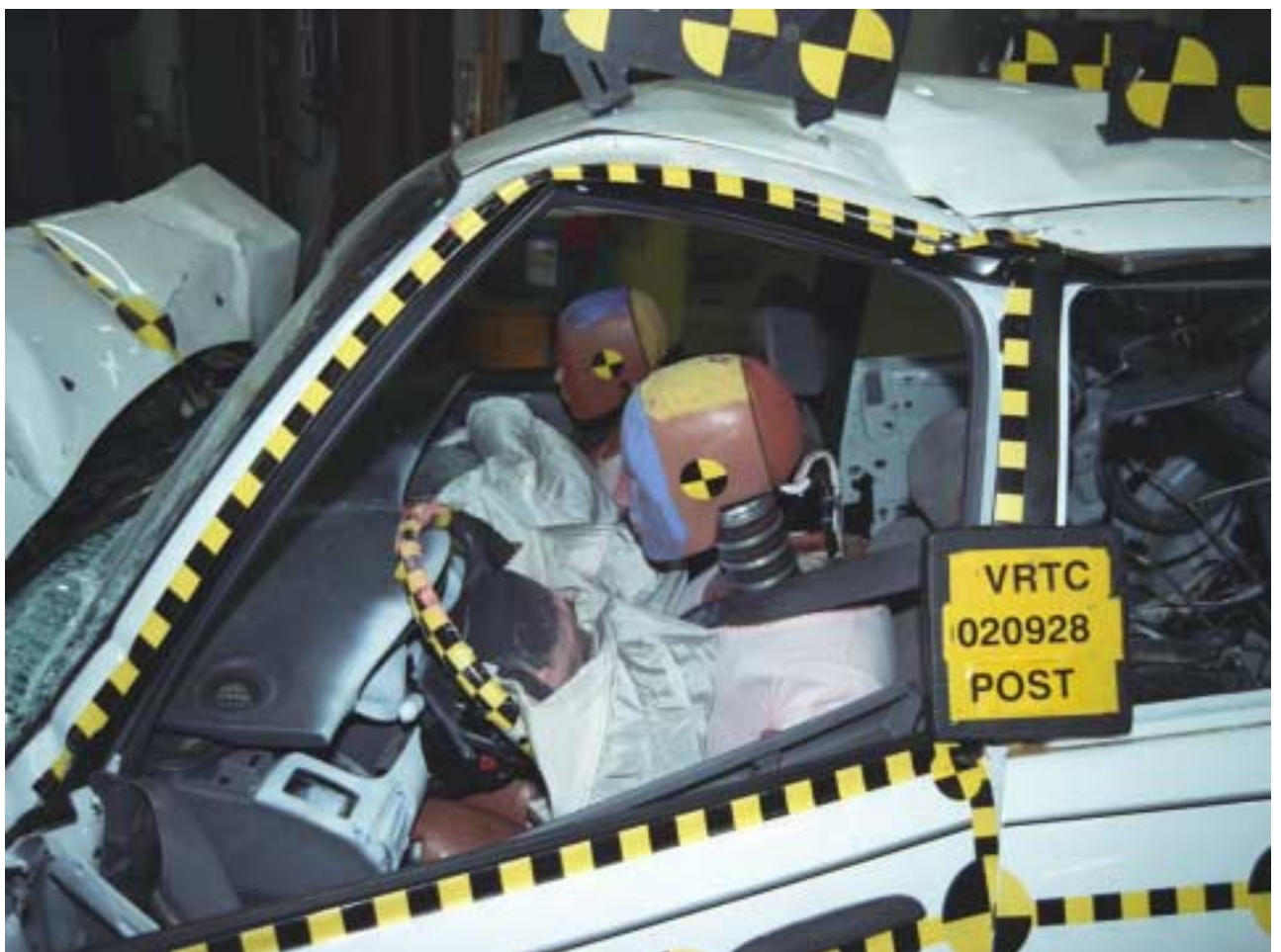
Figure A-68 Post-Test Target Vehicle Driver Dummy - View 2
