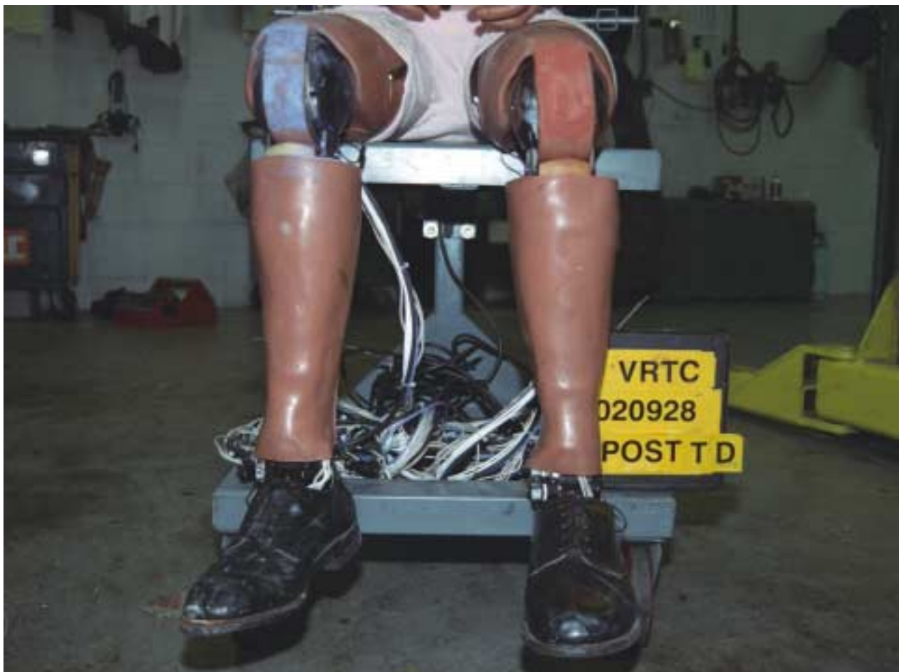
Figure A-103 Post-Test Target Vehicle Driver Dummy Knee Contact - View 1
