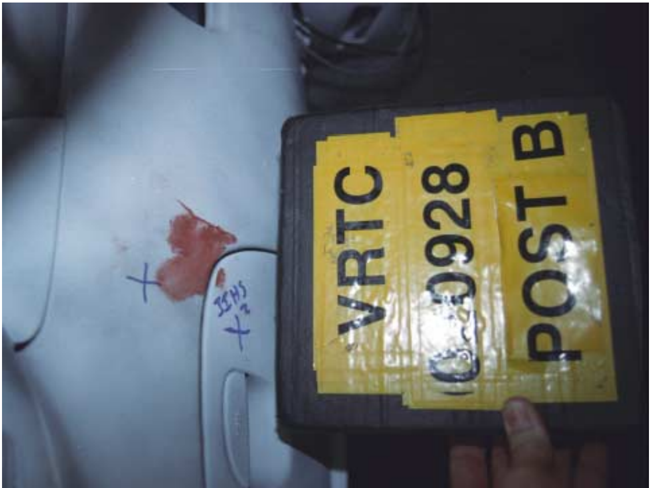
Figure A-118 Post-Test Bullet Vehicle Driver Dummy Knee Contact - View 3
