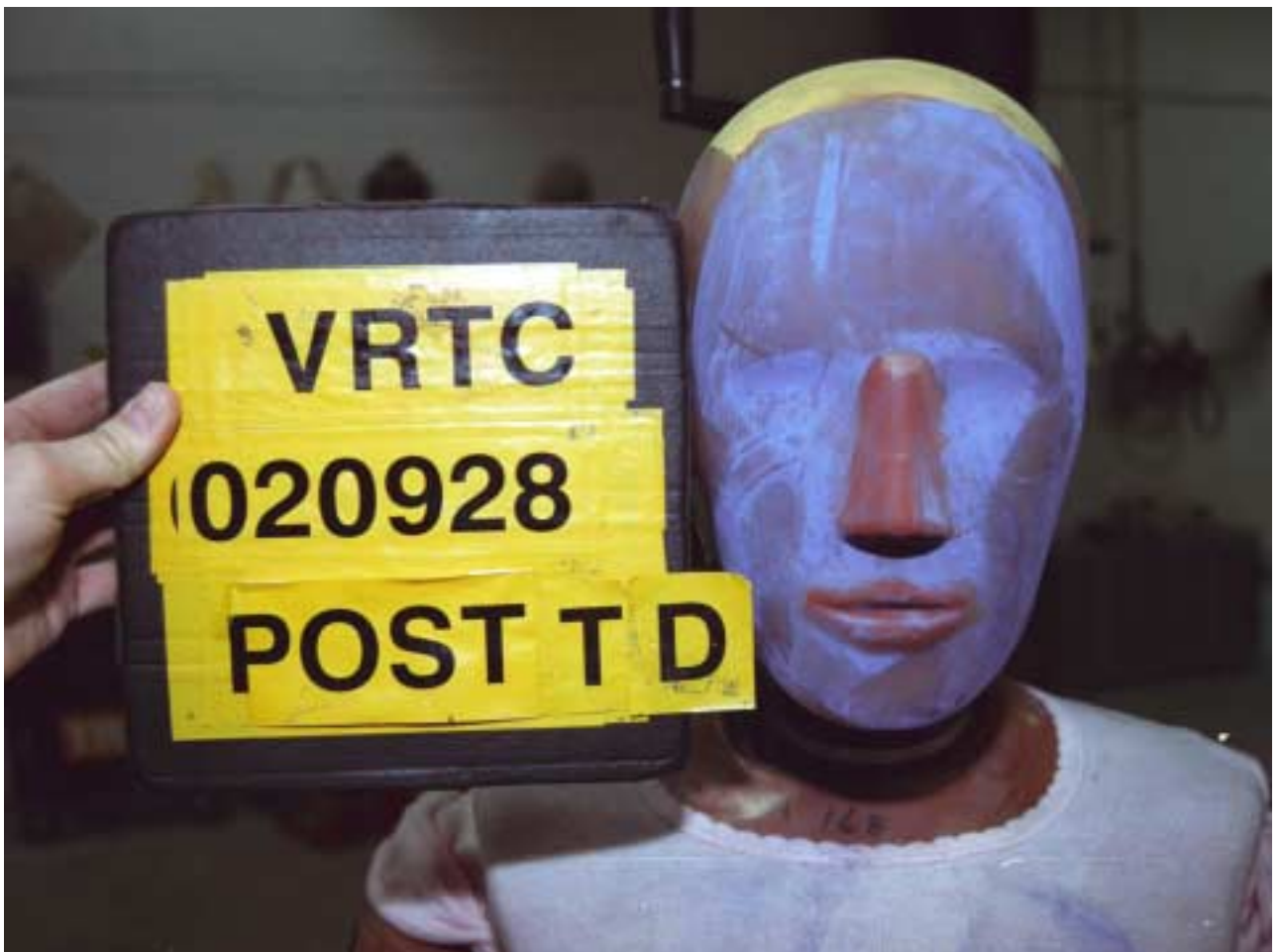
Figure A-99 Post-Test Target Vehicle Driver Dummy Head Contact - View 1
