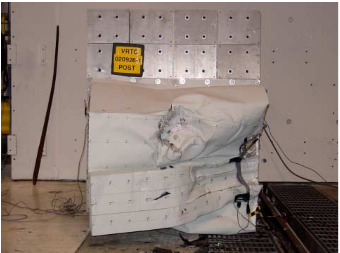
Figure A-35 Post-Test Front Barrier Face View
