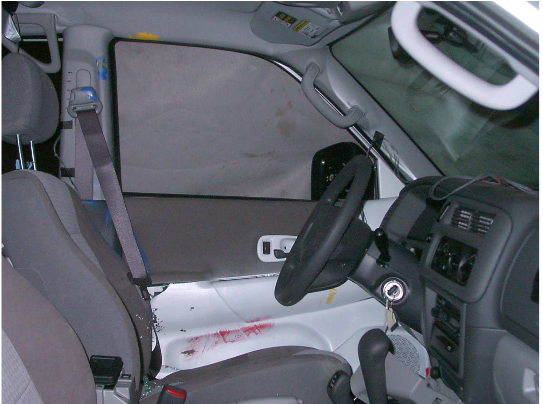
Figure A-37: Driver Dummy Contact Points Inside View, Post-Test (Vehicle Moved)
