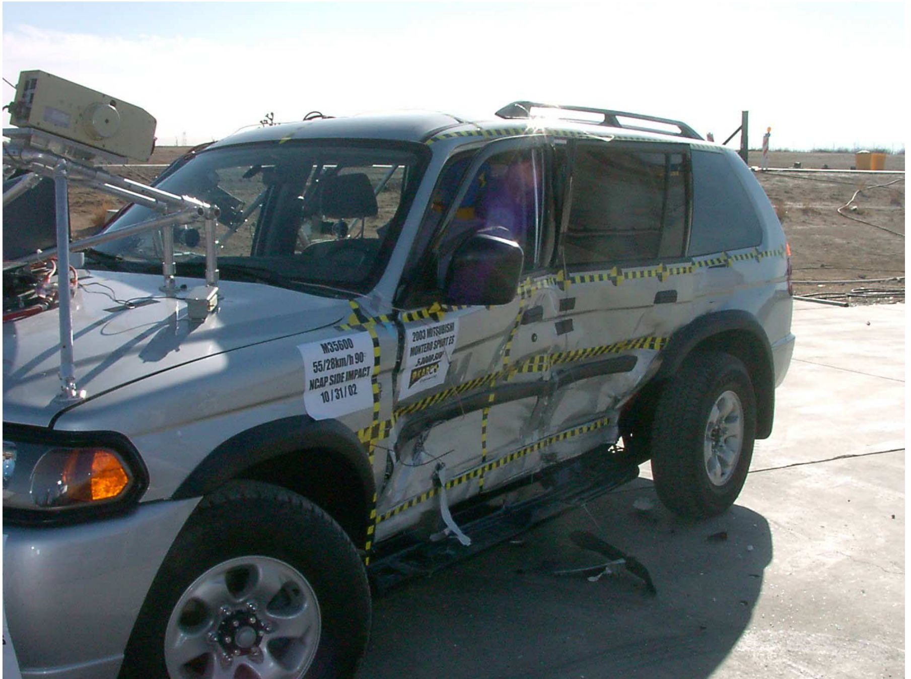
Figure A-22: Front \frac{3}{4} View of Left Side Doors, Post-Test
