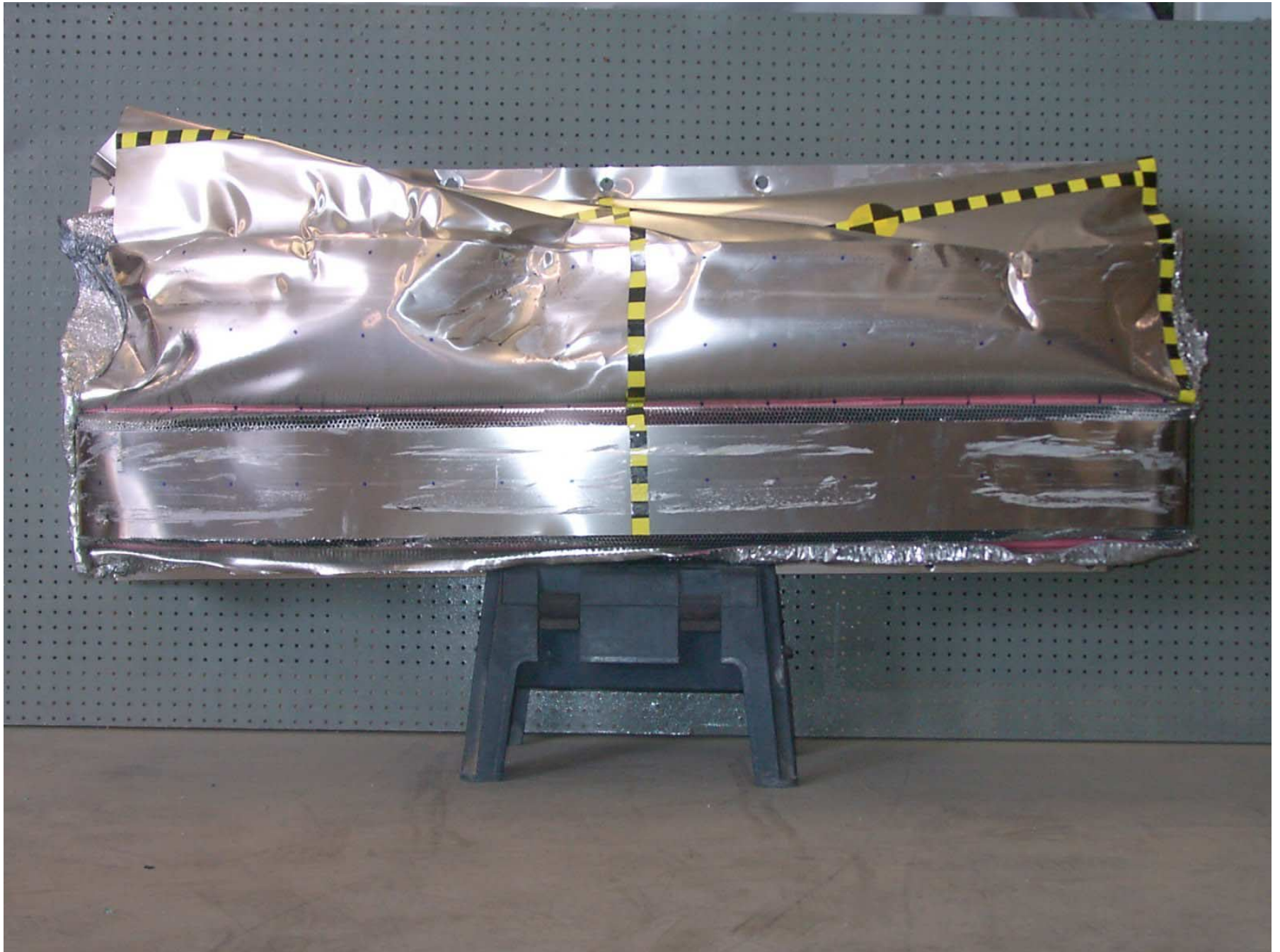
Figure A-48: Front View of Deformable Barrier, Post-Test
