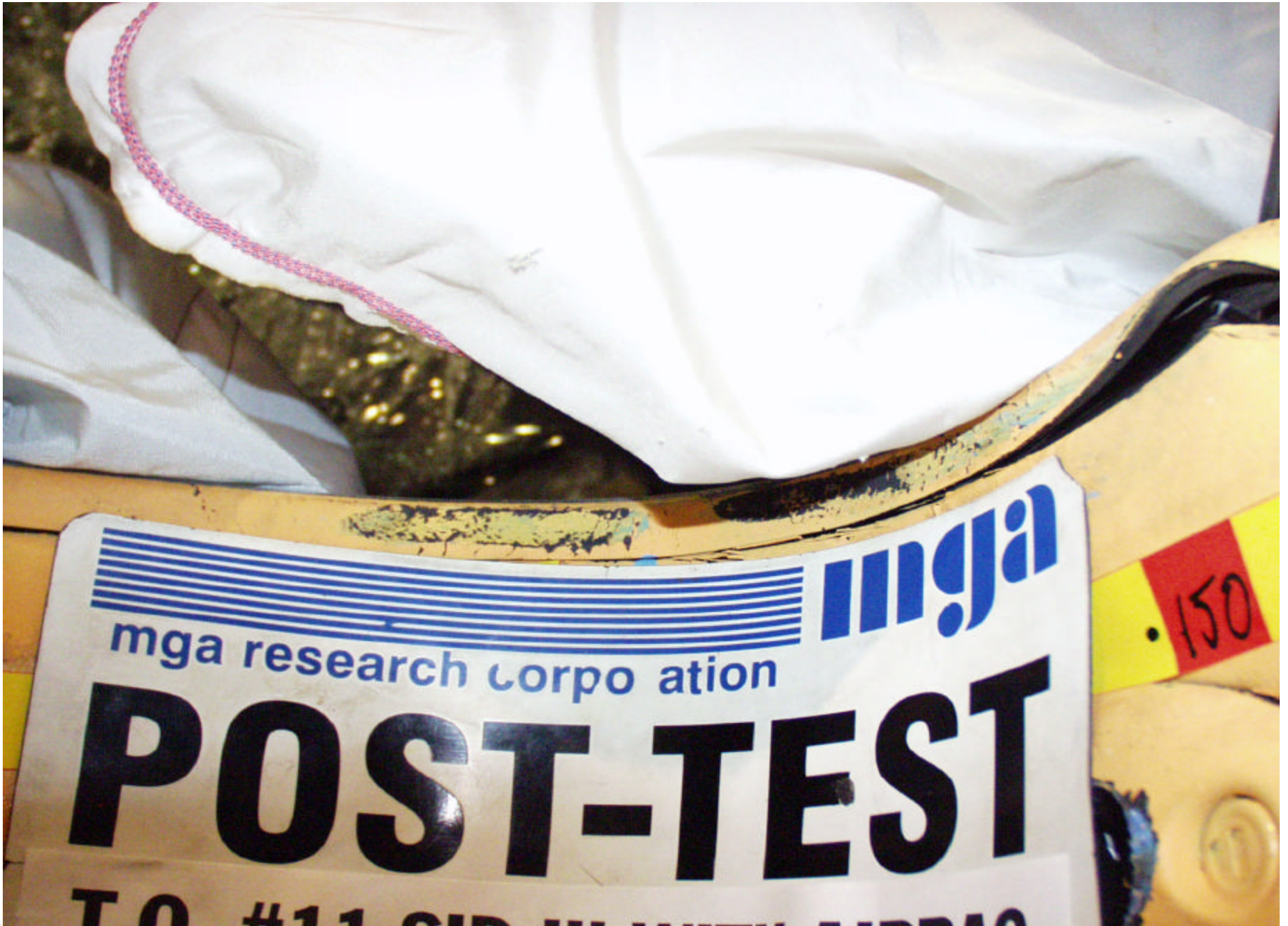
Airbag Damage (Outside View)
