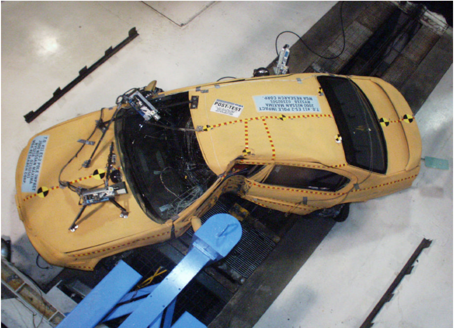
Post-Test Pole and Vehicle Overhead View
