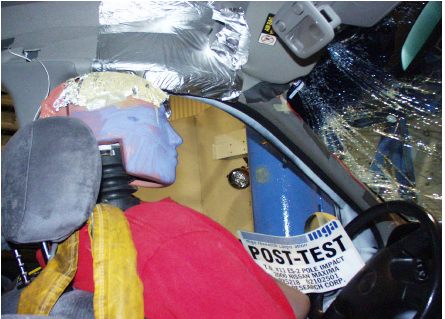
Post-Test Driver Dummy Contact to Pole
