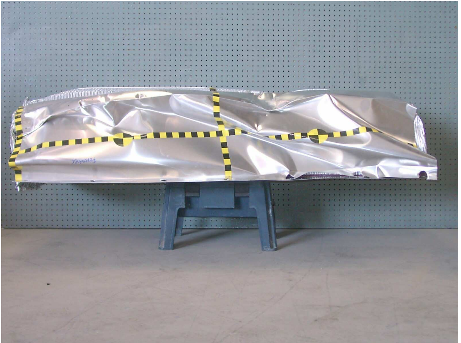
Figure A-50: Top View of Deformable Barrier, Post-Test
