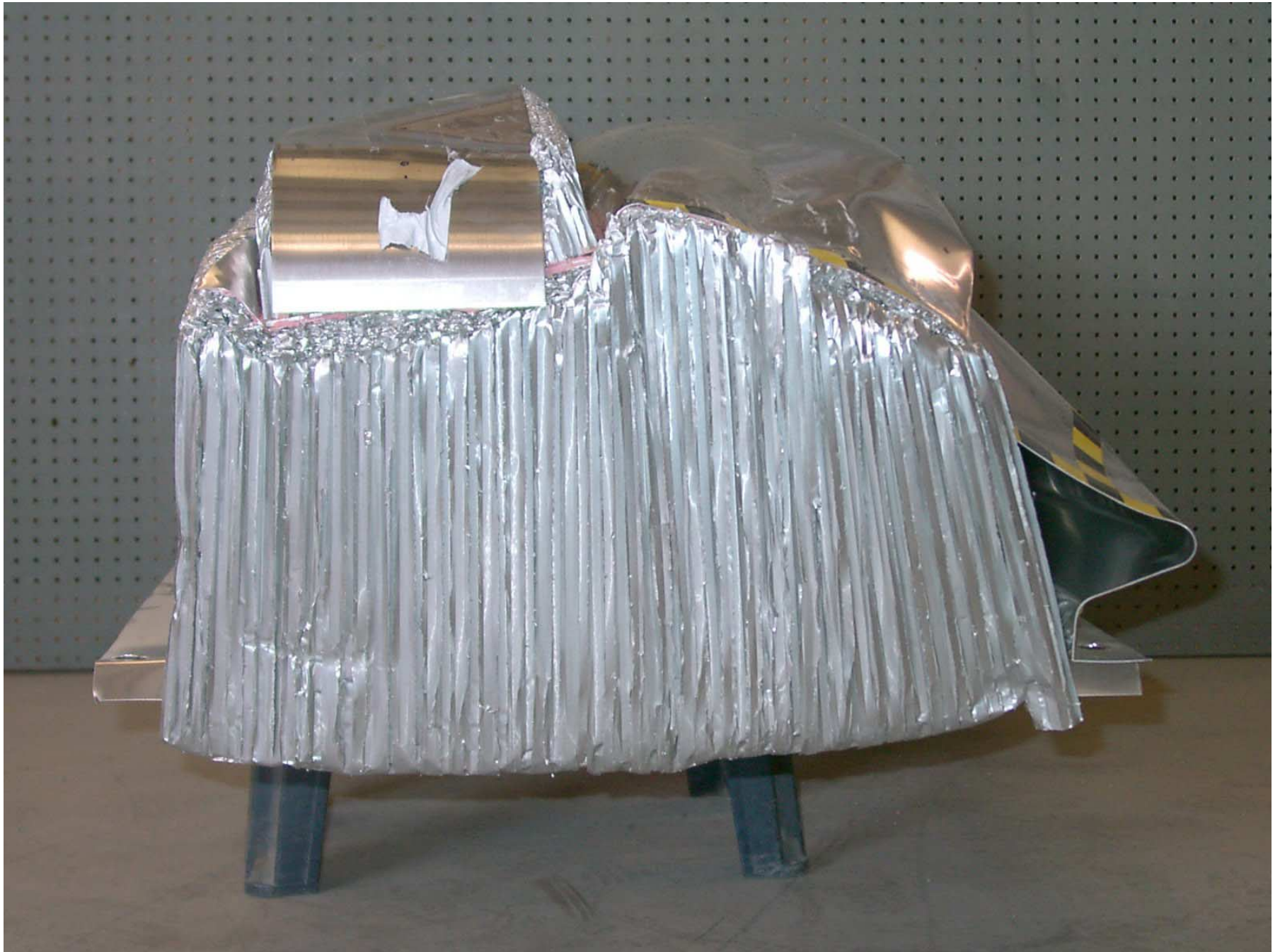
Figure A-54: Left Side View of Deformable Barrier, Post-Test
