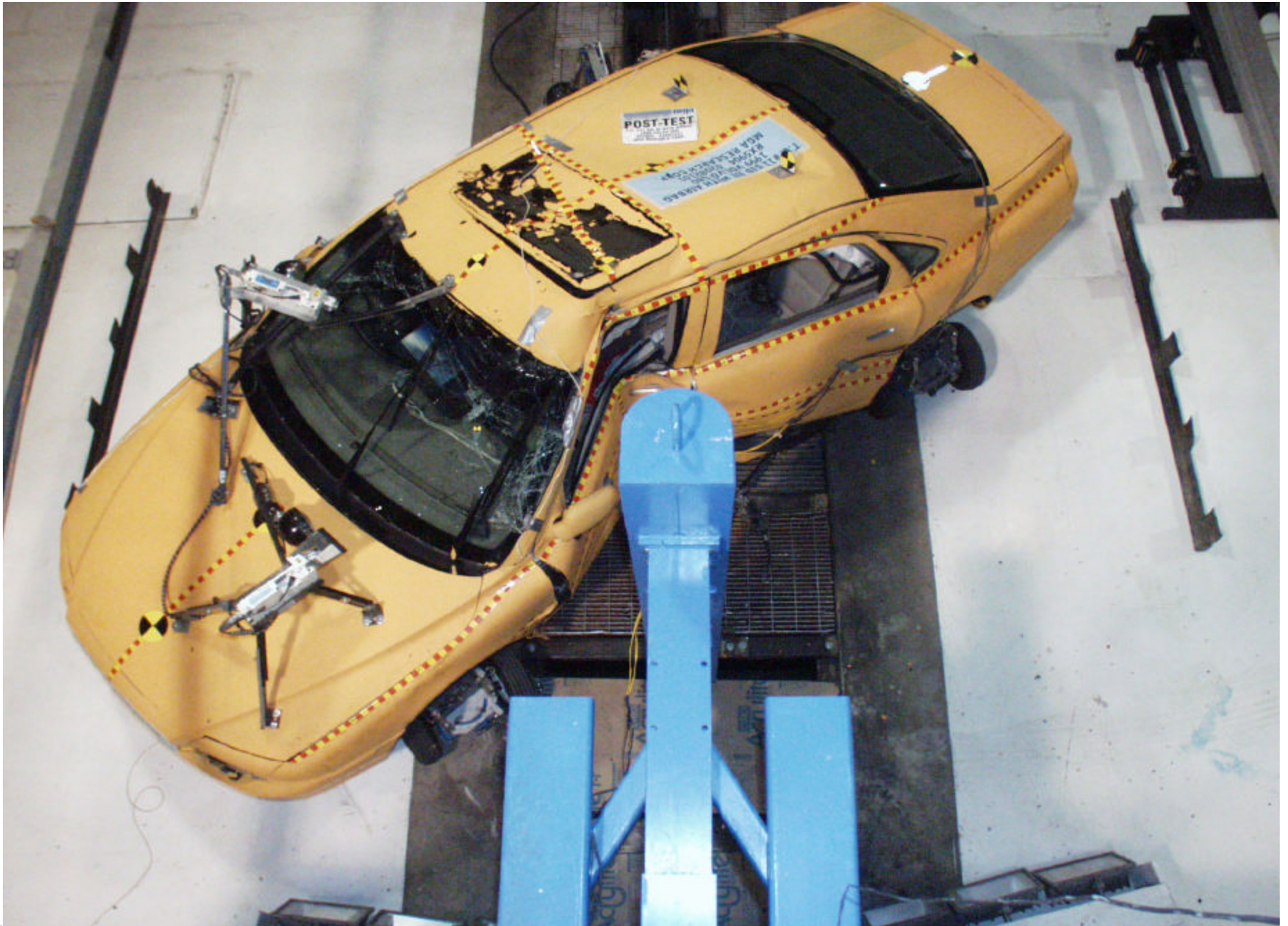
Post-Test Pole and Vehicle Overhead View
