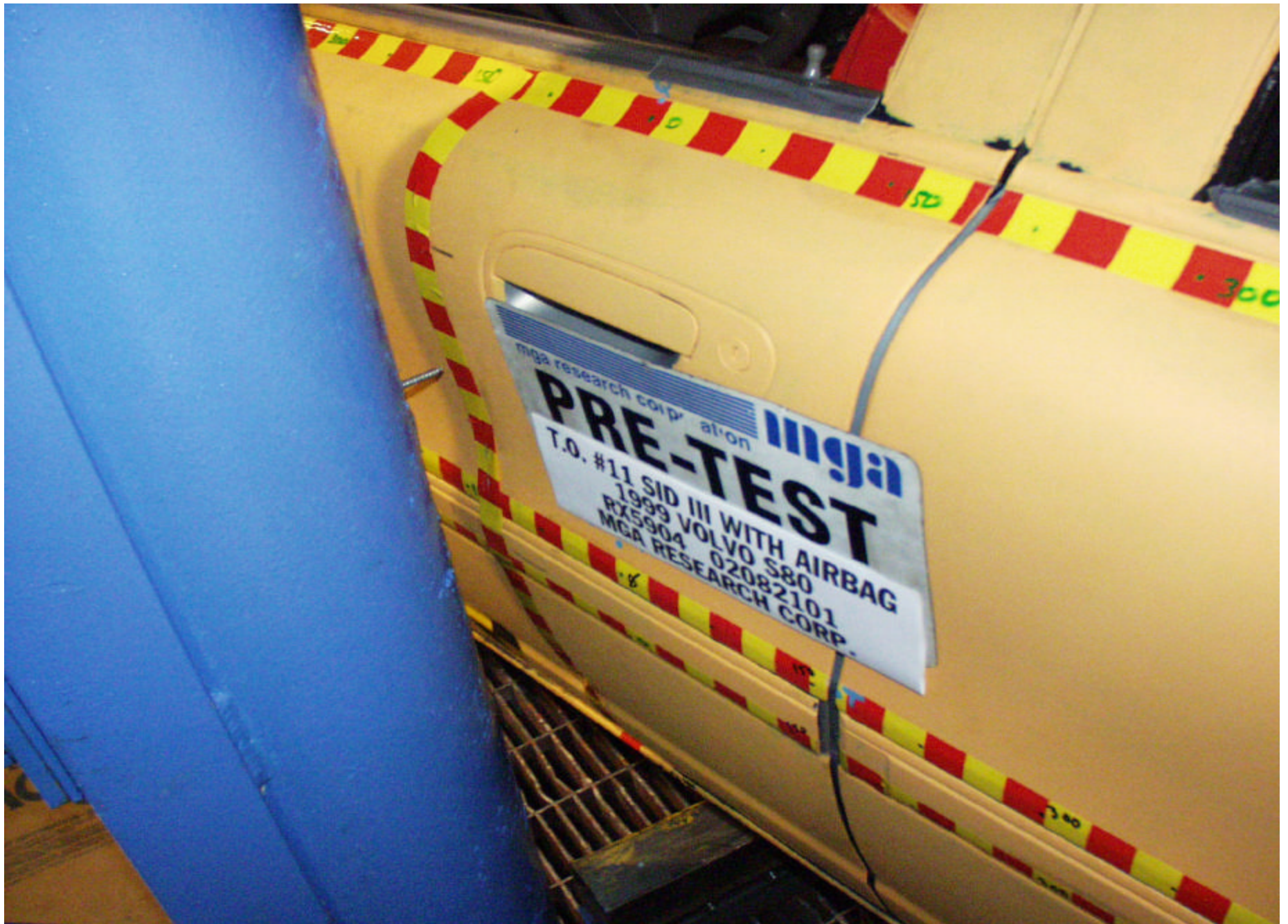
Pre-Test Impact Point on Vehicle
