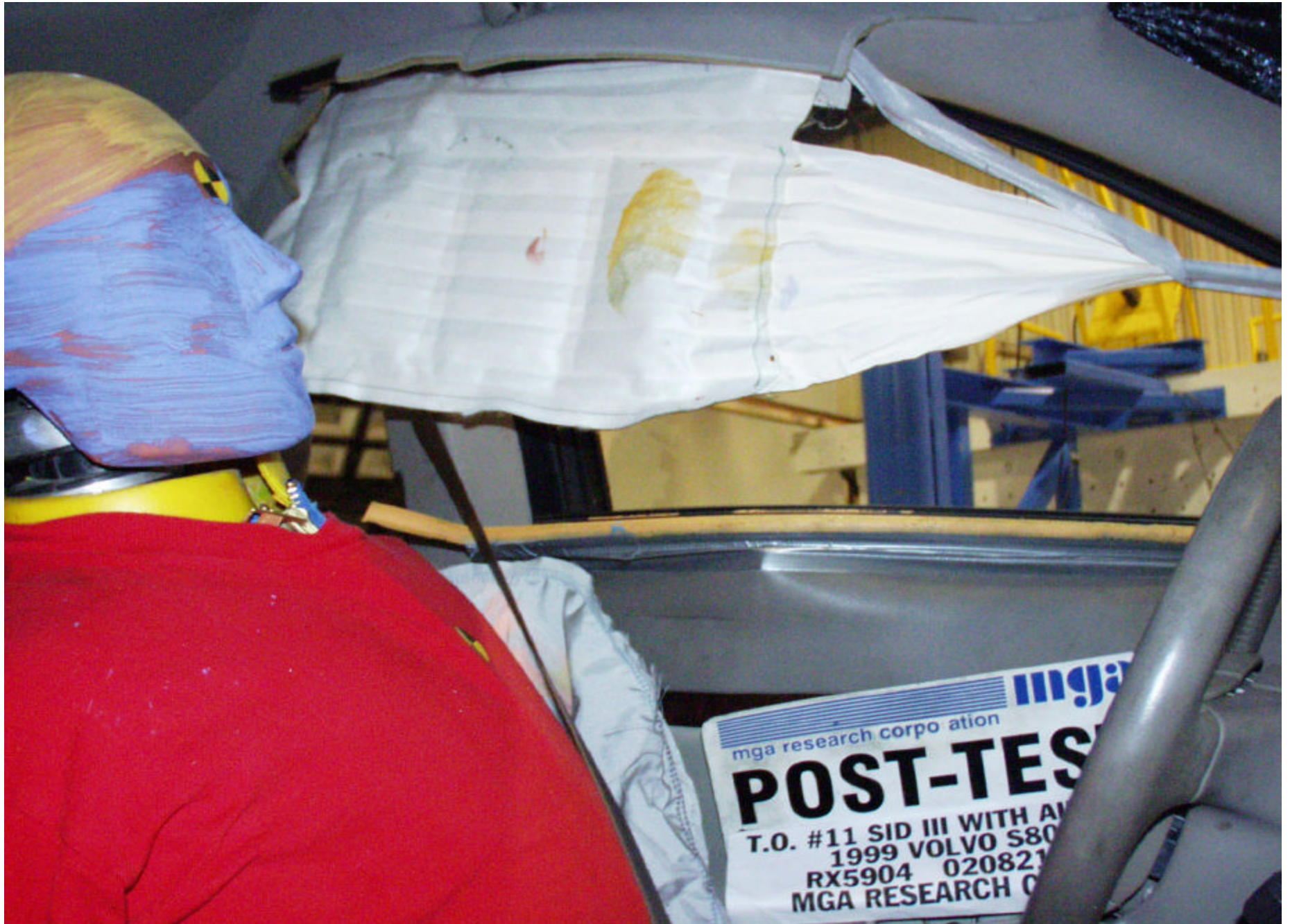
Post-Test Driver Dummy Head Contact
