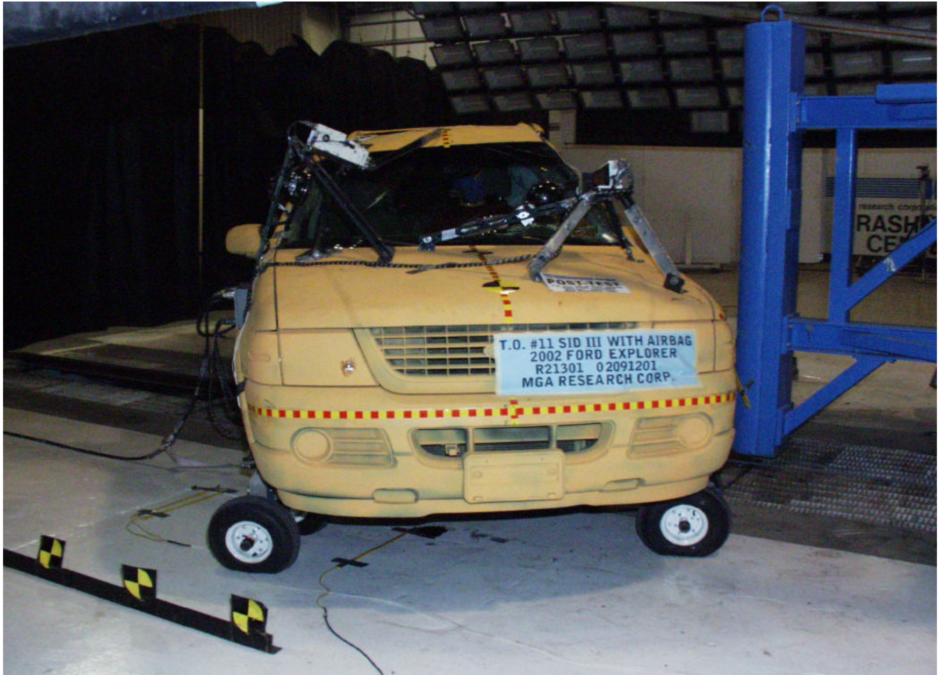
Post-Test Front View of Test Vehicle and Pole
