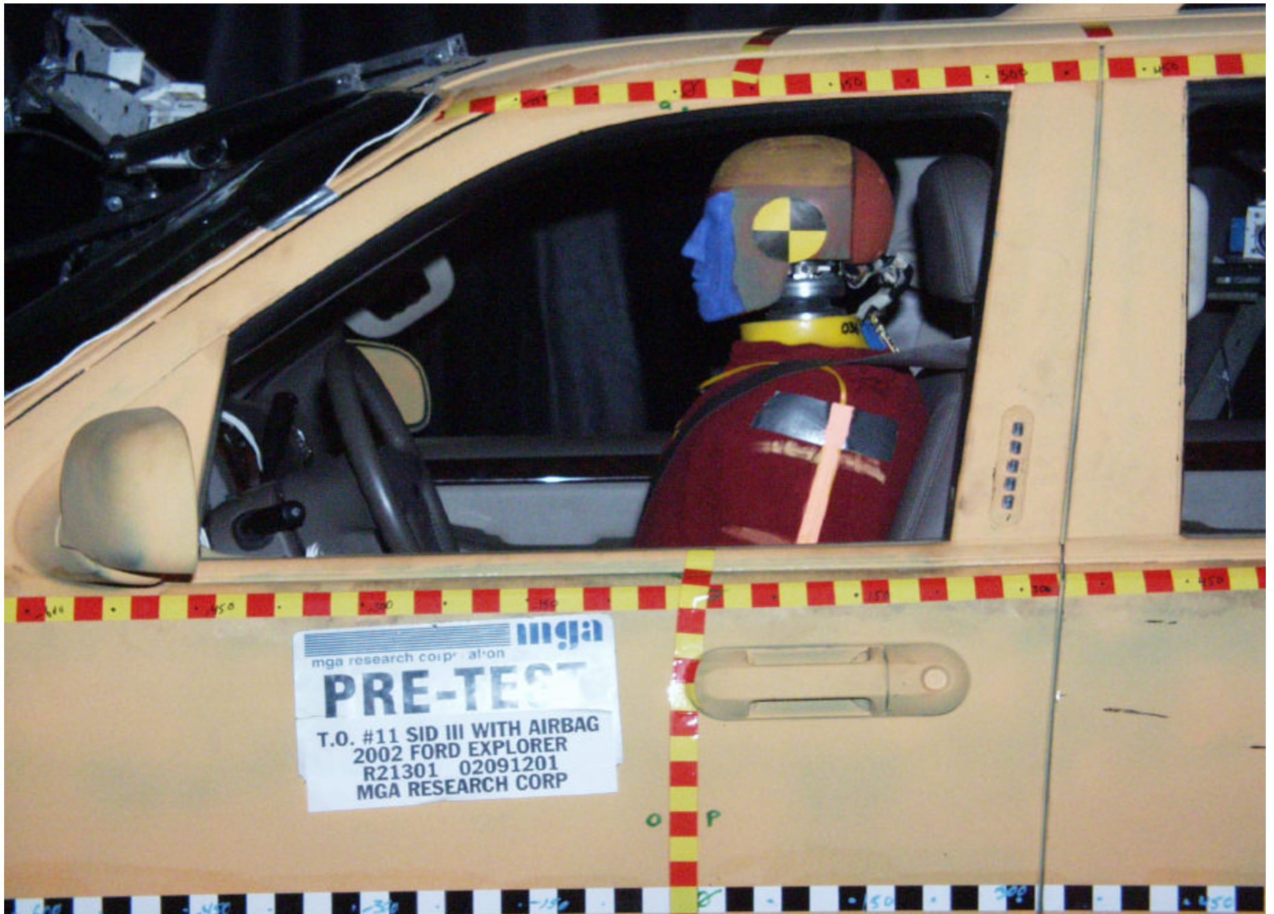
Pre-Test Driver Dummy Left Side View
