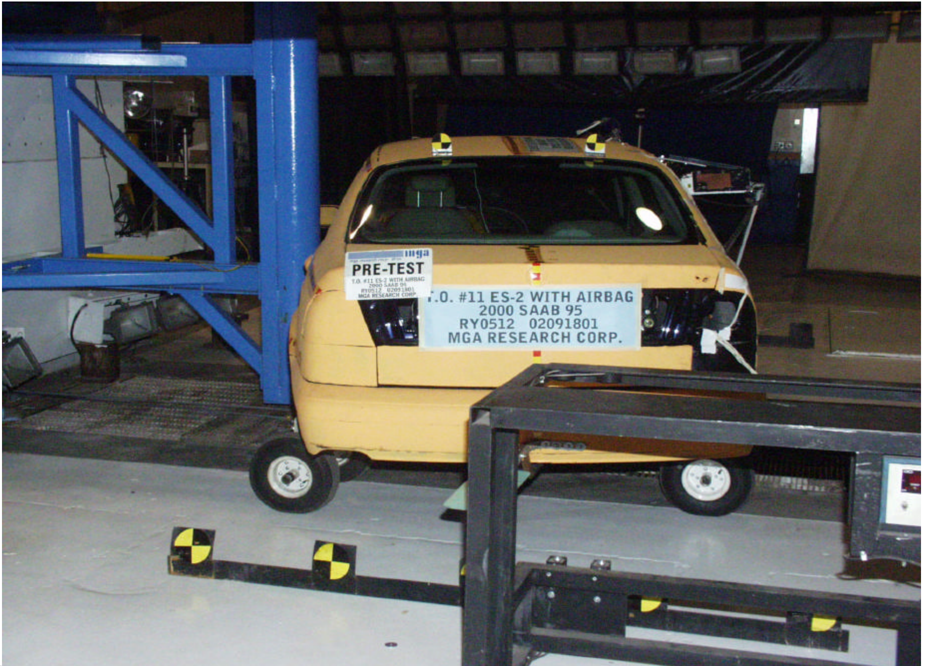
Pre-Test Vehicle Positioned Against Pole (right side)
