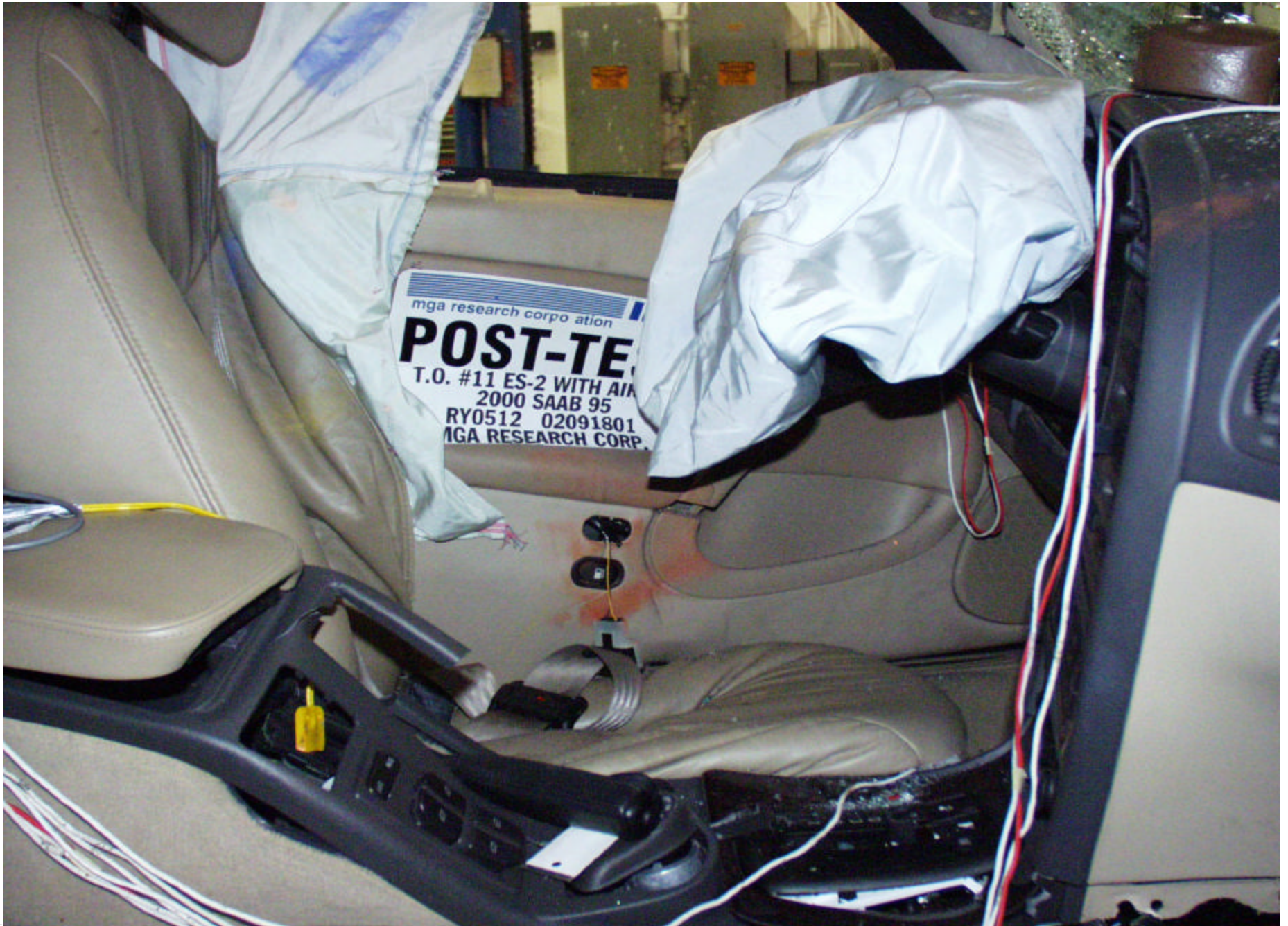
Post-Test Driver Dummy Lower Body Contact
