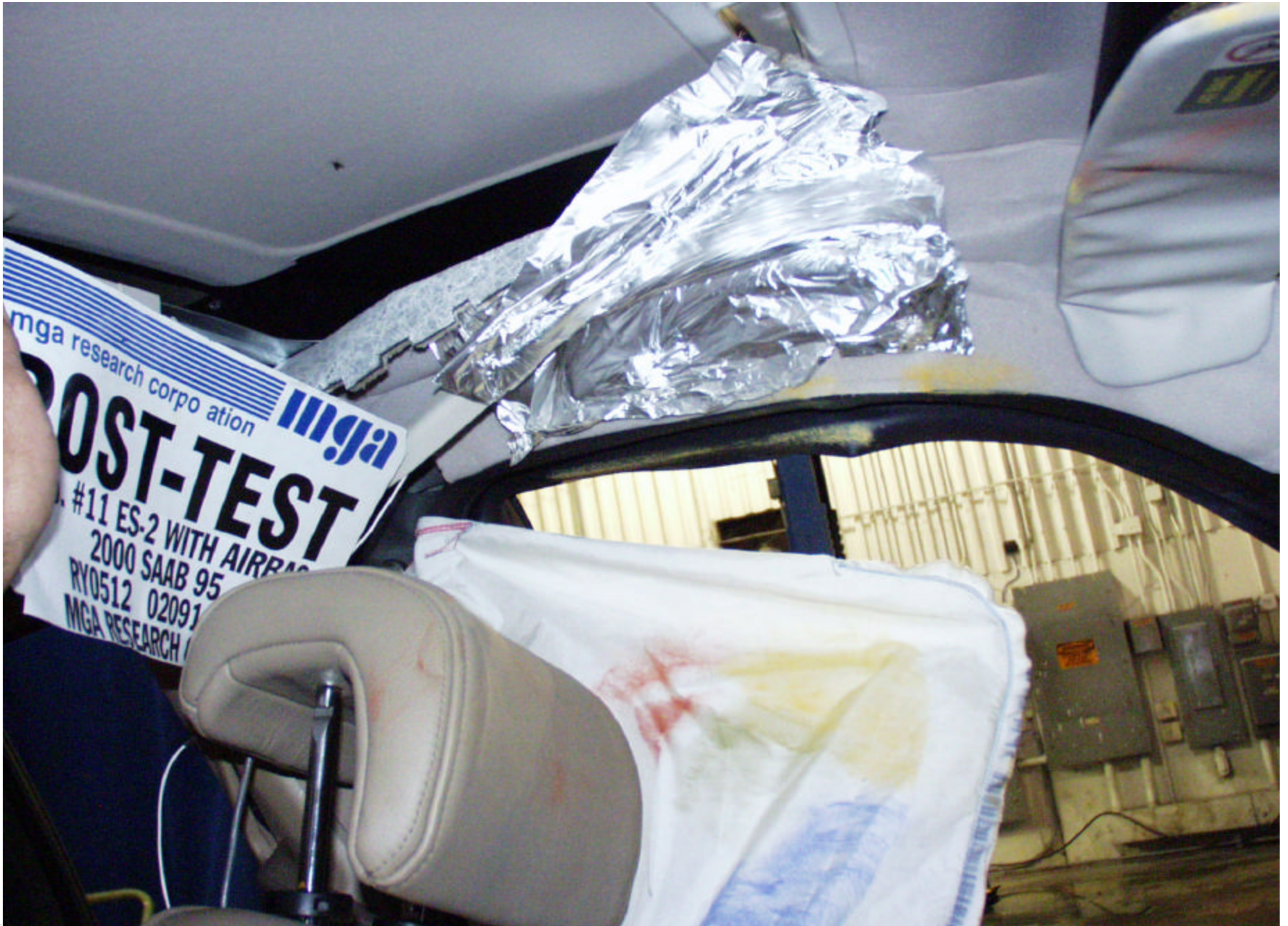
Post-Test Driver Dummy Head Contact
