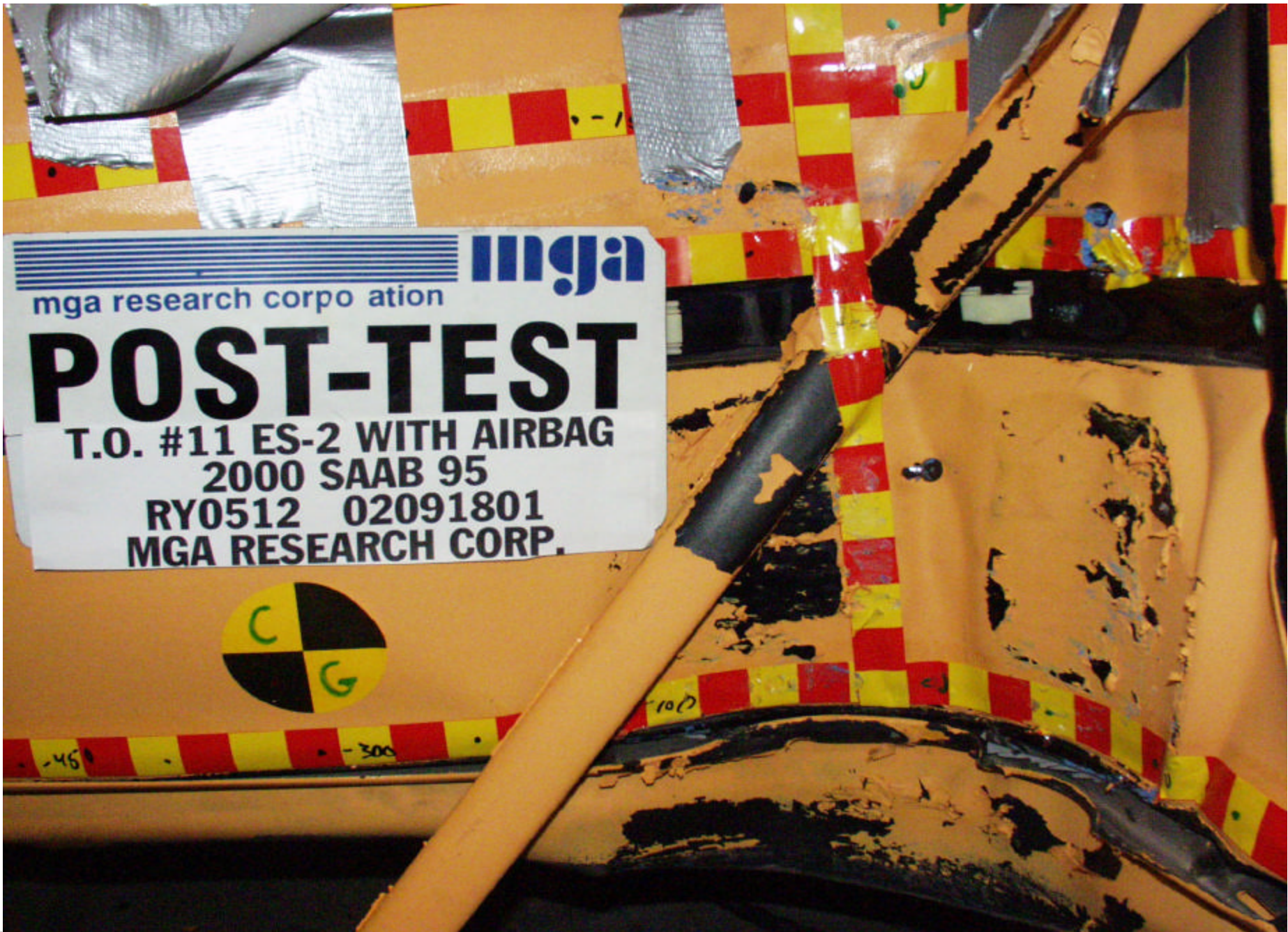
Post-Test Impact Point on Vehicle
