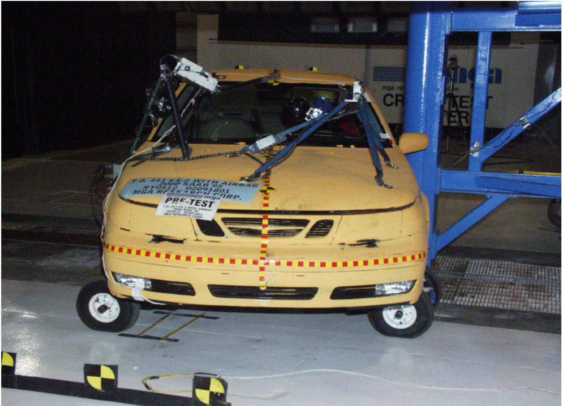
Pre-Test Vehicle Positioned Against Pole (left side)
