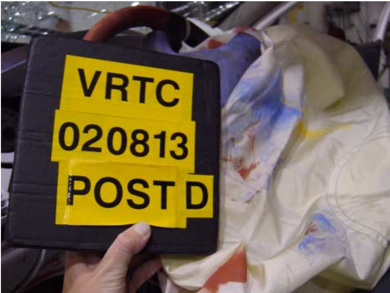
Figure A-68 Post-Test Driver Dummy Head Contact - View 2
