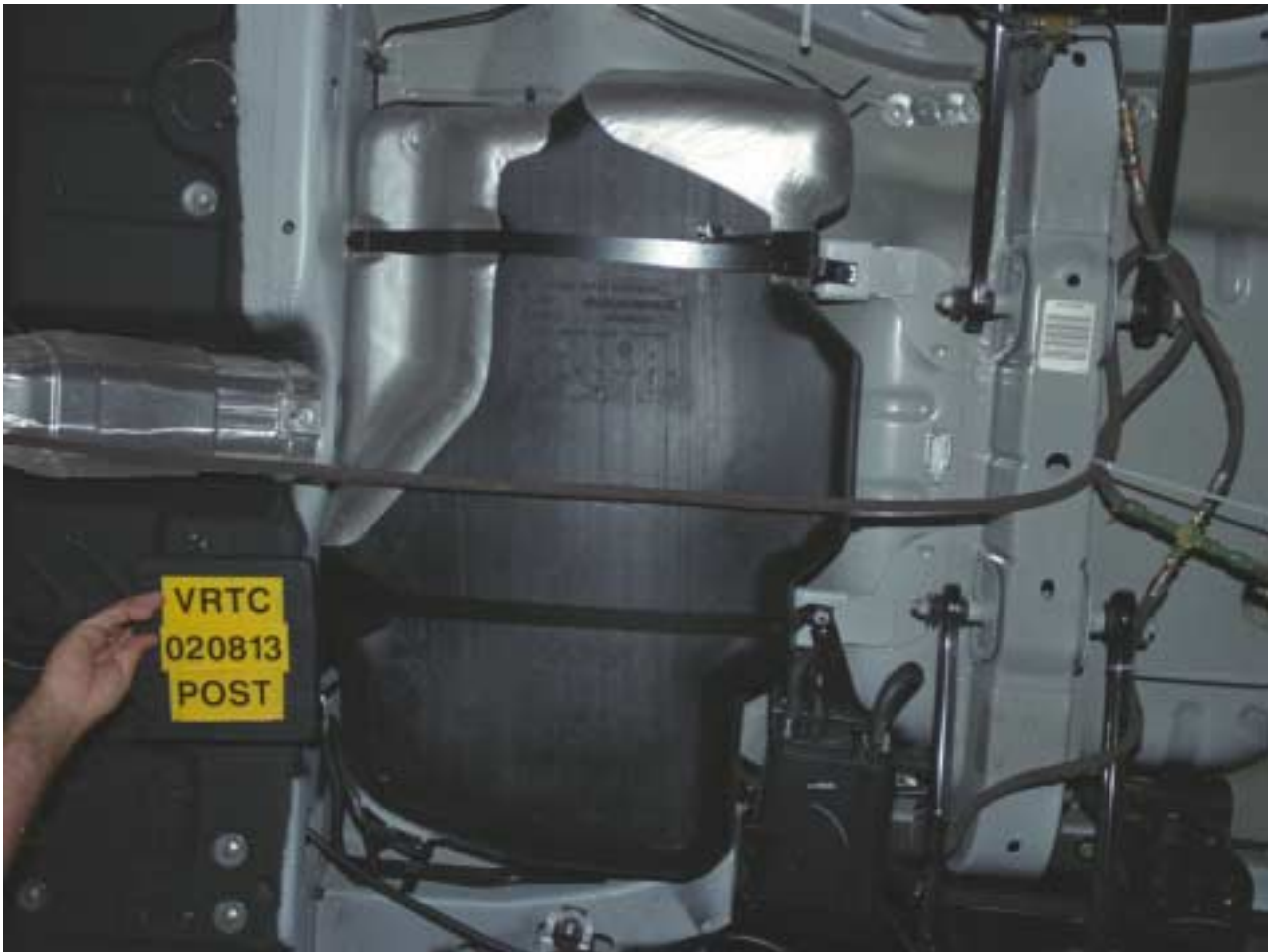
Figure A-27 Post-Test Fuel Tank View
