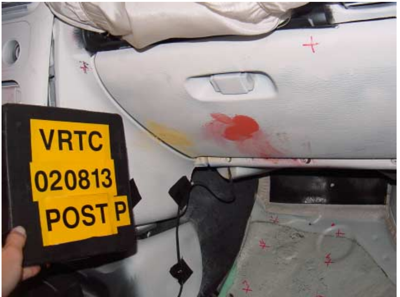
Figure A-80 Post-Test Passenger Dummy Knee Contact View
