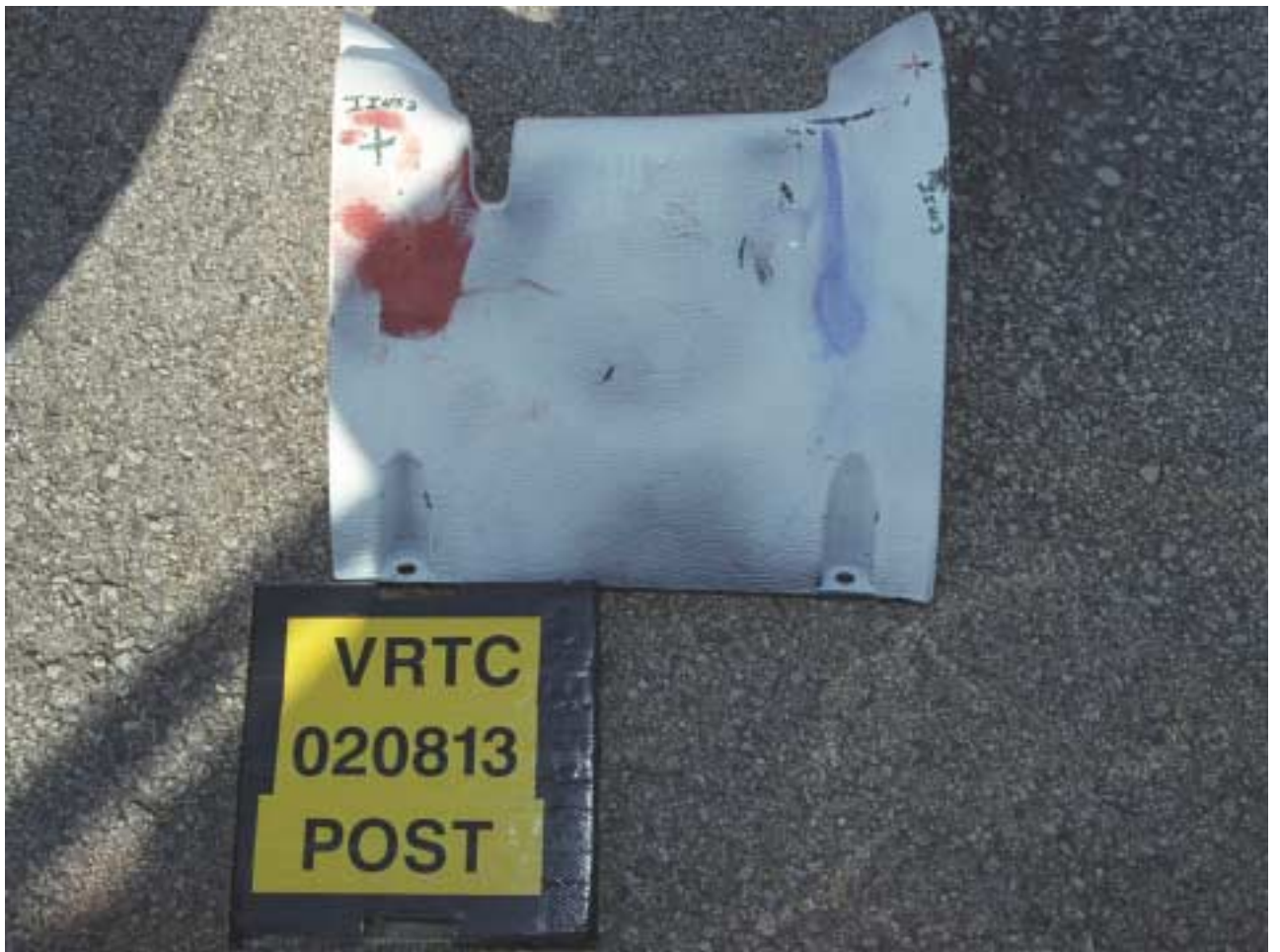
Figure A-74 Post-Test Driver Knee Contact - View 3
