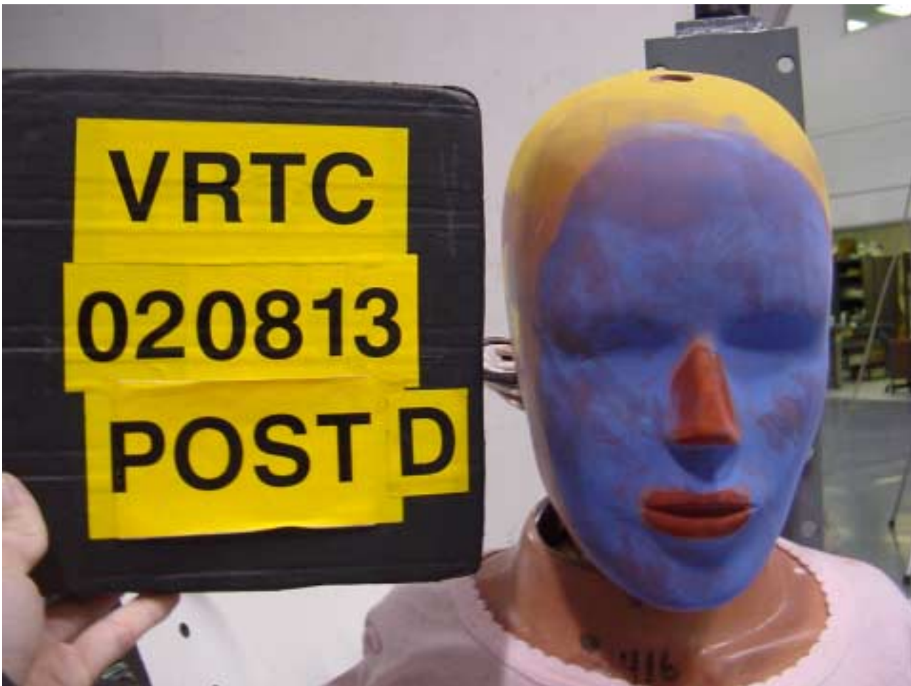
Figure A-67 Post-Test Driver Dummy Head Contact - View 1
