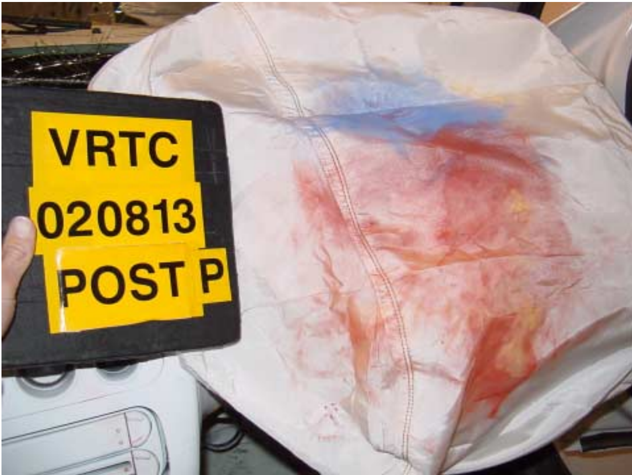
Figure A-78 Post-Test Passenger Dummy Head Contact - View 2
