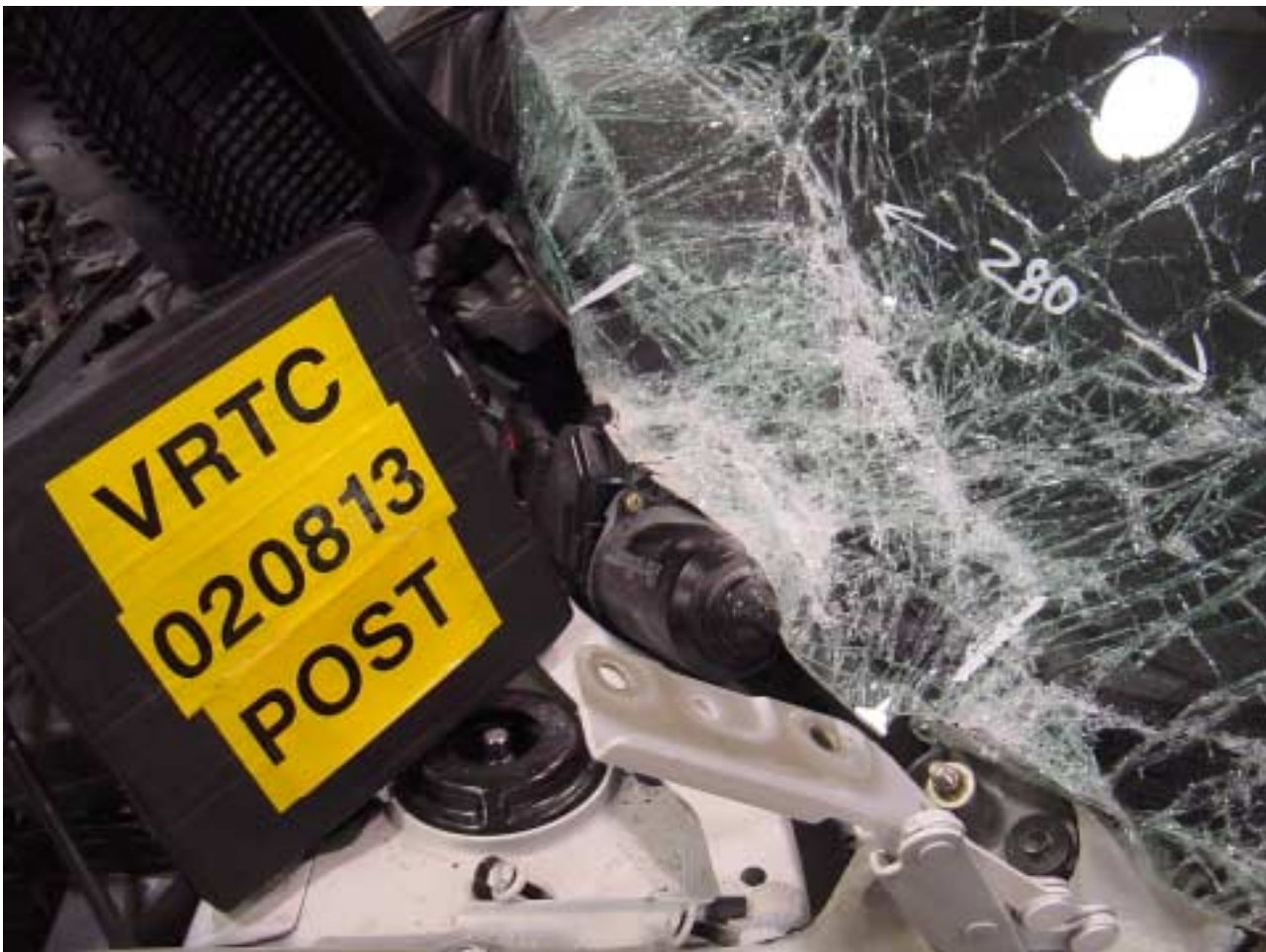
Figure A-36 Post-Test Left Side Windshield Close-up - View 1
