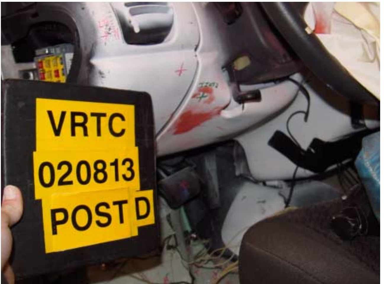
Figure A-73 Post-Test Driver Knee Contact - View 2
