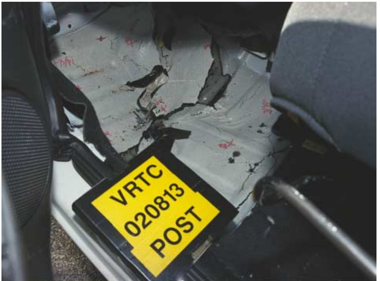
Figure A-75 Post-Test Driver Toeboard/Floorpan with Carpet Removed View
