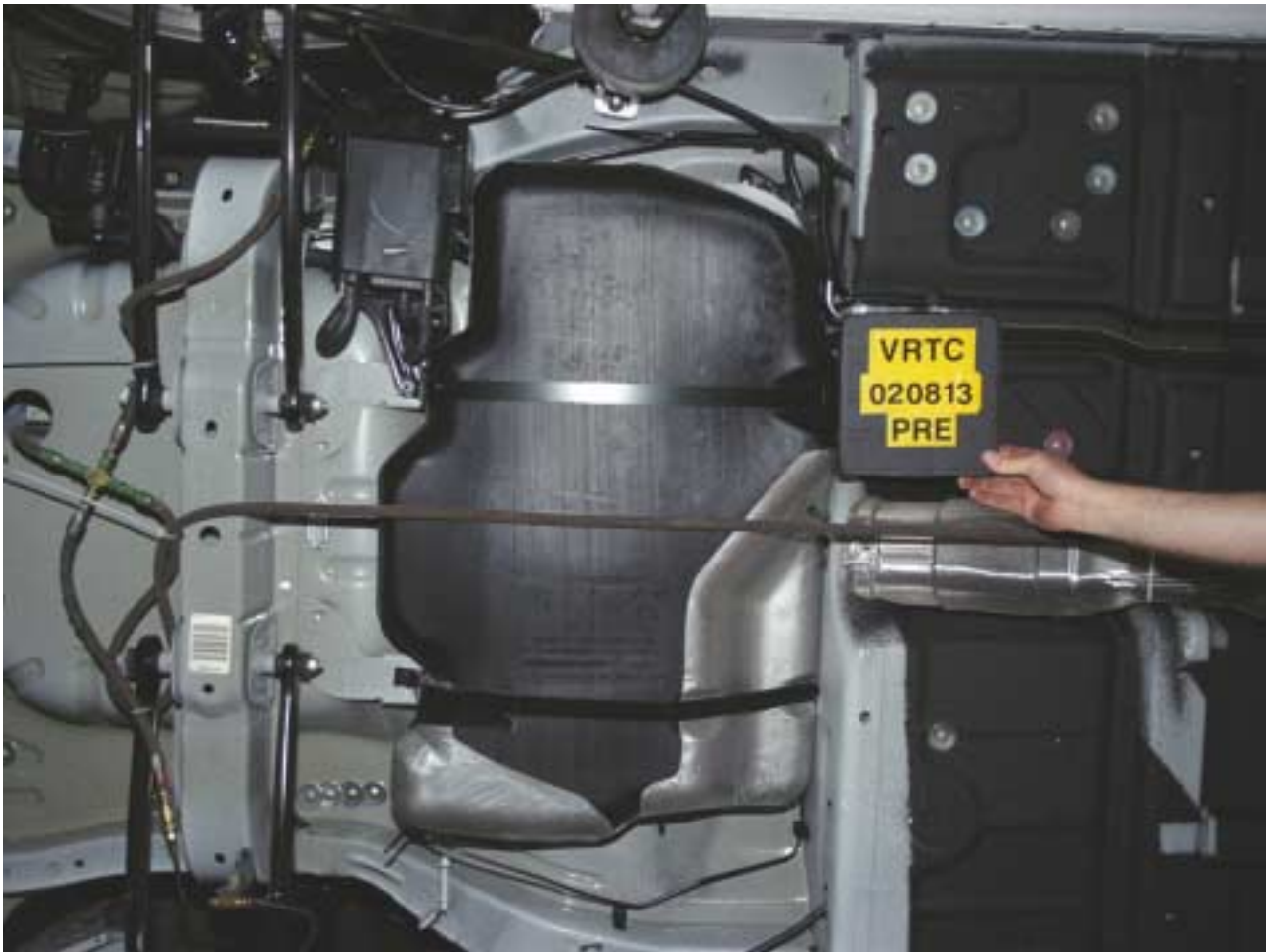
Figure A-26 Pre-Test Fuel Tank View
