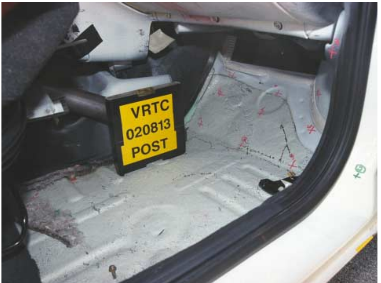
Figure A-81 Post-Test Passenger Toeboard/Floorpan with Carpet Removed View
