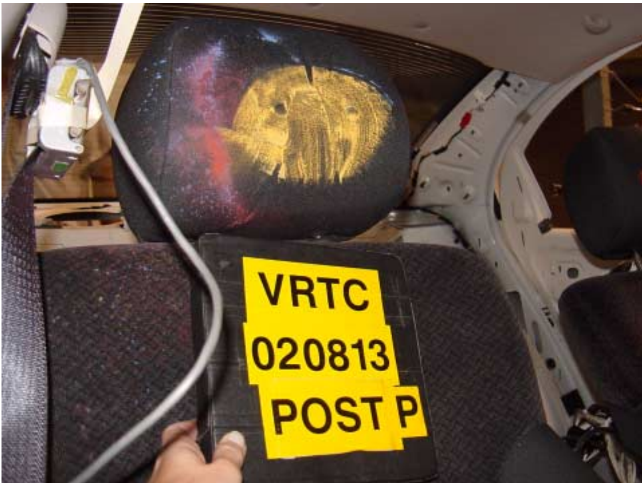
Figure A-79 Post-Test Passenger Dummy Head Contact - View 3
