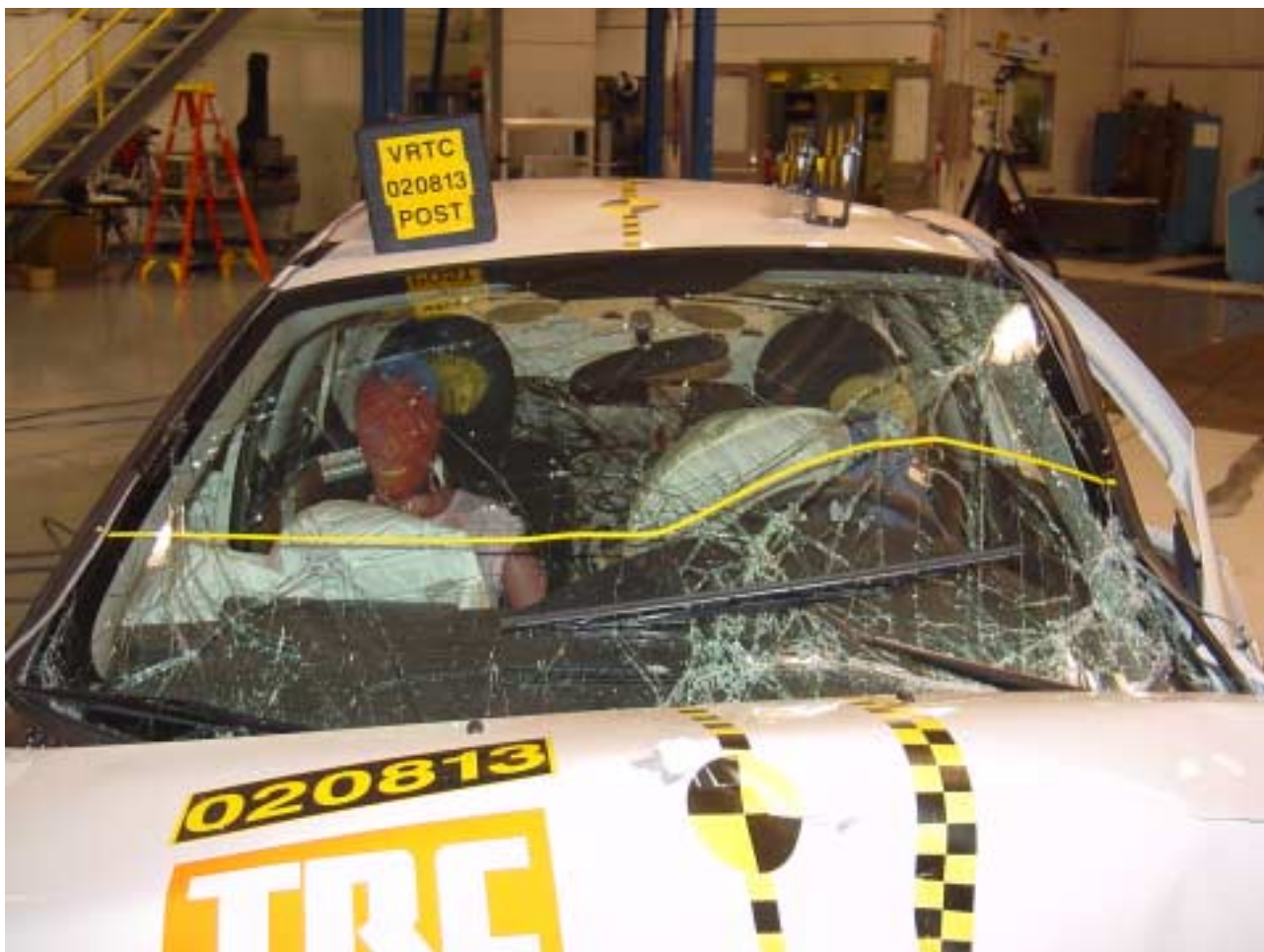
Figure A-33 Post-Test Windshield View
