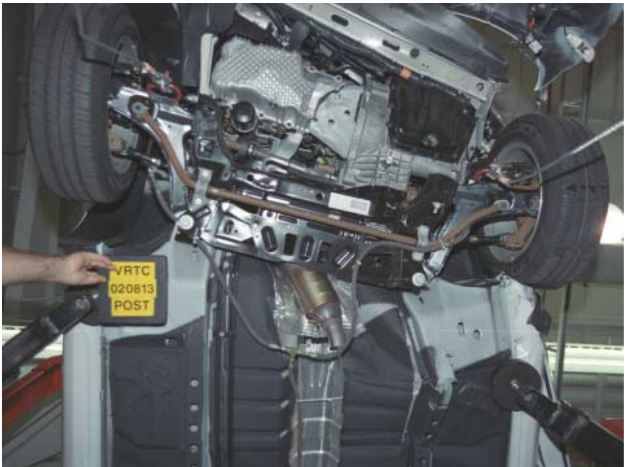
Figure A-21 Post-Test Front Mid Underbody View
