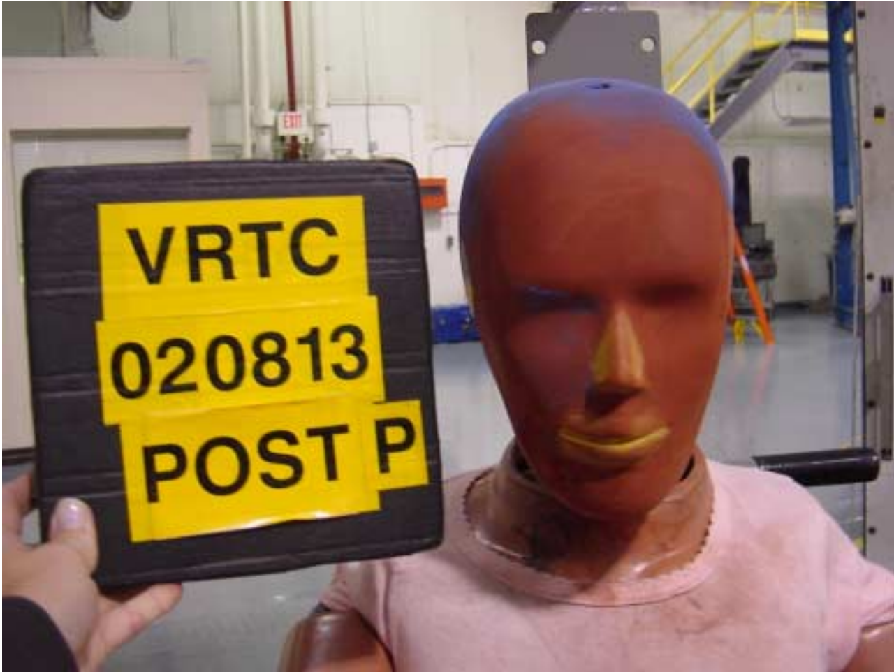
Figure A-77 Post-Test Passenger Dummy Head Contact - View 1
