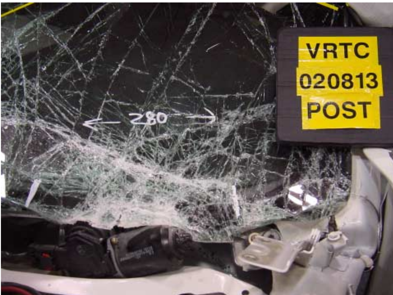
Figure A-37 Post-Test Left Side Windshield Close-up - View 2
