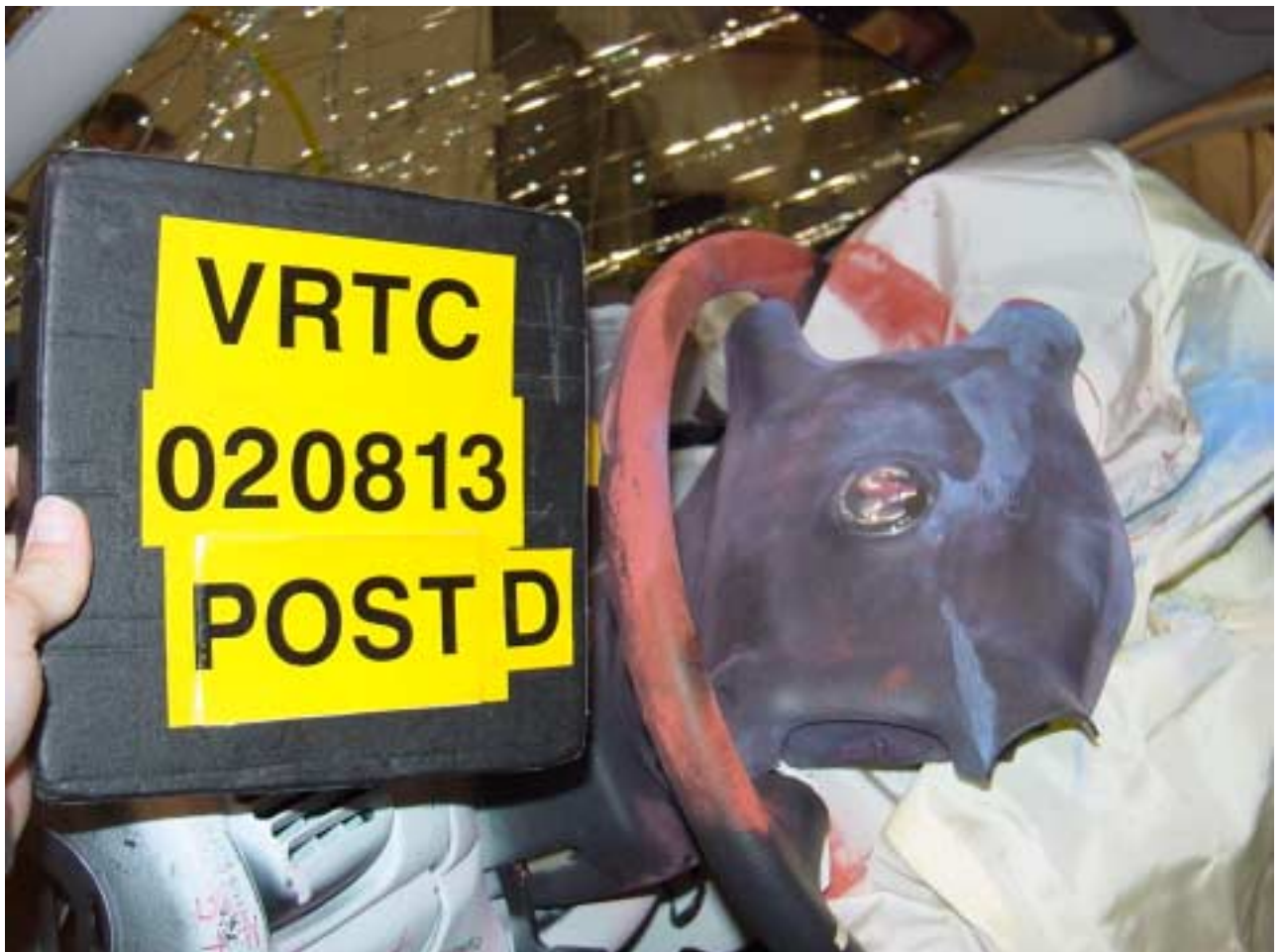
Figure A-71 Post-Test Driver Dummy Chest Contact View
