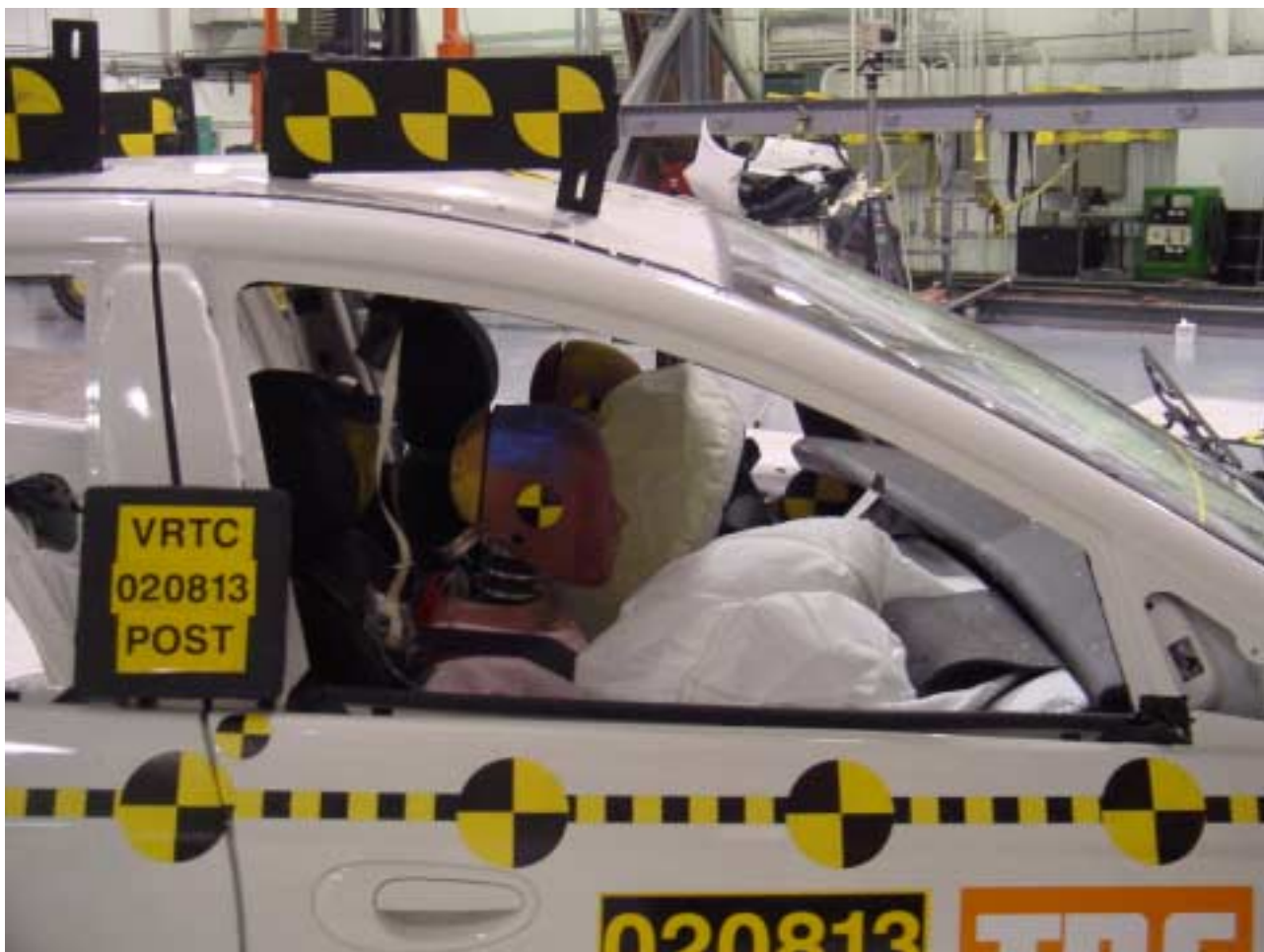
Figure A-61 Post-Test Passenger Dummy Position - View 2
