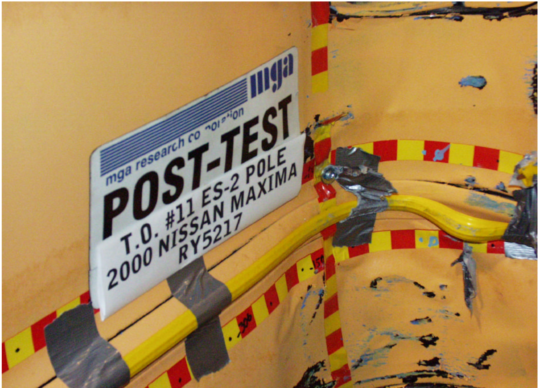
Post-Test Impact Point on Vehicle
