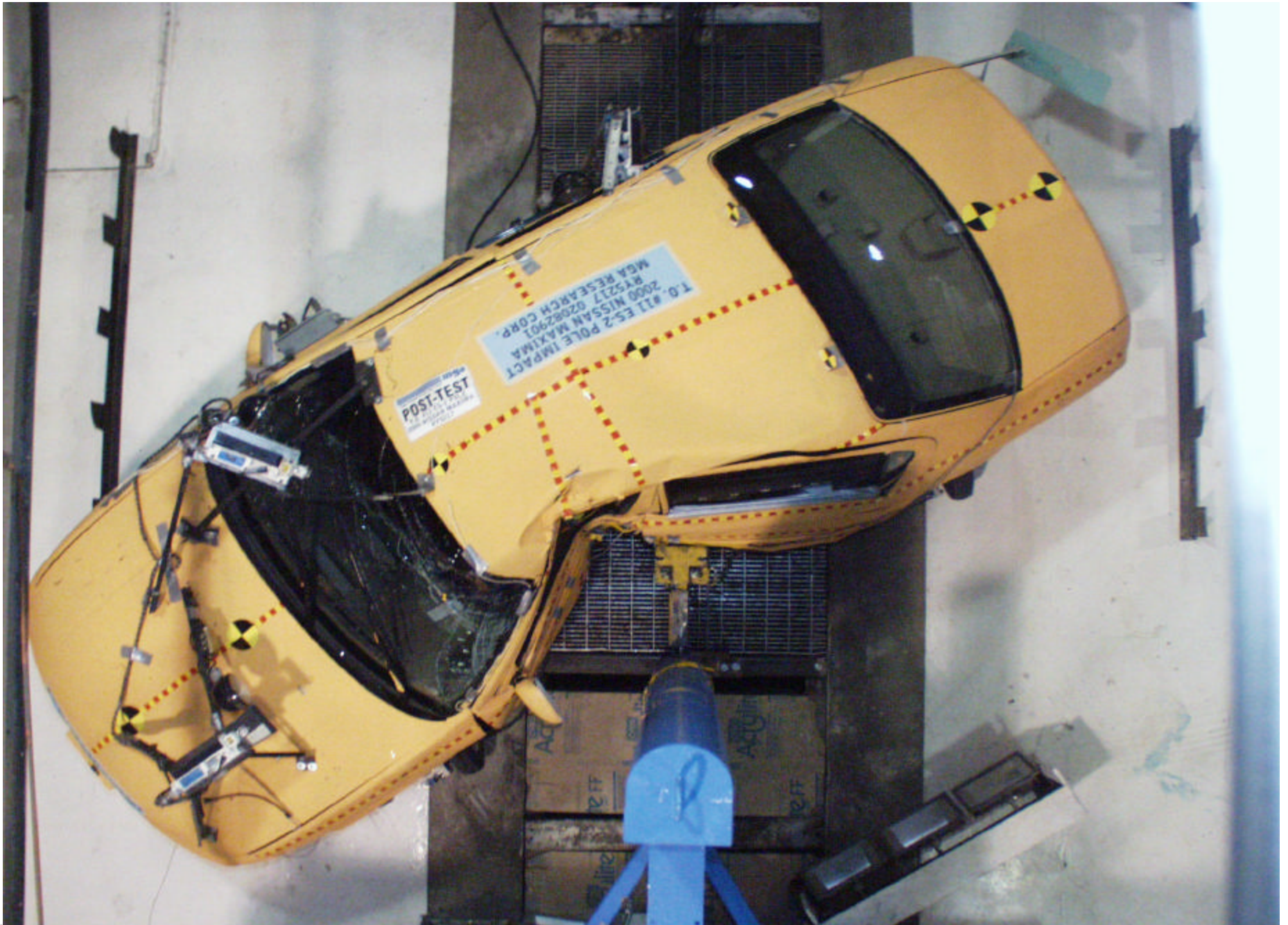
Post-Test Vehicle and Pole Overhead View
