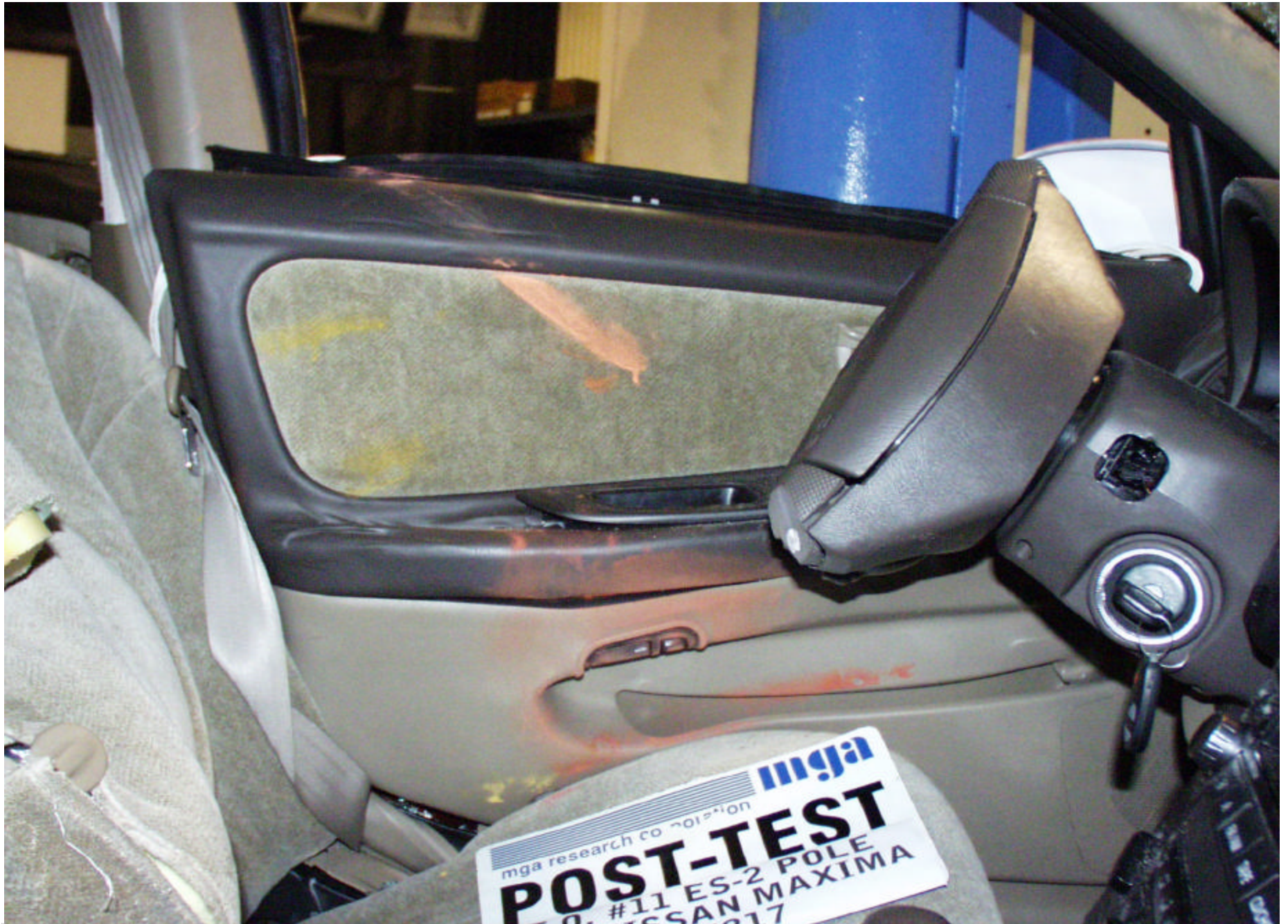
Post-Test Driver Dummy Contact
