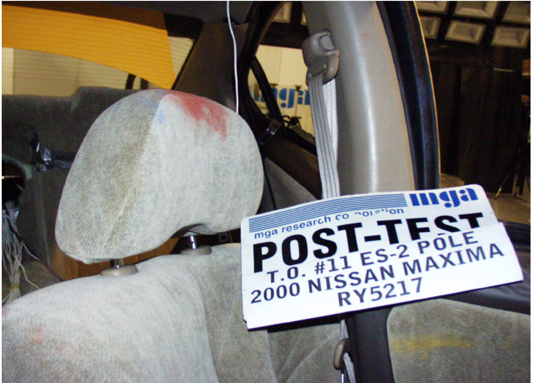
Post-Test Driver Dummy Head Contact
