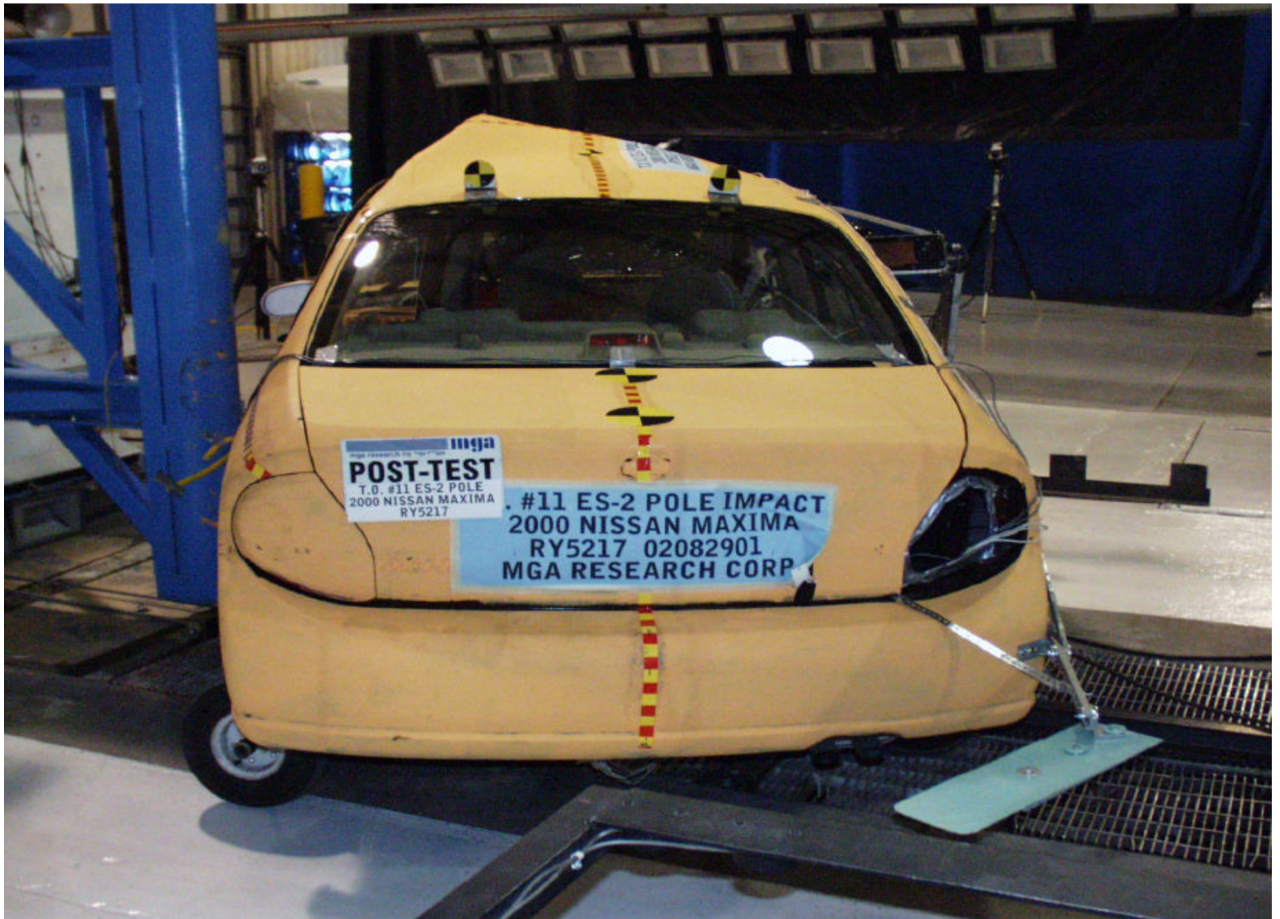
Post-Test Rear View of Test Vehicle and Pole
