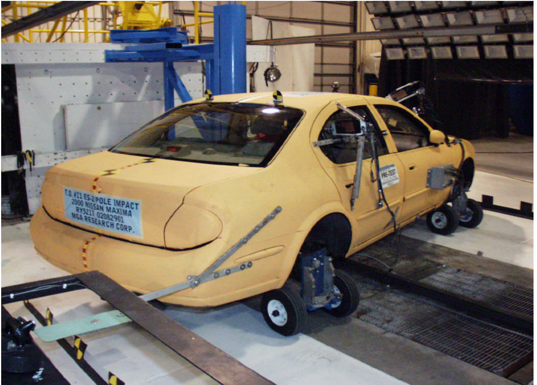
Pre-Test Right Rear \frac{3}{4} View of Test Vehicle and Pole
