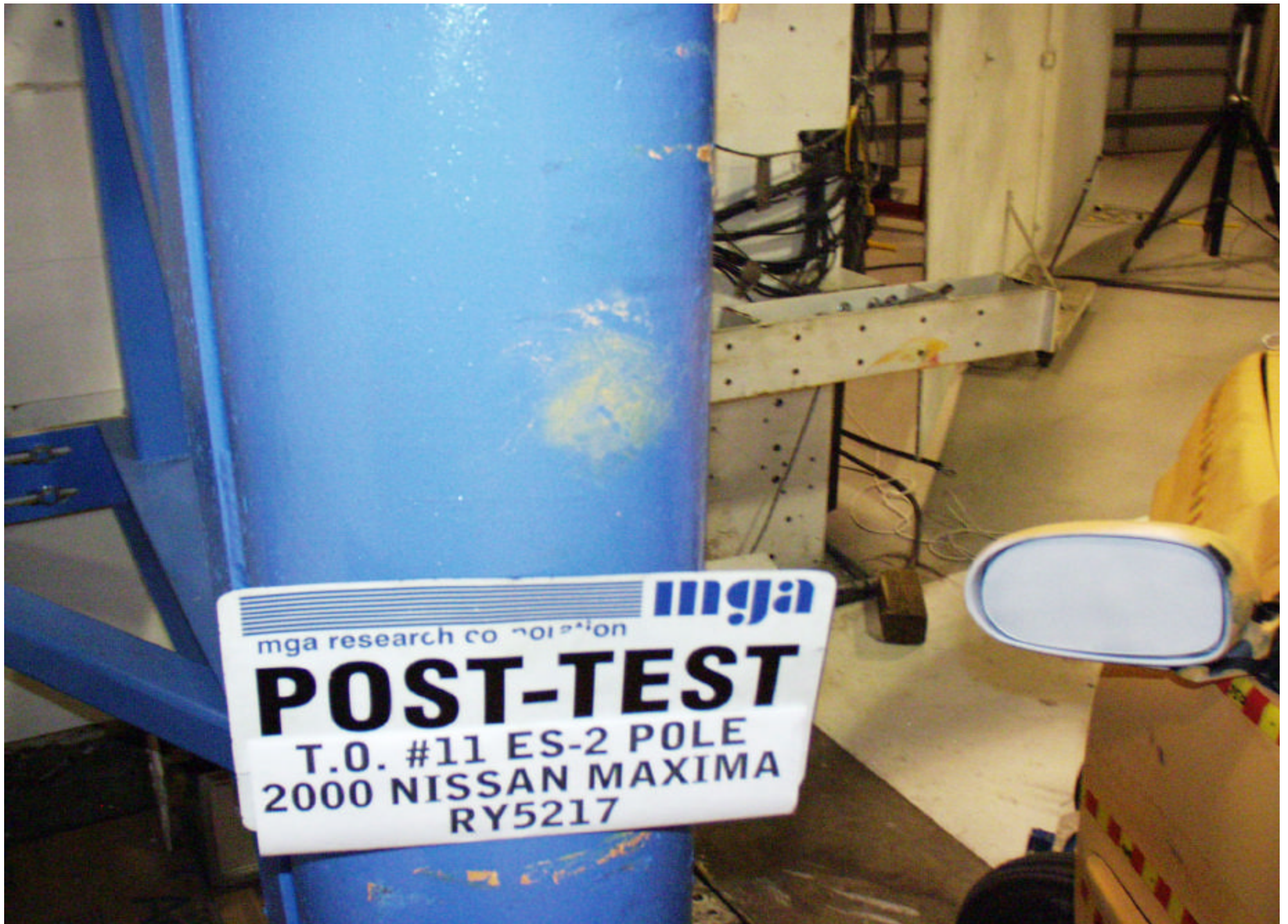
Post-Test Driver Dummy Pole Contact
