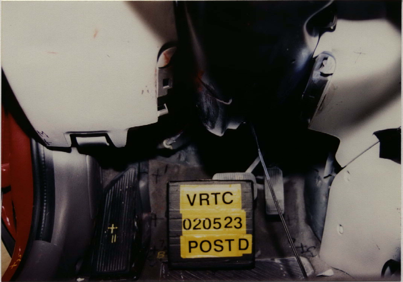
Figure A-59 Post-Test Driver Dummy Knee Contact and Toeboard Damage View
