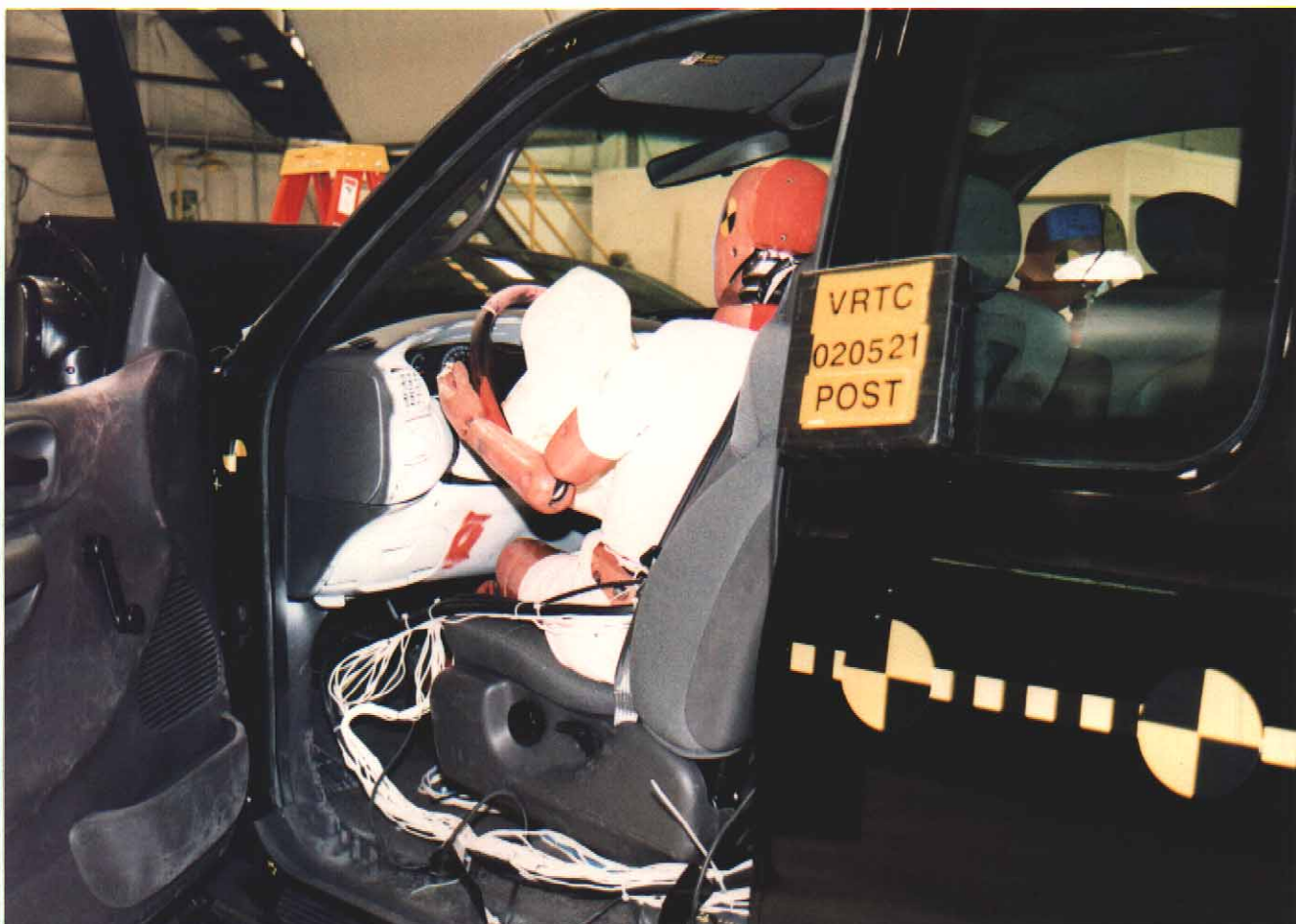
Figure A-44 Post-Test Driver Dummy & Vehicle Interior - View 2
