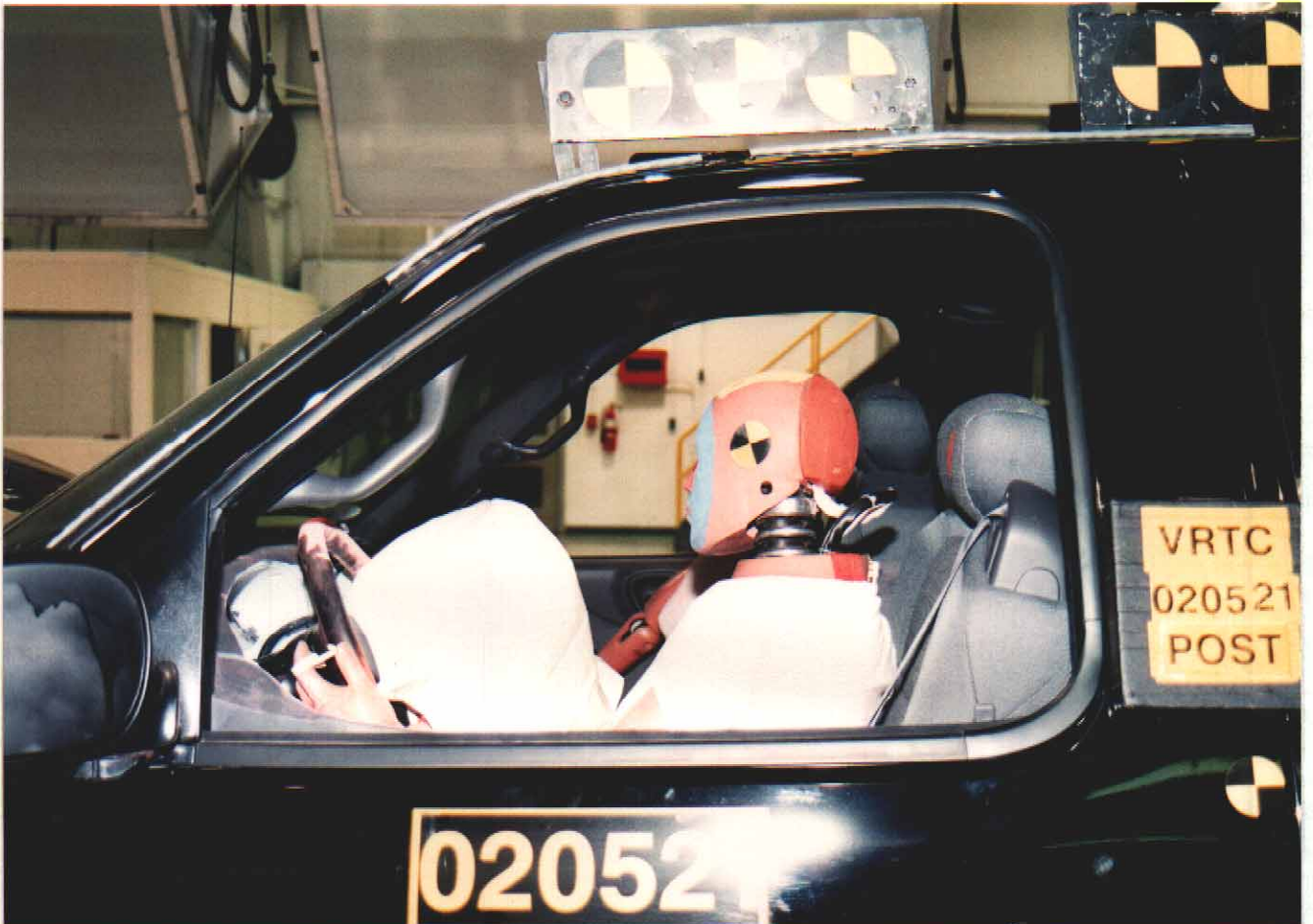
Figure A-40 Post-Test Driver Dummy Position - View 2
