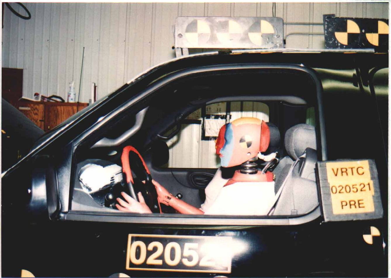
Figure A-39 Pre-Test Driver Dummy Position - View 2
