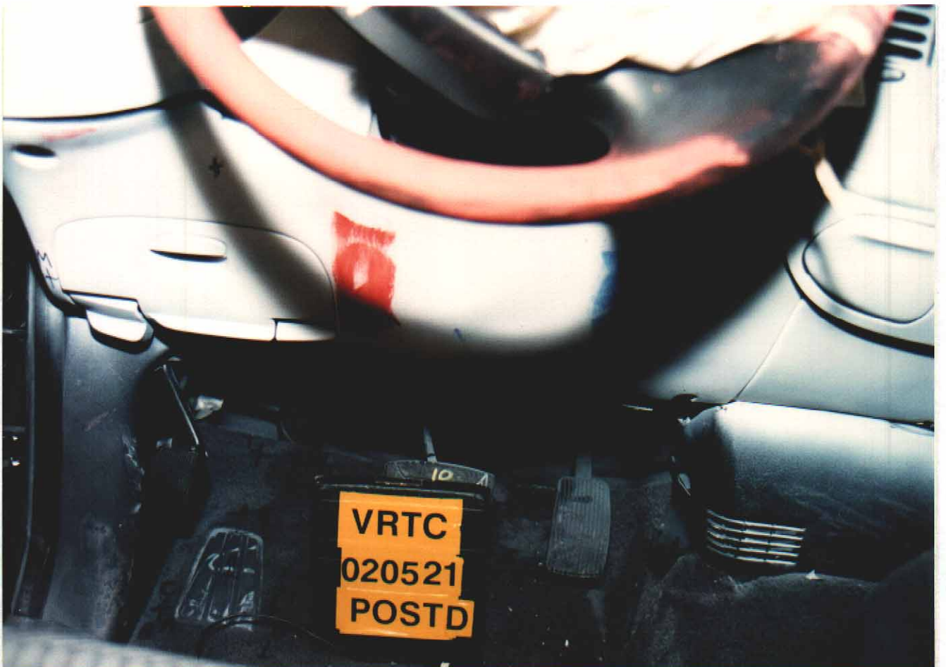
Figure A-58 Post-Test Driver Dummy Knee Contact - View 2
