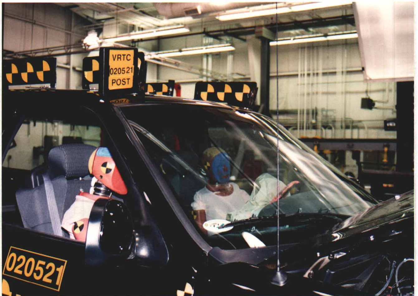
Figure A-34 Post-Test Right Front Windshield View
