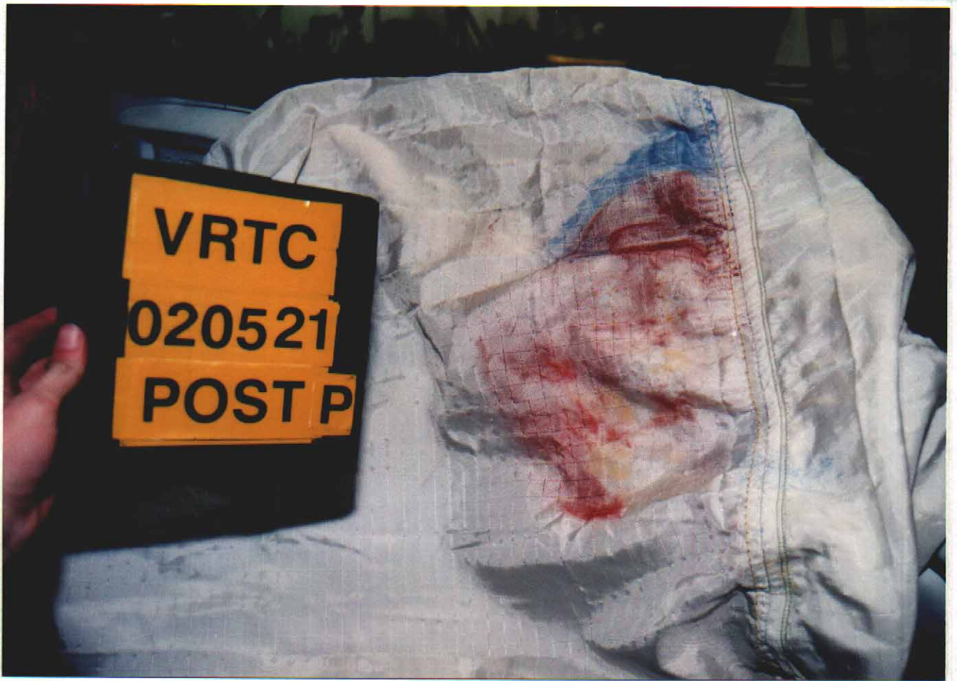
Figure A-61 Post-Test Passenger Dummy Head Contact - View 2
