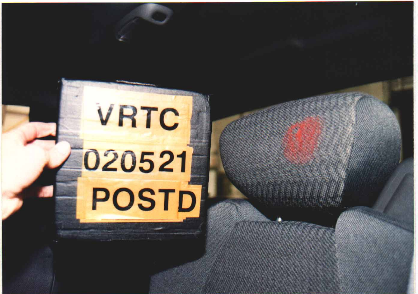
Figure A-56 Post-Test Driver Dummy Head Contact - View 3
