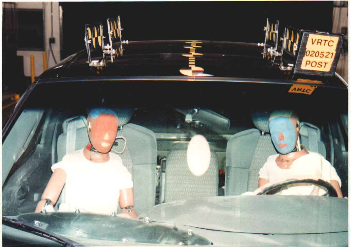
Figure A-36 Post-Test Driver and Passenger Dummies Front View
