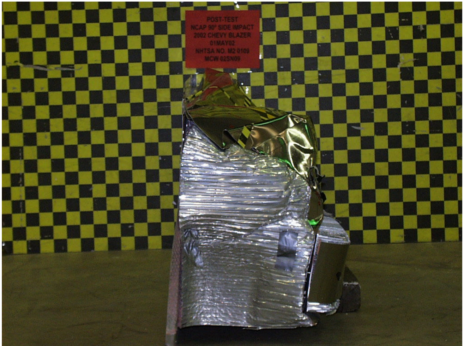
Figure A-49: POST-TEST ALUMINUM BARRIER RIGHT SIDE
