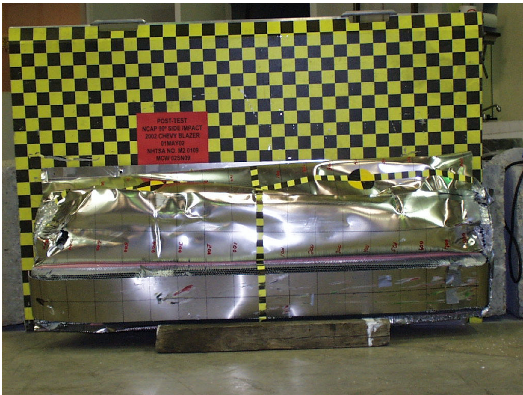
Figure A-45: POST-TEST ALUMINUM BARRIER FRONT
