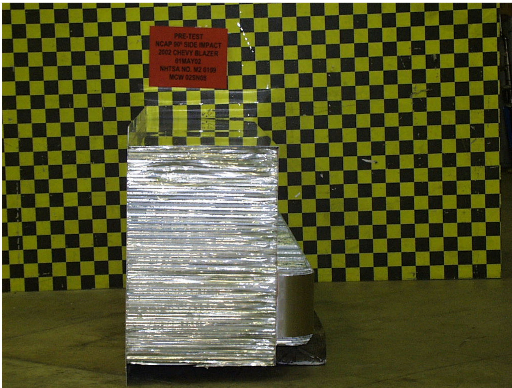
Figure A-48: PRE-TEST ALUMINUM BARRIER RIGHT SIDE
