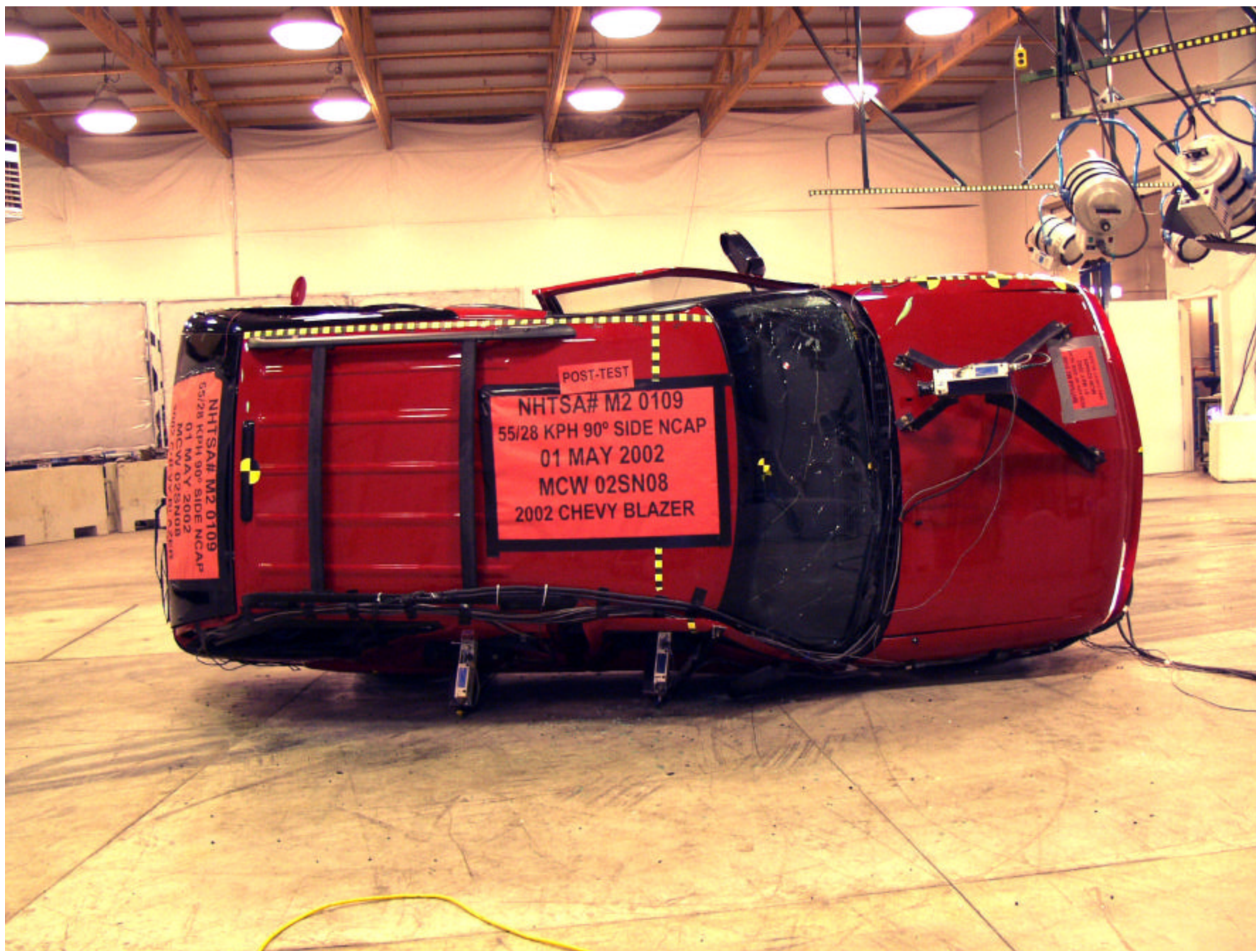
Figure A-17: TOP OF VEHICLE IN POST-TEST POSITION
