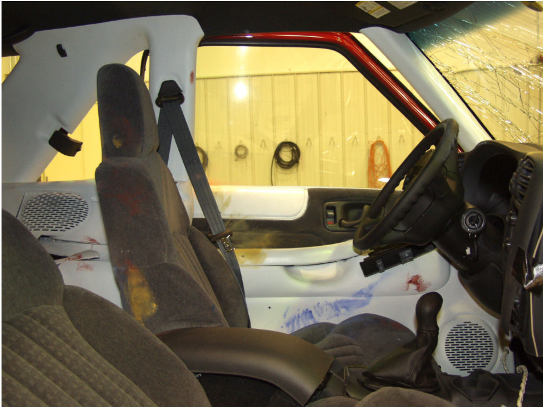
Figure A-28: POST-TEST INTERIOR OF FRONT DOOR SHOWING SID IMPACT LOCATIONS (Vehicle moved from post-crash position)
