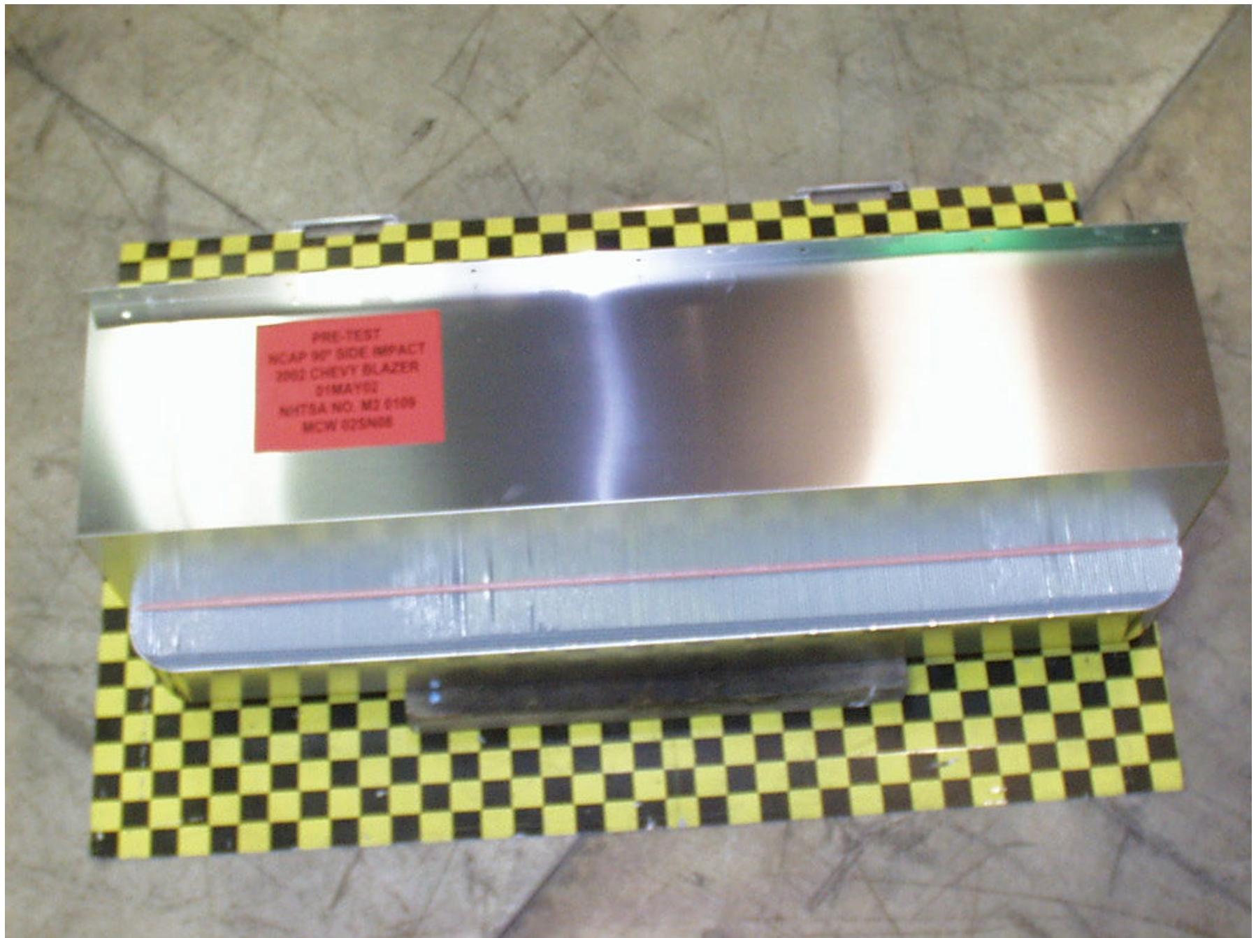
Figure A-50: PRE-TEST ALUMINUM BARRIER OVERHEAD
