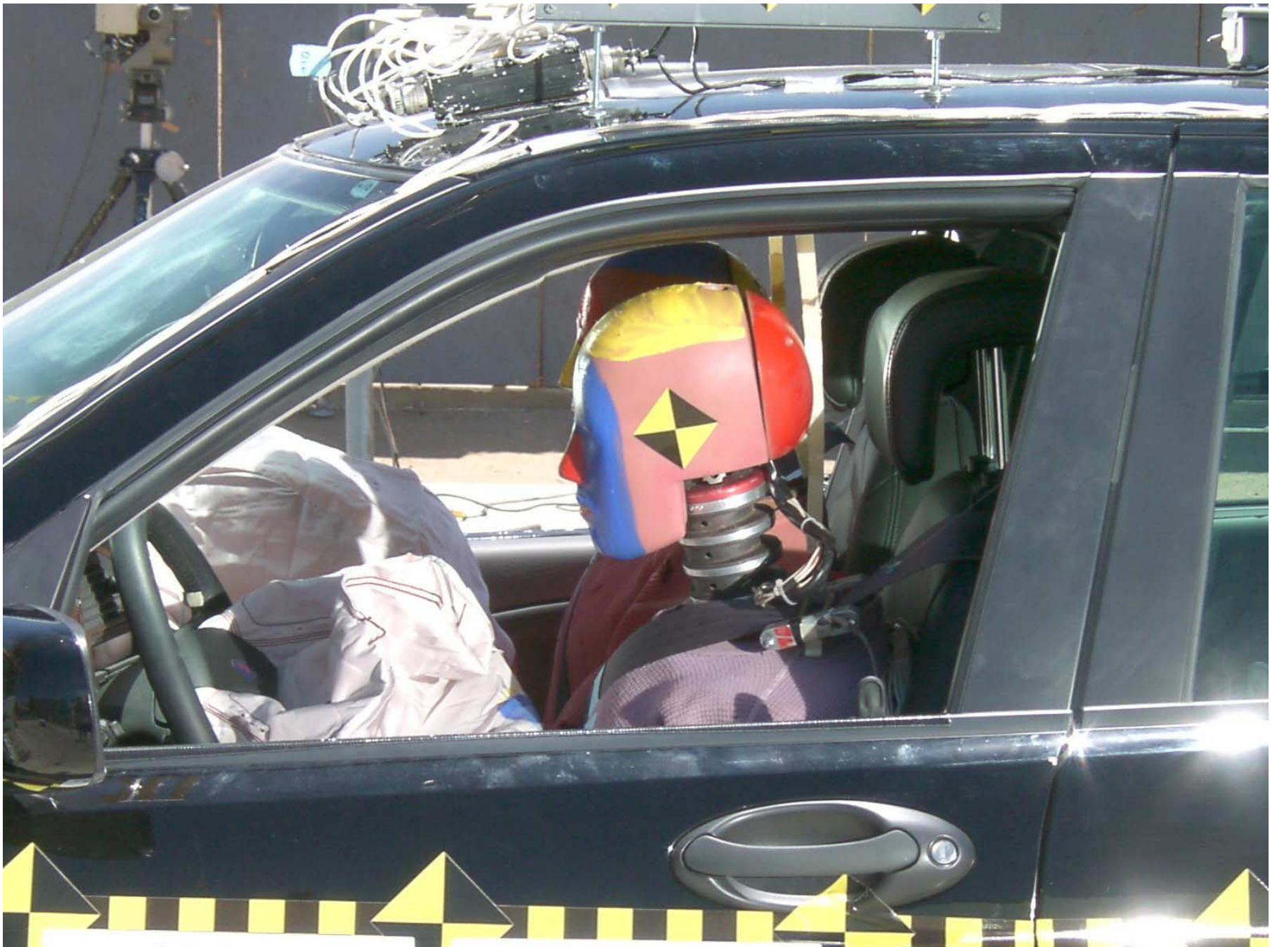
Figure A-28: Driver Dummy Through Window, Post-Test
