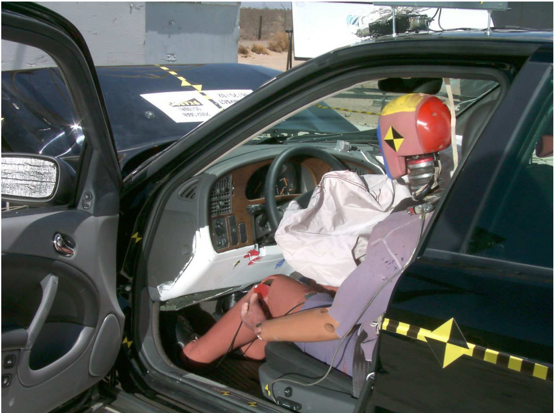
Figure A-30: Driver Dummy Door Open, Post-Test
