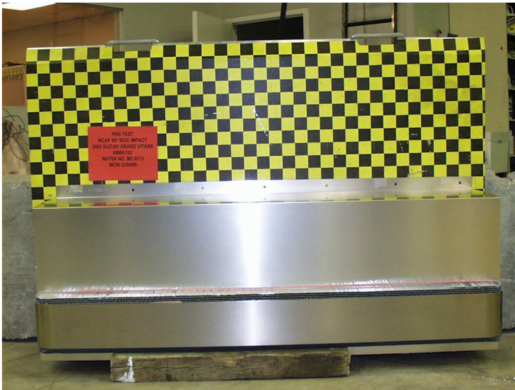
Figure A-45: PRE-TEST ALUMINUM BARRIER FRONT
