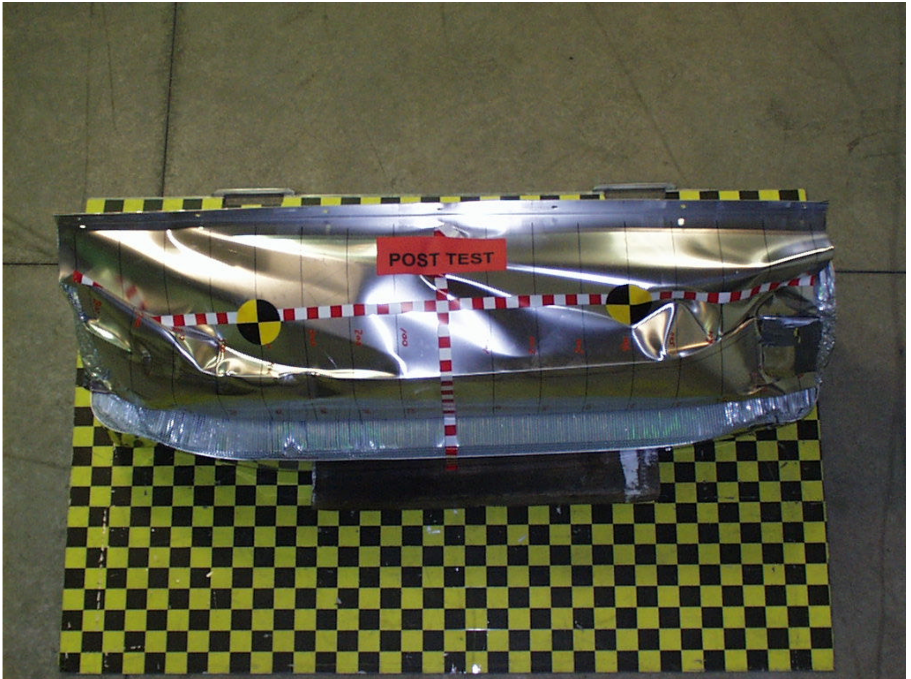
Figure A-52: POST-TEST ALUMINUM BARRIER OVERHEAD
