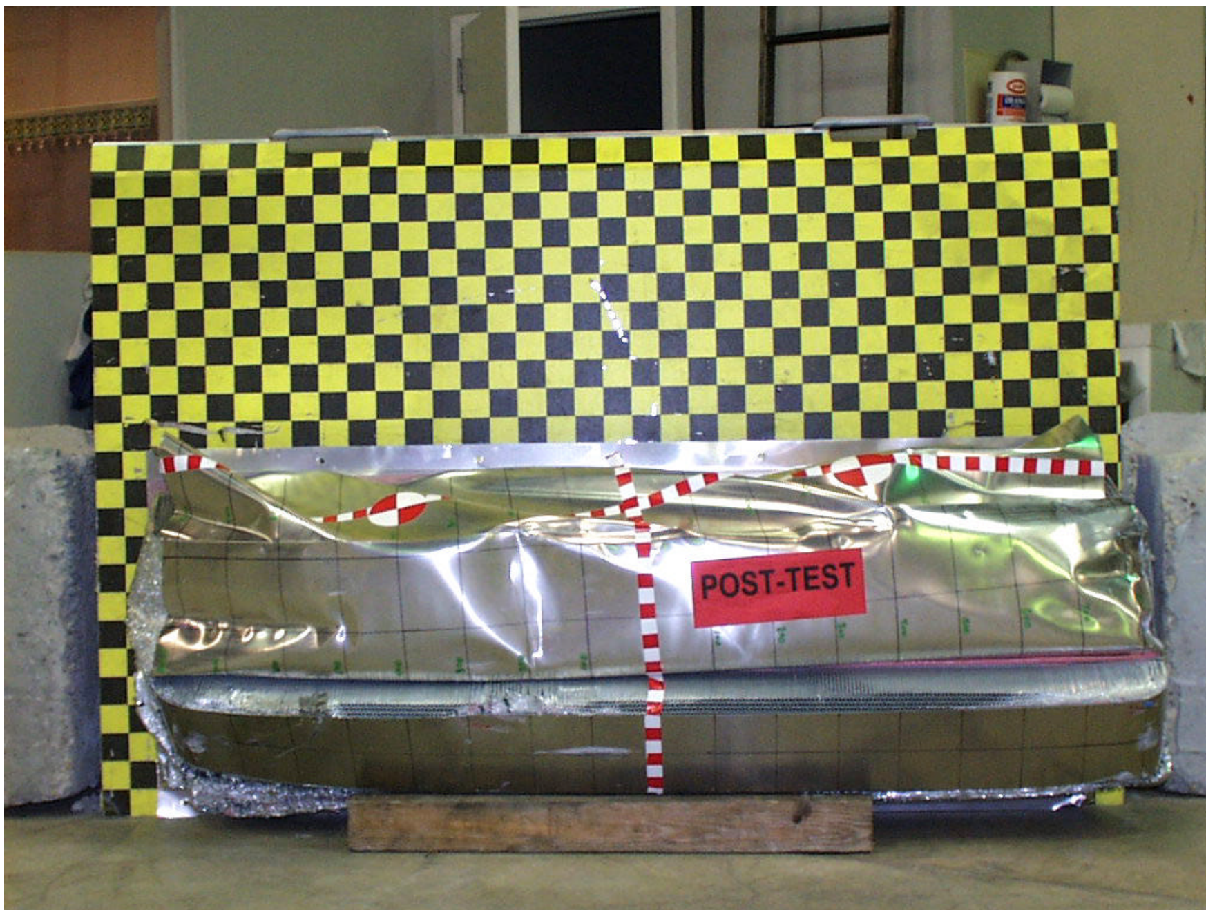
Figure A-46: POST-TEST ALUMINUM BARRIER FRONT
