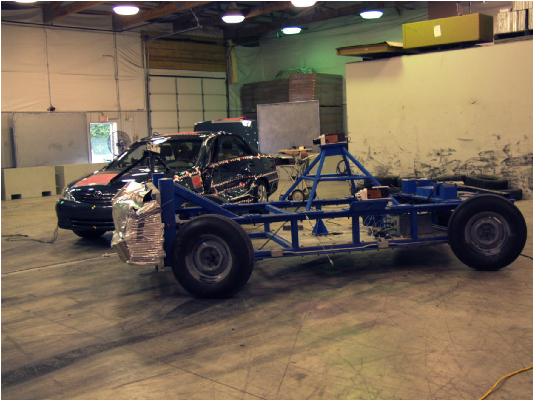
Figure A-30: POST-TEST LEFT SIDE VIEW OF MDB
