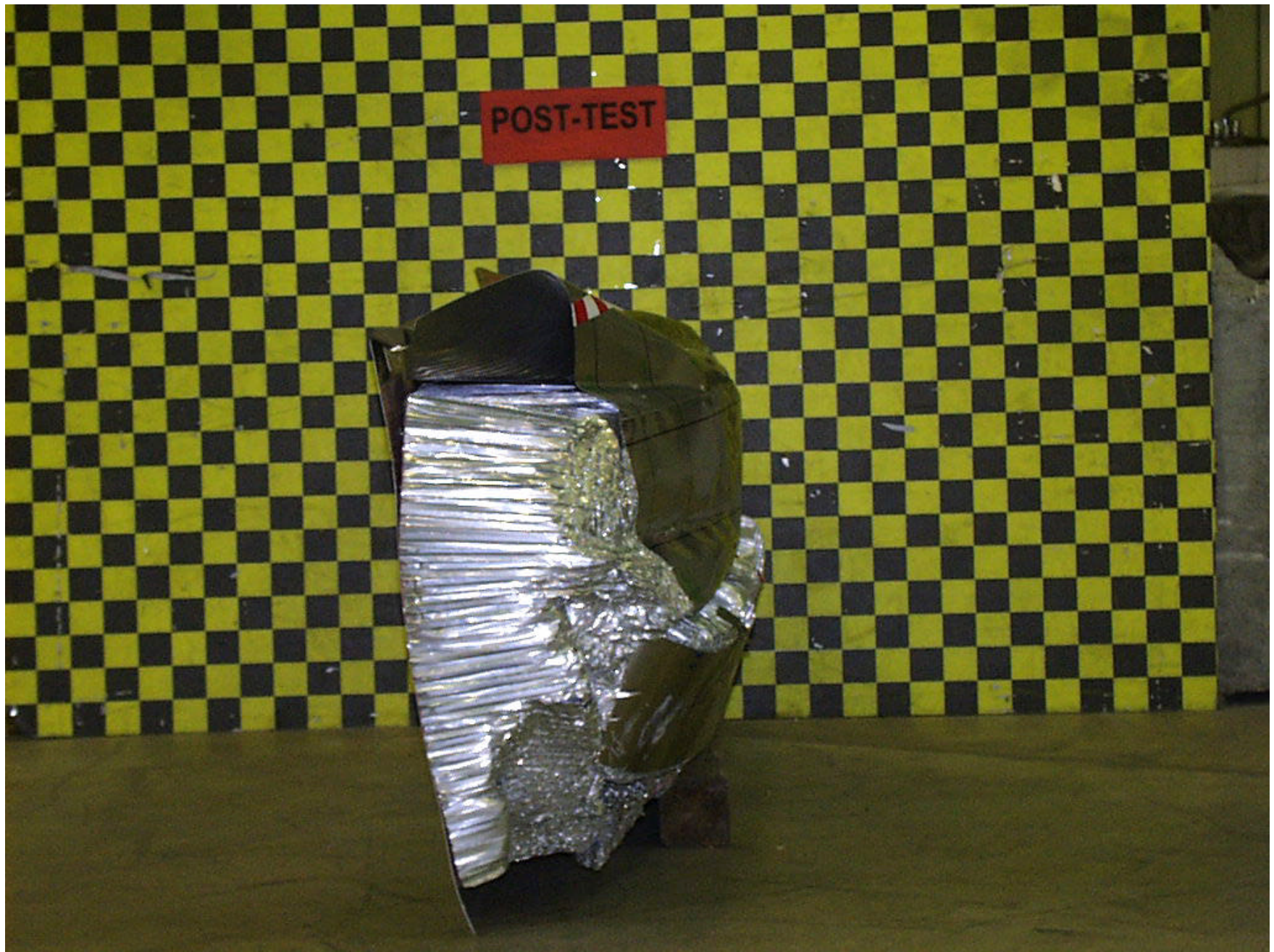
Figure A-50: POST-TEST ALUMINUM BARRIER RIGHT SIDE
