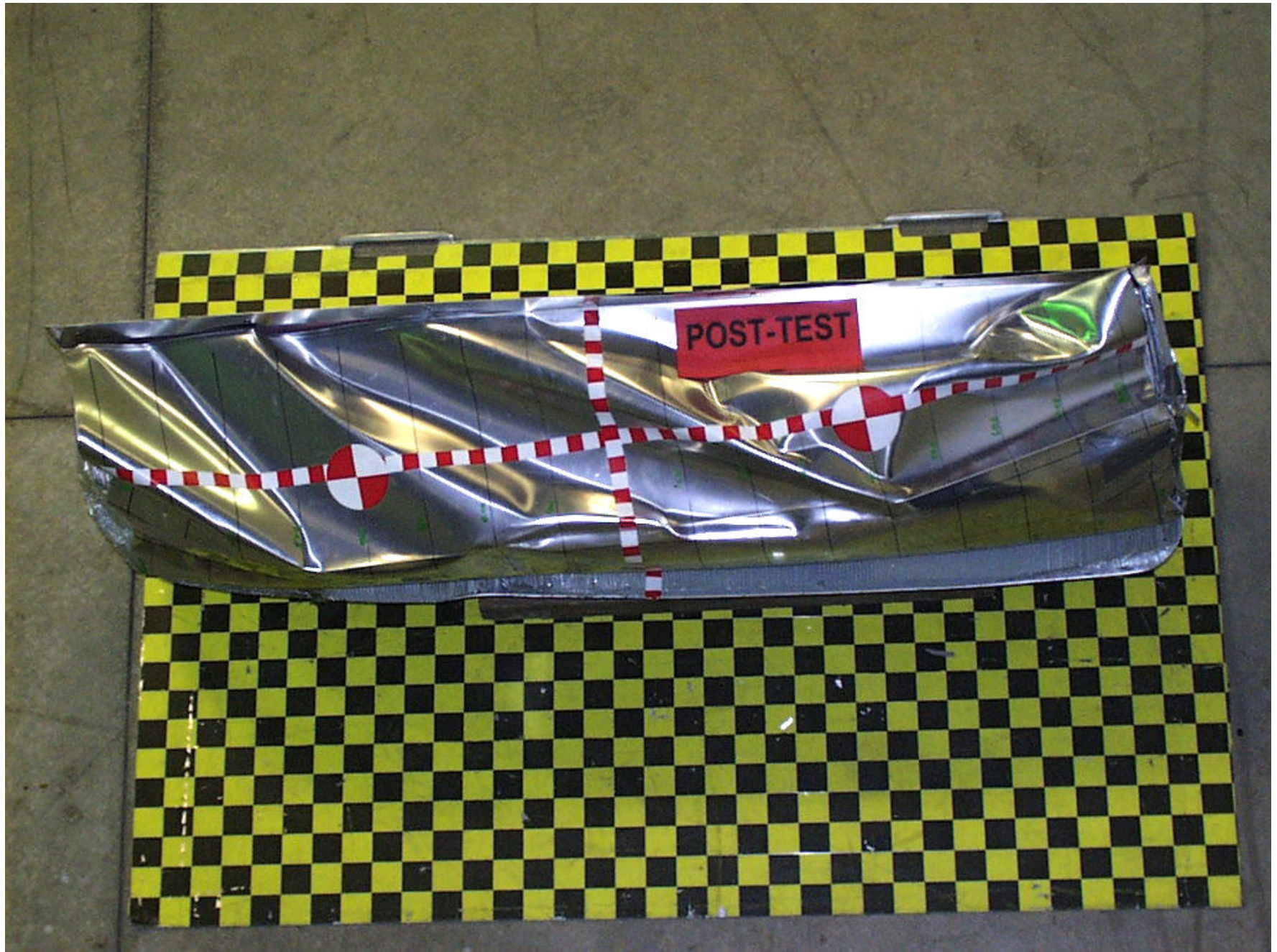
Figure A-52: POST-TEST ALUMINUM BARRIER OVERHEAD
