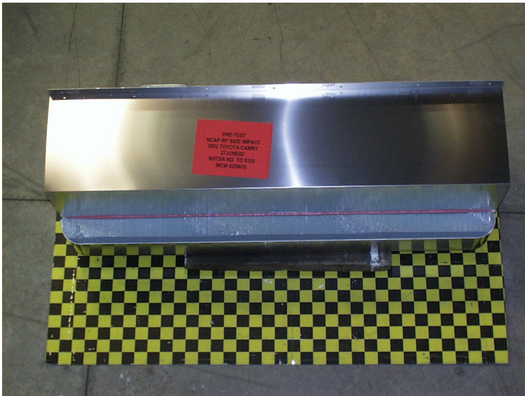
Figure A-51: PRE-TEST ALUMINUM BARRIER OVERHEAD
