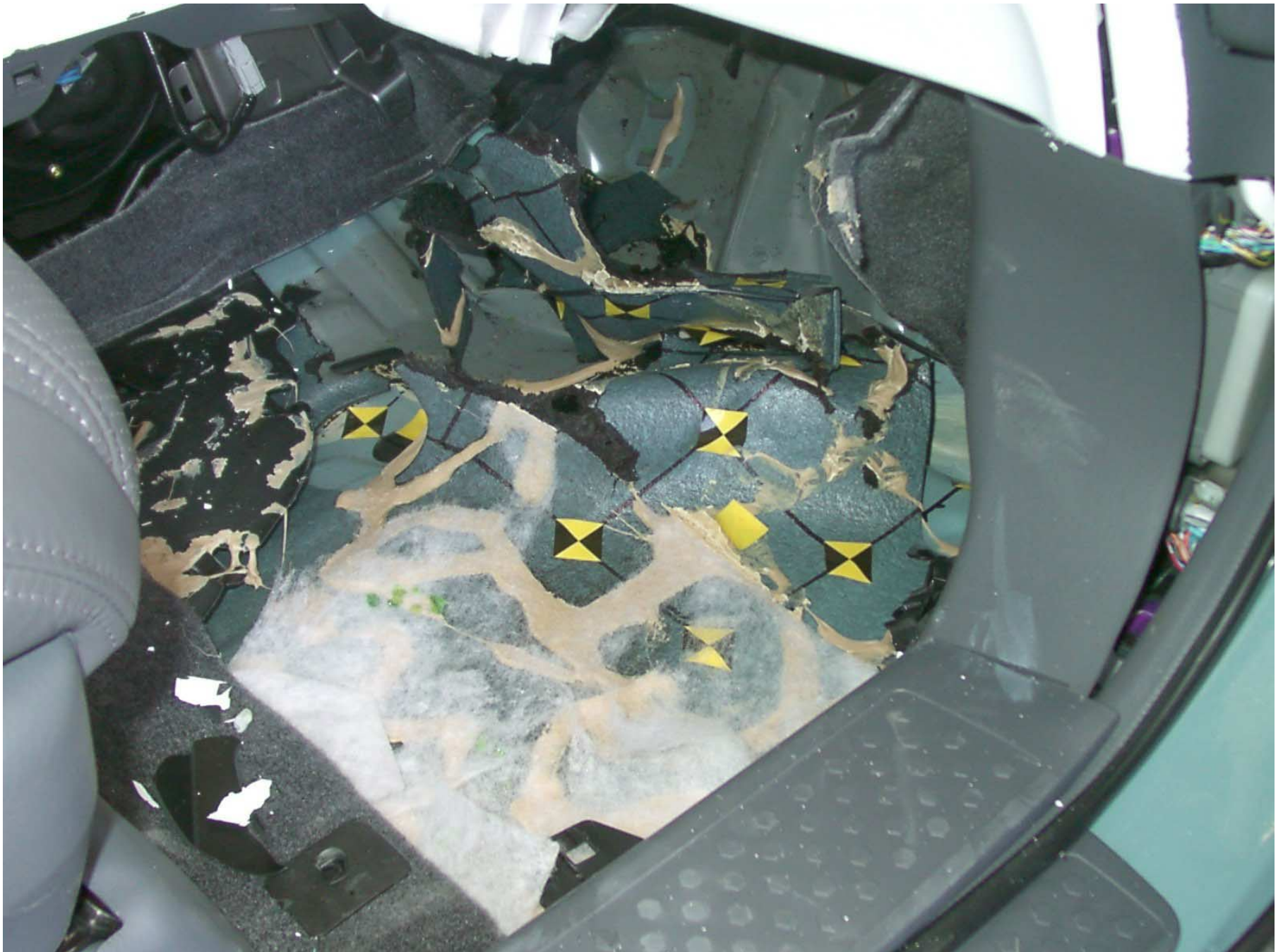
Figure A-52: Passenger Side Floor Pan, Post-Test
