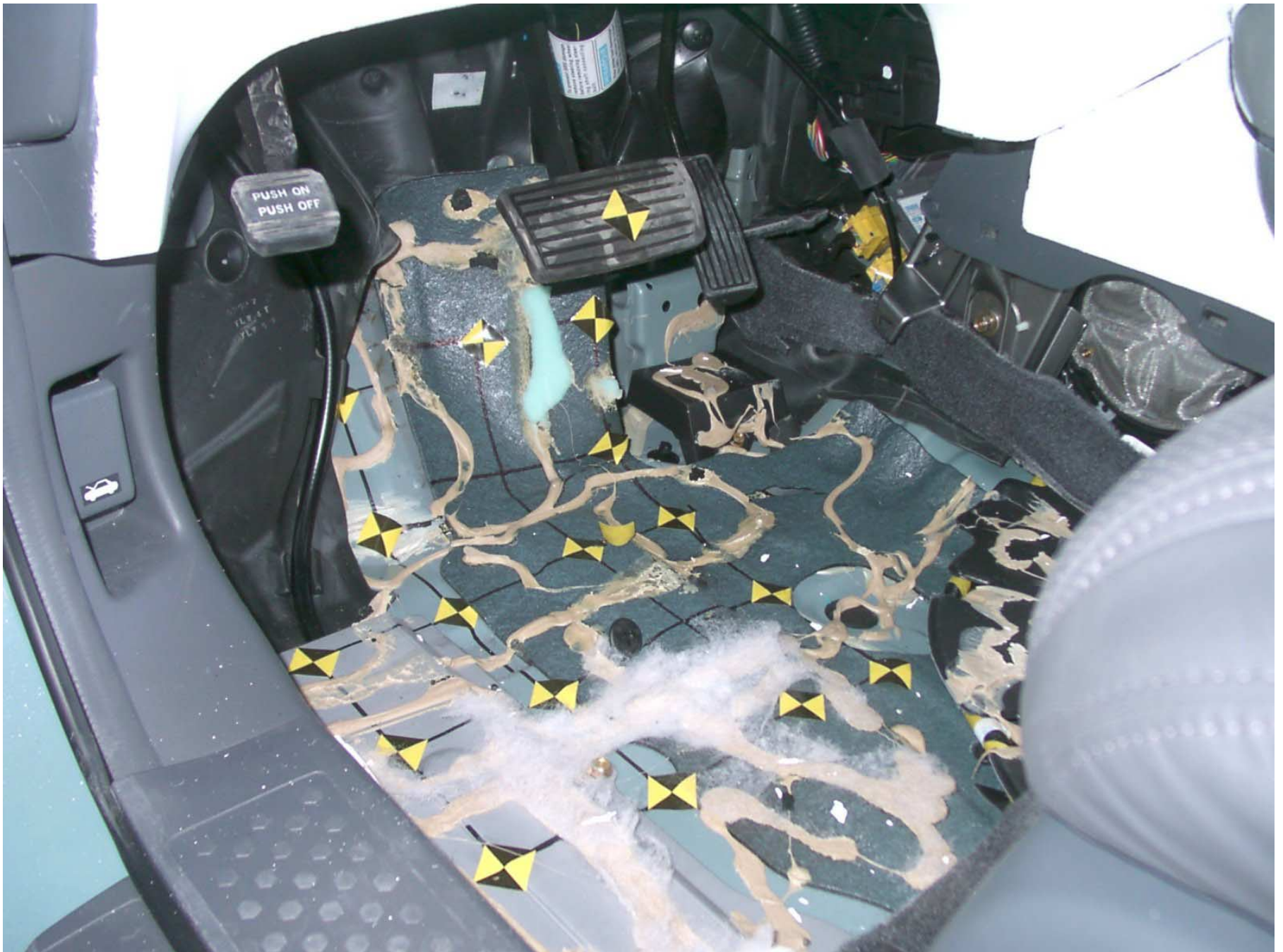
Figure A-38: Driver Side Floor Pan, Post-Test
