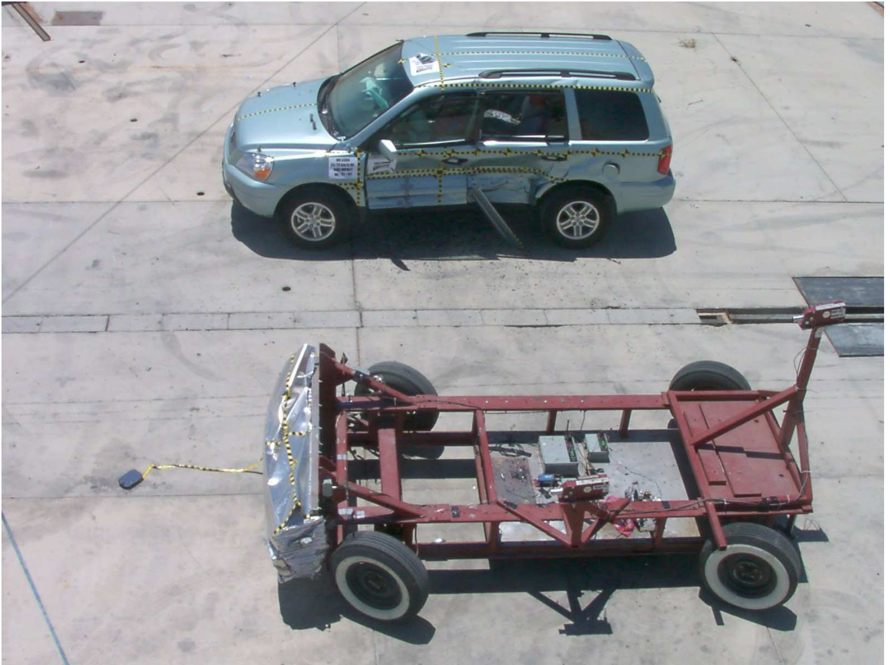
Figure A-16: Overhead Overall View, Post-Test
