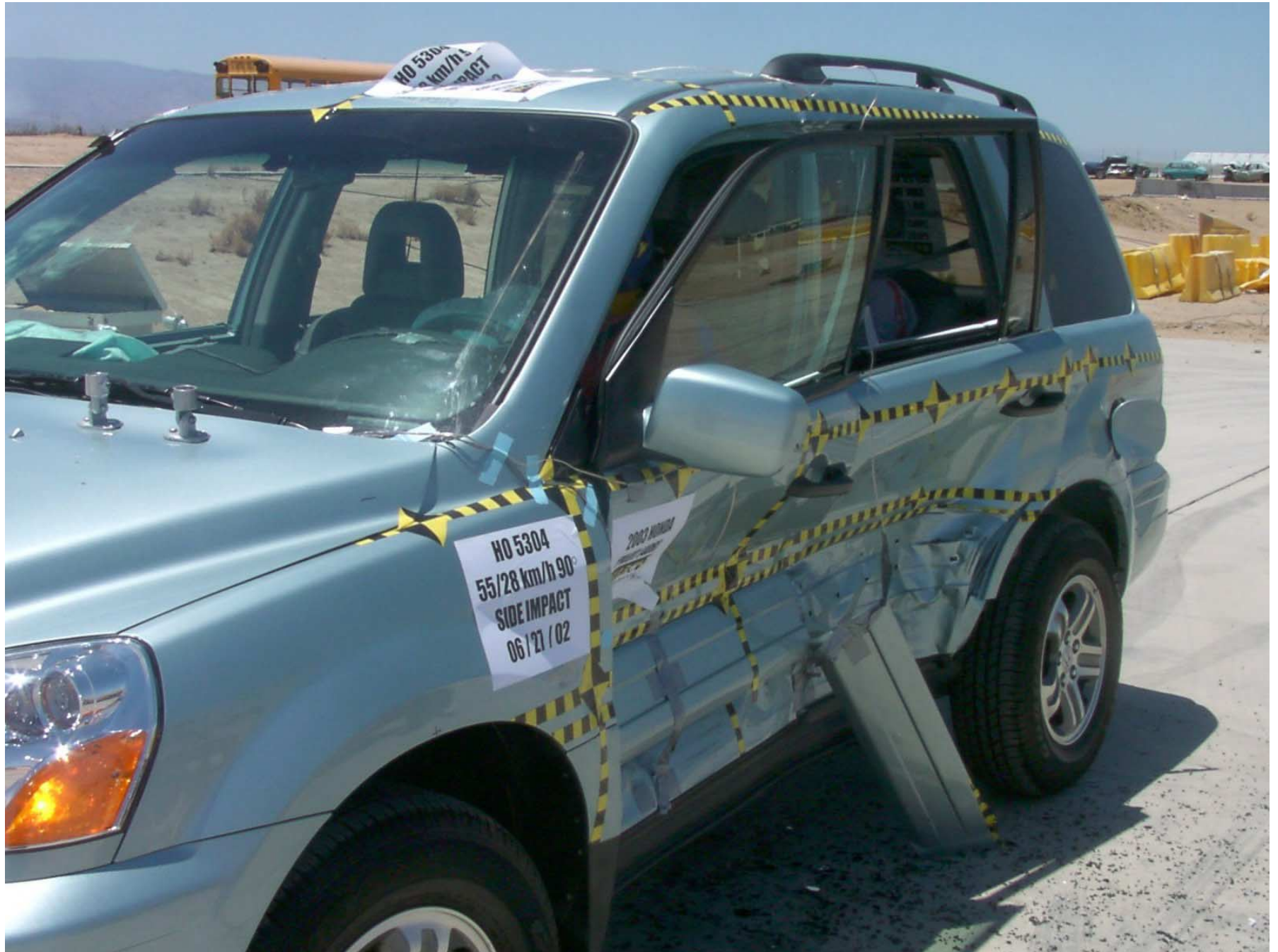
Figure A-21: Front \frac{3}{4} View of Left Side Doors, Post-Test
