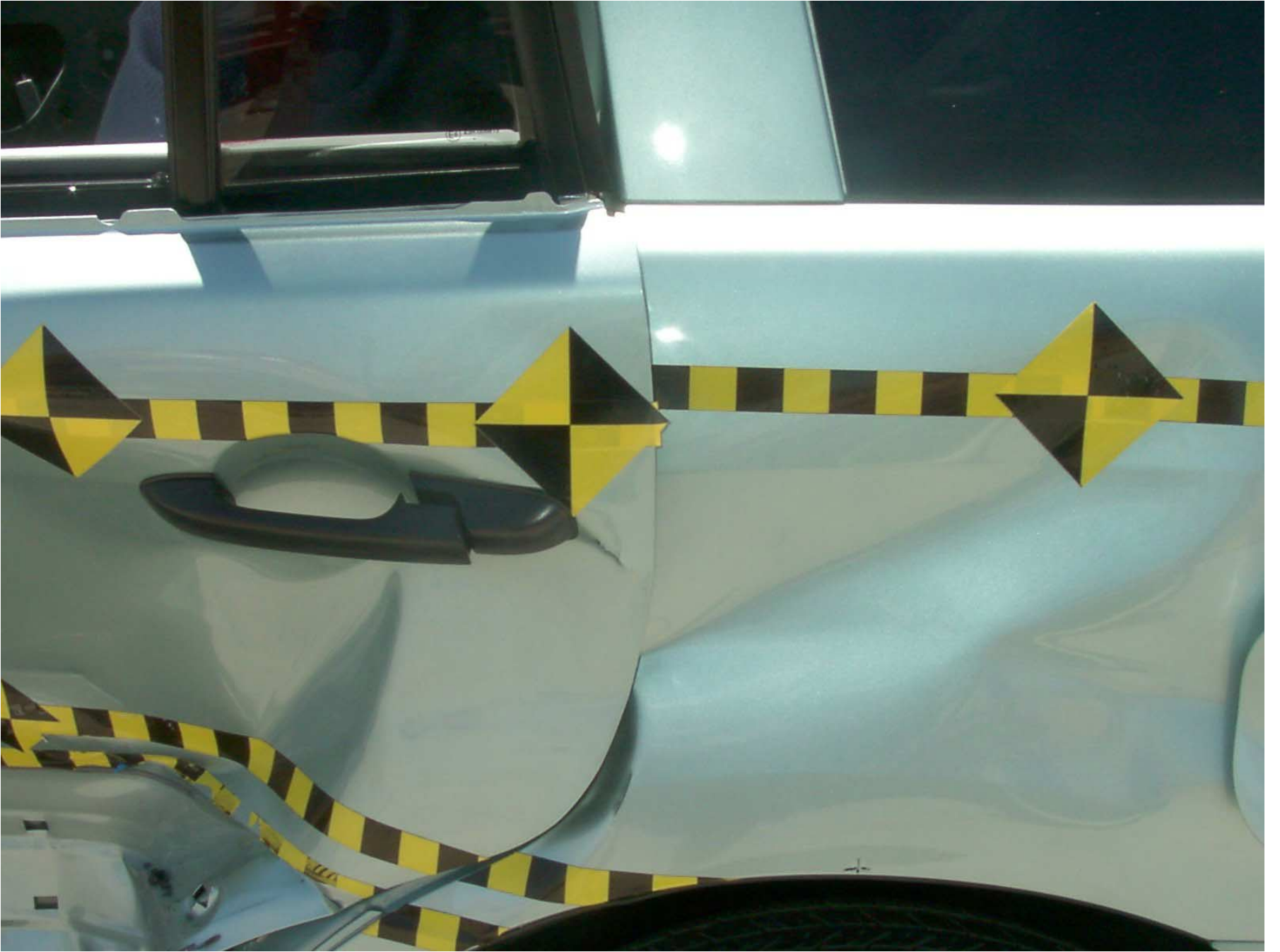
Figure A-24: Left Rear Door Closed, Post-Test
