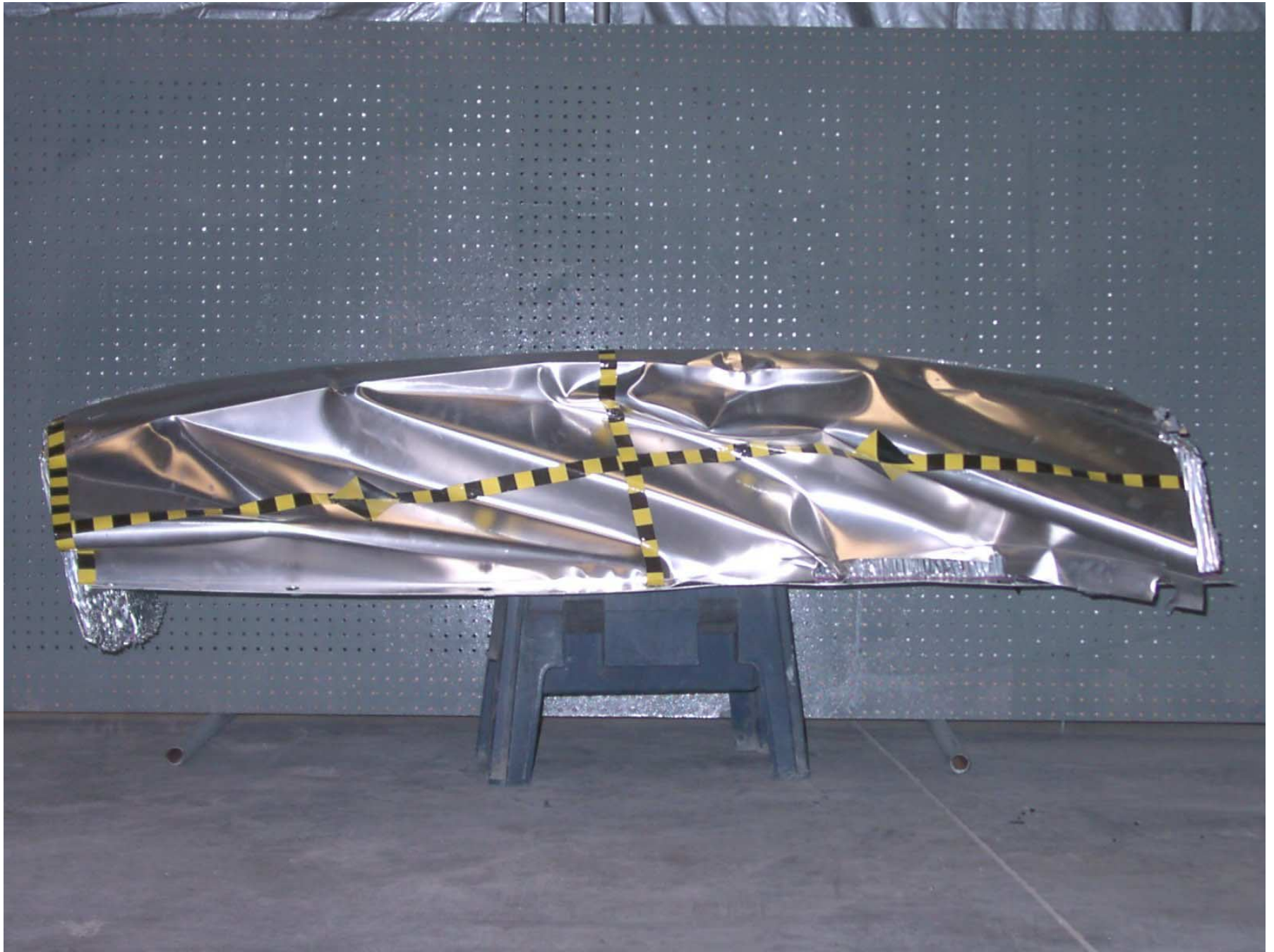
Figure A-46: Top View of Deformable Barrier, Post-Test
