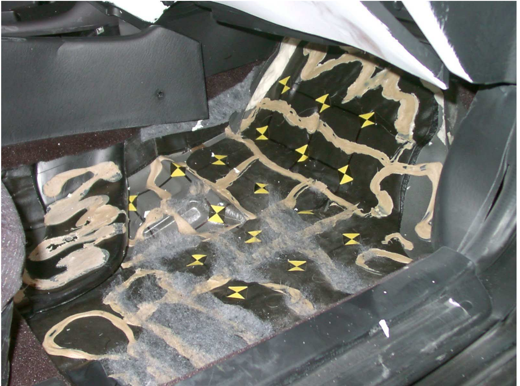
Figure A-52: Passenger Side Floor Pan, Post-Test
