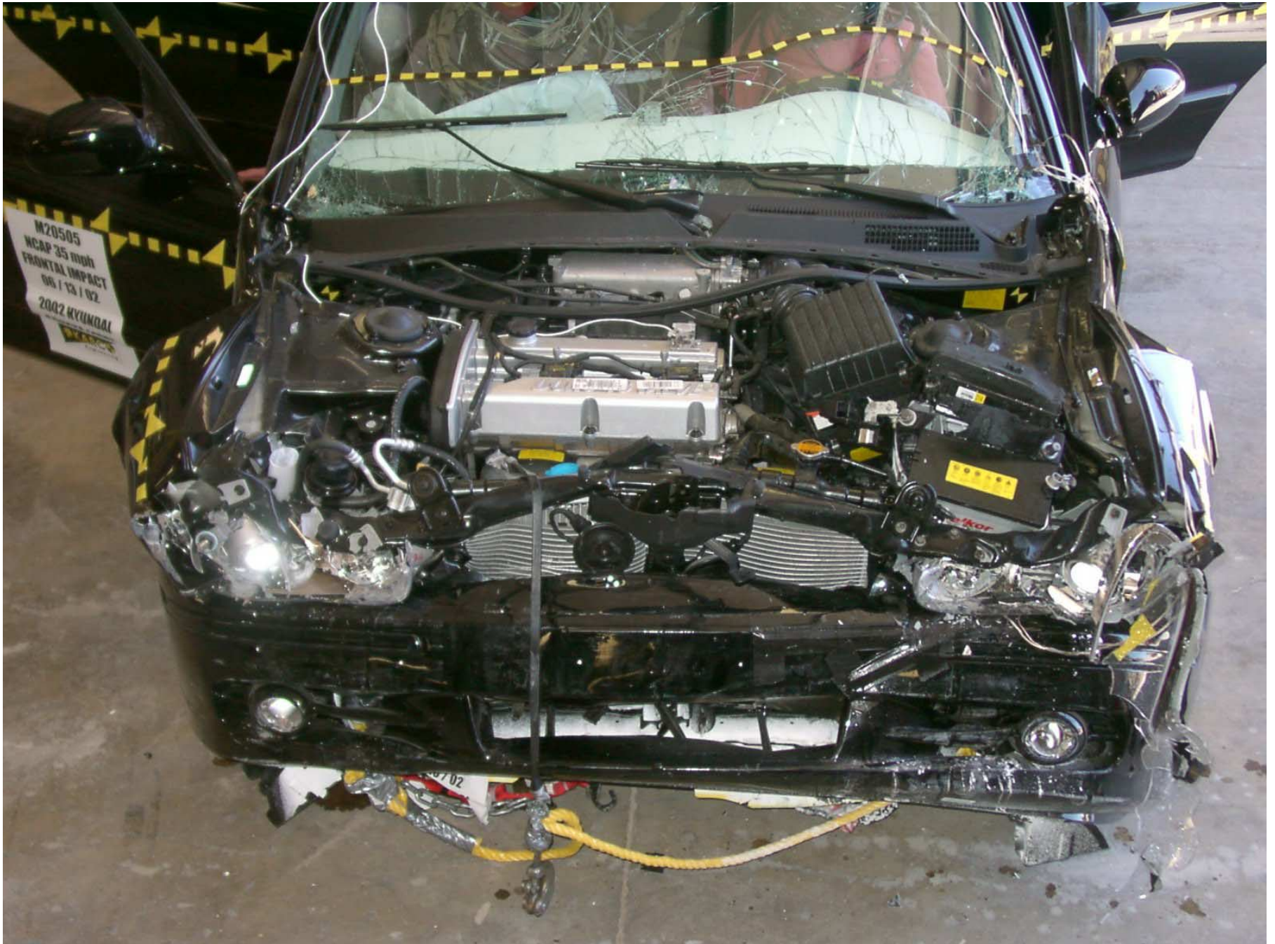
Figure A-18: Engine Compartment, Post-Test
