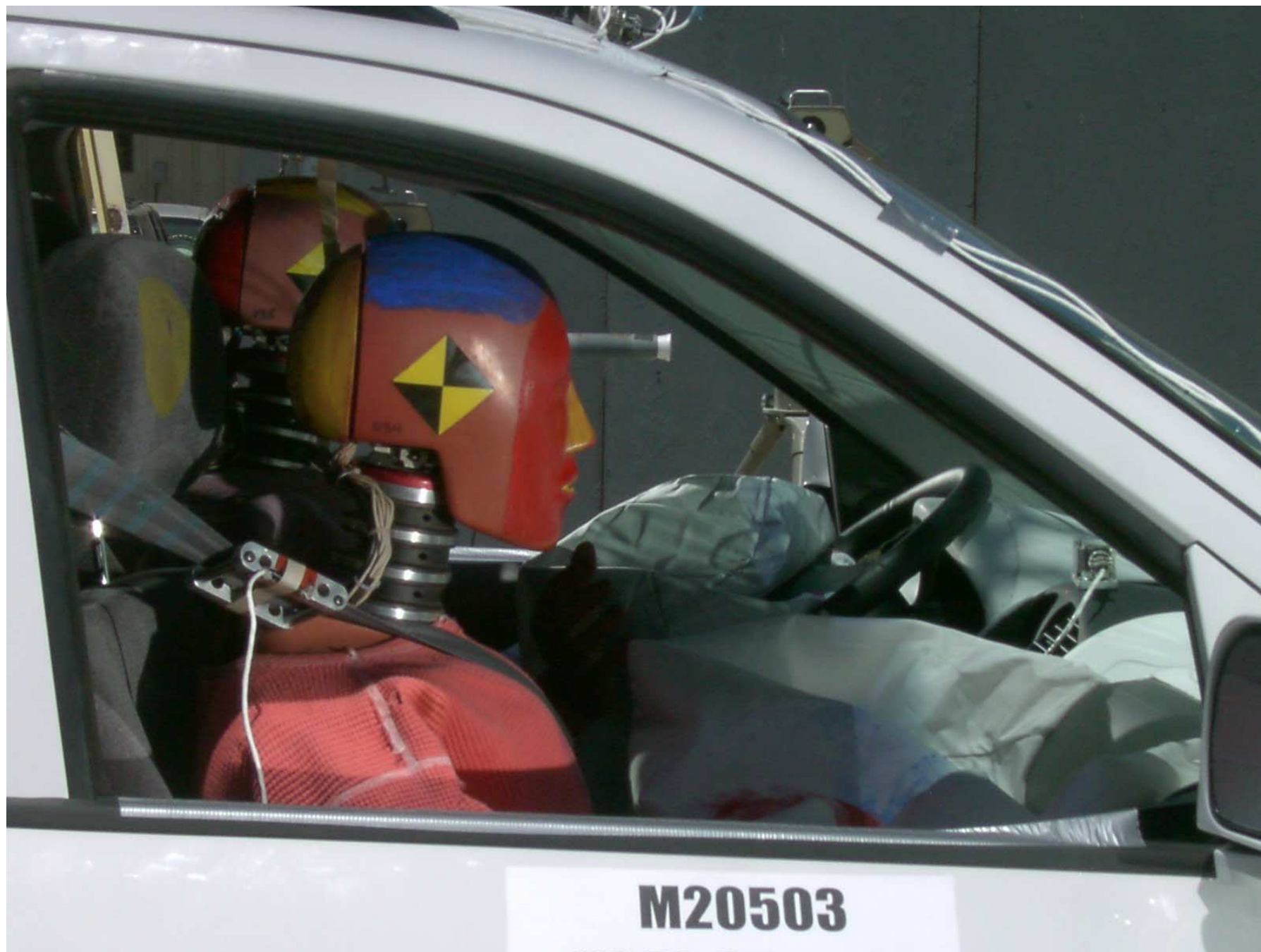
Figure A-44: Passenger Dummy Through Window, Post-Test
