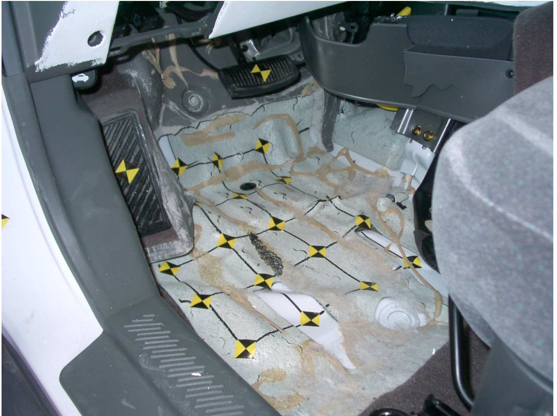
Figure A-38: Driver Side Floor Pan, Post-Test
