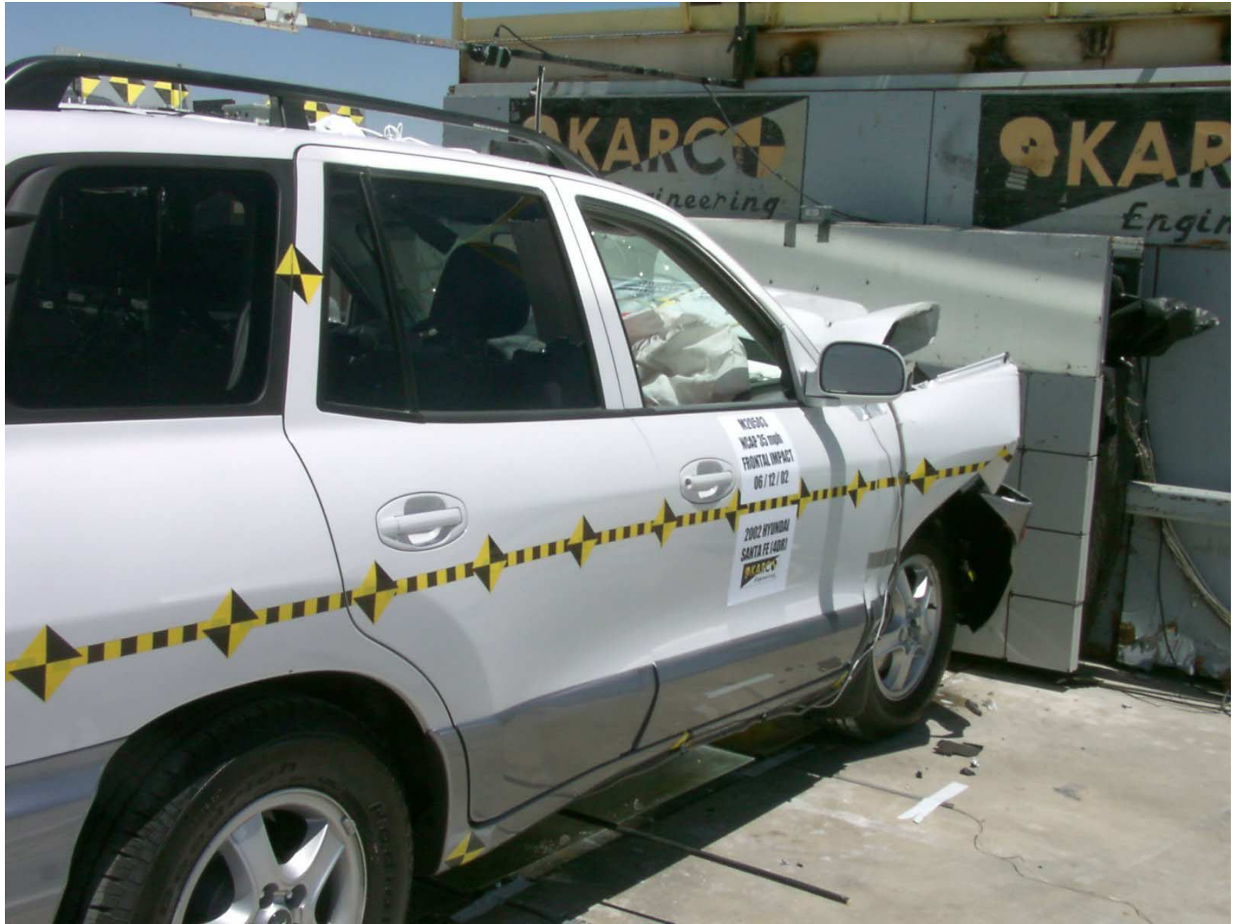
Figure A-58: 3/4 Right Rear View of Doors After Impact
