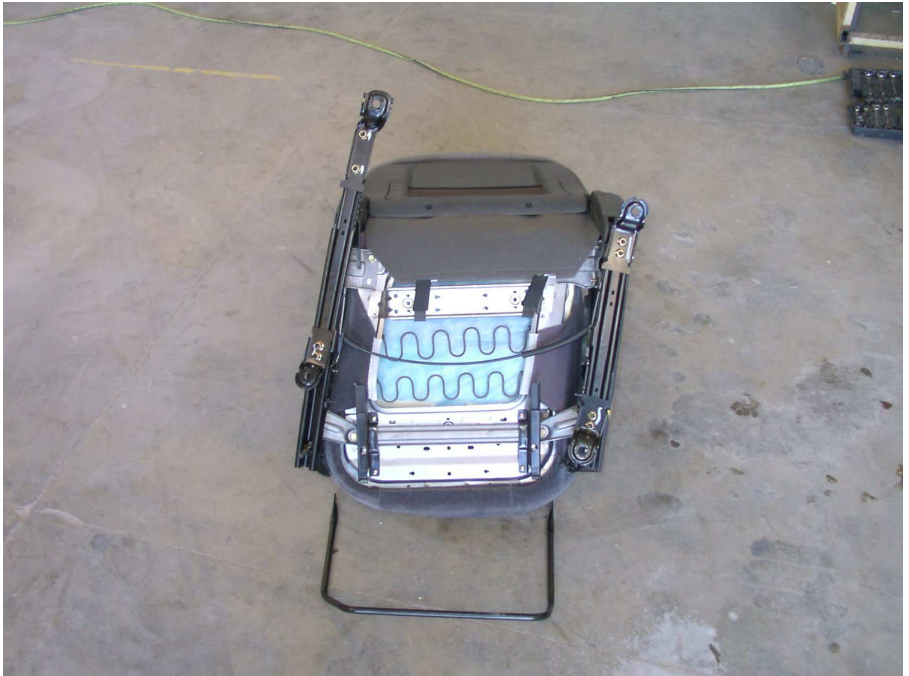
Figure A-62: Right Side Seat Track Damage, Post-Test
