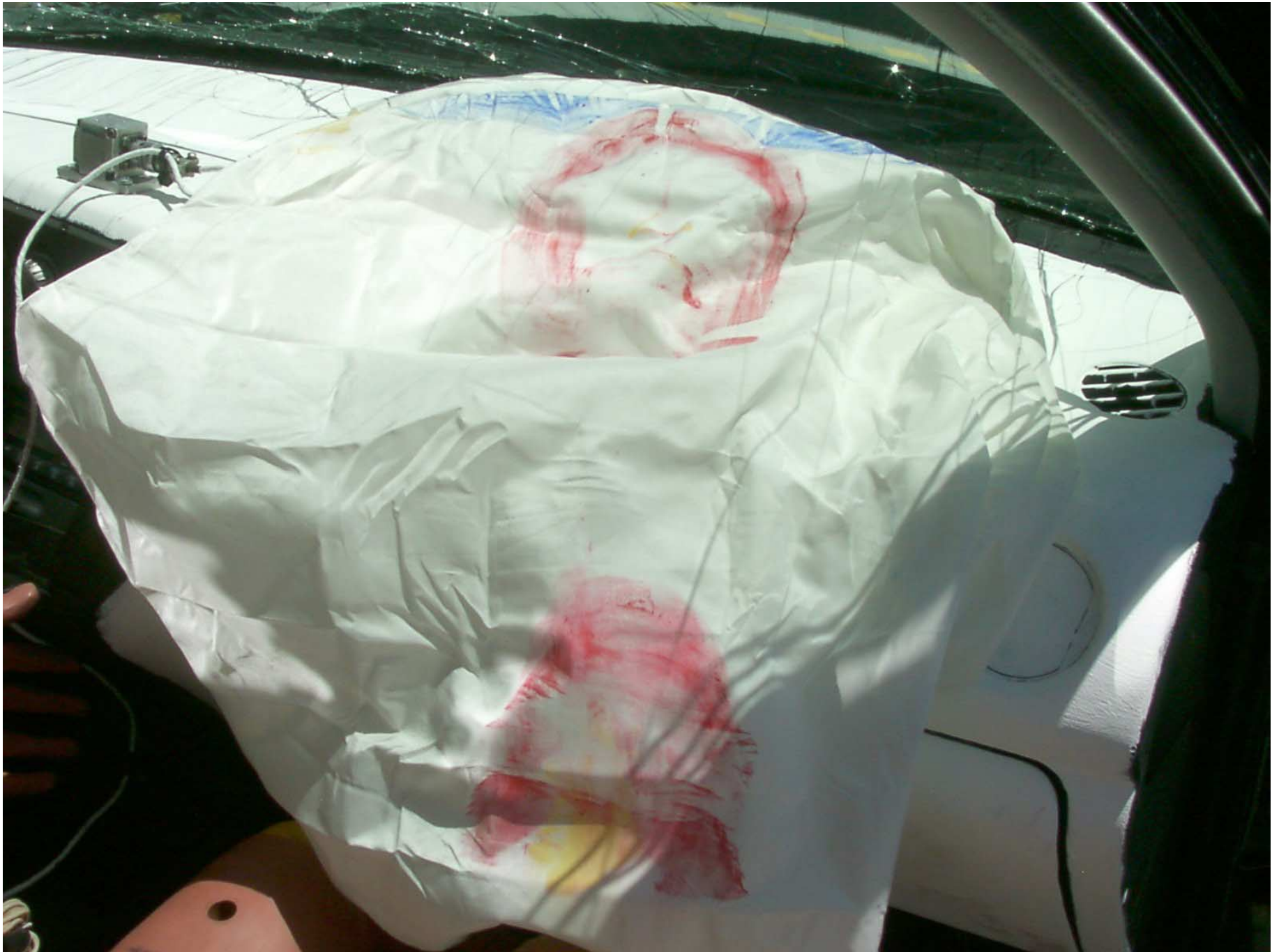
Figure A-56: Passenger Dummy Contact, Post-Test
