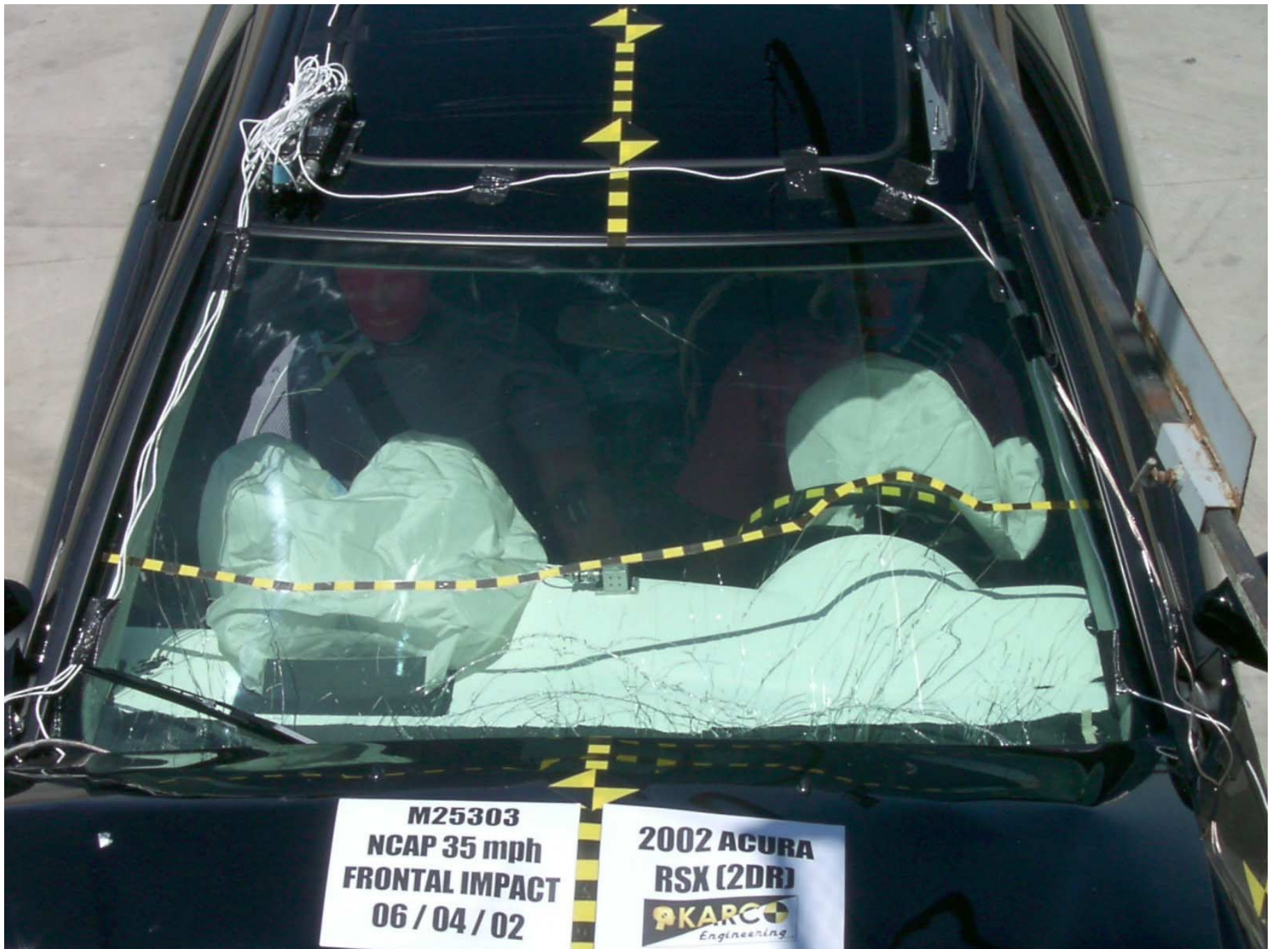
Figure A-16: Windshield, Post-Test
