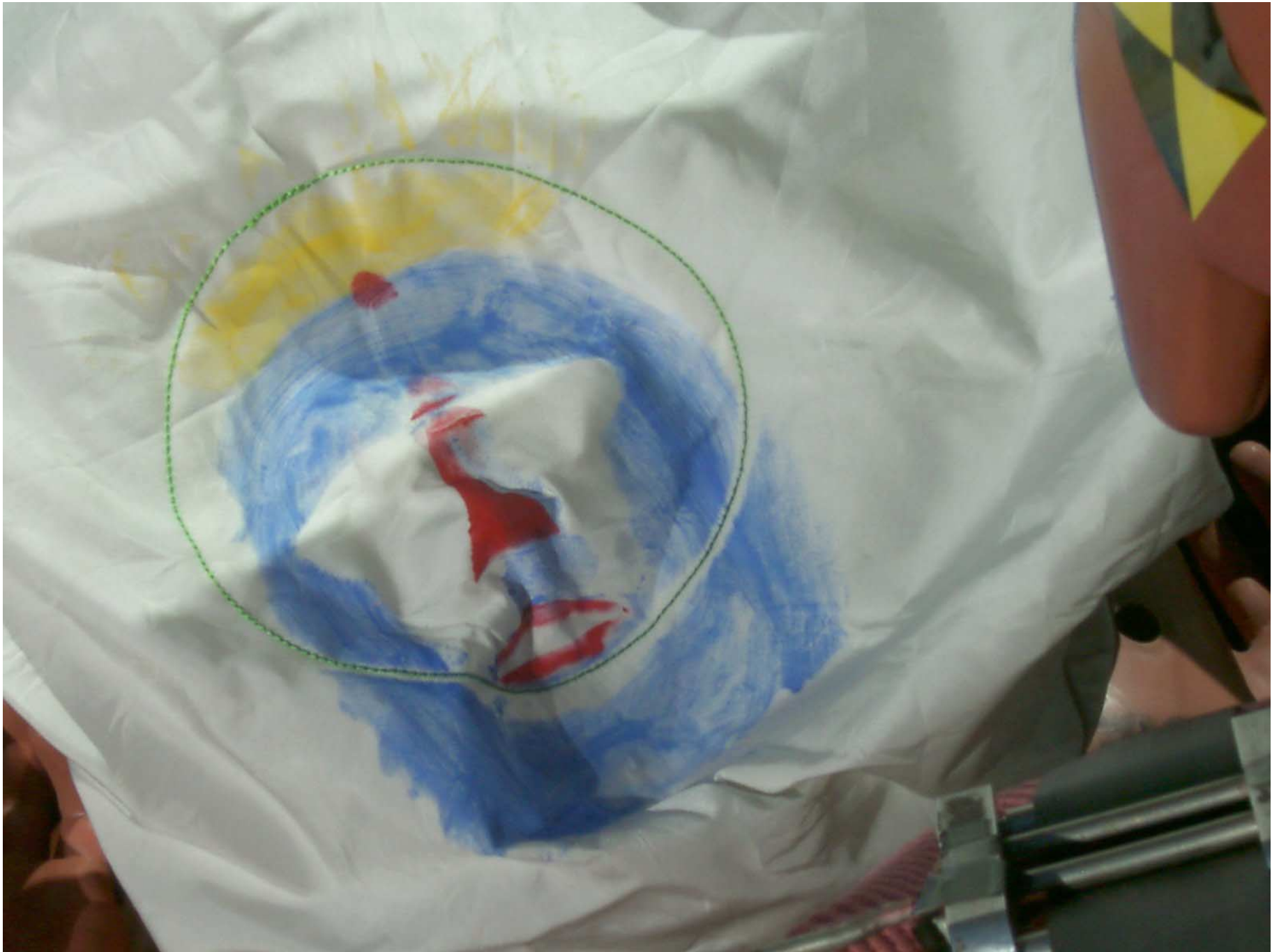
Figure A-40: Driver Dummy Contact, Post-Test
