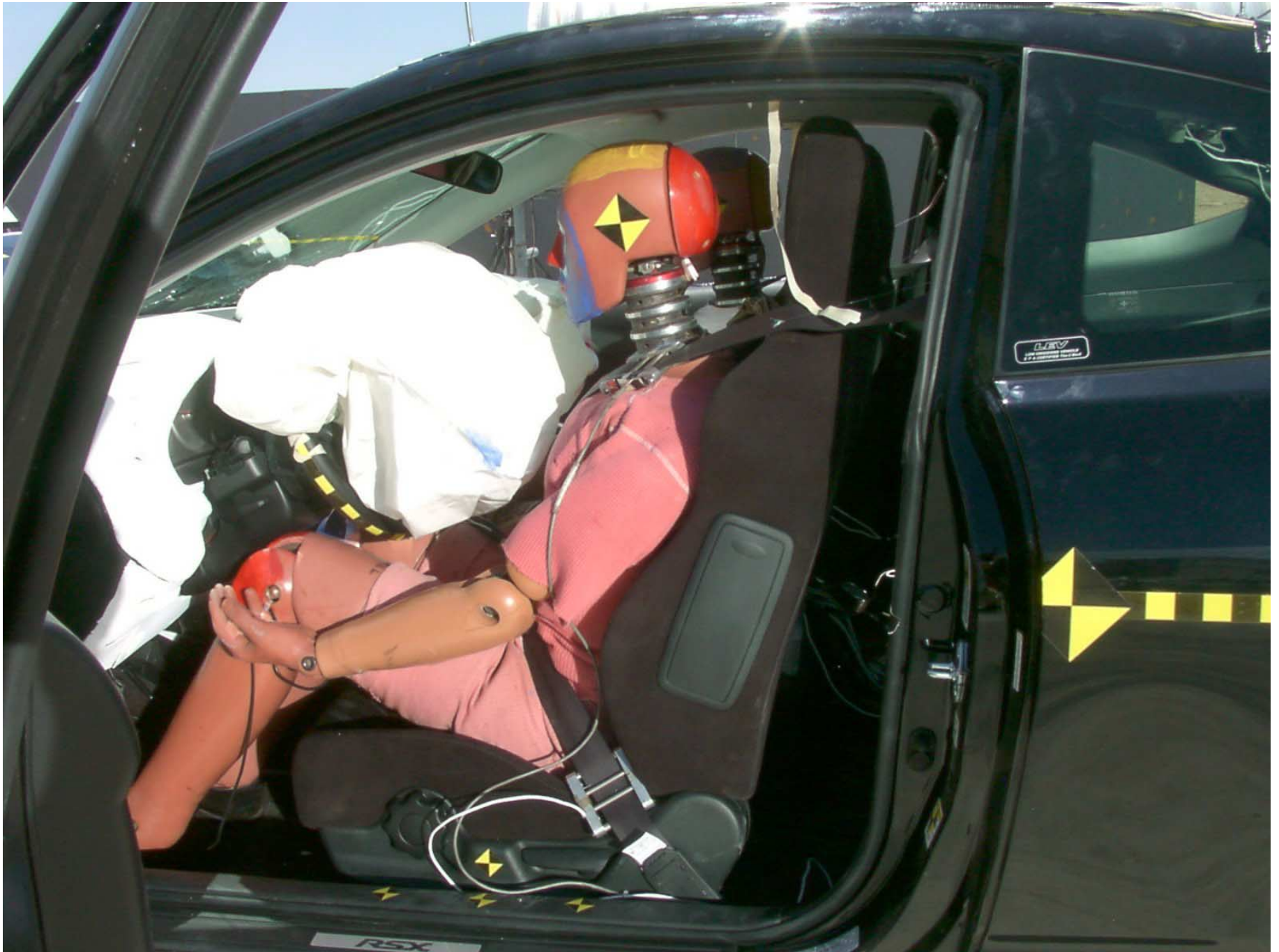
Figure A-32: Driver Dummy 90° To Vehicle, Post-Test
