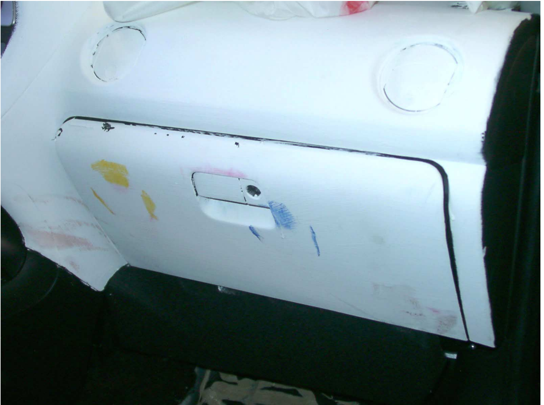
Figure A-54: Passenger Side Knee Bolster, Post-Test
