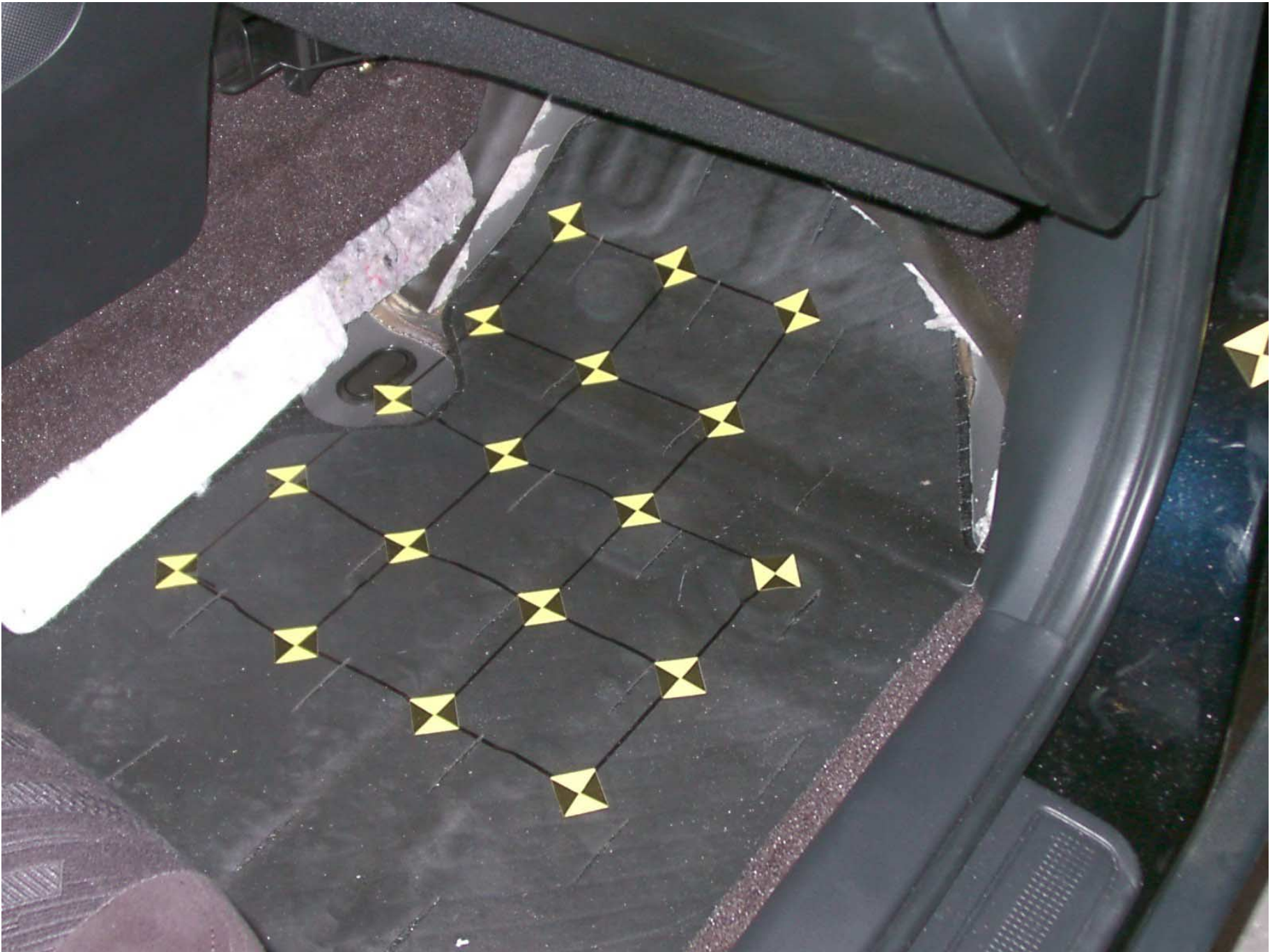
Figure A-51: Passenger Side Floor Pan, Pre-Test
