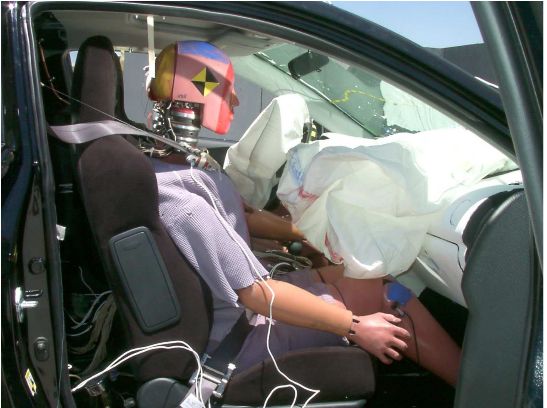
Figure A-48: Passenger Dummy 90° To Vehicle, Post-Test
