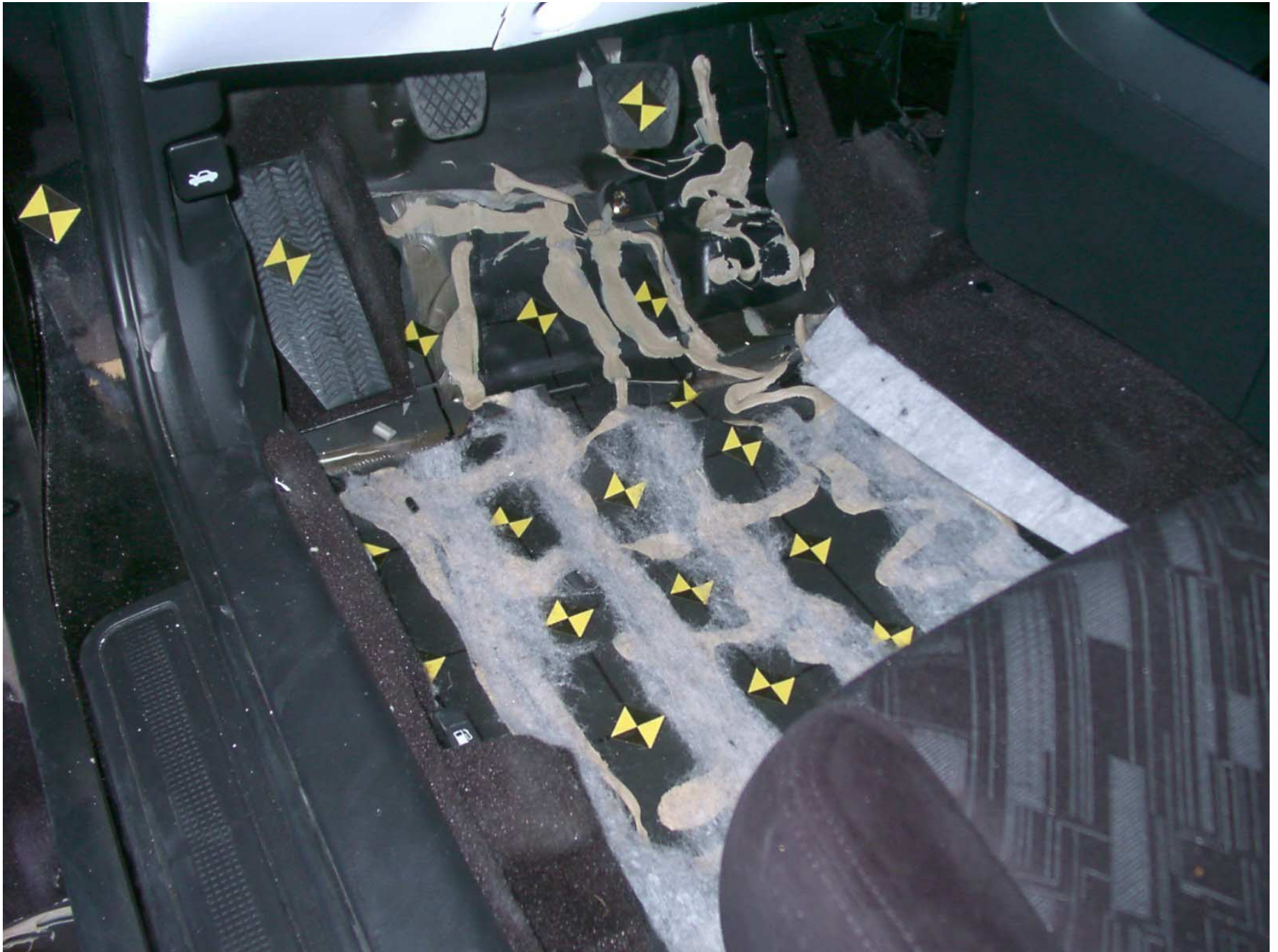
Figure A-38: Driver Side Floor Pan, Post-Test
