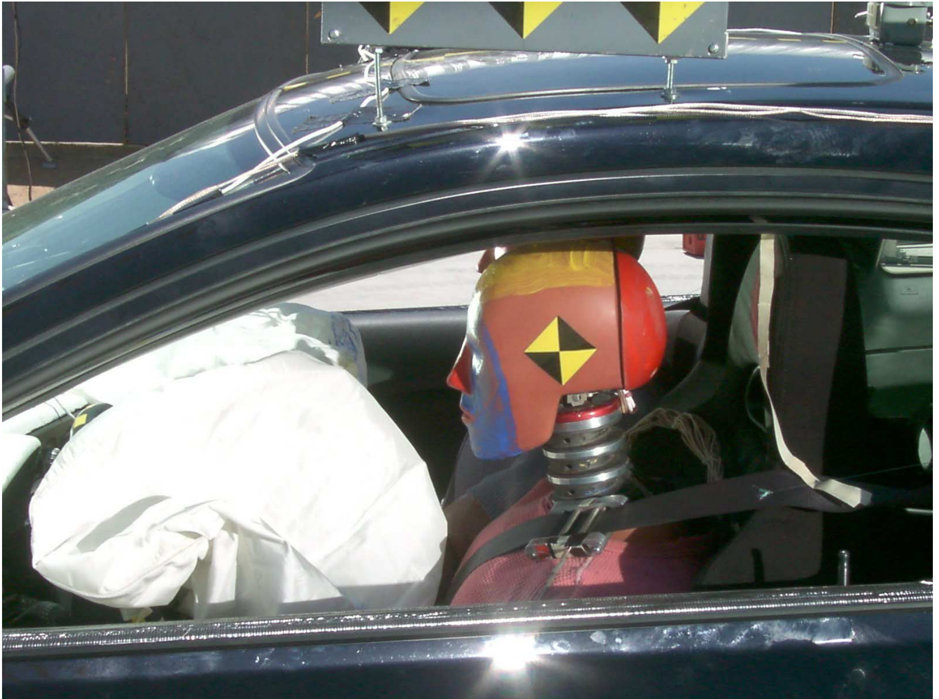
Figure A-28: Driver Dummy Through Window, Post-Test
