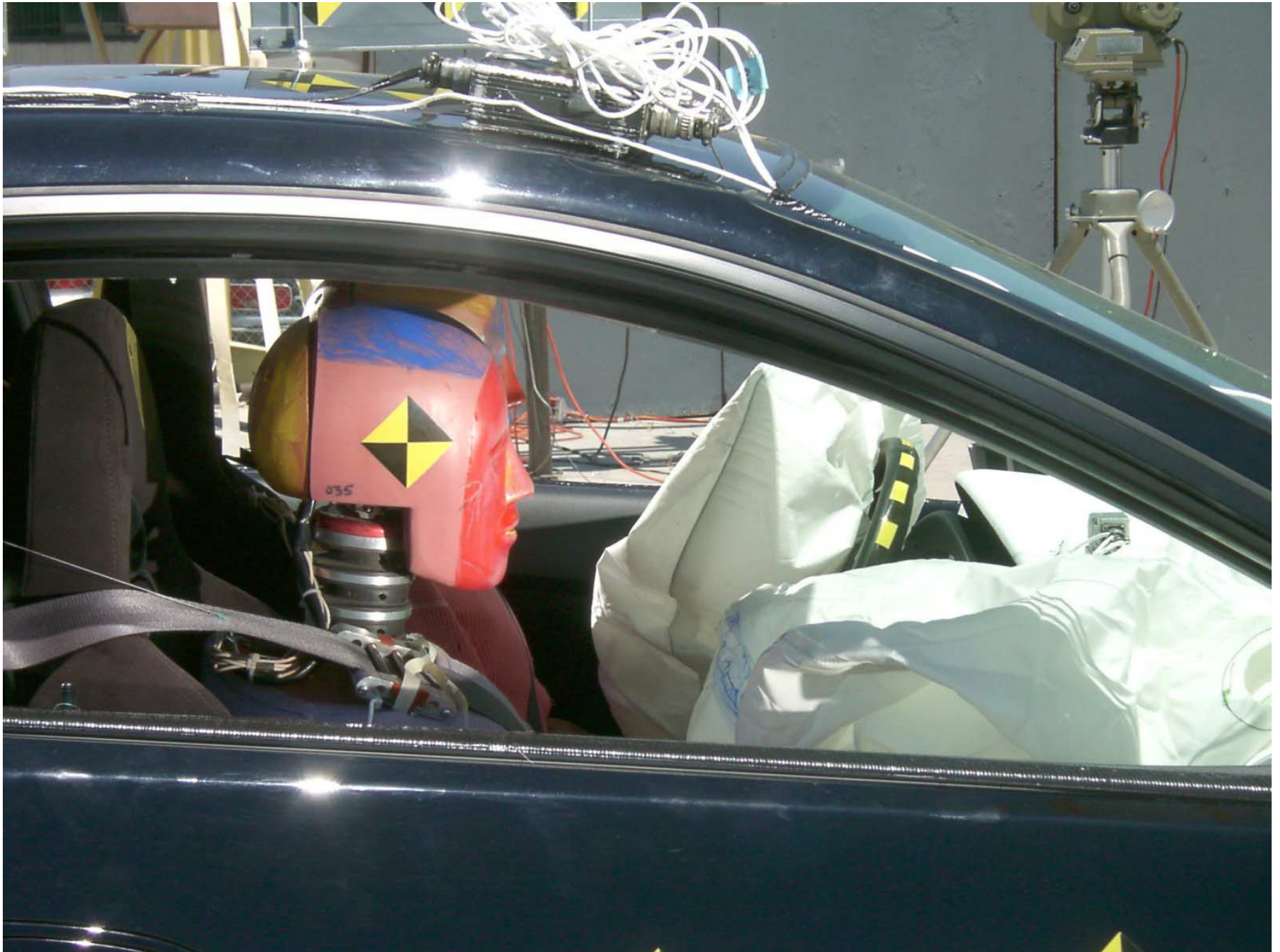
Figure A-44: Passenger Dummy Through Window, Post-Test
