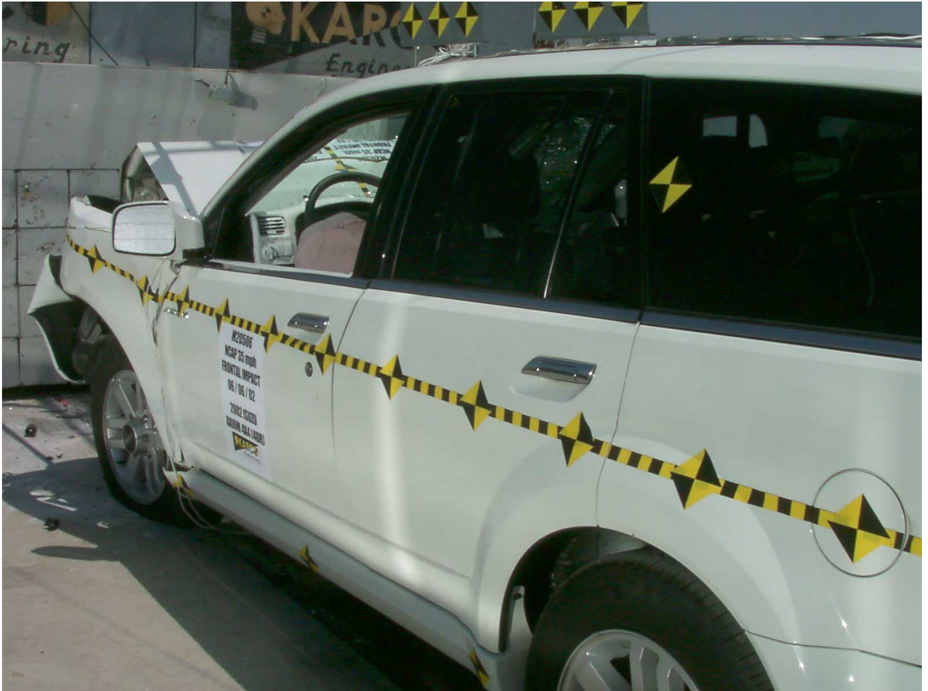
Figure A-57: Left Rear View of Doors After Impact
