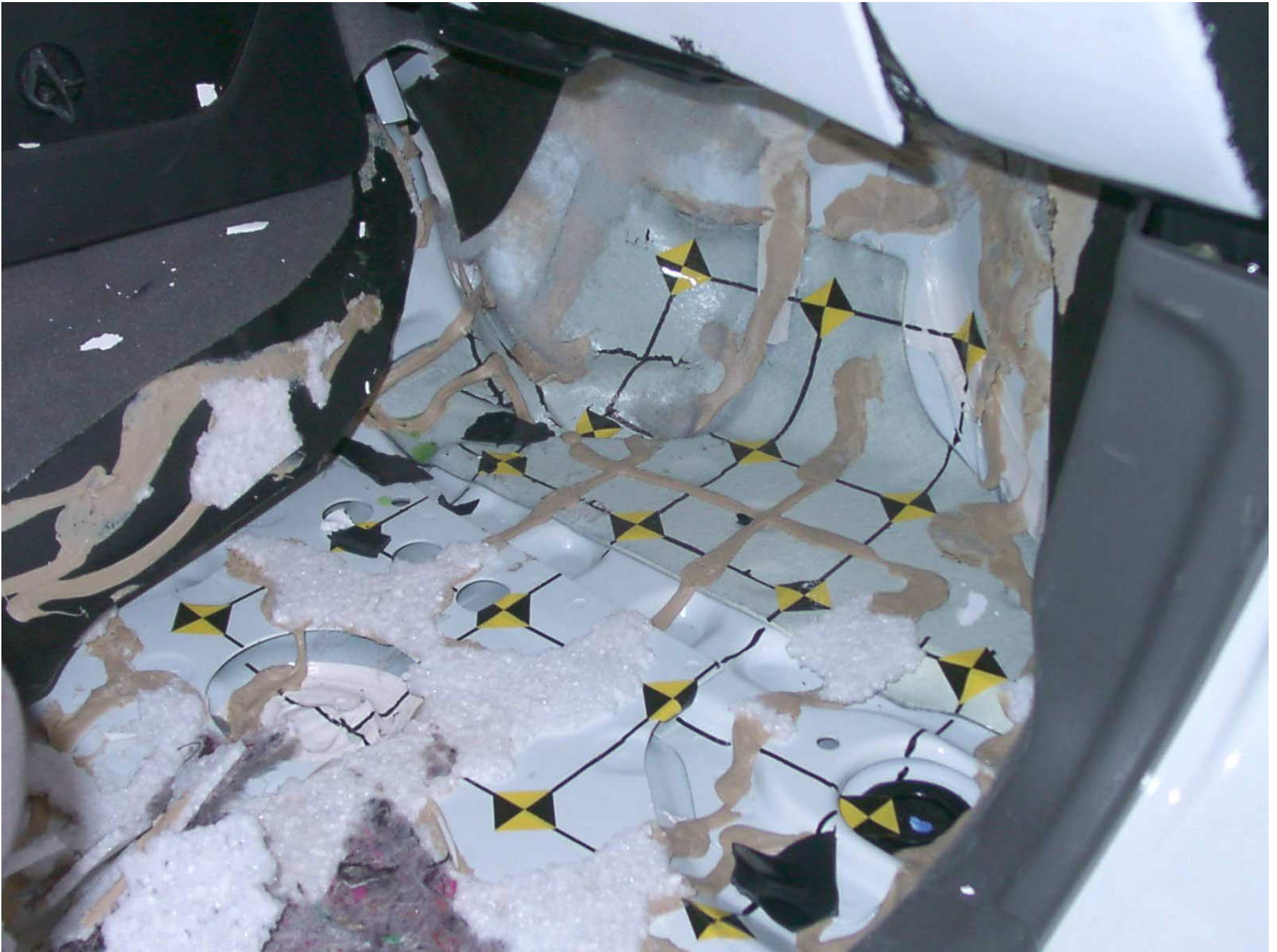
Figure A-52: Passenger Side Floor Pan, Post-Test
