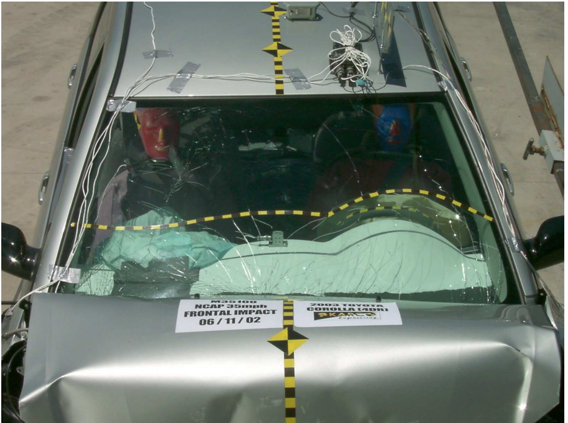
Figure A-16: Windshield, Post-Test
