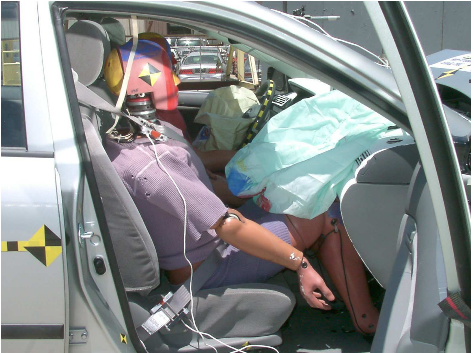
Figure A-48: Passenger Dummy 90° To Vehicle, Post-Test
