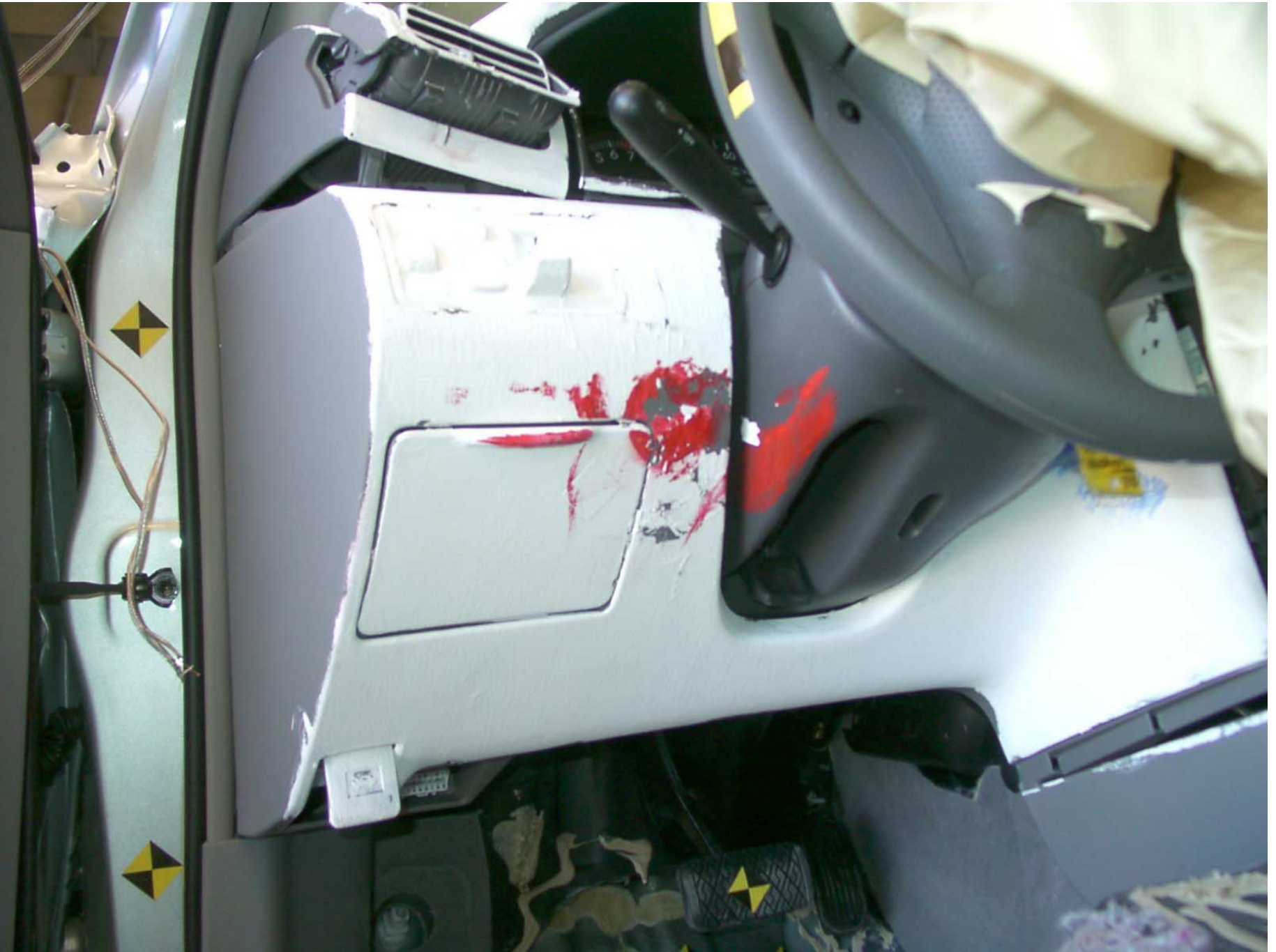
Figure A-36: Driver Side Knee Bolster, Post-Test
