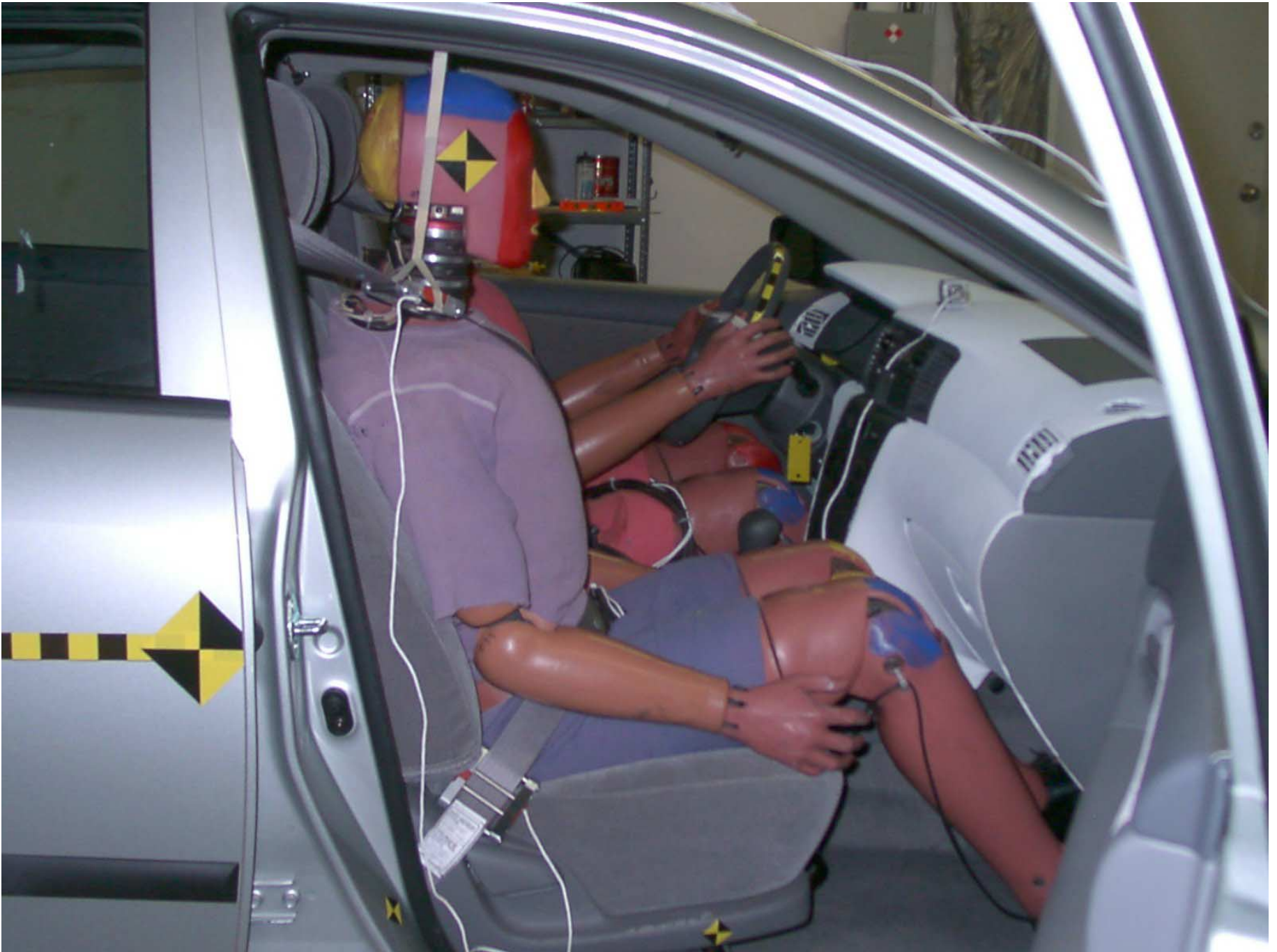
Figure A-47: Passenger Dummy 90° To Vehicle, Pre-Test
