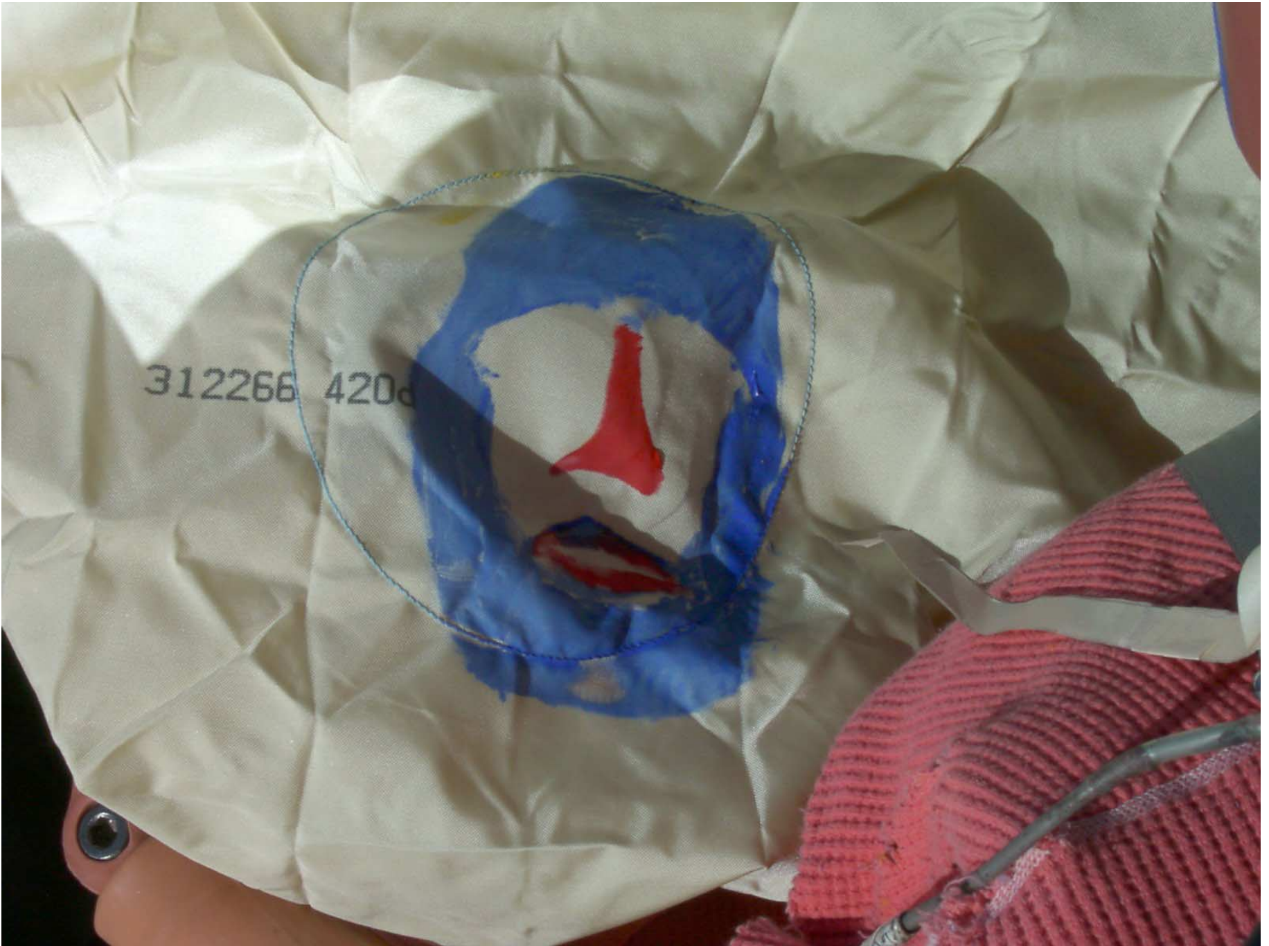
Figure A-40: Driver Dummy Contact, Post-Test
