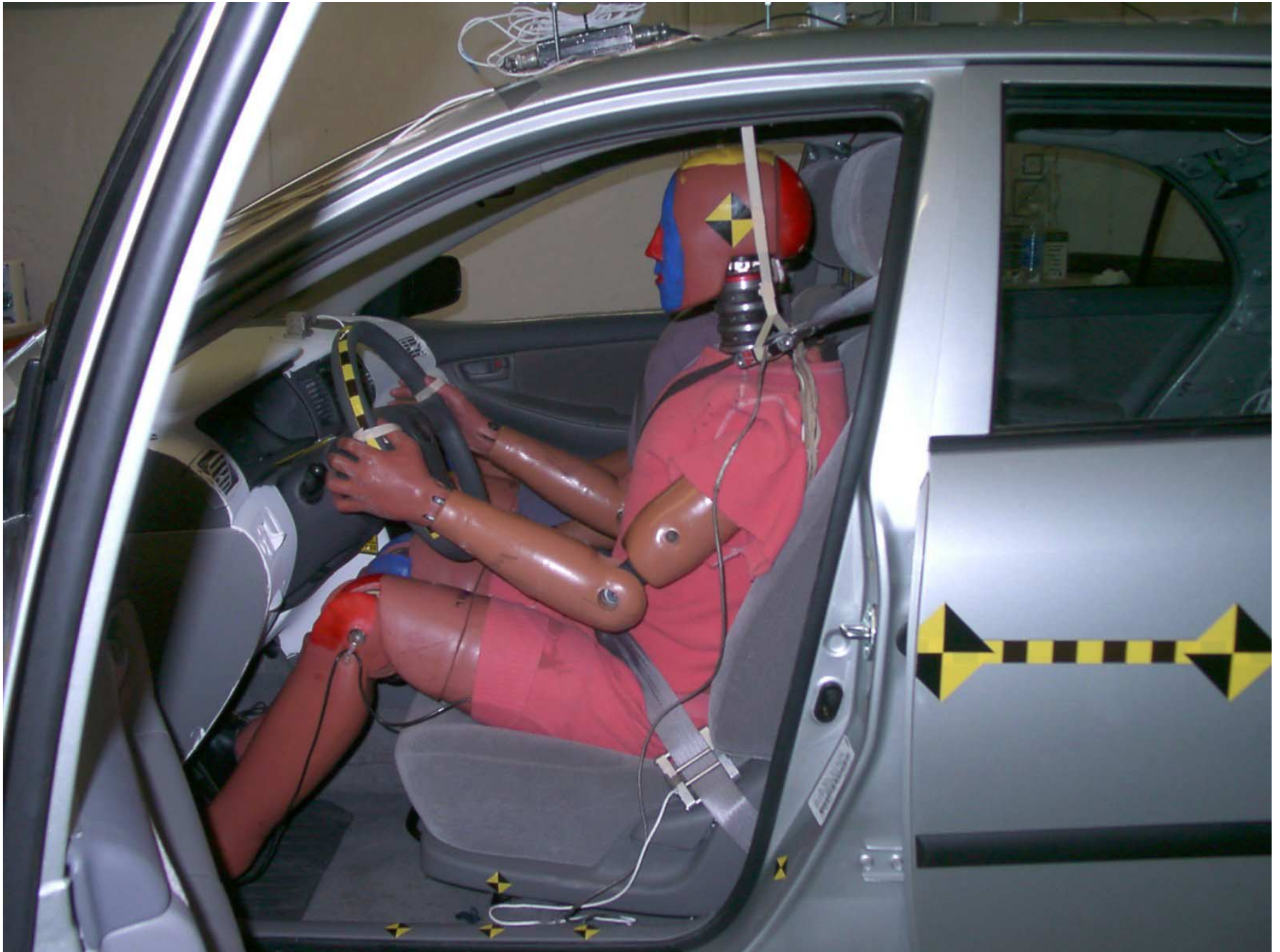
Figure A-31: Driver Dummy 90° To Vehicle, Pre-Test
