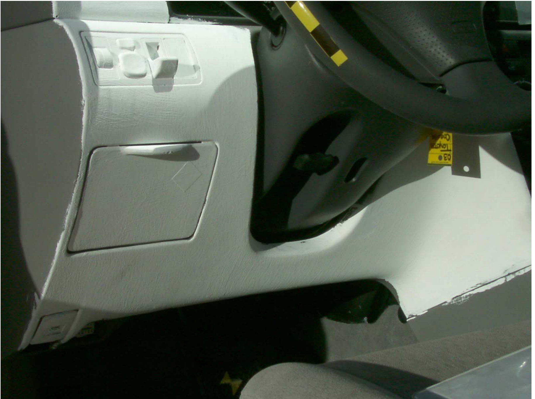
Figure A-35: Driver Side Knee Bolster, Pre-Test
