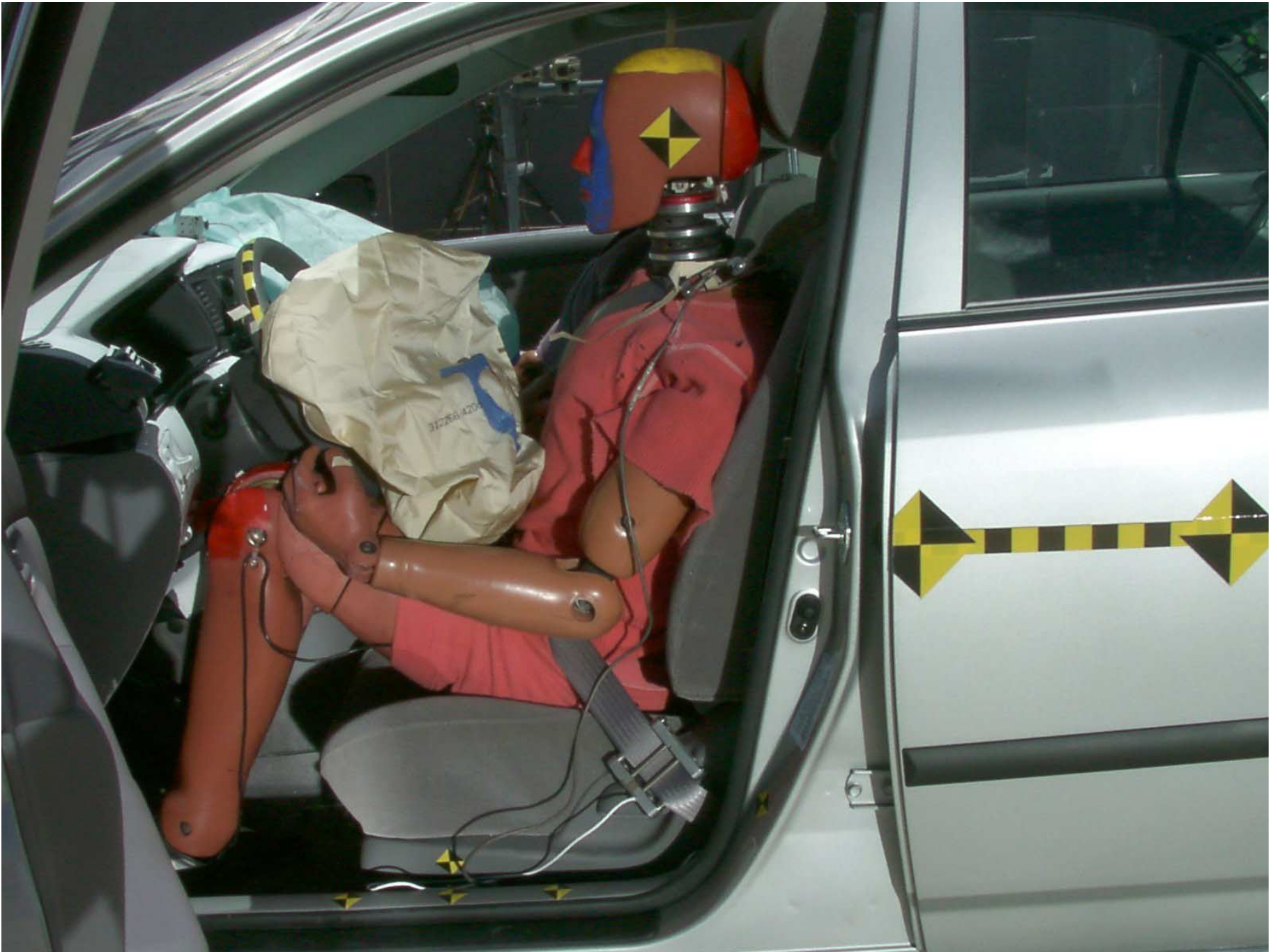
Figure A-32: Driver Dummy 90° To Vehicle, Post-Test
