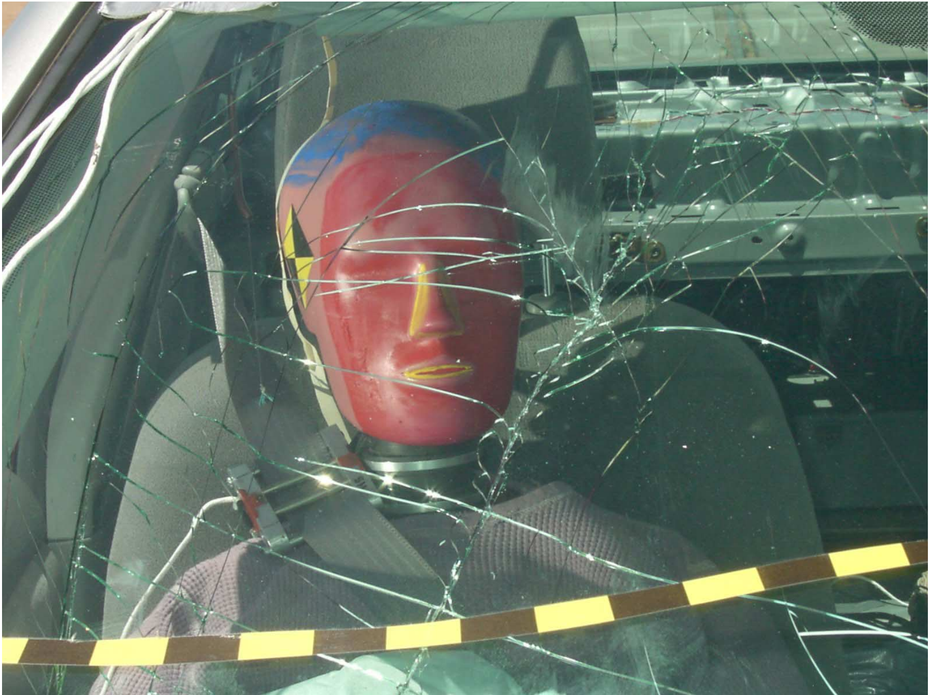
Figure A-42: Passenger Dummy Front View, Post-Test
