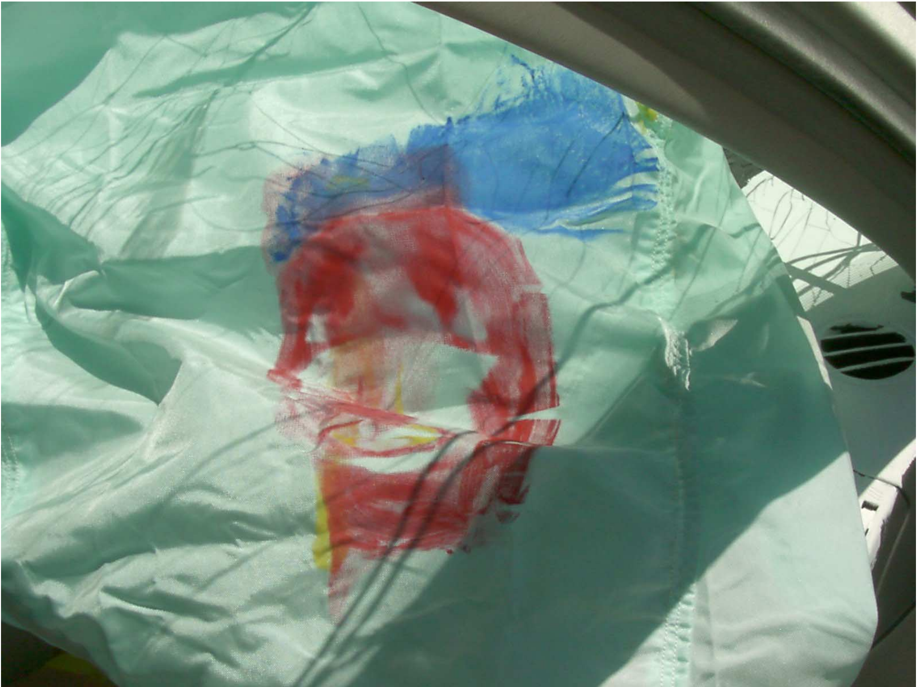
Figure A-56: Passenger Dummy Contact, Post-Test
