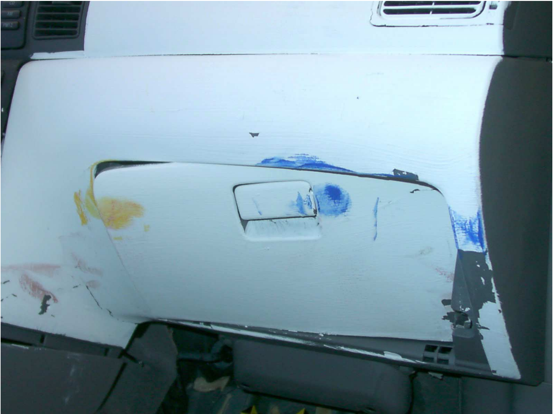
Figure A-54: Passenger Side Knee Bolster, Post-Test
