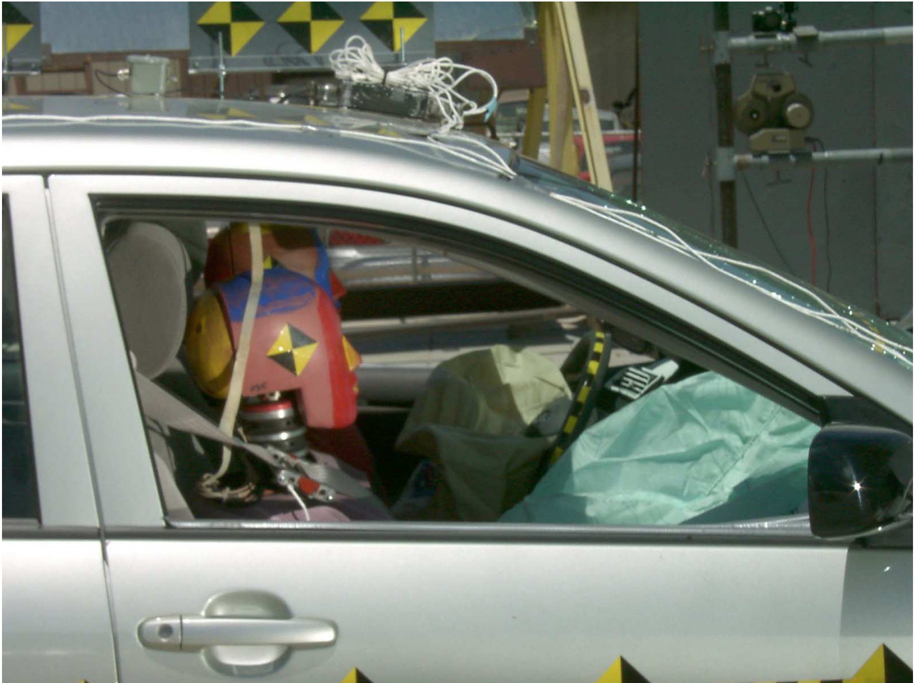
Figure A-44: Passenger Dummy Through Window, Post-Test
