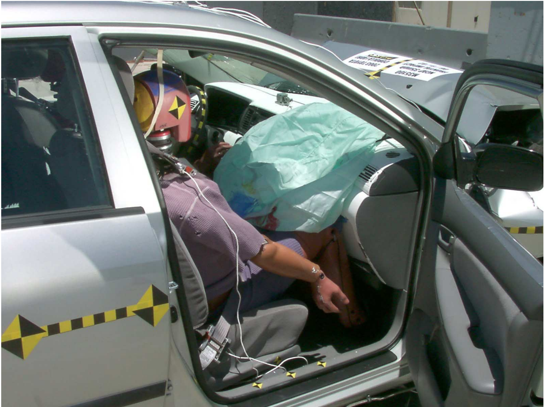
Figure A-46: Passenger Dummy Door Open, Post-Test
