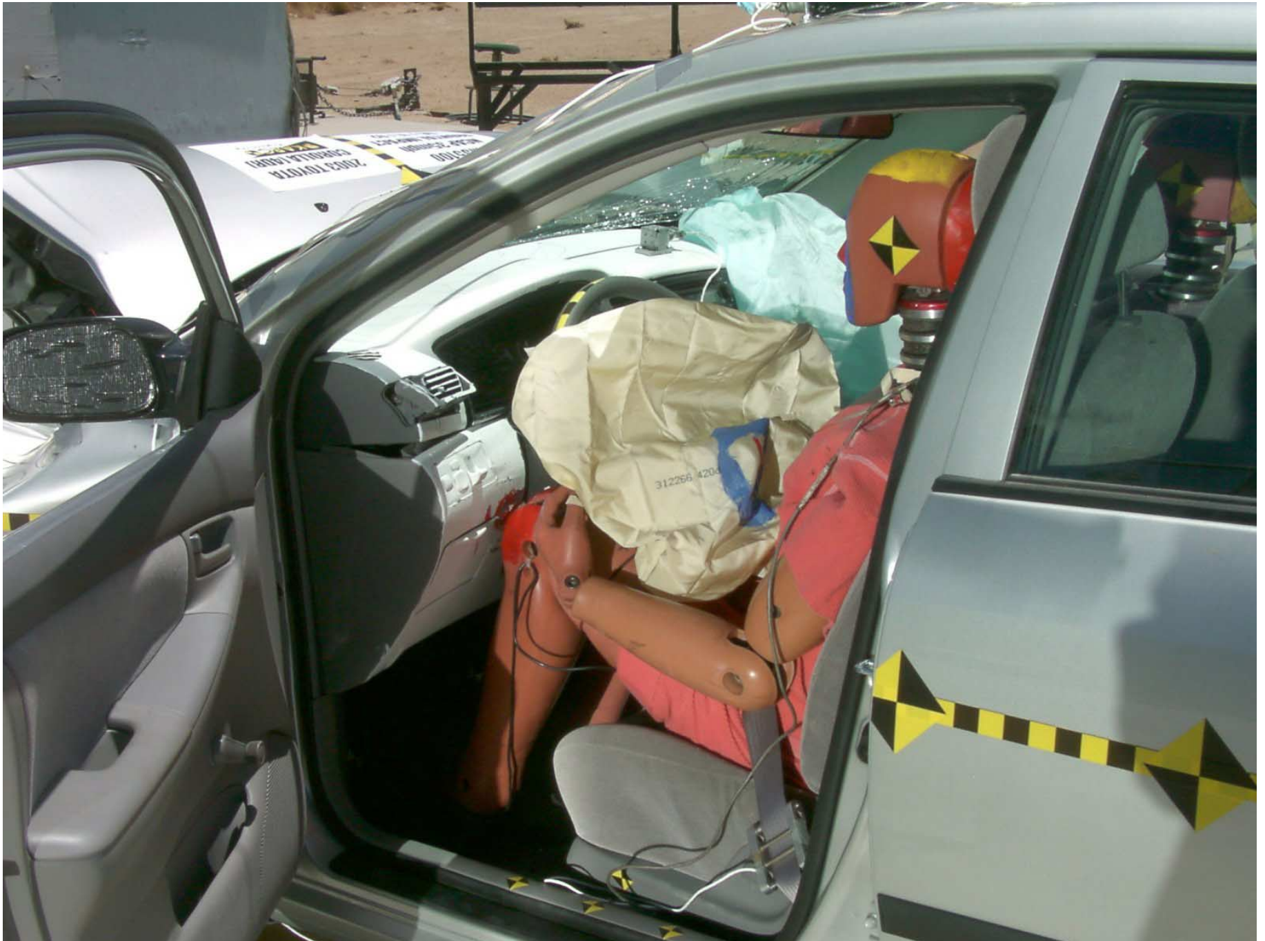
Figure A-30: Driver Dummy Door Open, Post-Test
