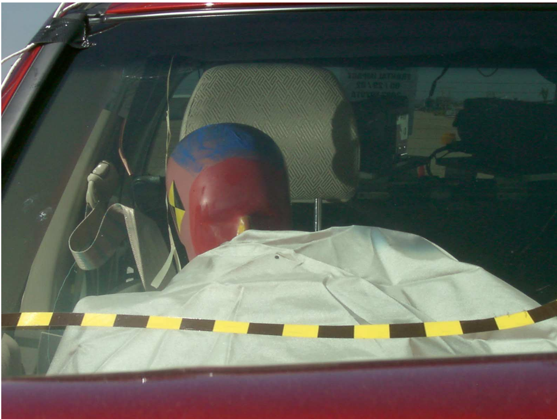
Figure A-42: Passenger Dummy Front View, Post-Test
