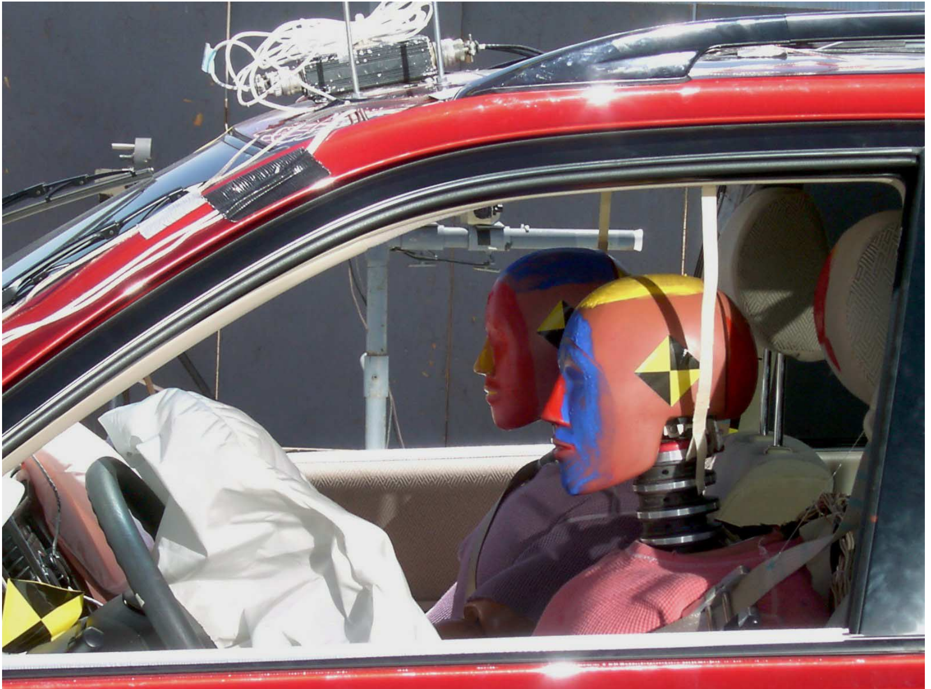
Figure A-28: Driver Dummy Through Window, Post-Test
