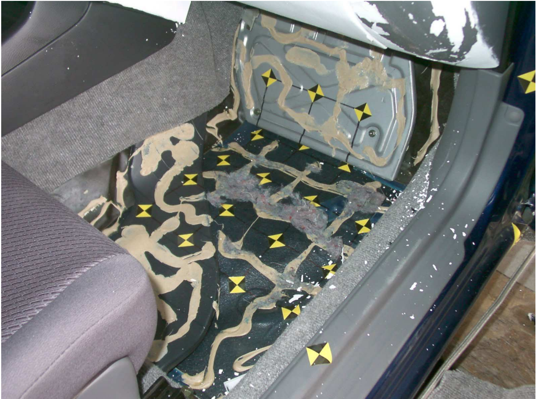
Figure A-52: Passenger Side Floor Pan, Post-Test
