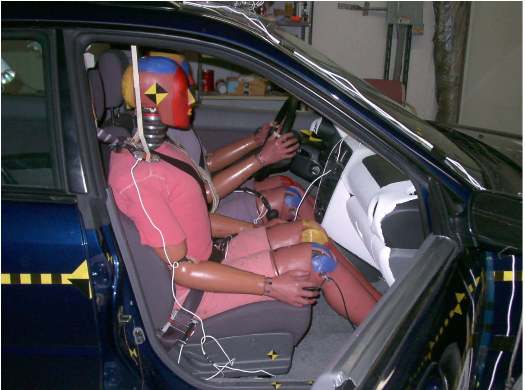
Figure A-47: Passenger Dummy 90° To Vehicle, Pre-Test
