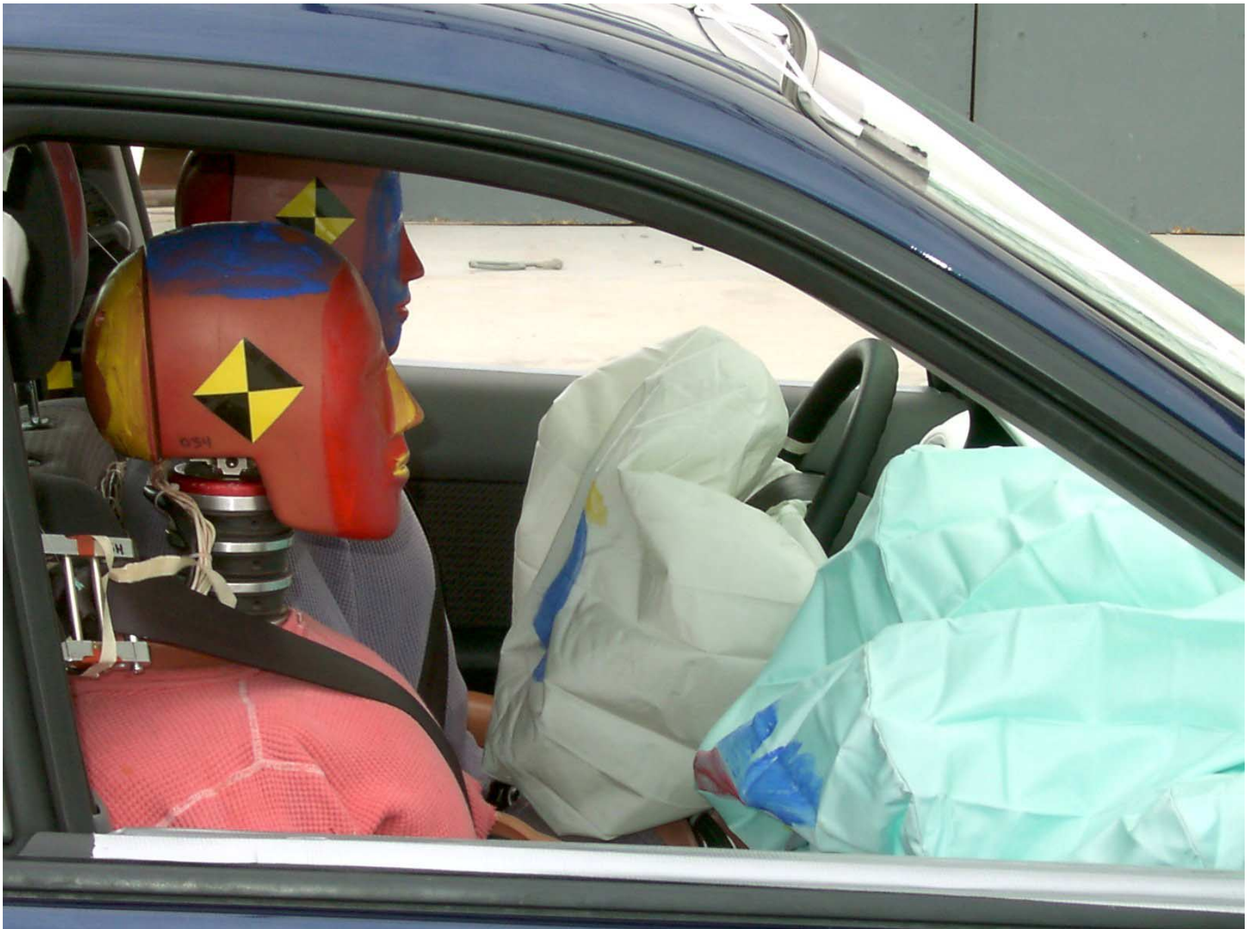
Figure A-44: Passenger Dummy Through Window, Post-Test
