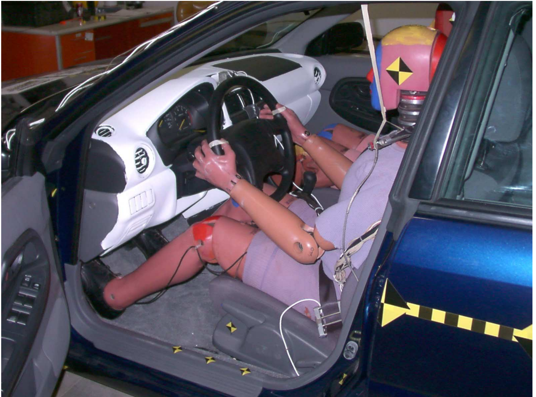
Figure A-29: Driver Dummy Door Open, Pre-Test
