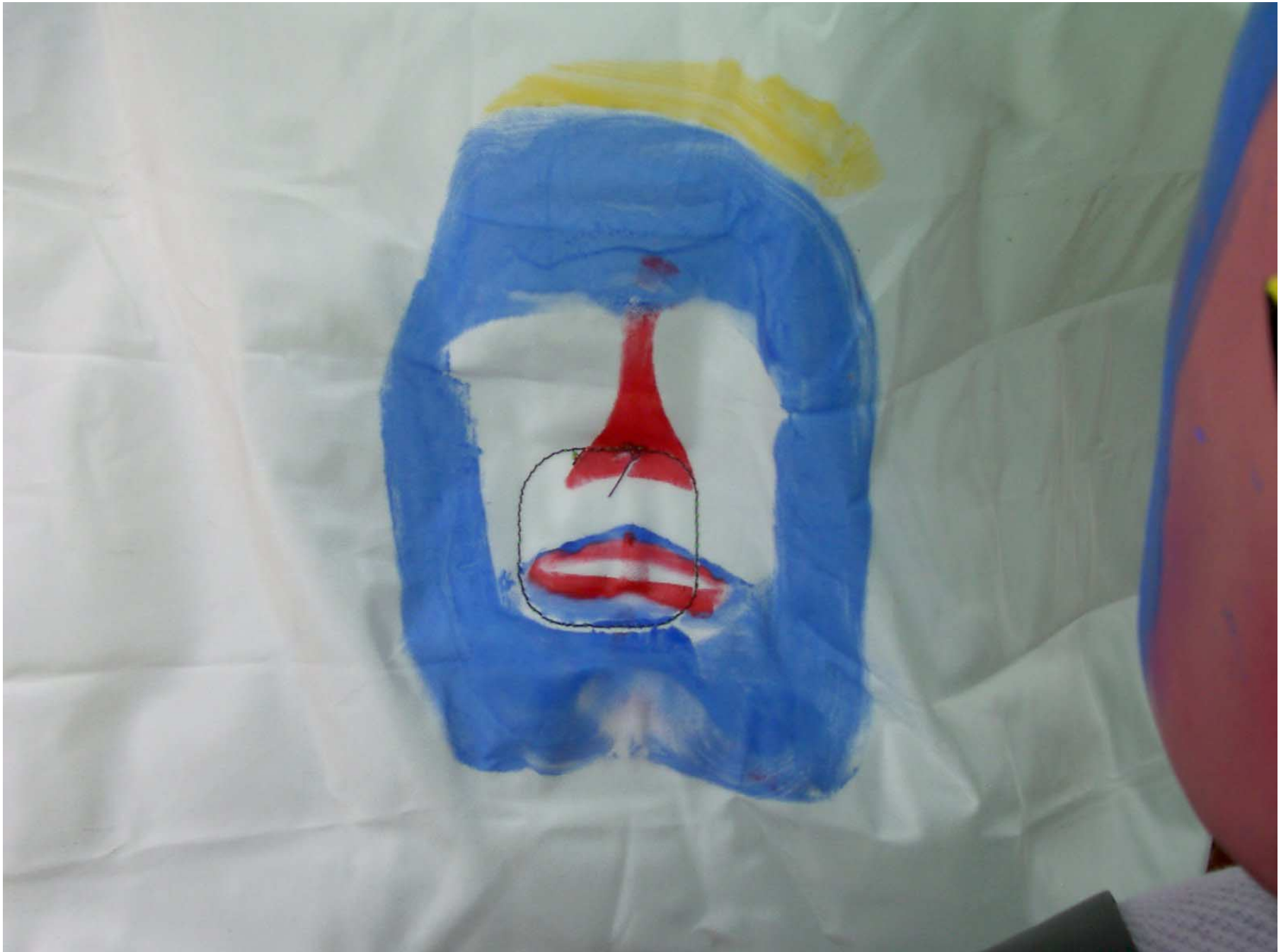
Figure A-40: Driver Dummy Contact, Post-Test
