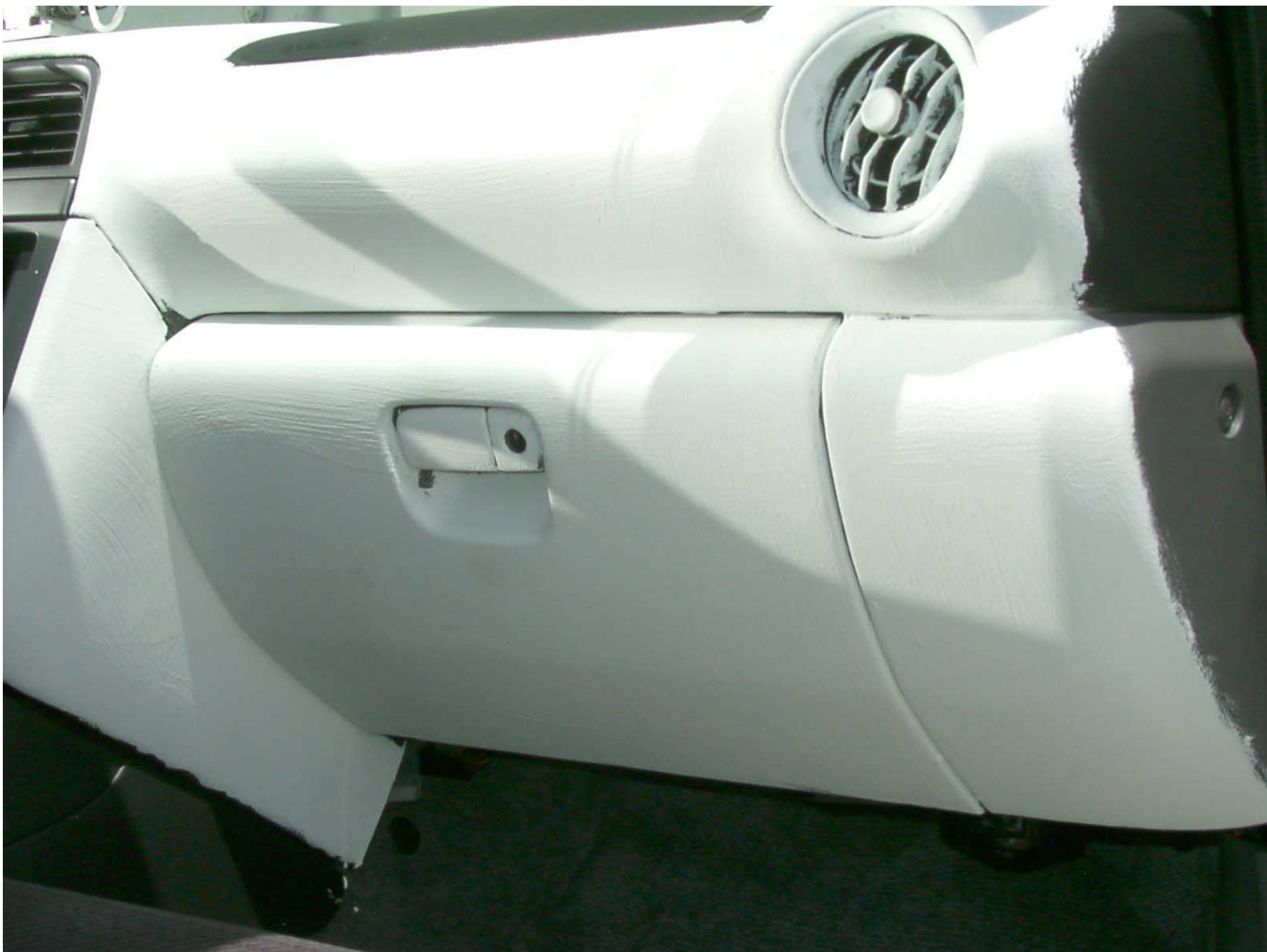
Figure A-53: Passenger Side Knee Bolster, Pre-Test
