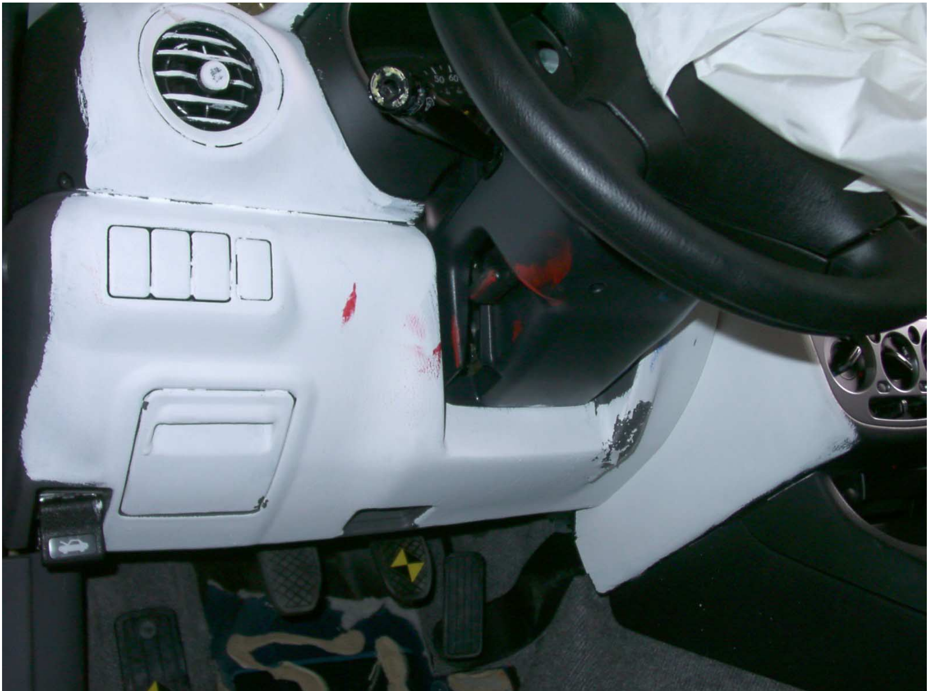
Figure A-36: Driver Side Knee Bolster, Post-Test
