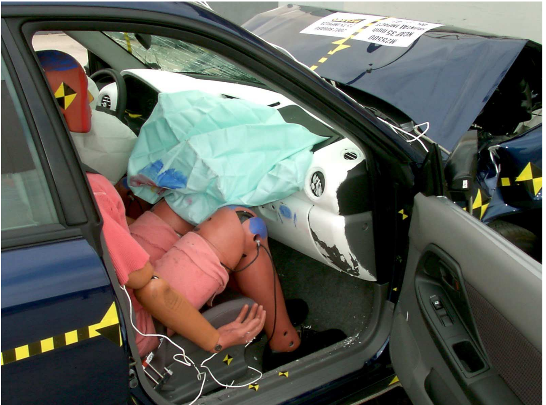
Figure A-46: Passenger Dummy Door Open, Post-Test
