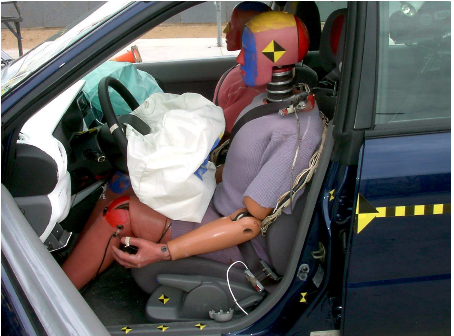
Figure A-32: Driver Dummy 90° To Vehicle, Post-Test
