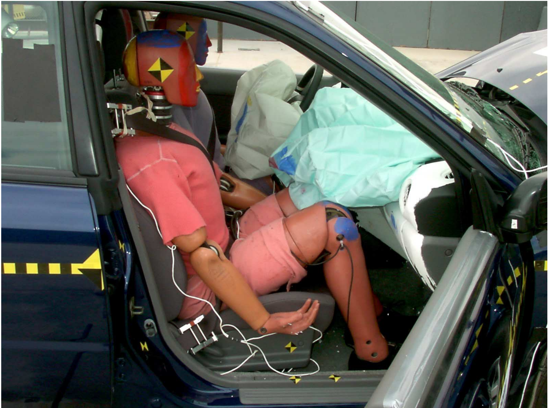
Figure A-48: Passenger Dummy 90° To Vehicle, Post-Test
