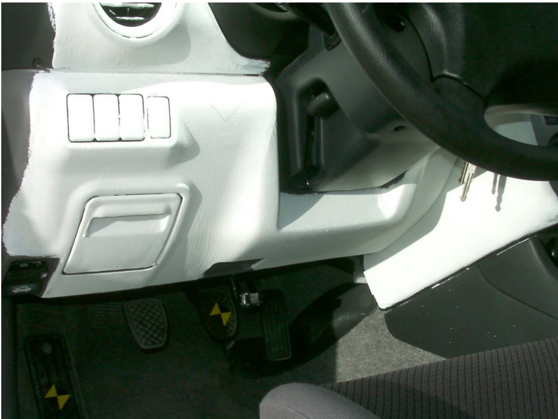
Figure A-35: Driver Side Knee Bolster, Pre-Test
