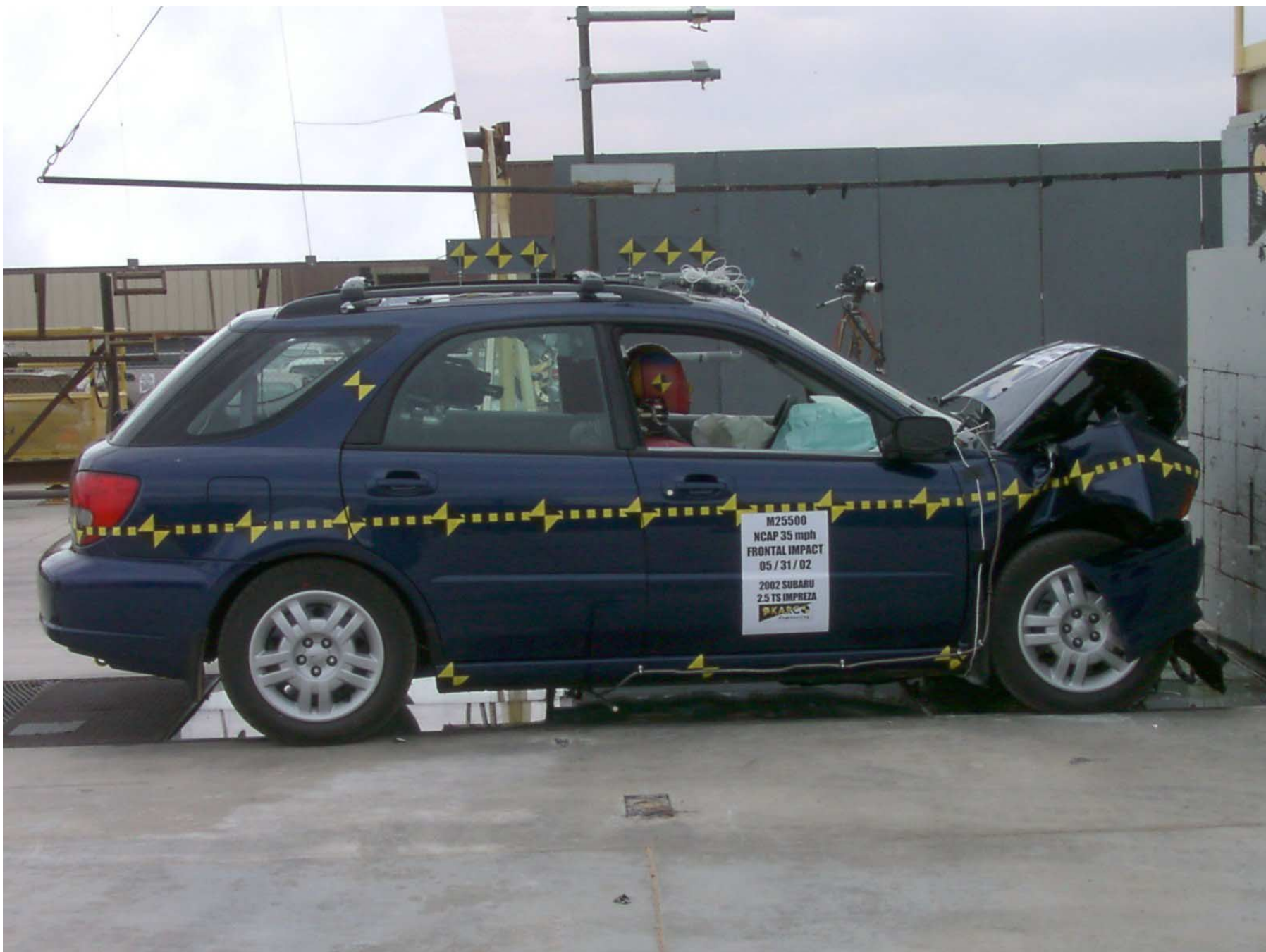
Figure A-10: Right Side View, Post-Test
