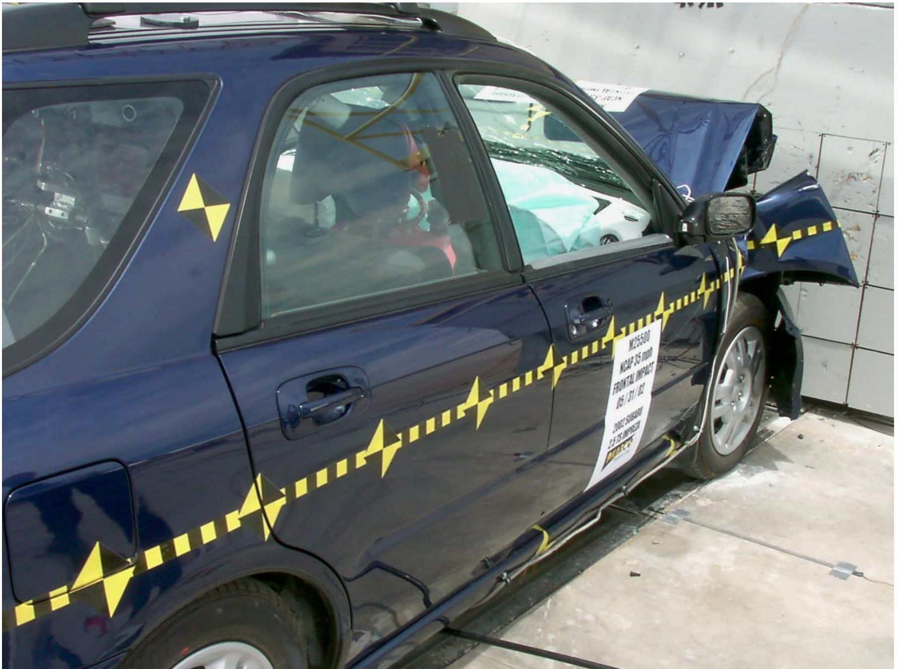
Figure A-58: ¾Right Rear View of Doors After Impact
