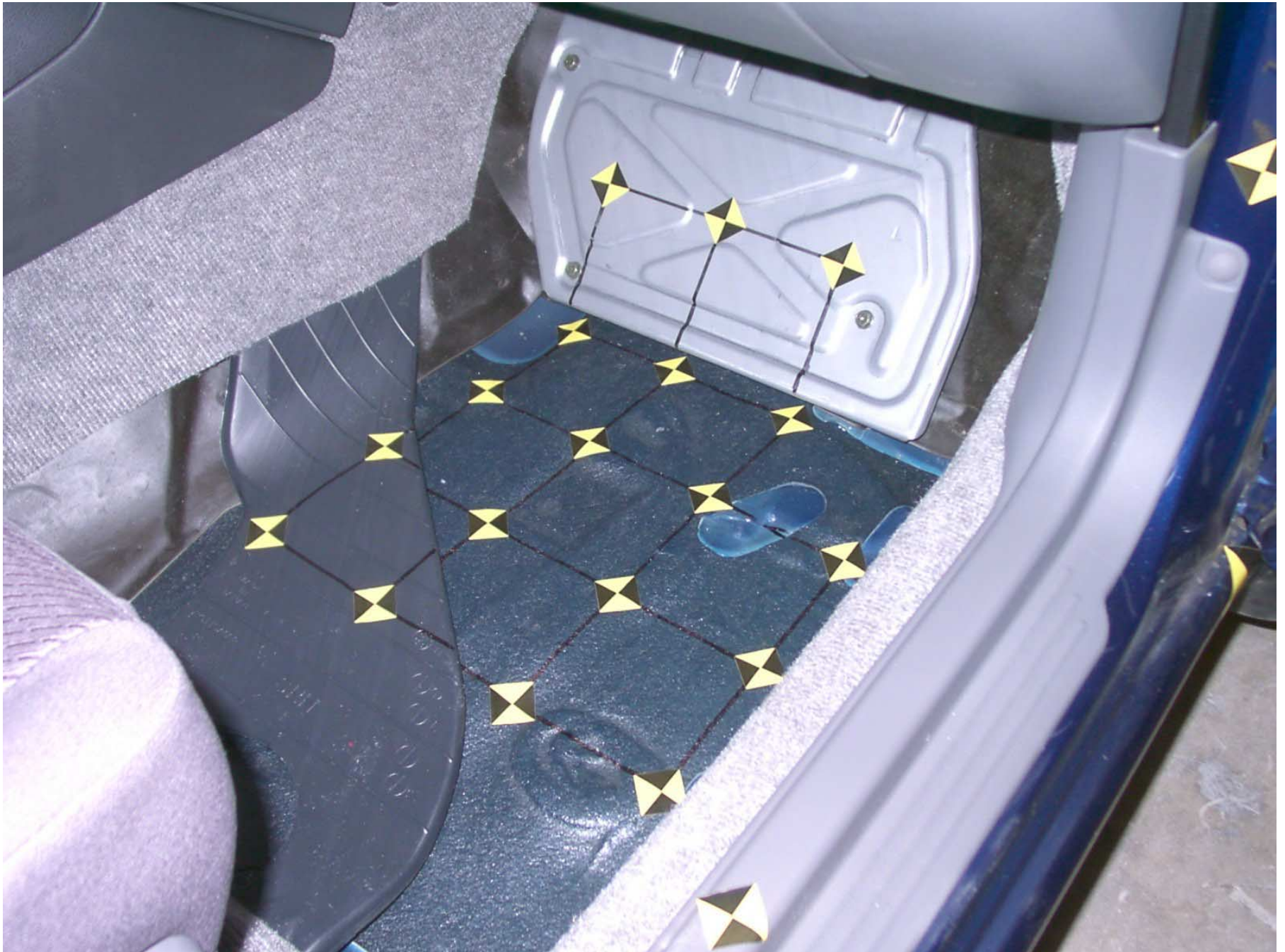
Figure A-51: Passenger Side Floor Pan, Pre-Test
