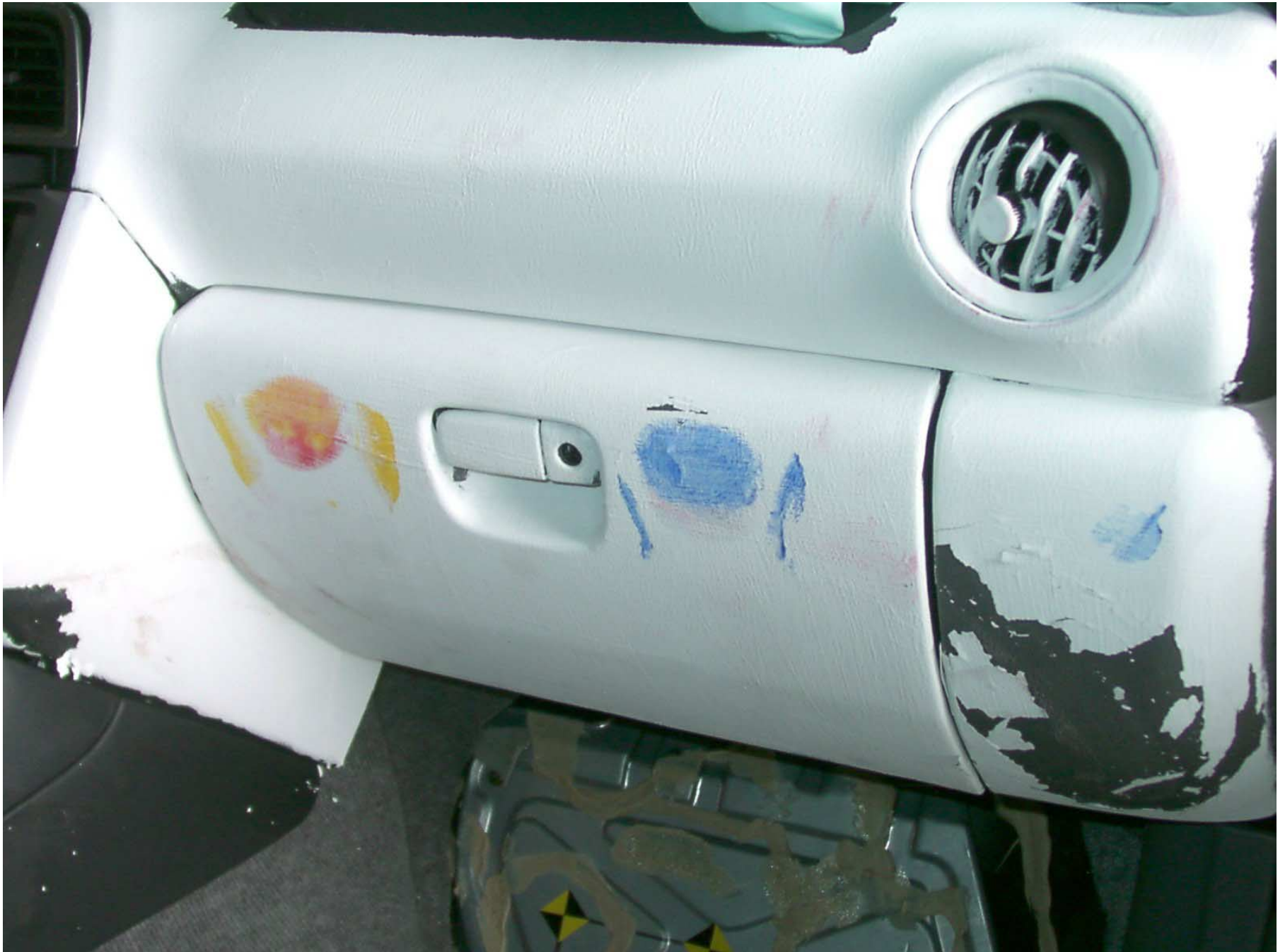
Figure A-54: Passenger Side Knee Bolster, Post-Test
