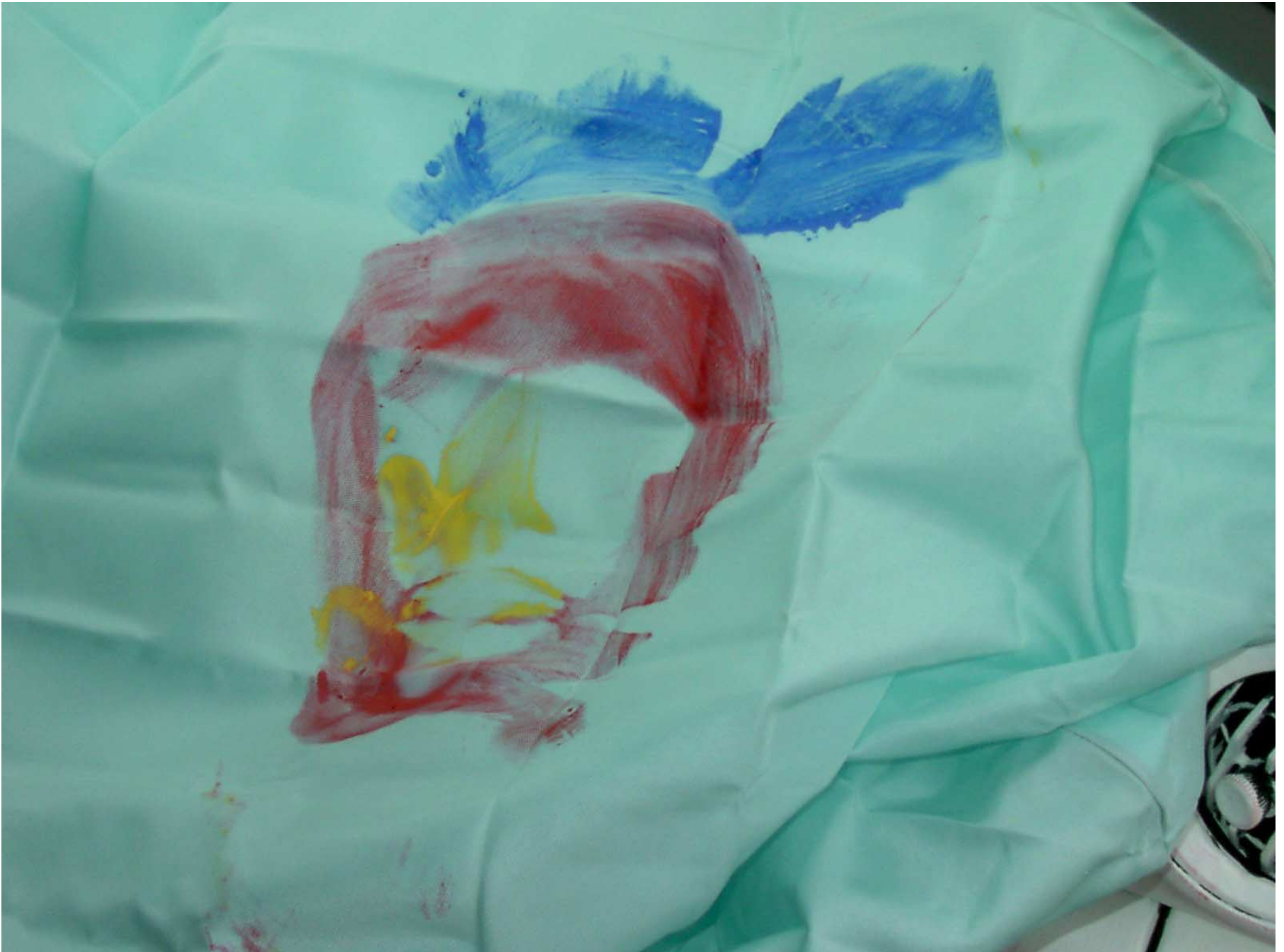
Figure A-56: Passenger Dummy Contact, Post-Test
