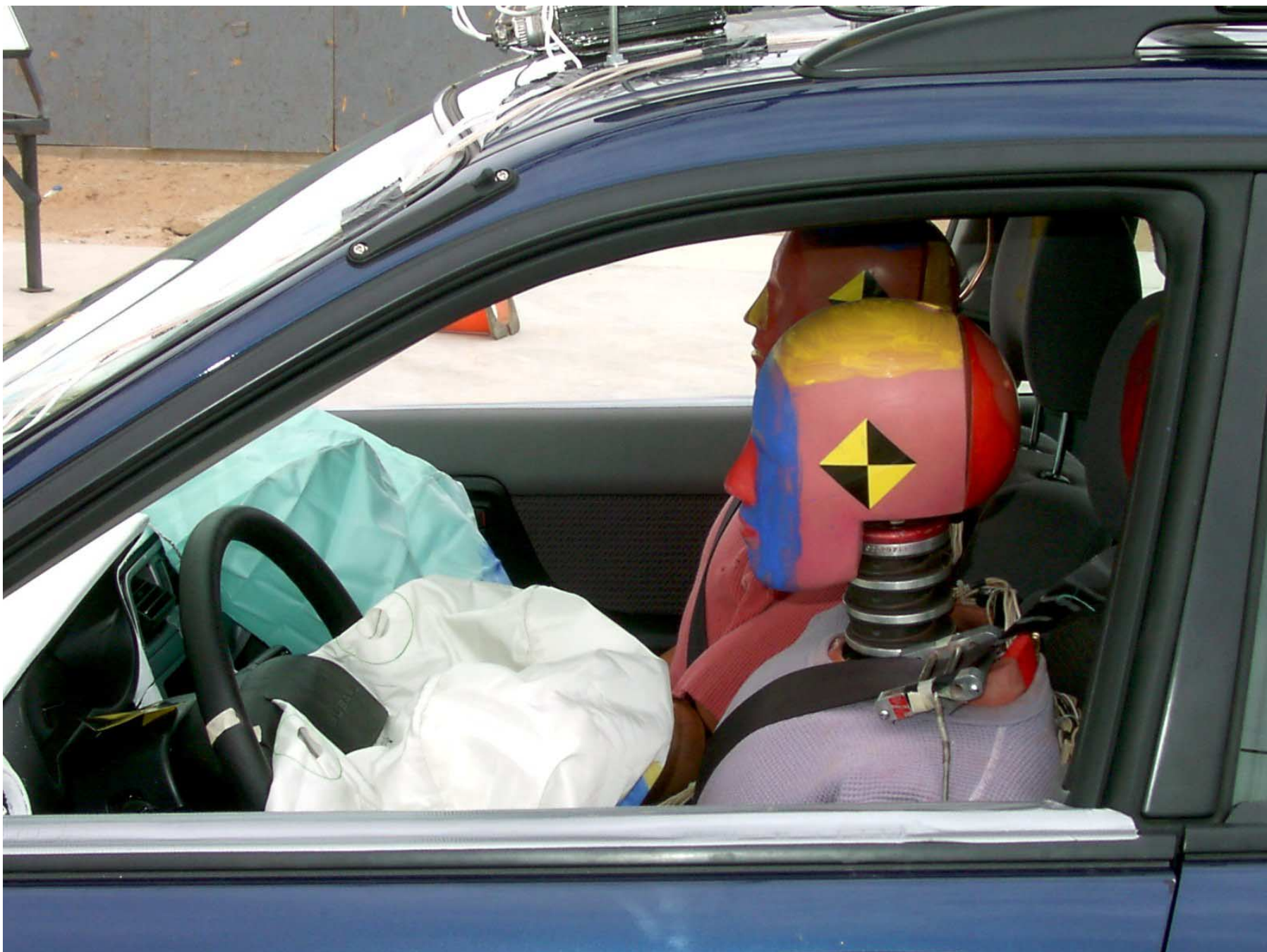
Figure A-28: Driver Dummy Through Window, Post-Test
