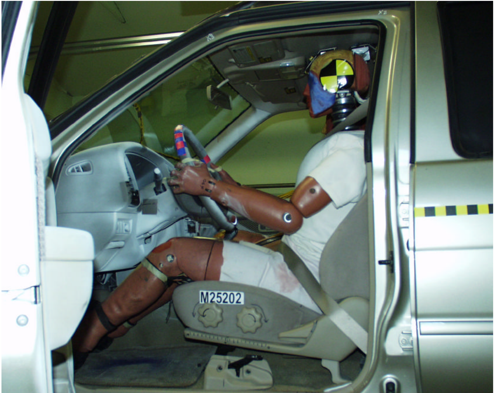
Figure A-22: PRE-TEST DRIVER POSITION VIEW
