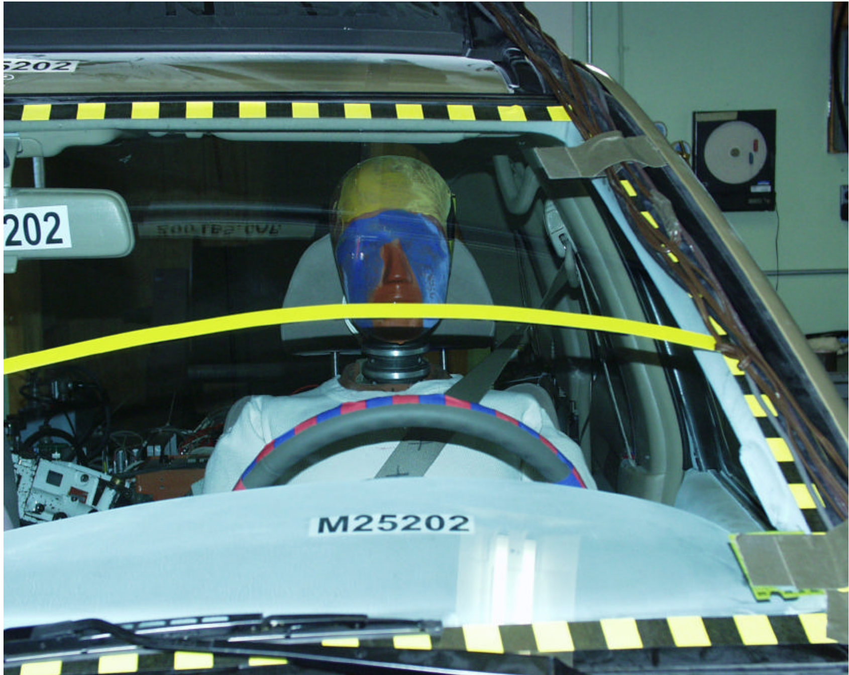
Figure A-30: PRE-TEST DRIVER HEAD LOCATION
