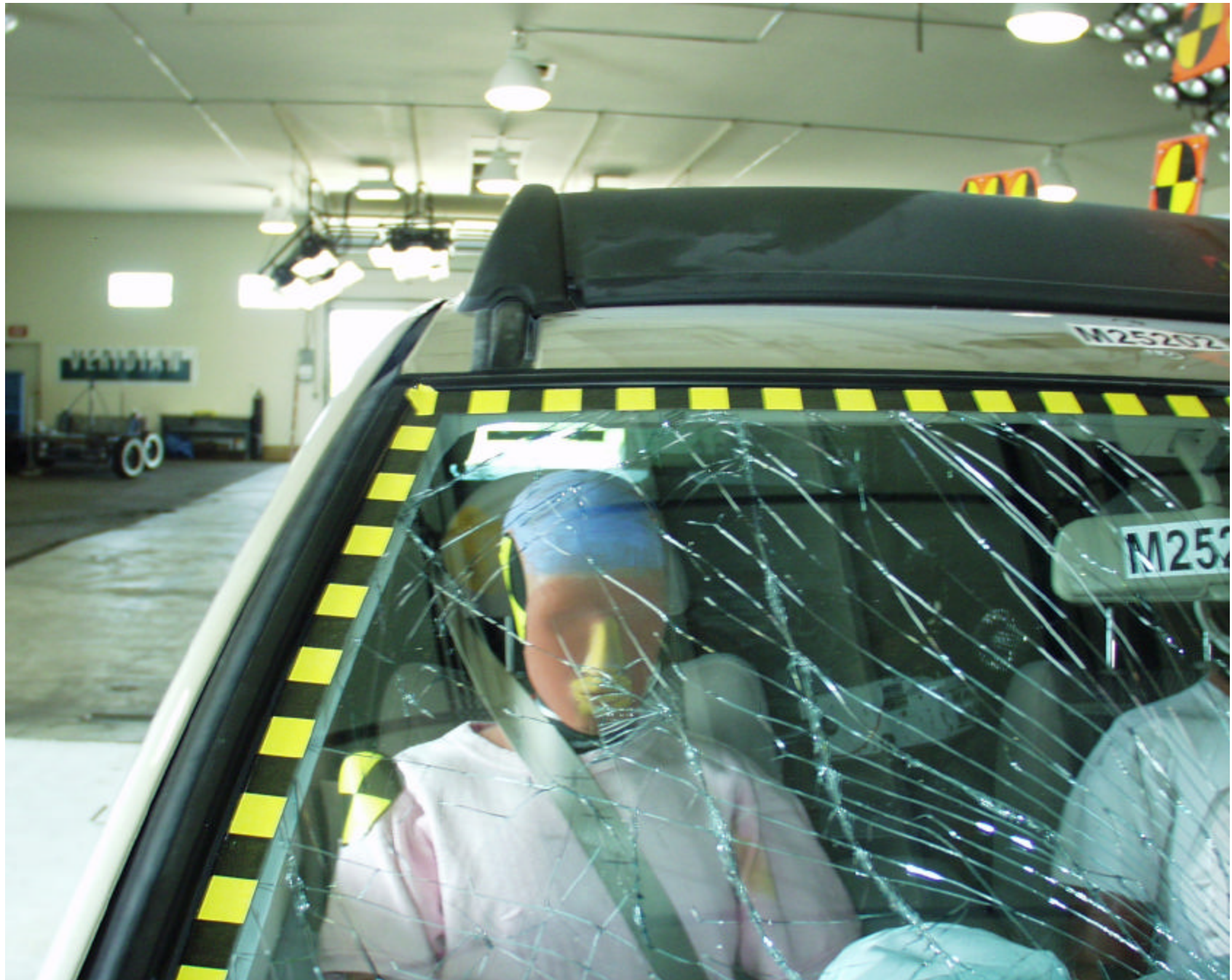
Figure A-33: POST-TEST PASSENGER HEAD LOCATION
