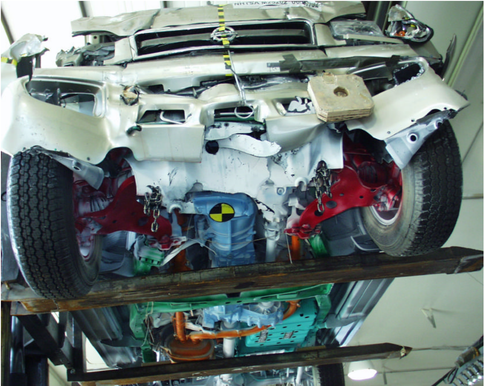
Figure A-17: POST-TEST FRONT UNDERBODY VIEW
