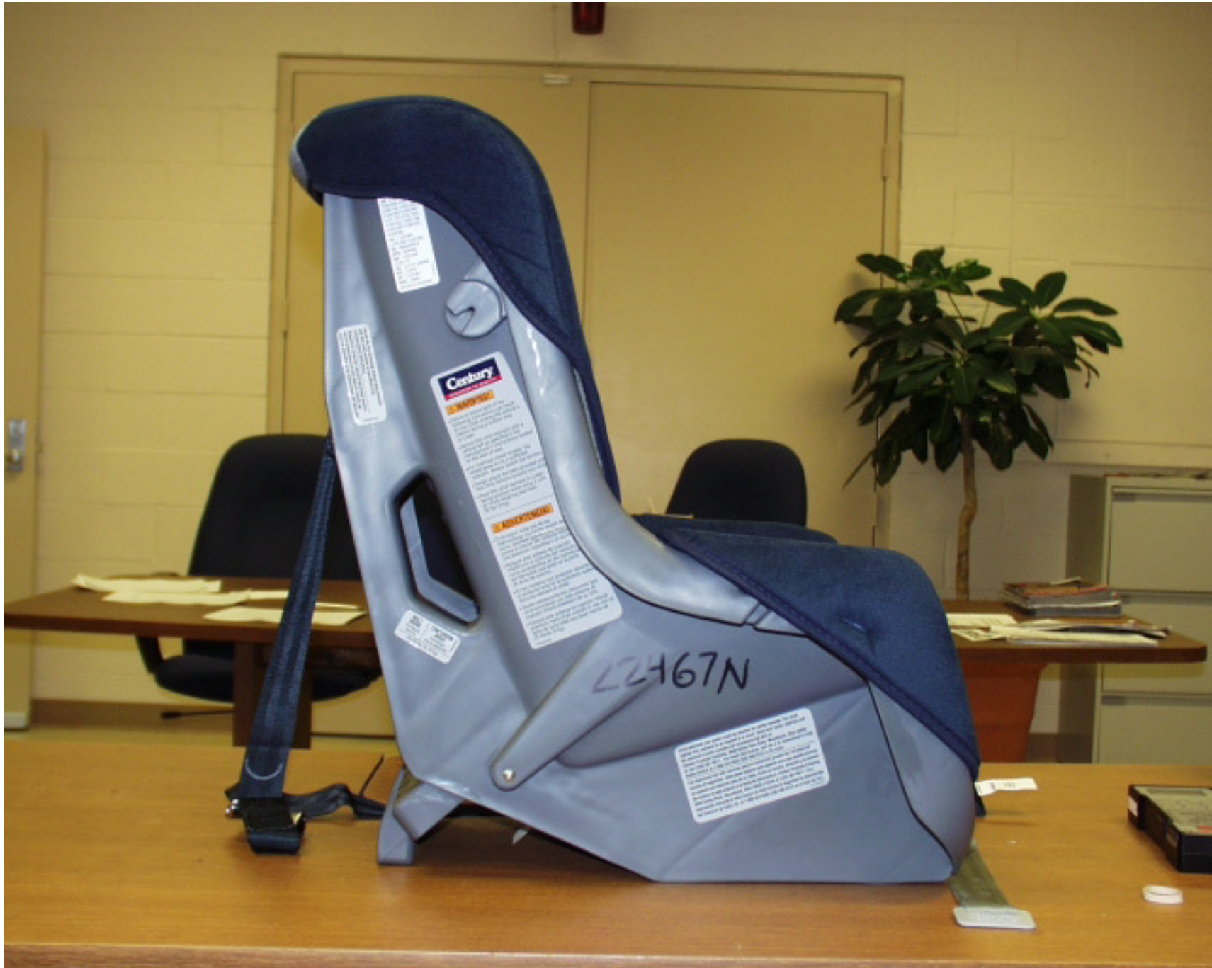
Run #22467 Photo 18 - Post-Test Right View of Child Seat - P4
