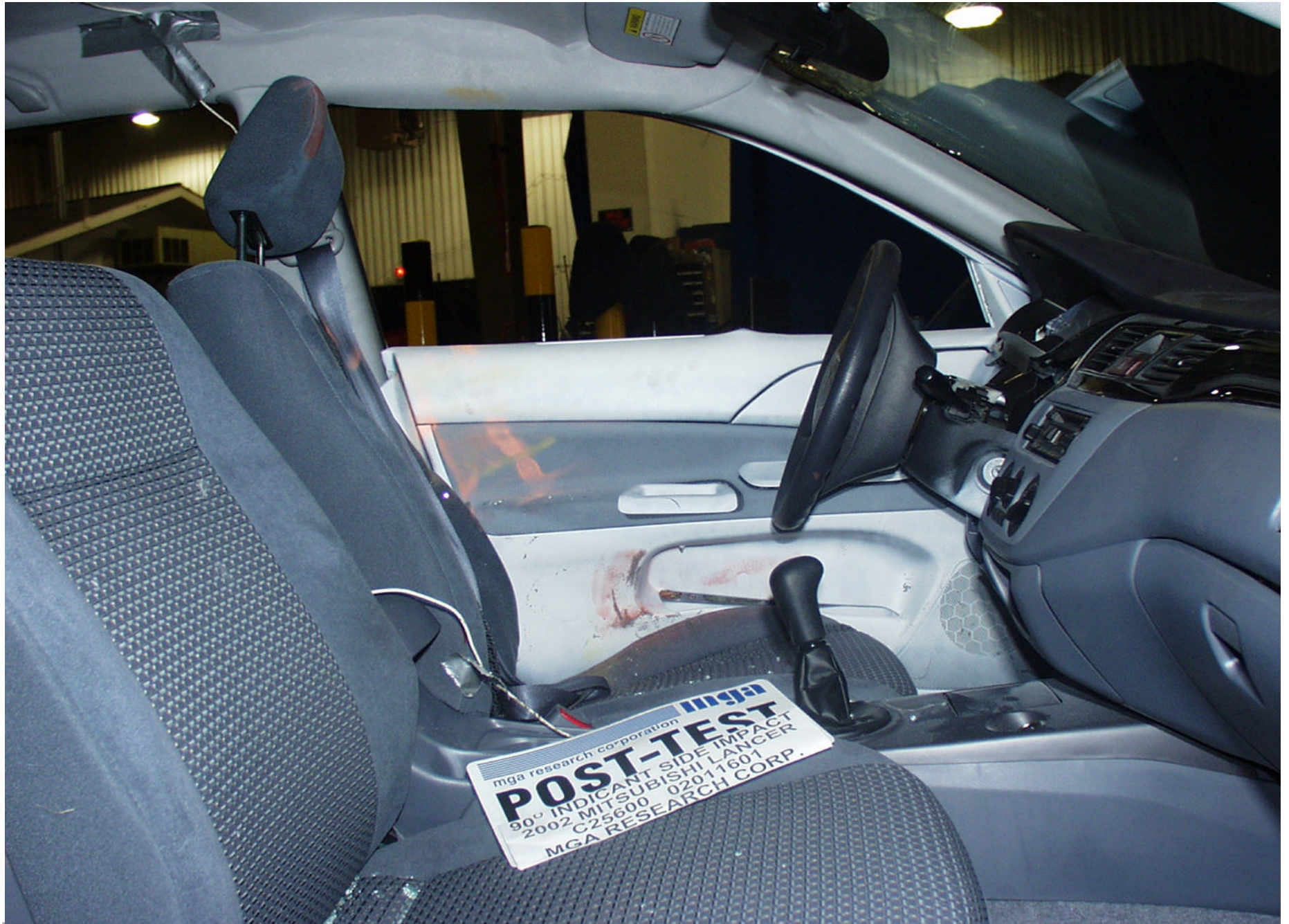
Post-Test Driver Dummy Contact
