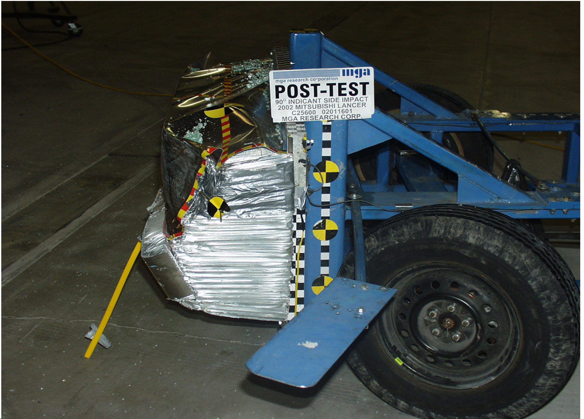
Post-Test MDB Left Side View
