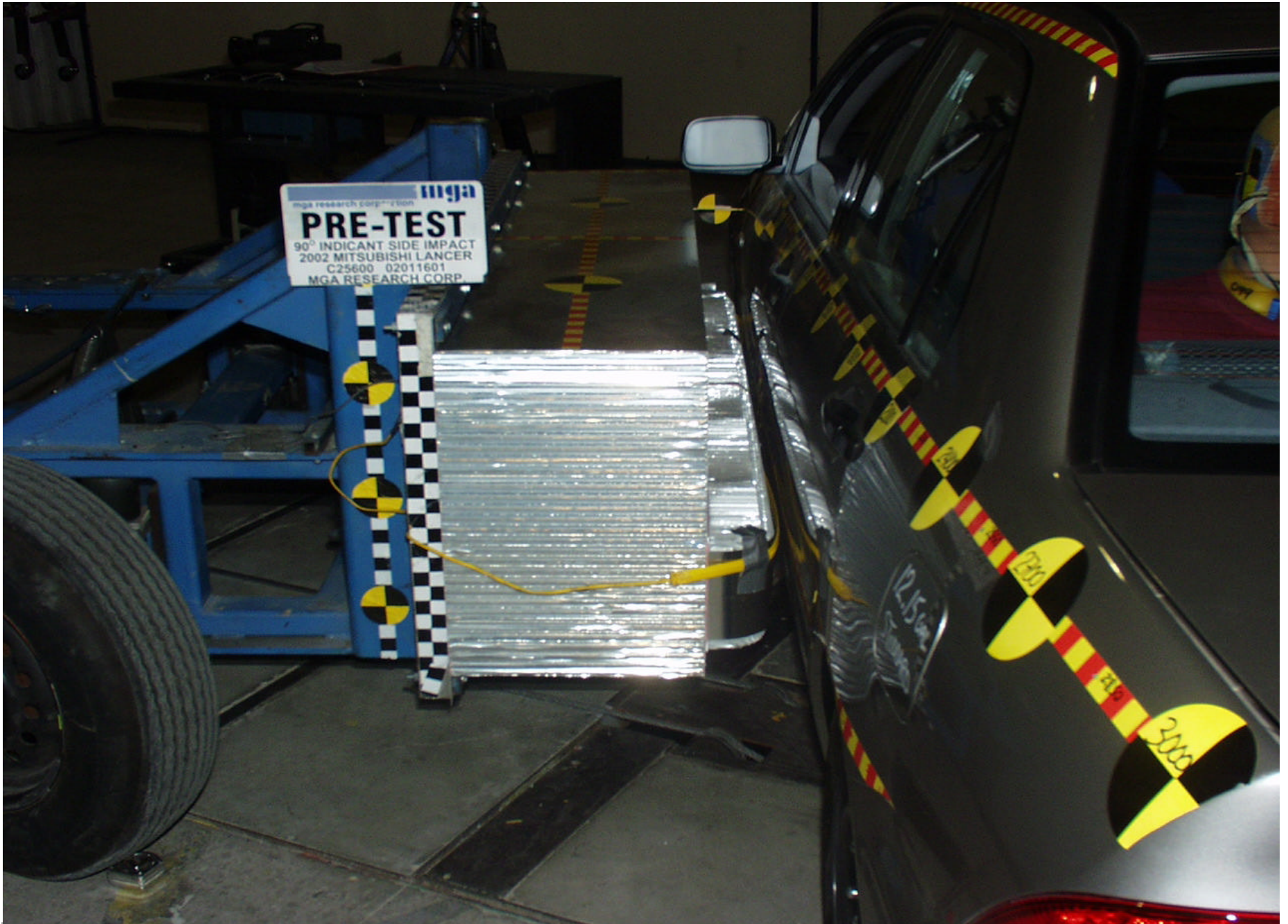
Pre-Test MDB Positioned Against Vehicle (right side)
