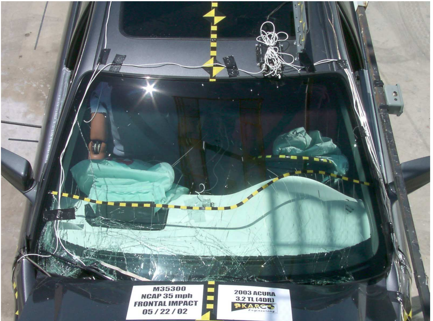
Figure A-16: Windshield, Post-Test
