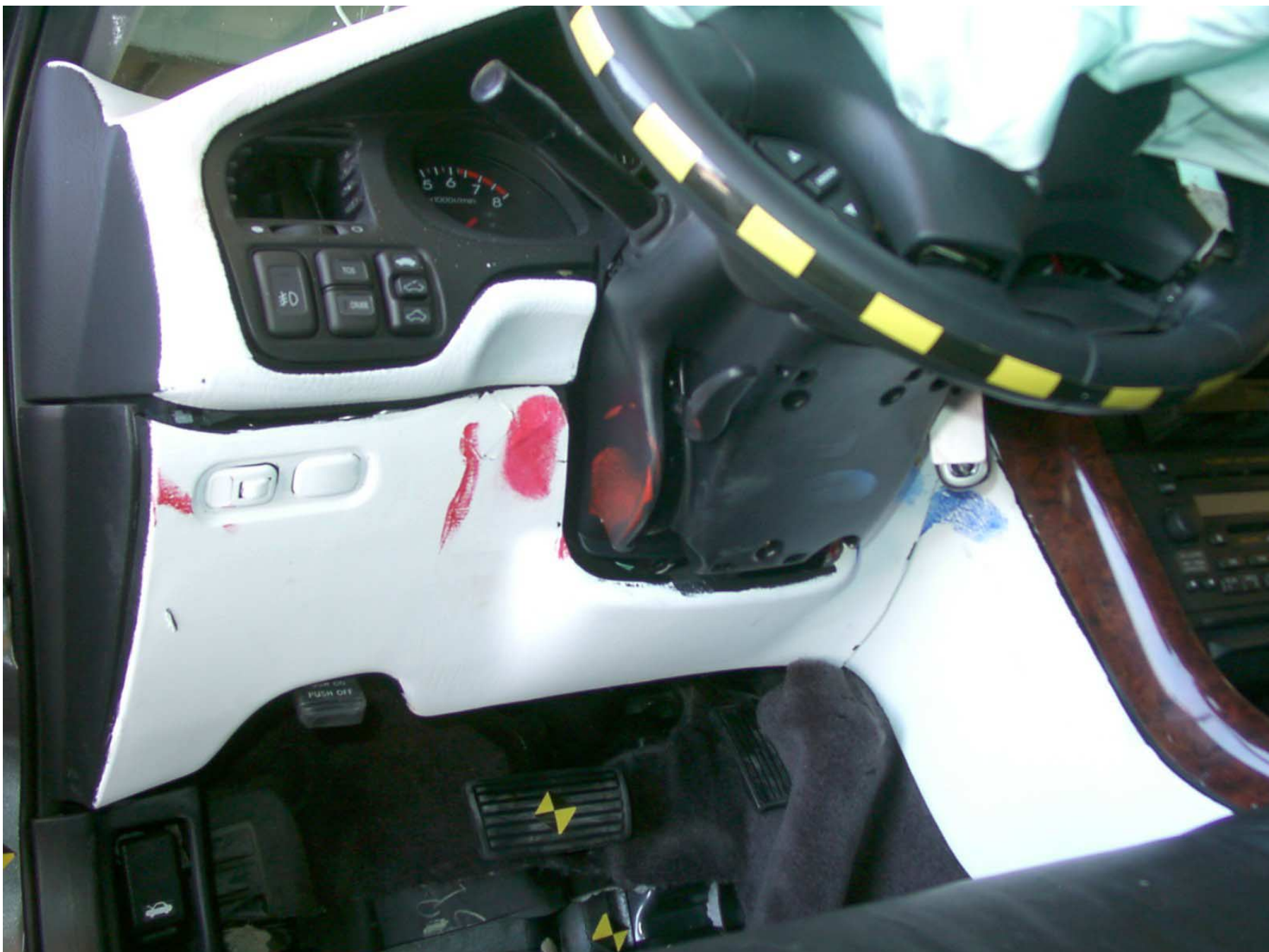
Figure A-36: Driver Side Knee Bolster, Post-Test
