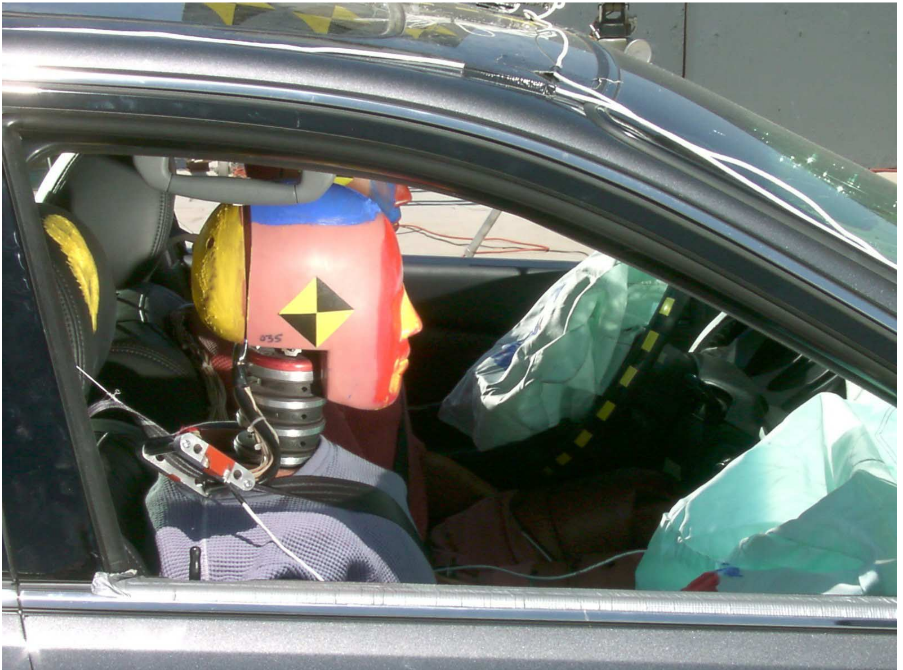
Figure A-44: Passenger Dummy Through Window, Post-Test
