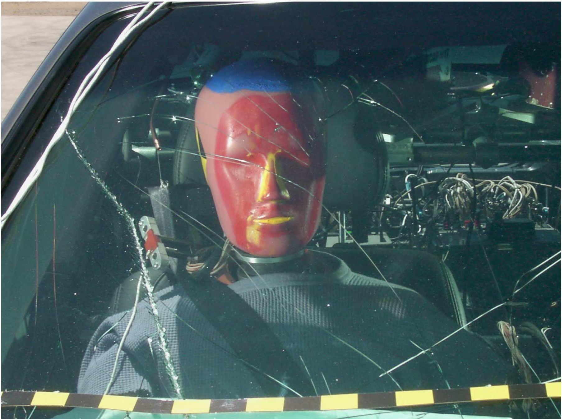
Figure A-42: Passenger Dummy Front View, Post-Test
