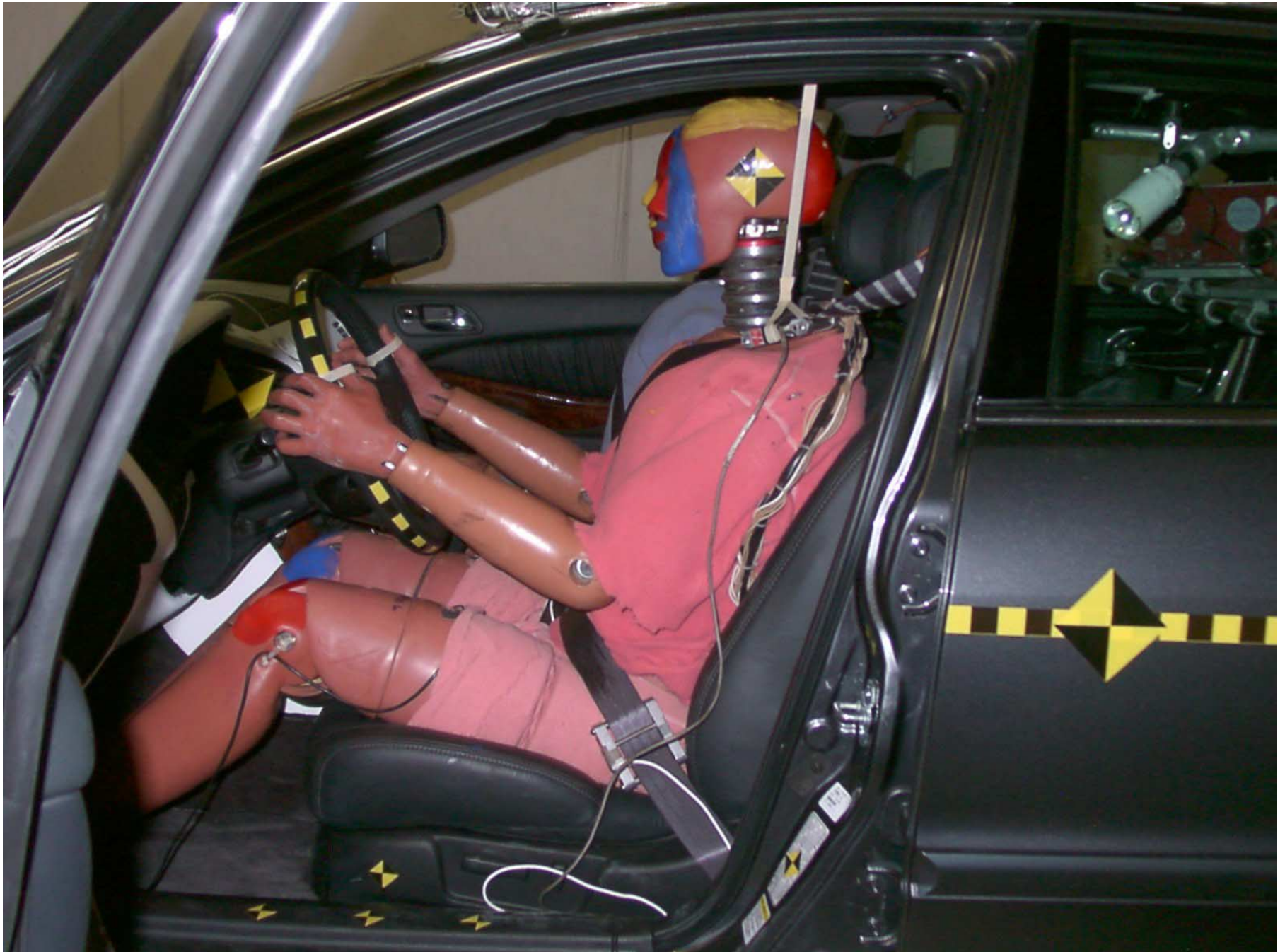
Figure A-31: Driver Dummy 90° To Vehicle, Pre-Test
