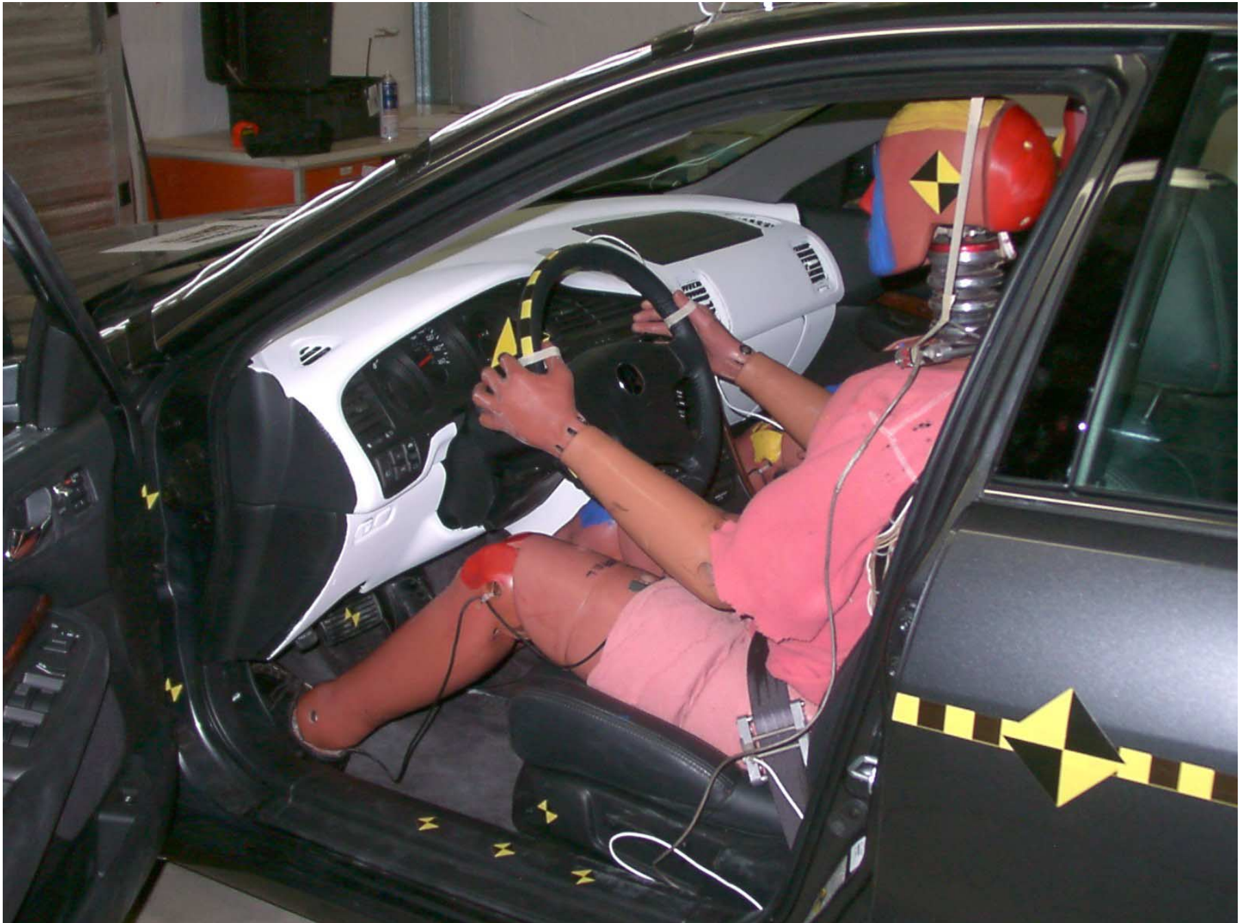
Figure A-29: Driver Dummy Door Open, Pre-Test
