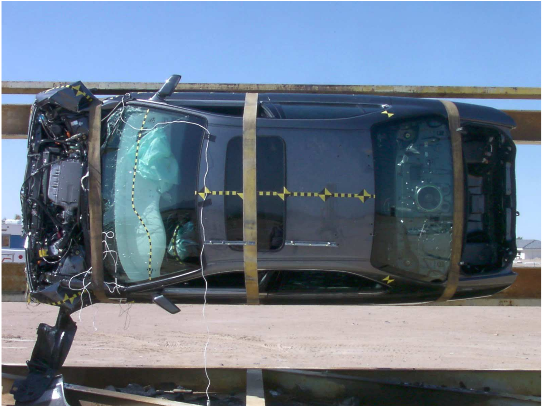
Figure A-59: Vehicle on Rollover Device
