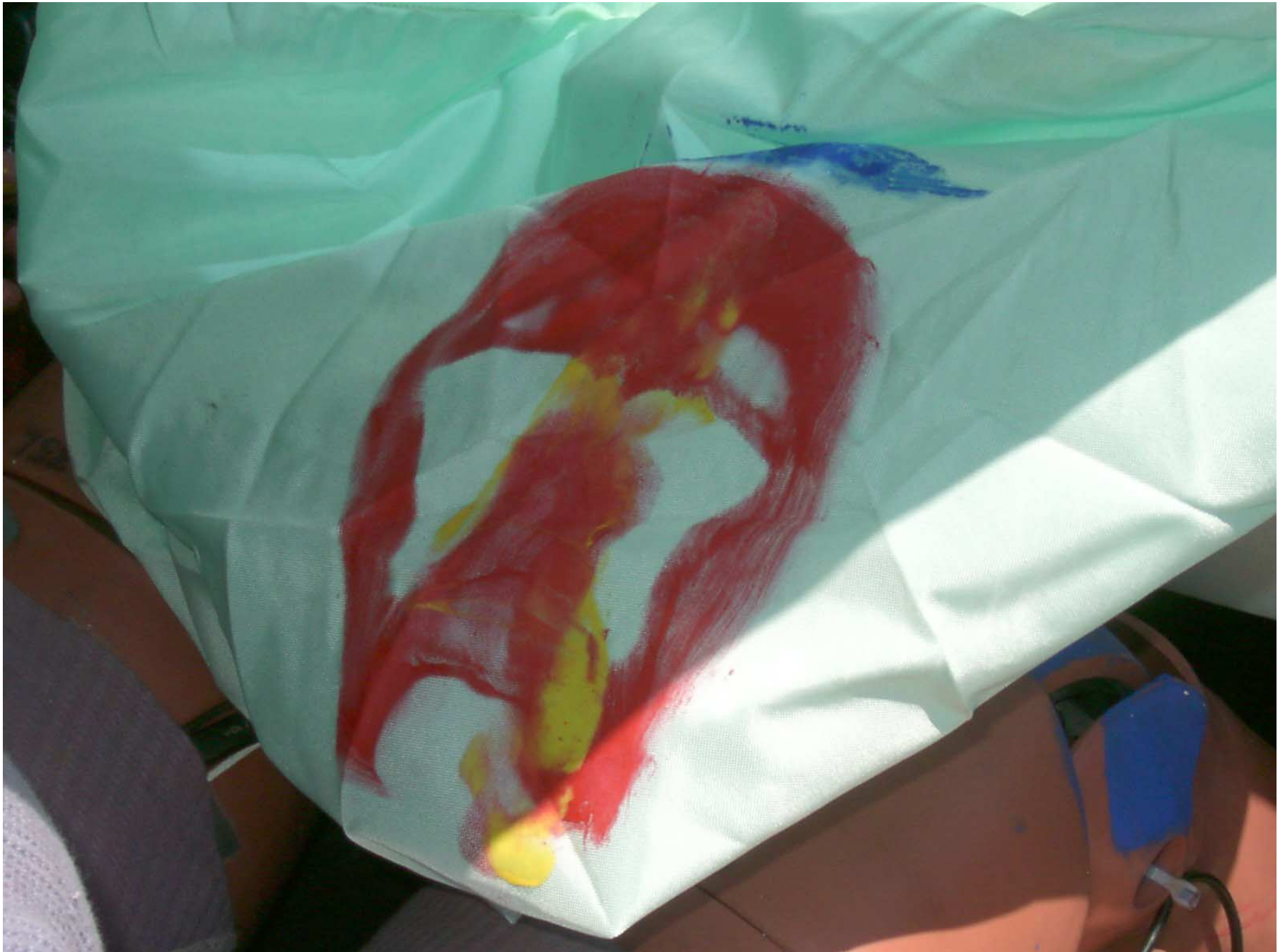
Figure A-56: Passenger Dummy Contact, Post-Test
