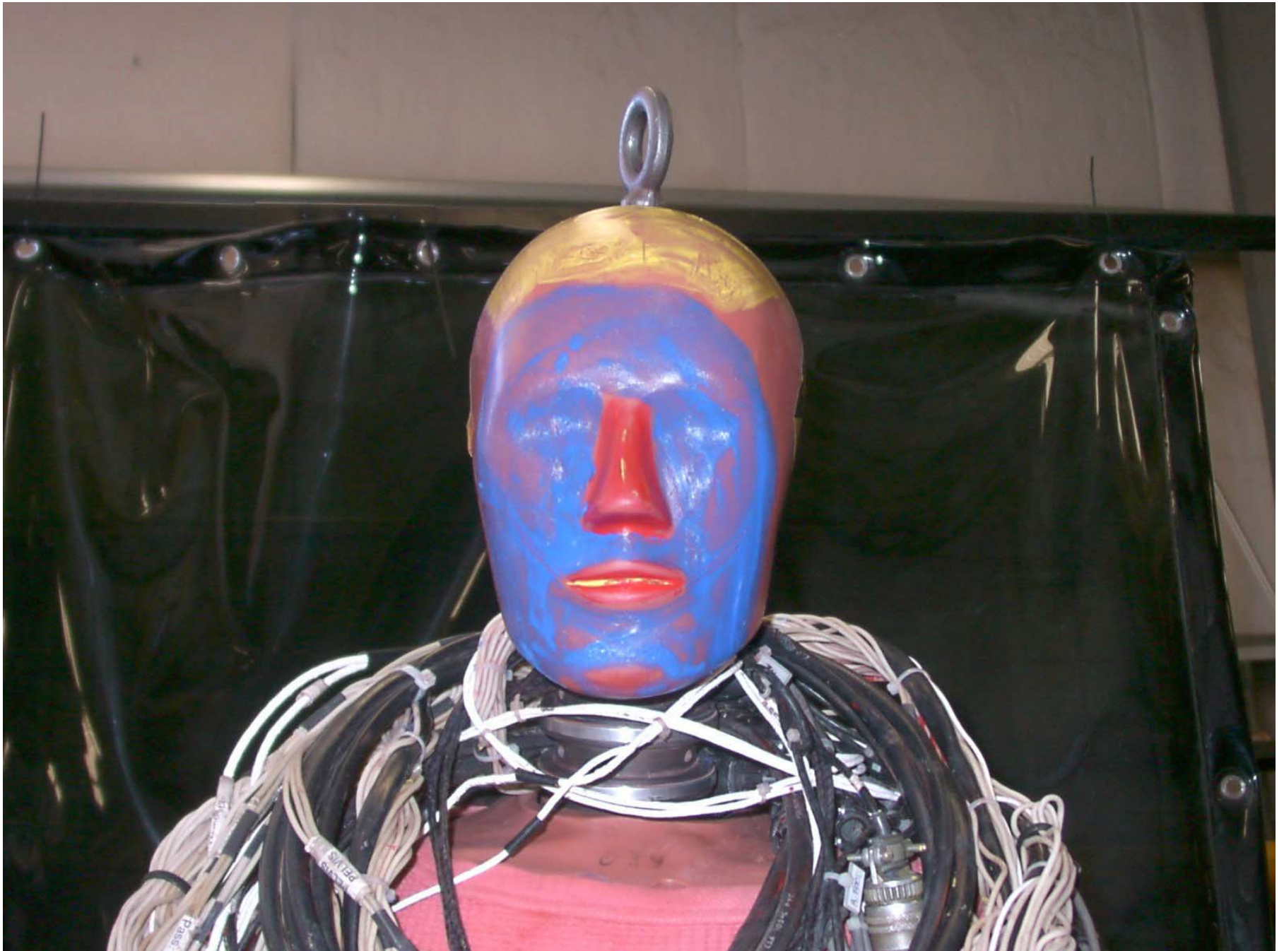
Figure A-39: Driver Dummy Head, Post-Test
