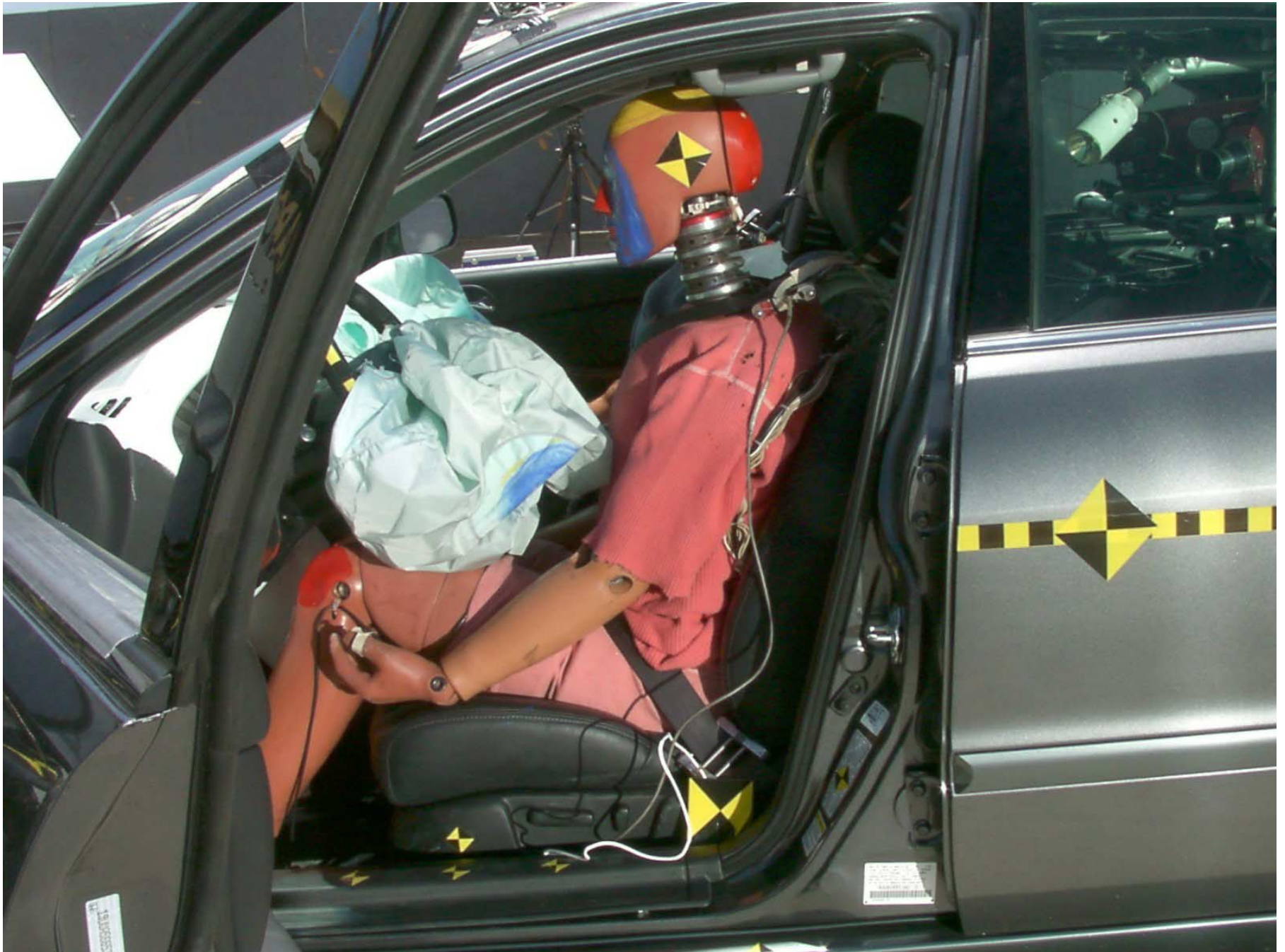
Figure A-32: Driver Dummy 90° To Vehicle, Post-Test
