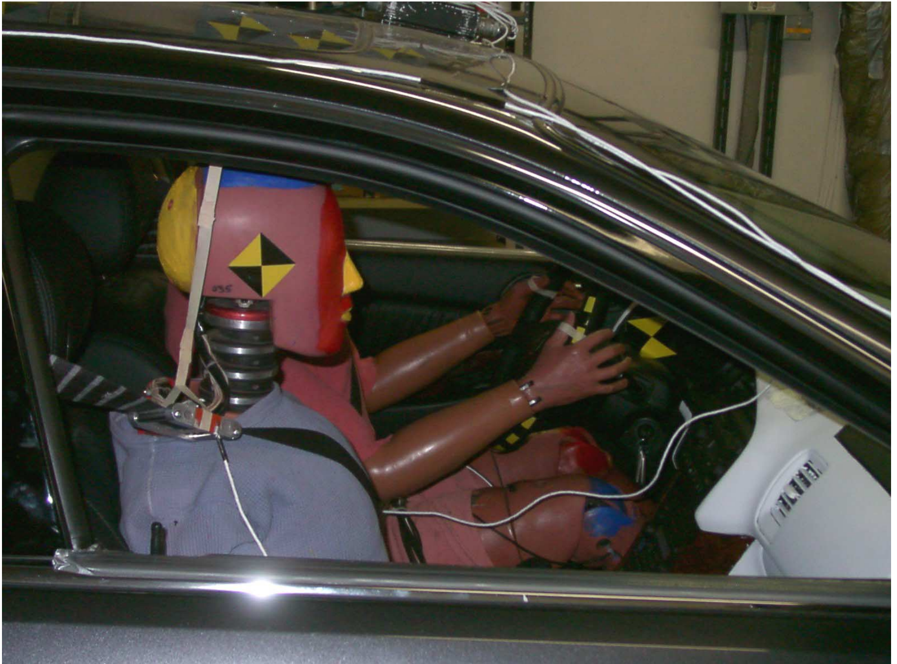
Figure A-43: Passenger Dummy Through Window, Pre-Test
