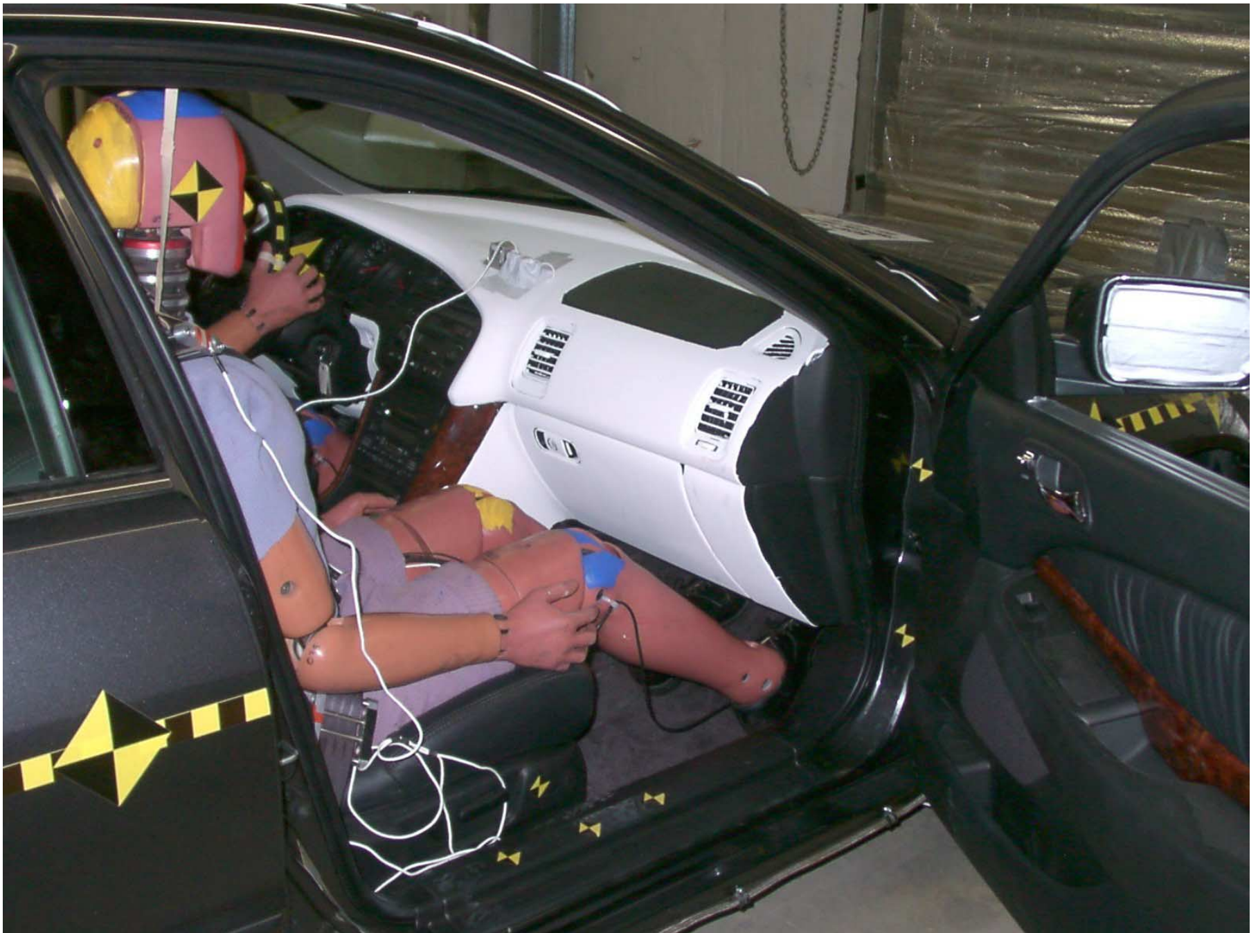
Figure A-45: Passenger Dummy Door Open, Pre-Test
