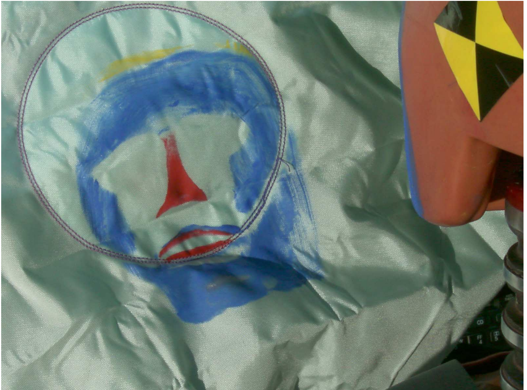
Figure A-40: Driver Dummy Contact, Post-Test
