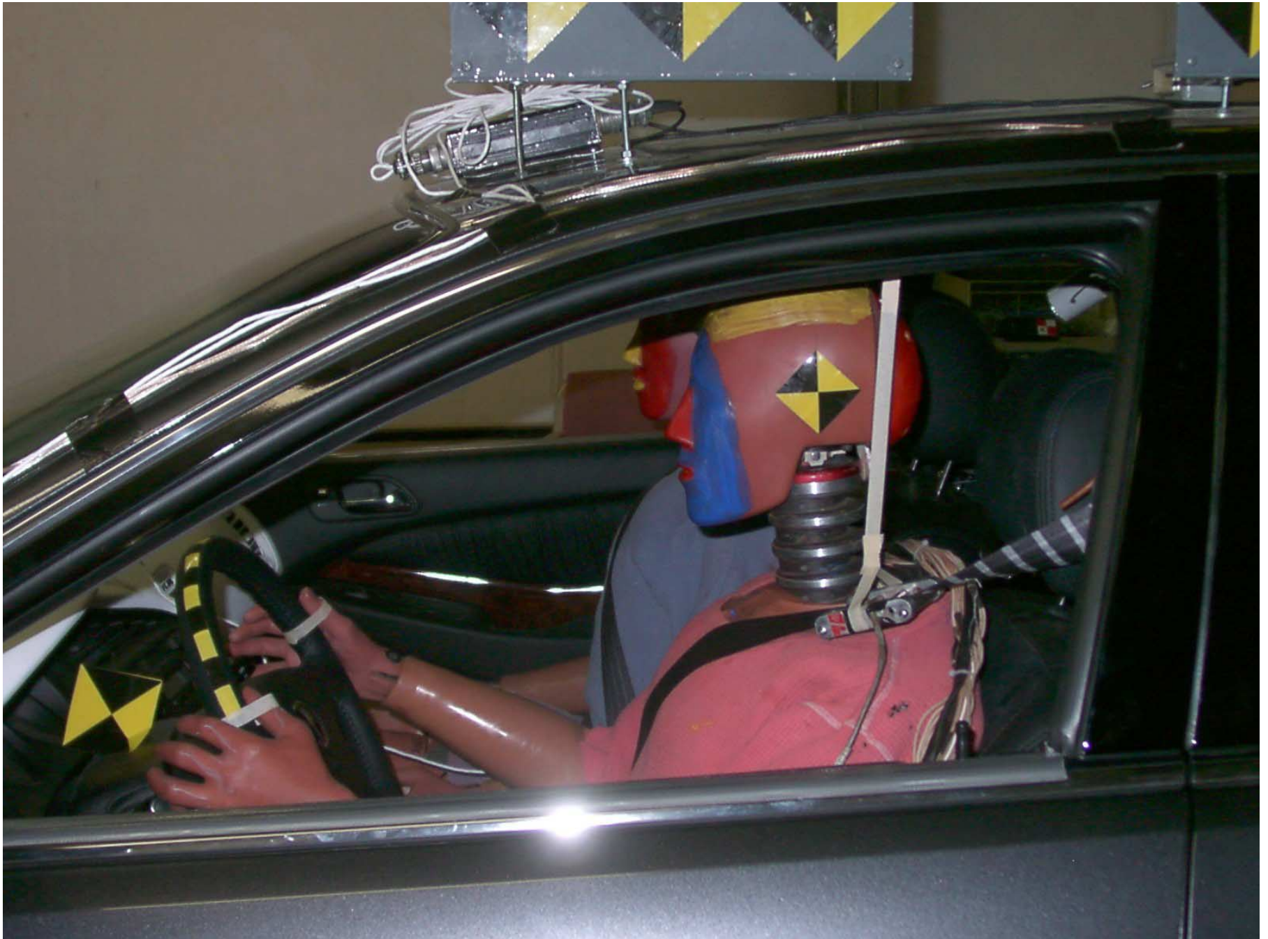
Figure A-27: Driver Dummy Through Window, Pre-Test
