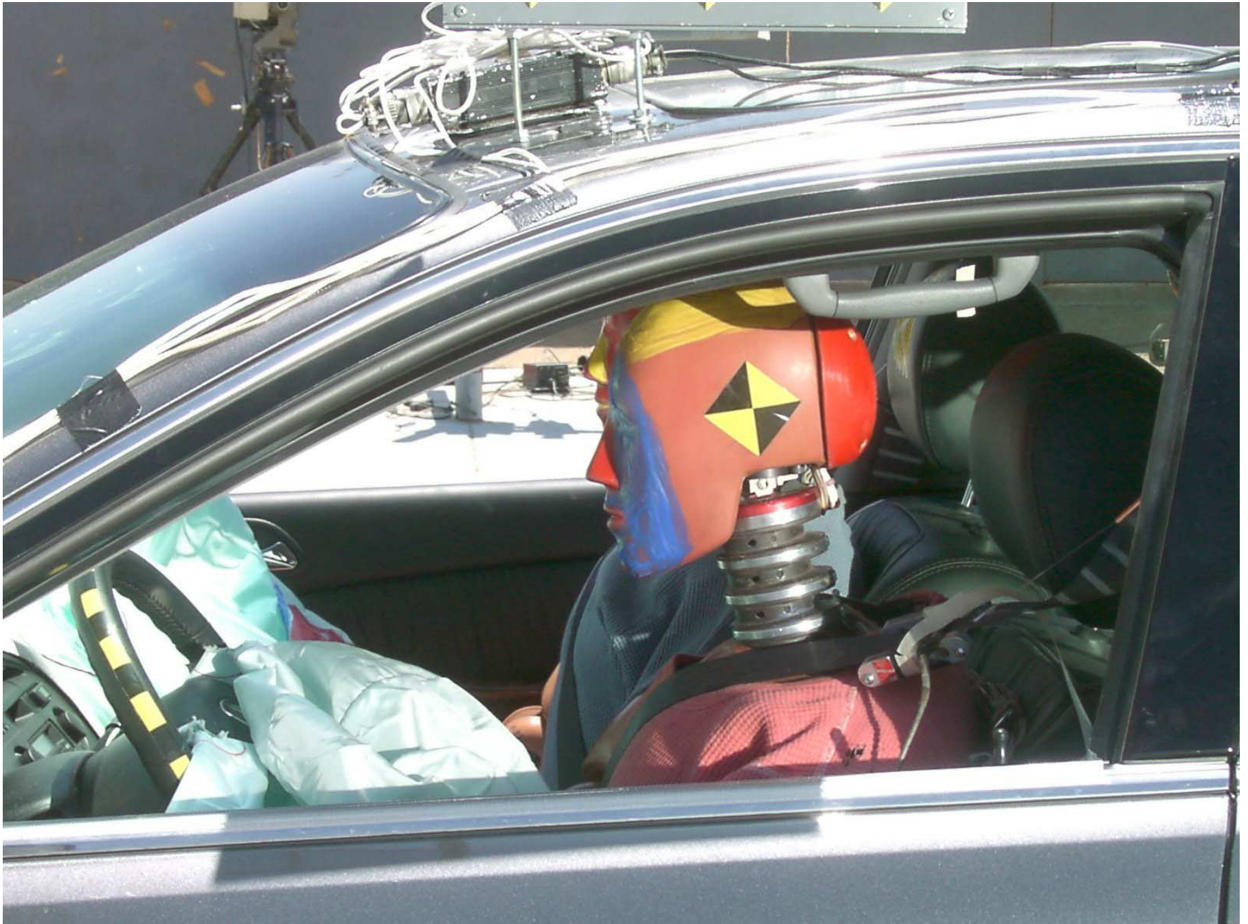
Figure A-28: Driver Dummy Through Window, Post-Test
