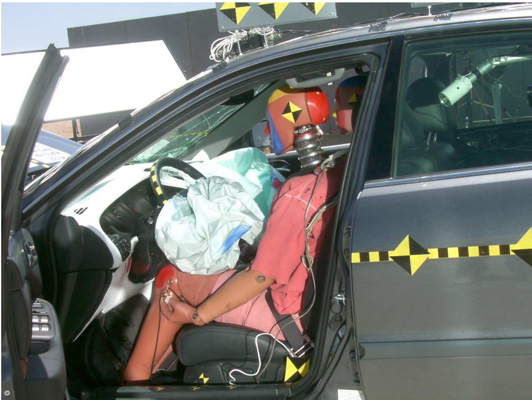
Figure A-30: Driver Dummy Door Open, Post-Test
