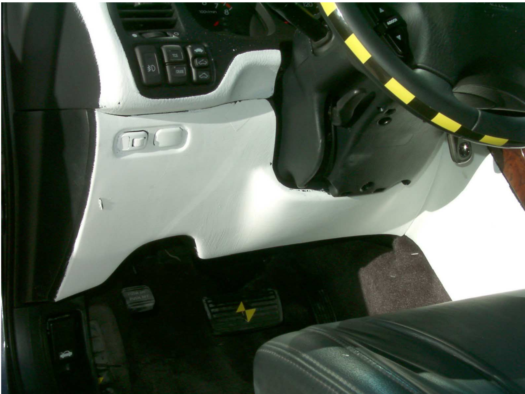
Figure A-35: Driver Side Knee Bolster, Pre-Test
