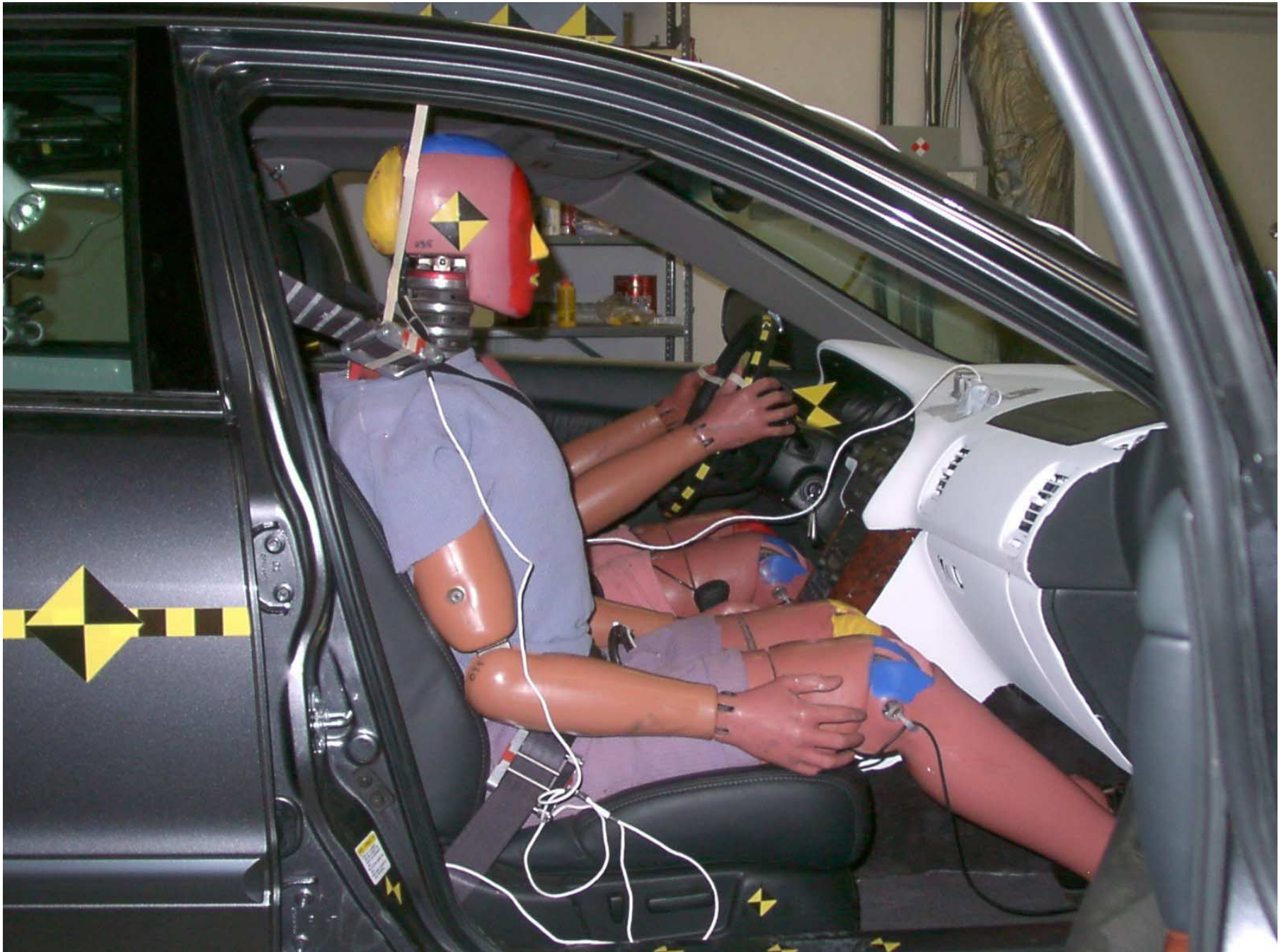
Figure A-47: Passenger Dummy 90° To Vehicle, Pre-Test
