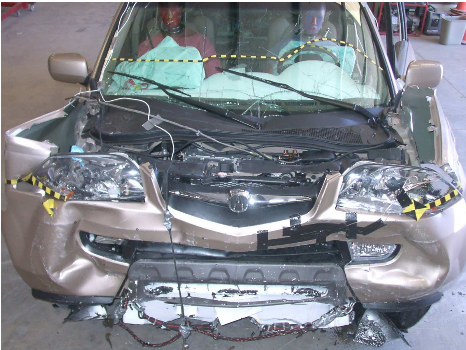
Figure A-18: Engine Compartment, Post-Test
