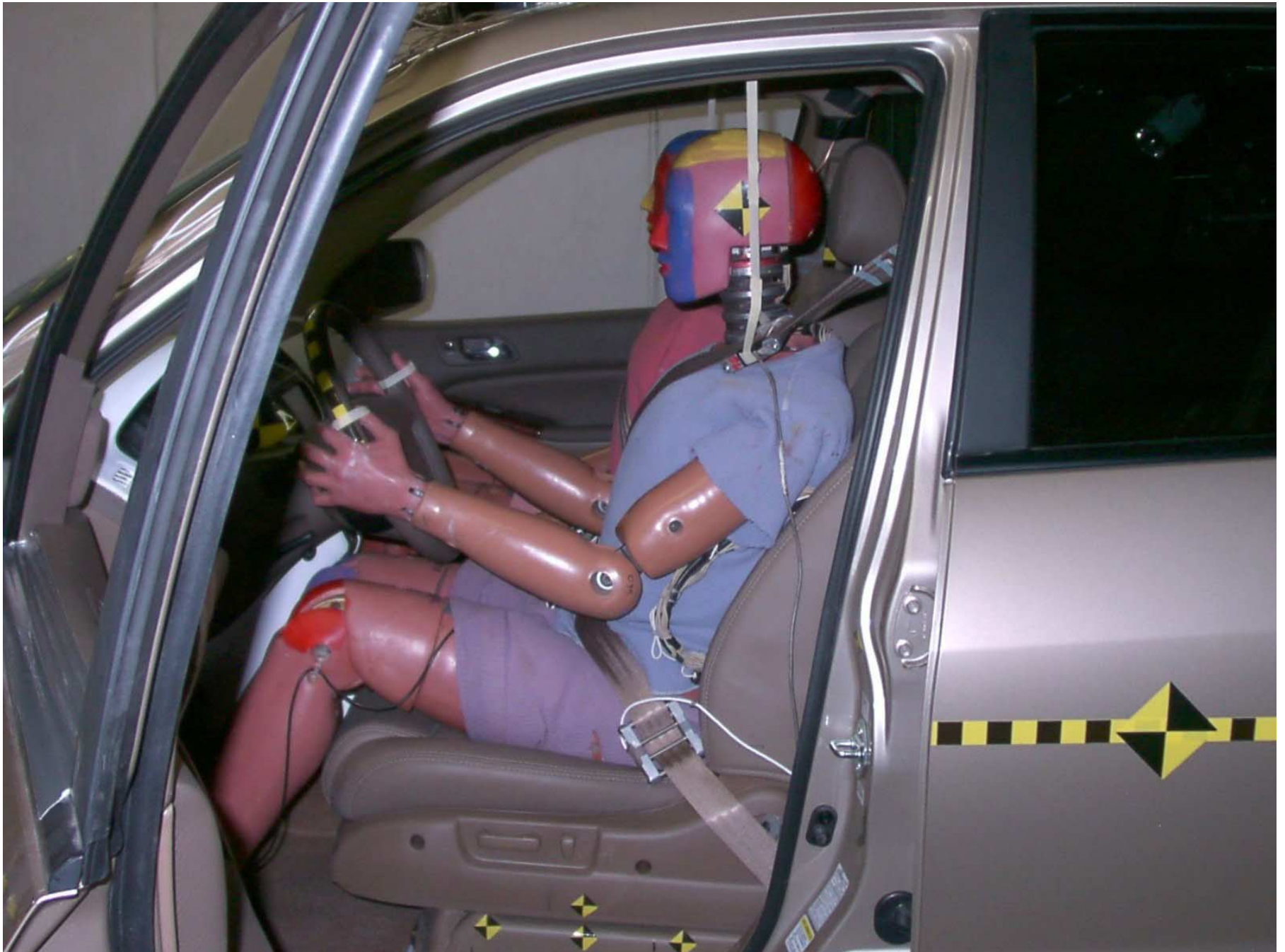
Figure A-31: Driver Dummy 90° To Vehicle, Pre-Test
