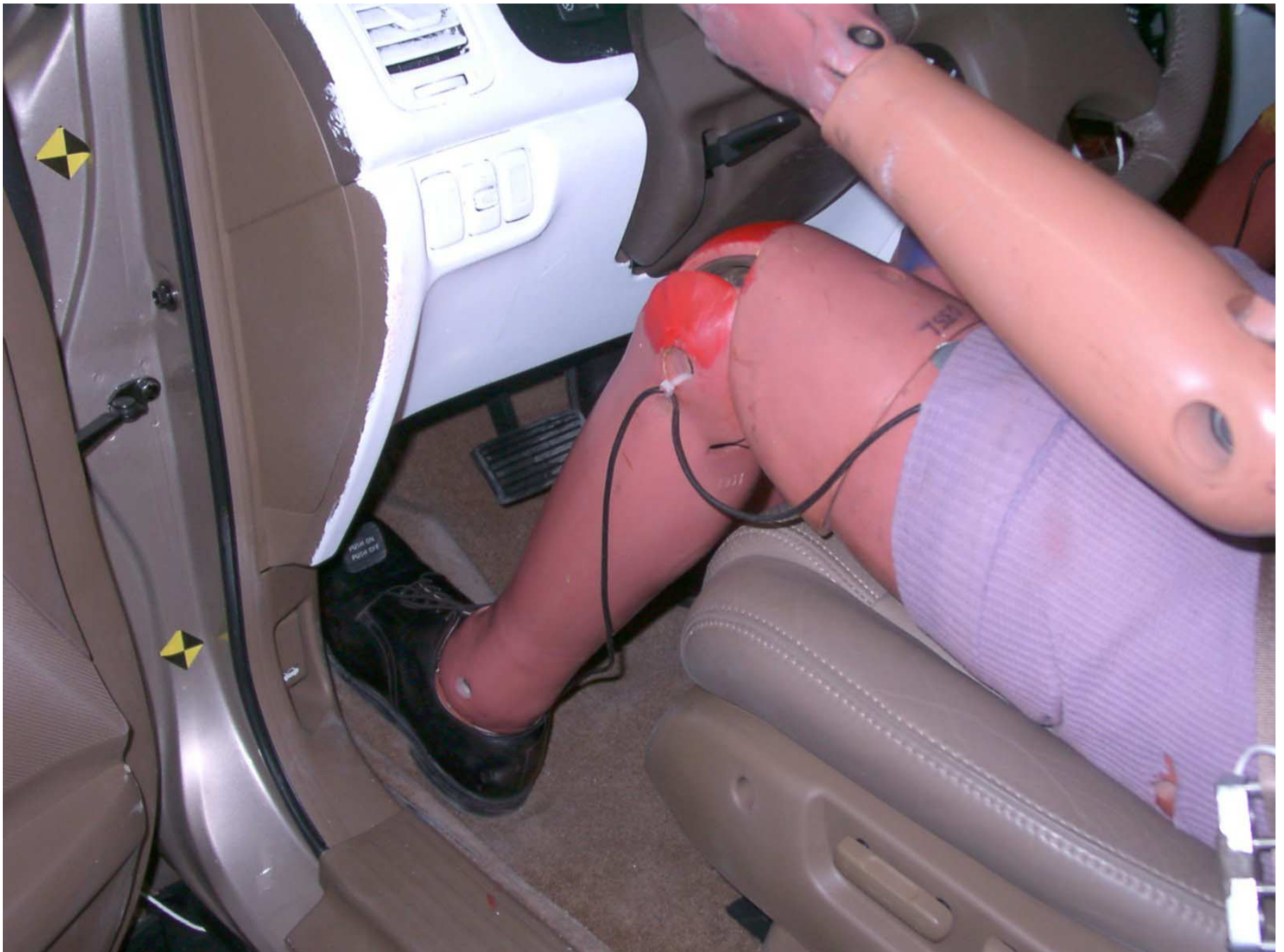
Figure A-33: Driver Dummy Feet, Pre-Test
