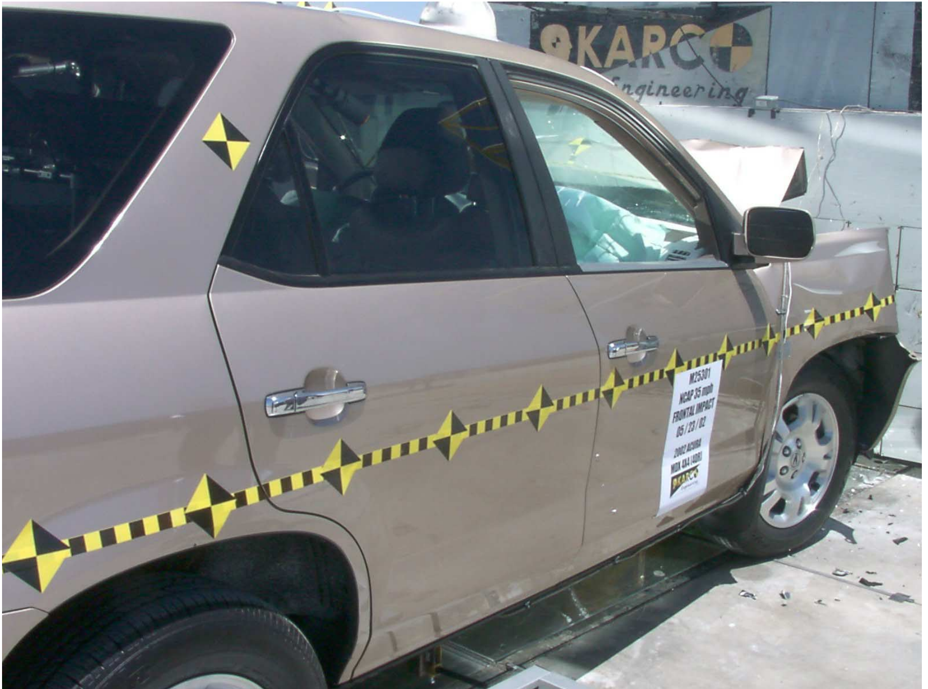
Figure A-58: \frac{3}{4} Right Rear View of Doors After Impact
