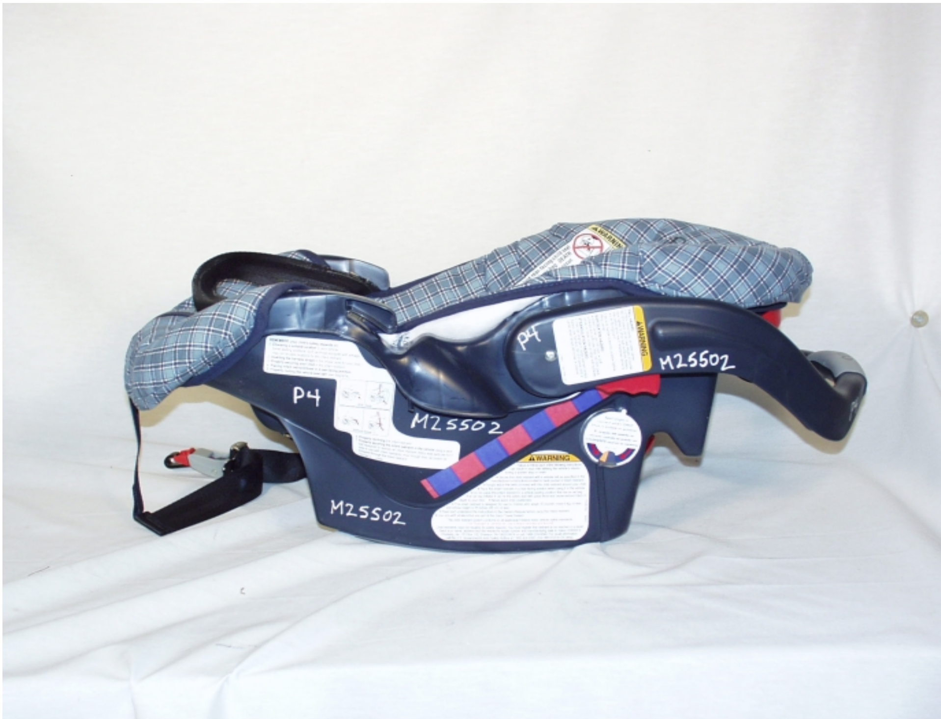
Figure 3-16 POST-TEST LEFT SIDE VIEW OF POSITION 4 CRS
