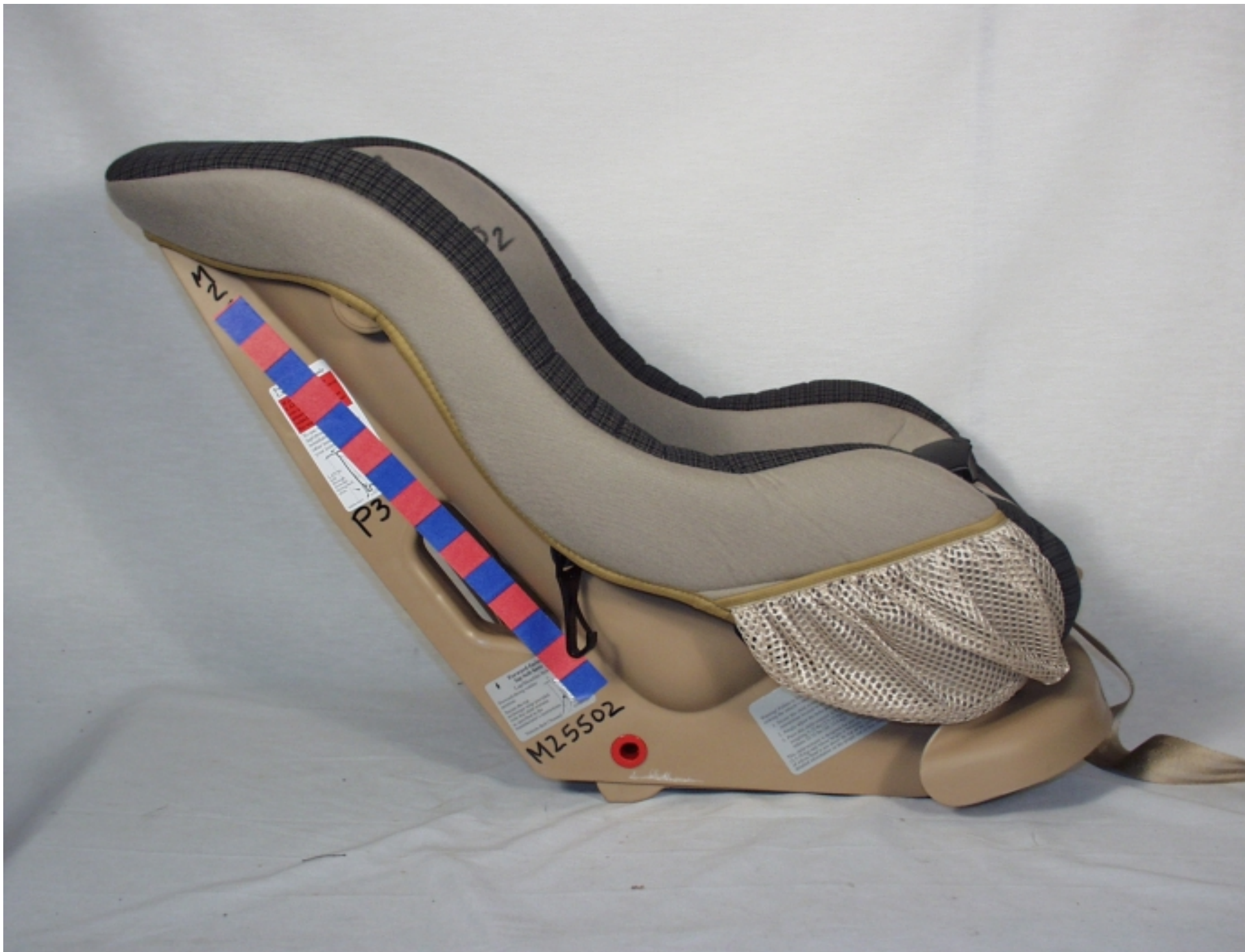
Figure 3-9 POST-TEST RIGHT SIDE VIEW OF POSITION 3 CRS
