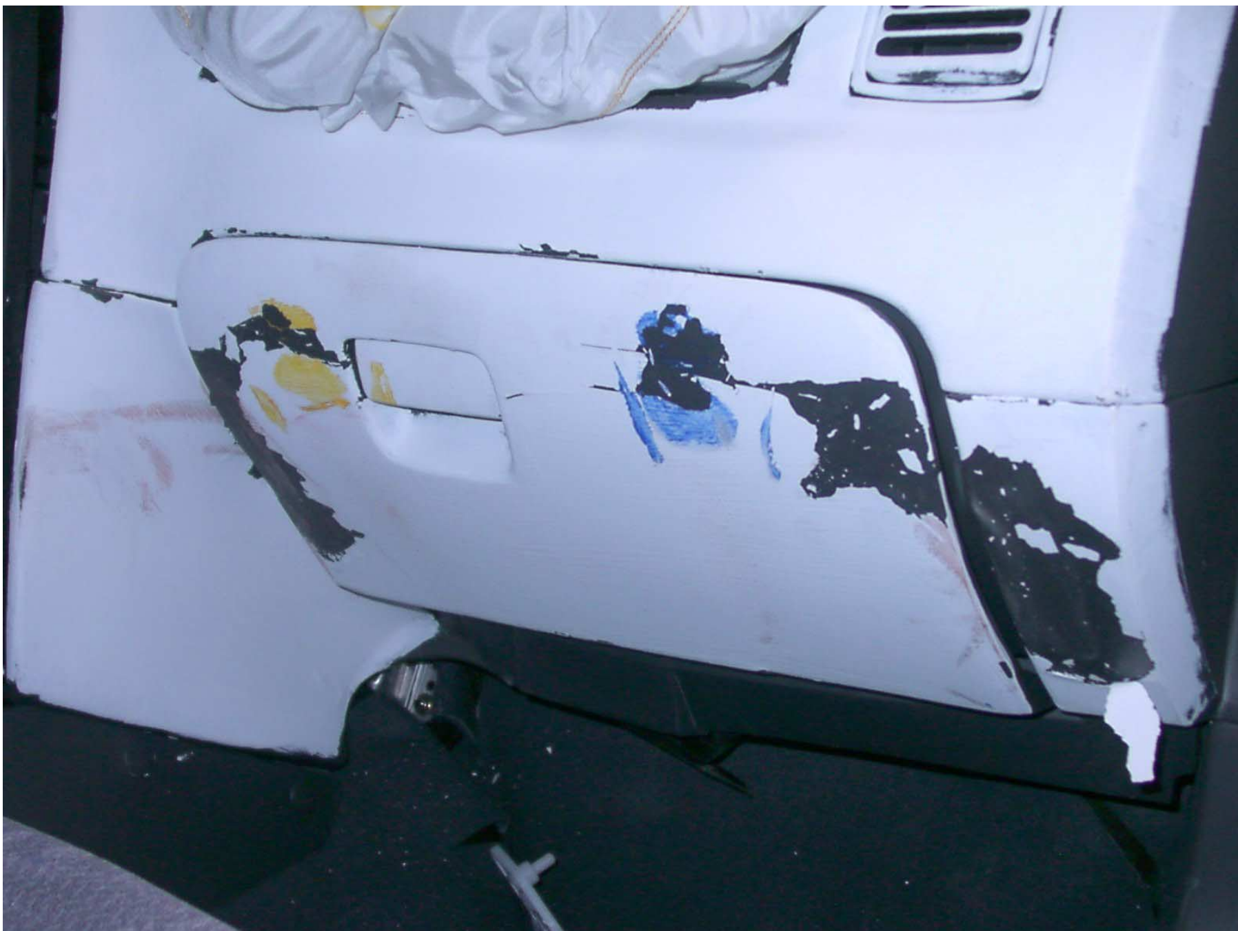
Figure A-54: Passenger Side Knee Bolster, Post-Test
