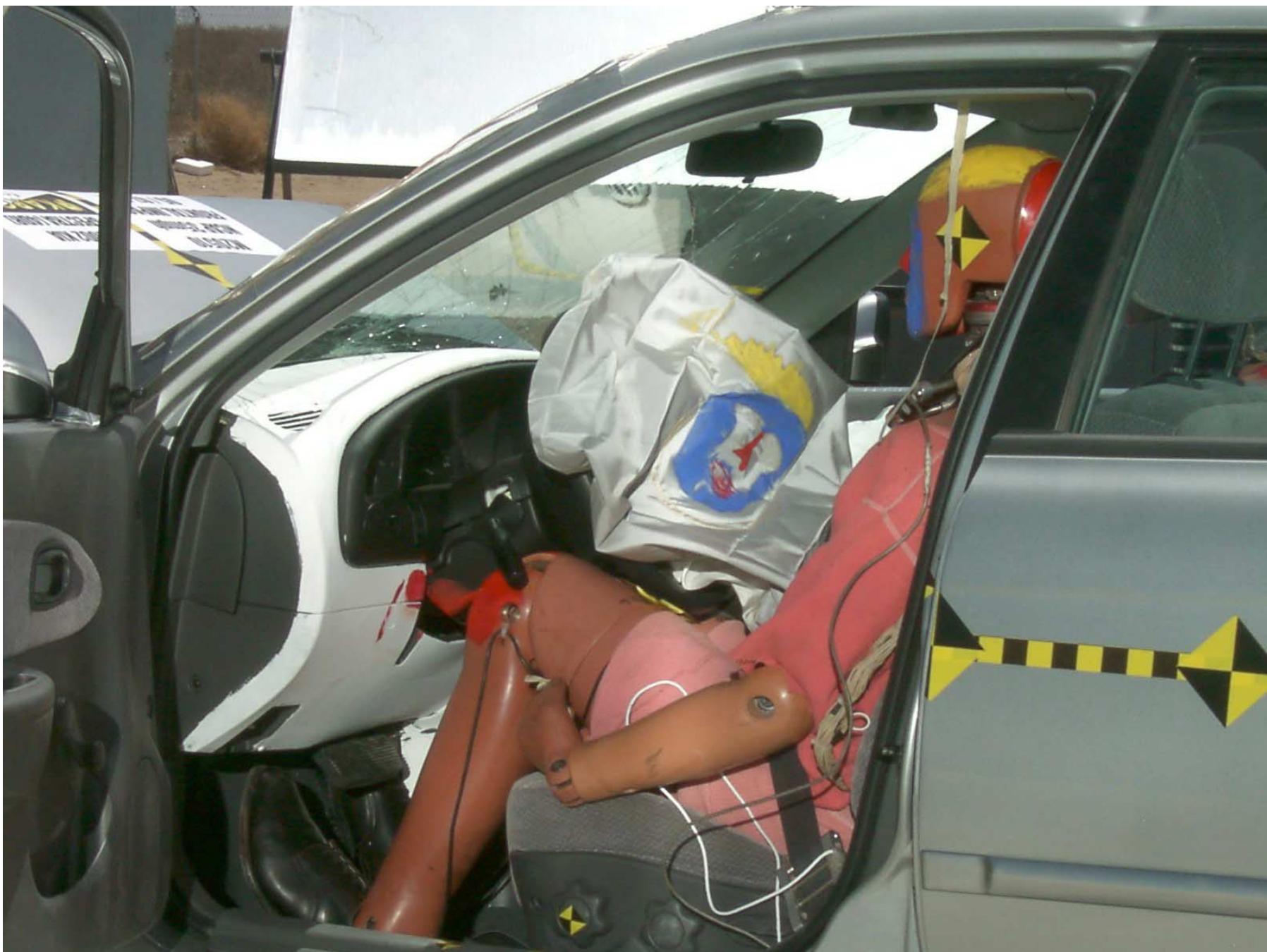
Figure A-30: Driver Dummy Door Open, Post-Test
