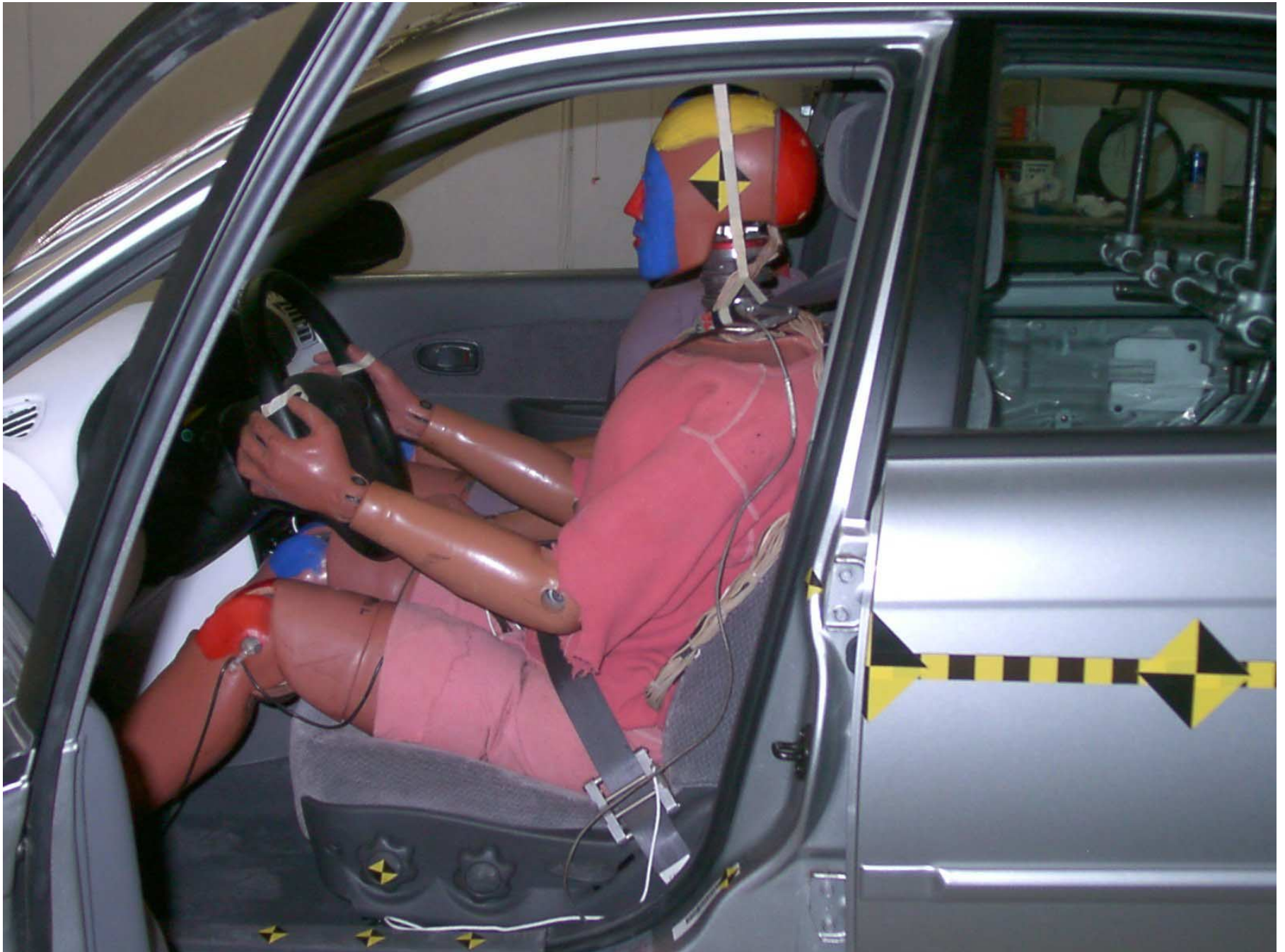
Figure A-31: Driver Dummy 90° To Vehicle, Pre-Test
