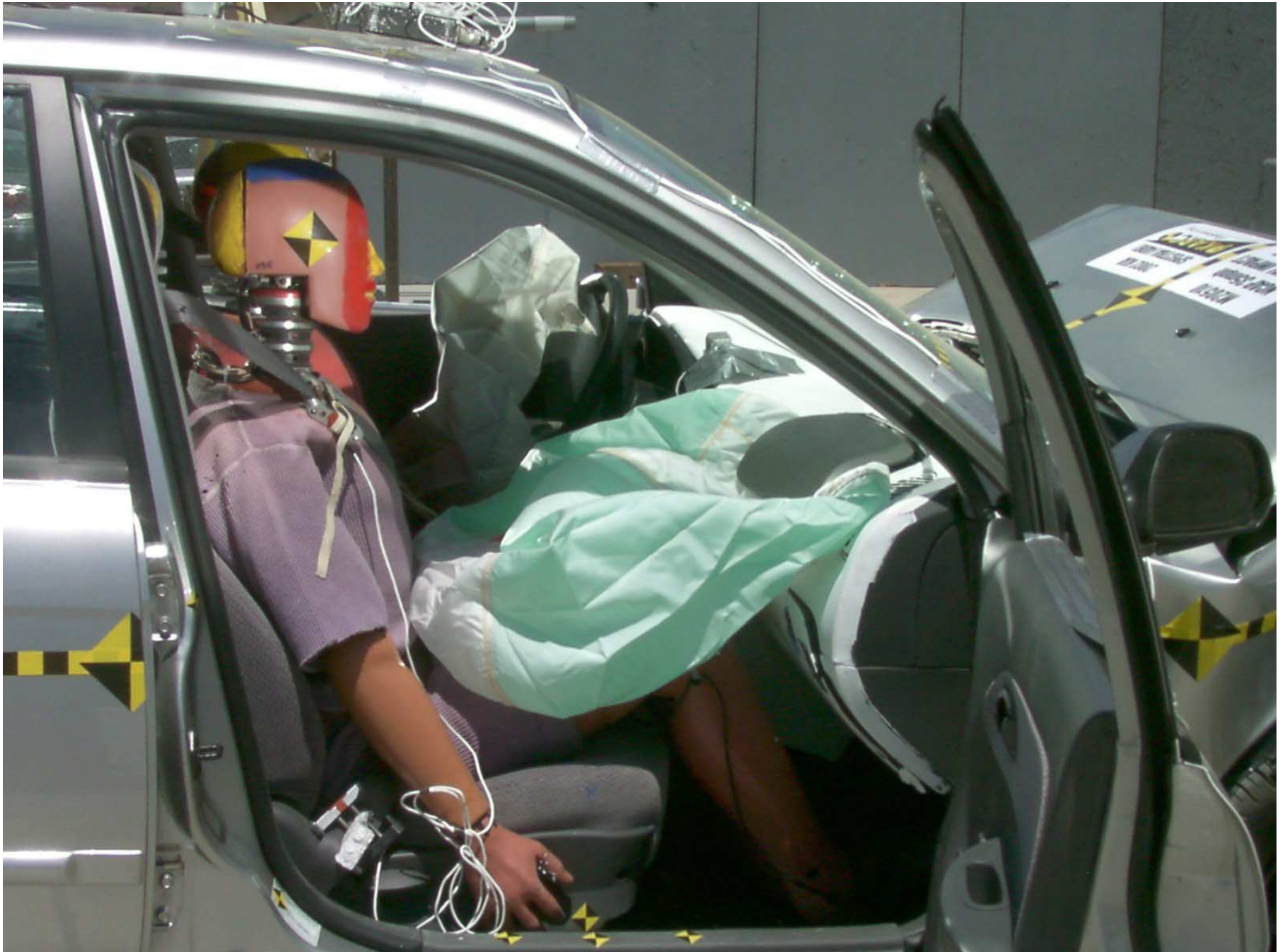
Figure A-48: Passenger Dummy 90° To Vehicle, Post-Test
