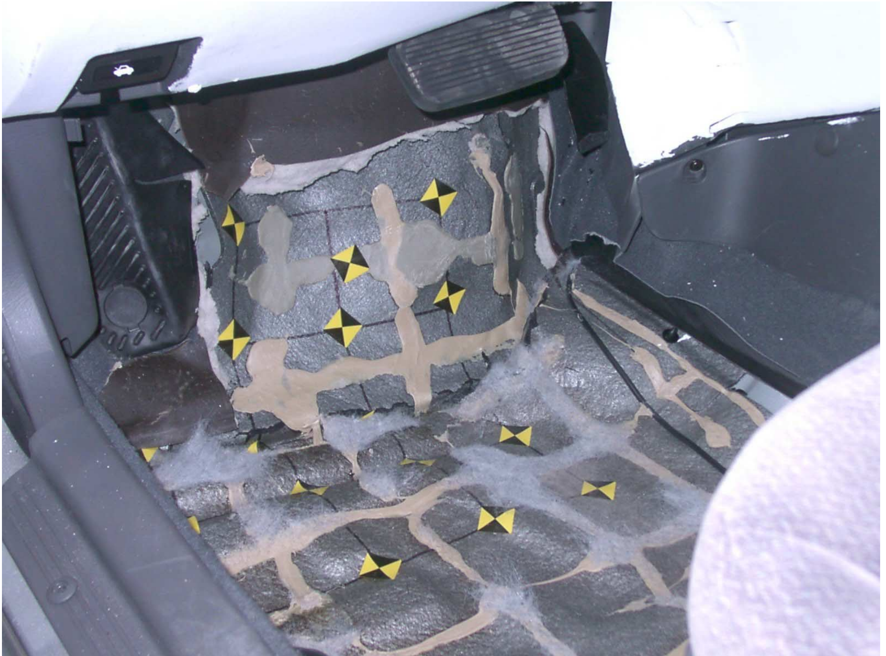
Figure A-38: Driver Side Floor Pan, Post-Test
