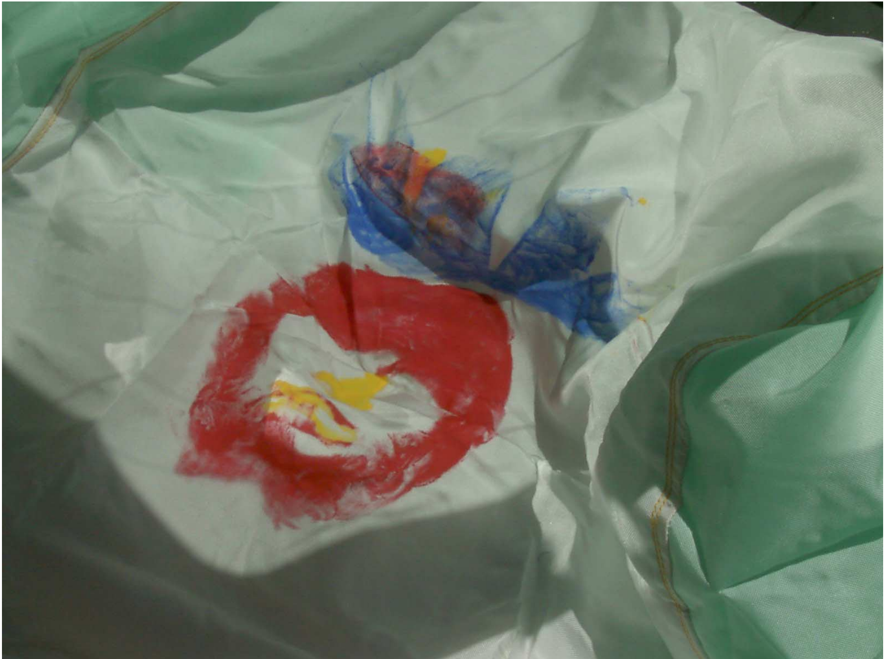
Figure A-56: Passenger Dummy Contact, Post-Test
