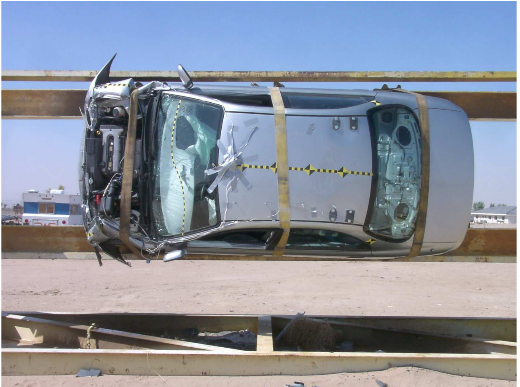
Figure A-59: Vehicle on Rollover Device
