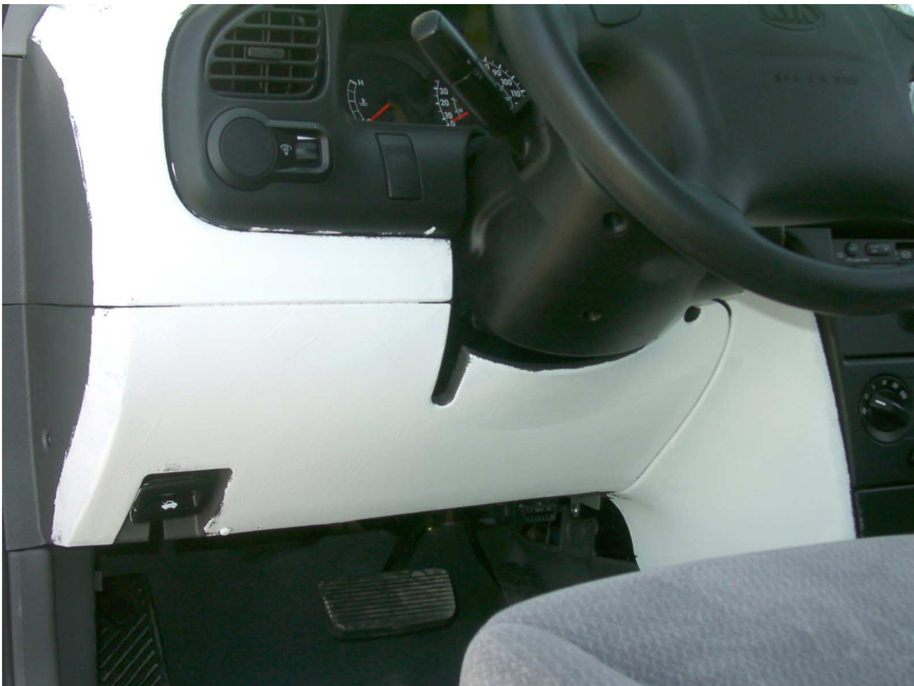
Figure A-35: Driver Side Knee Bolster, Pre-Test
