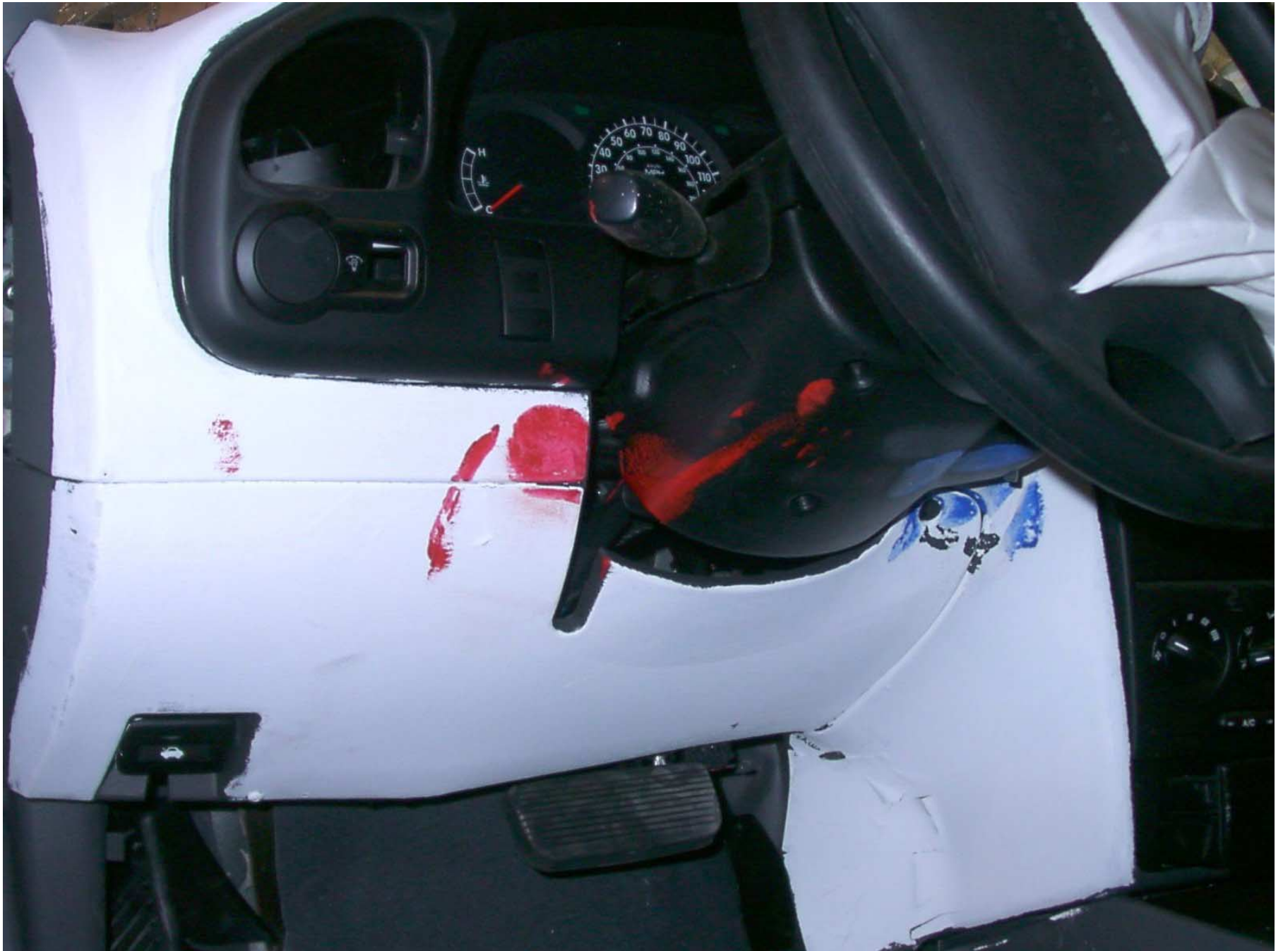
Figure A-36: Driver Side Knee Bolster, Post-Test
