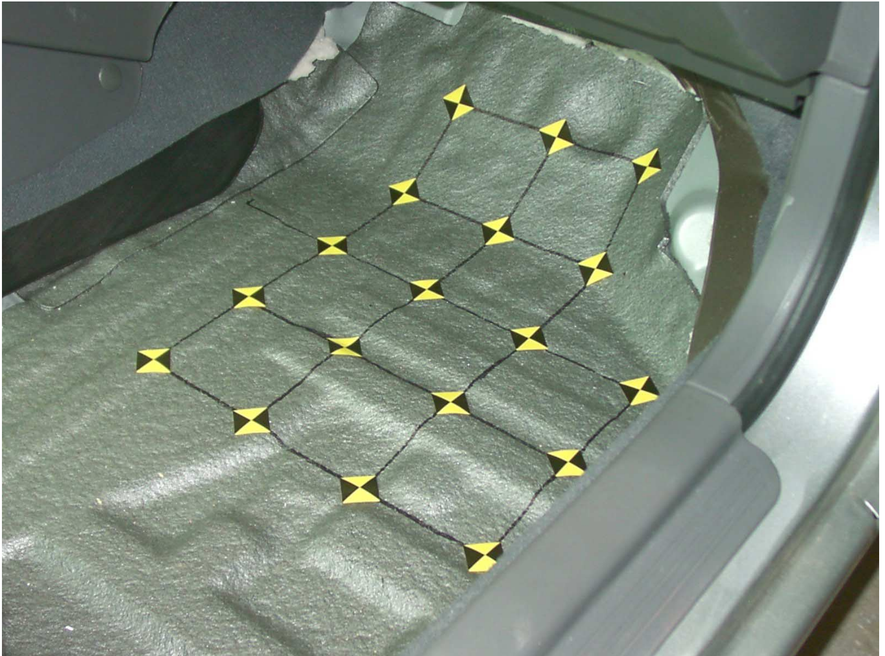
Figure A-51: Passenger Side Floor Pan, Pre-Test
