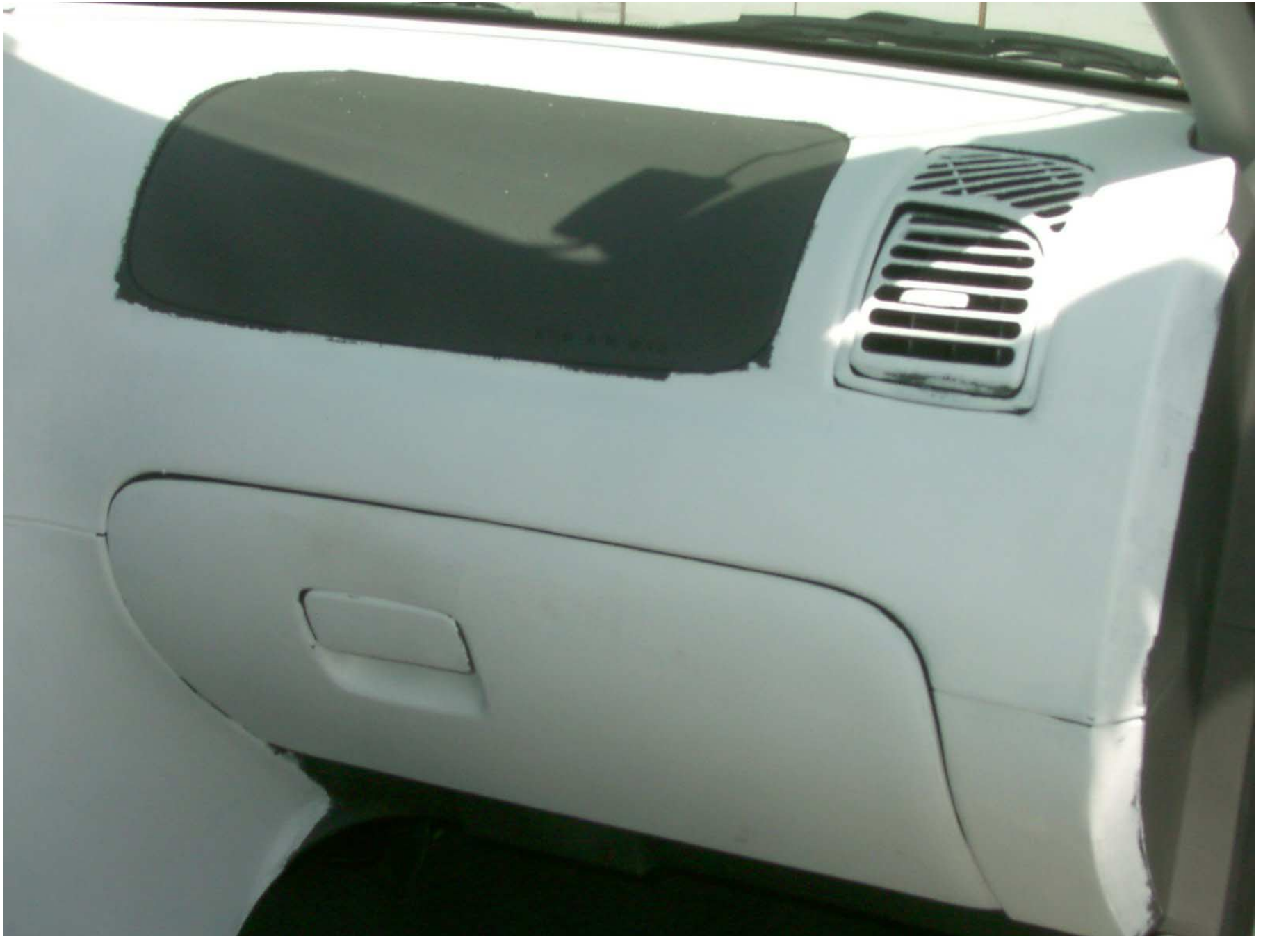
Figure A-53: Passenger Side Knee Bolster, Pre-Test
