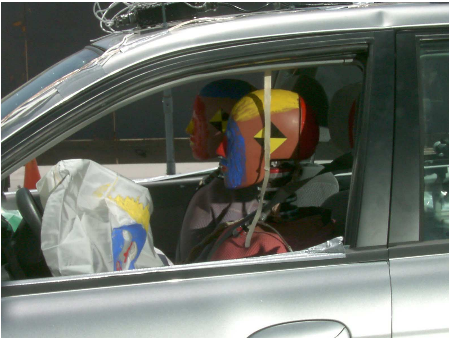
Figure A-28: Driver Dummy Through Window, Post-Test
