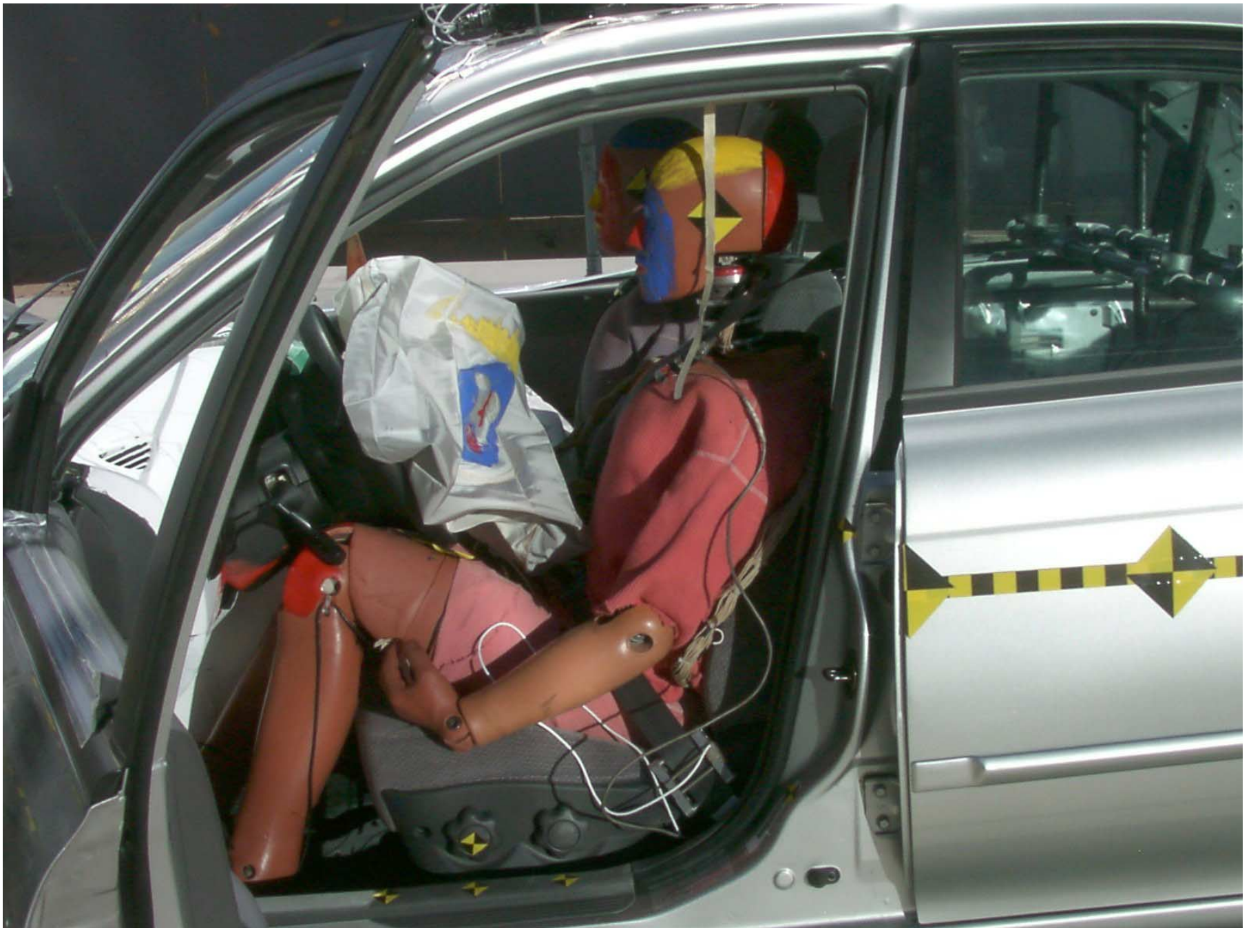
Figure A-32: Driver Dummy 90° To Vehicle, Post-Test
