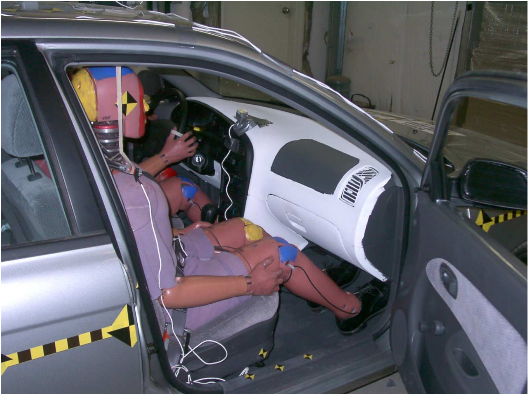
Figure A-45: Passenger Dummy Door Open, Pre-Test
