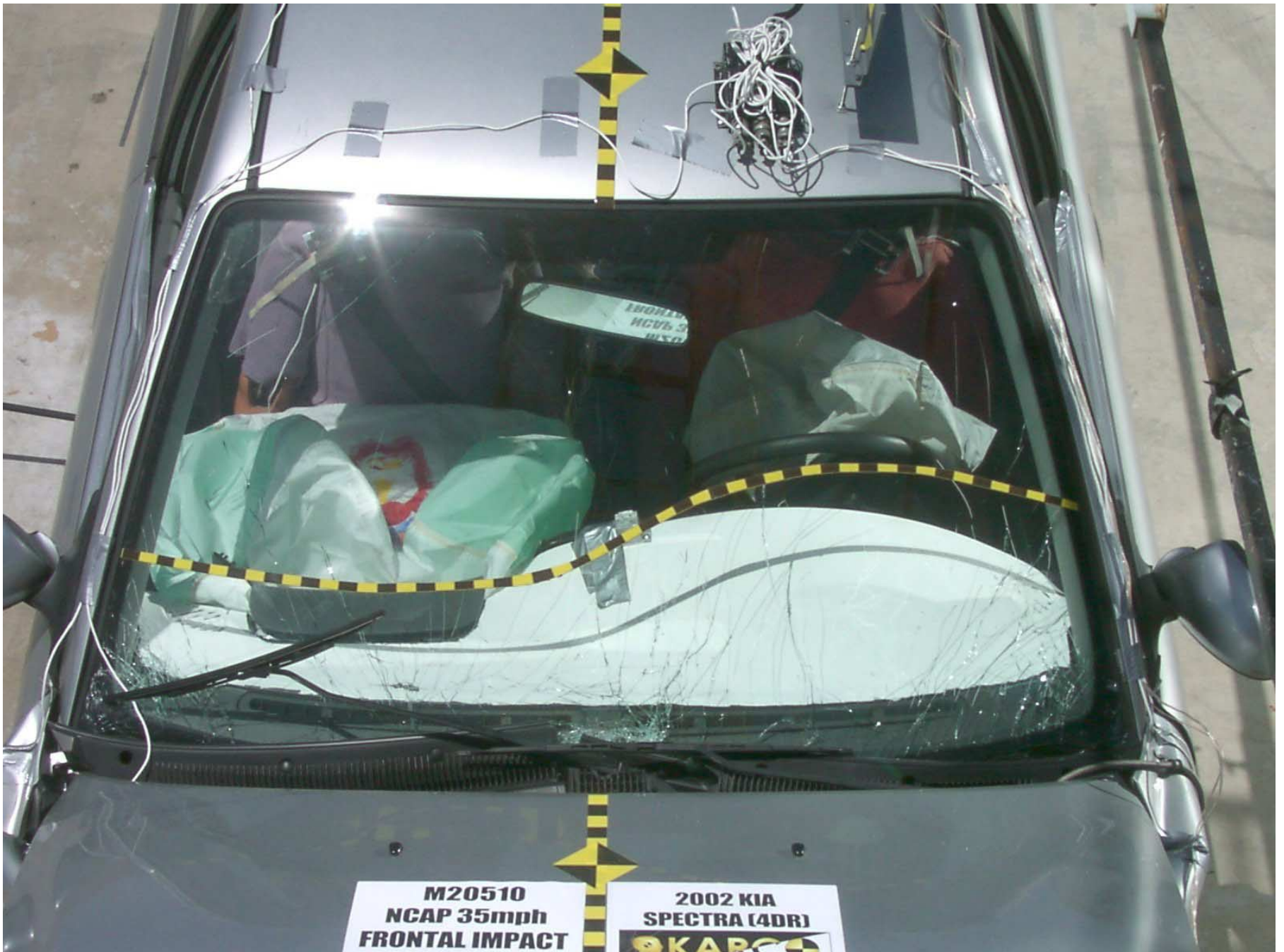
Figure A-16: Windshield, Post-Test
